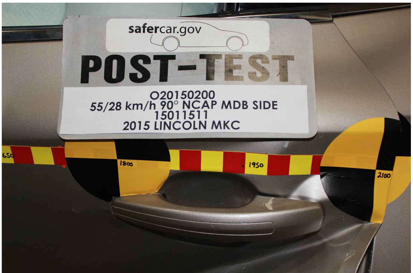
Post-Test Left Rear Door Latch Close-Up
