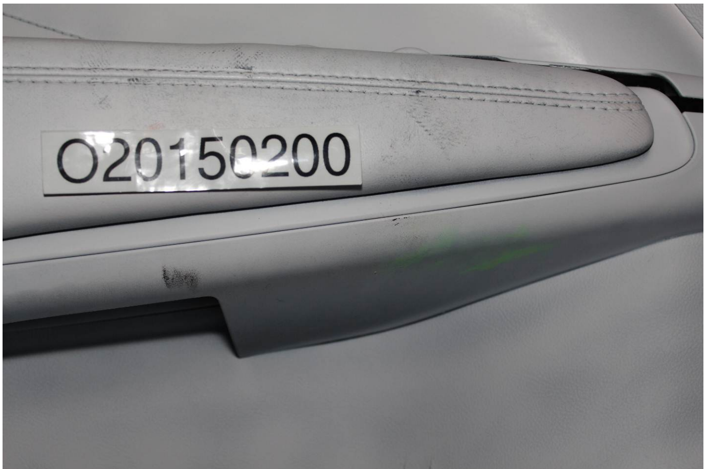
Post-Test Driver Dummy Close-up Knee Contact View
