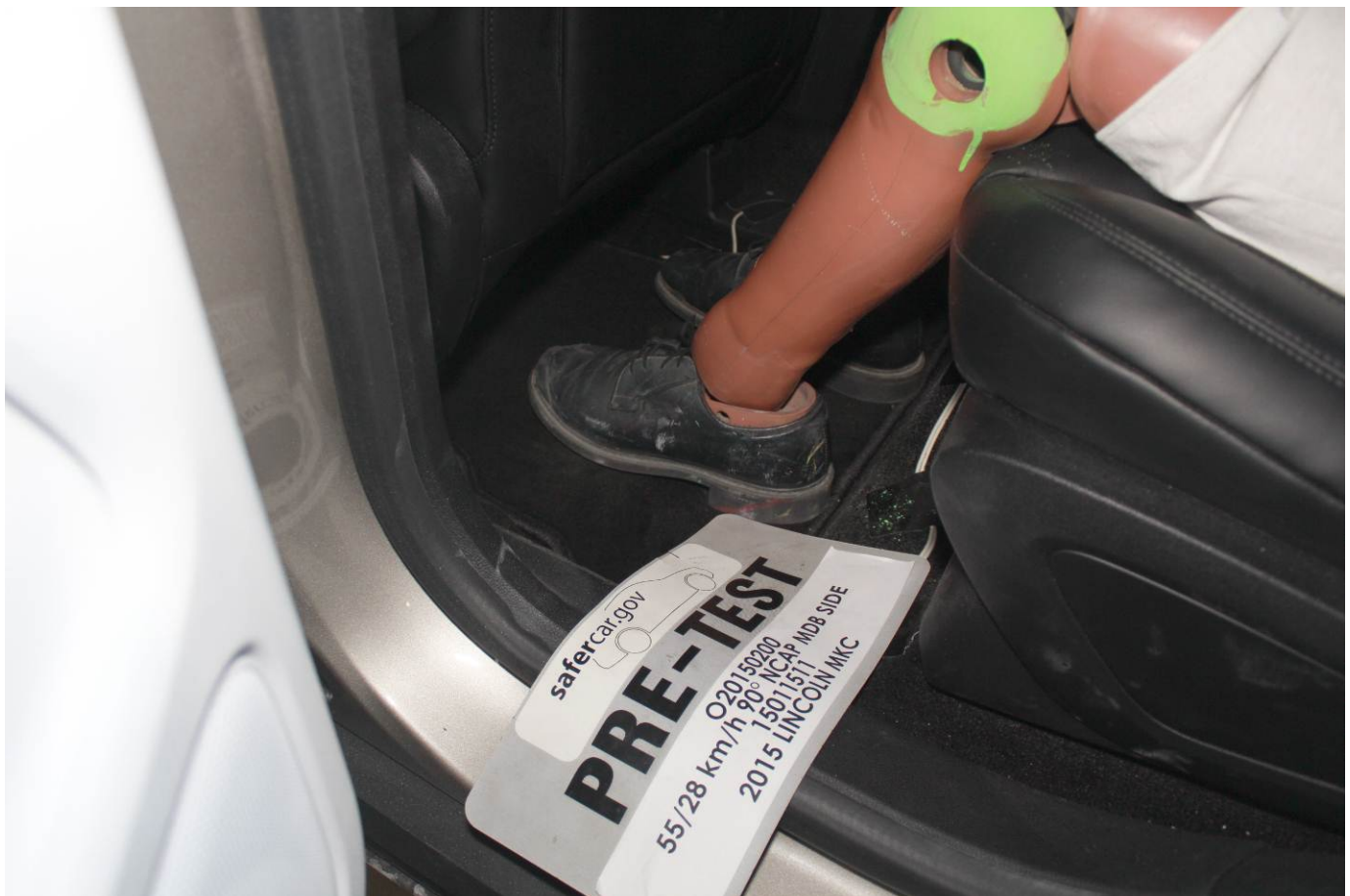
Pre-Test Placement of Rear Passenger Dummy's Feet
