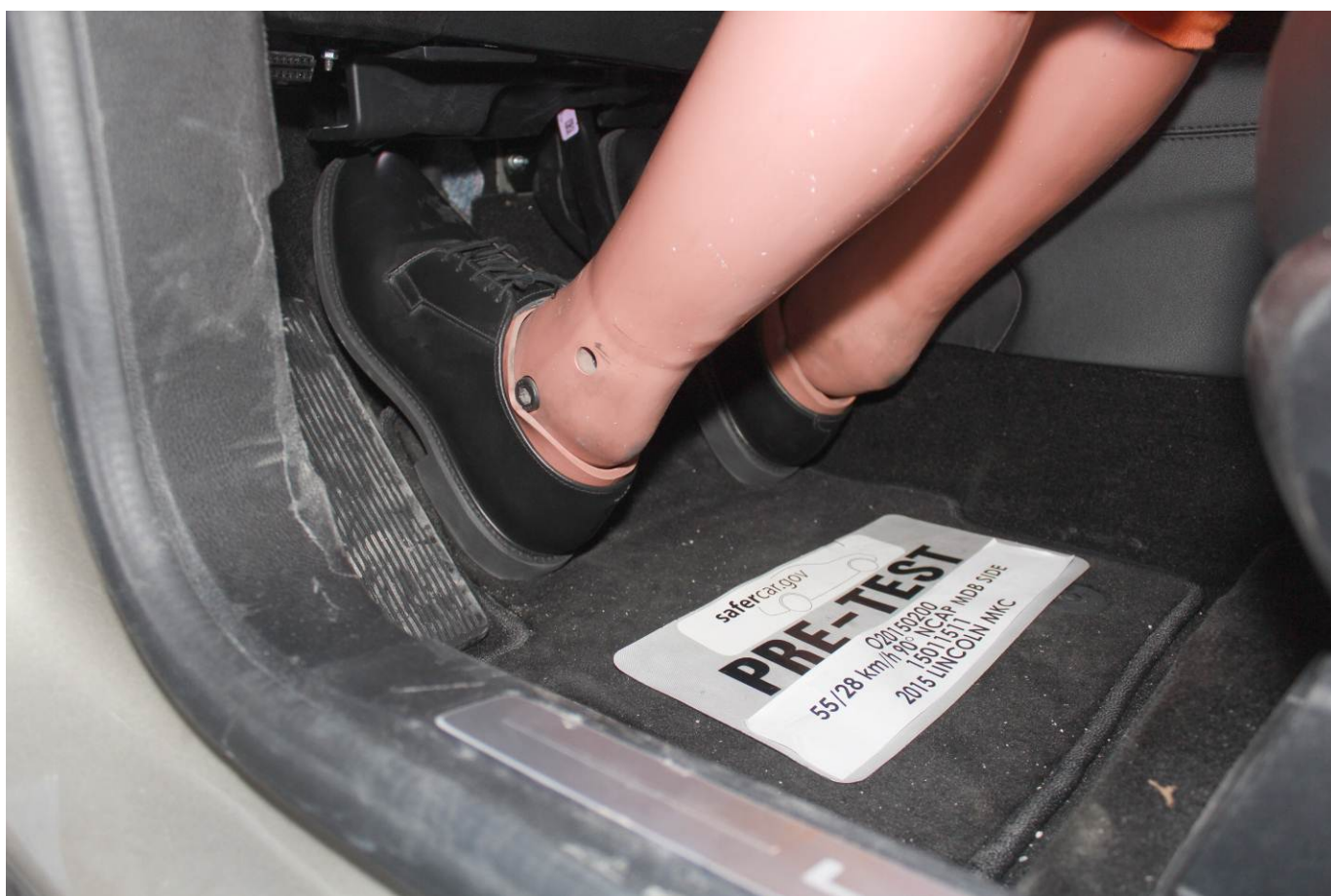
Pre-Test Placement of Driver Dummy's Feet
