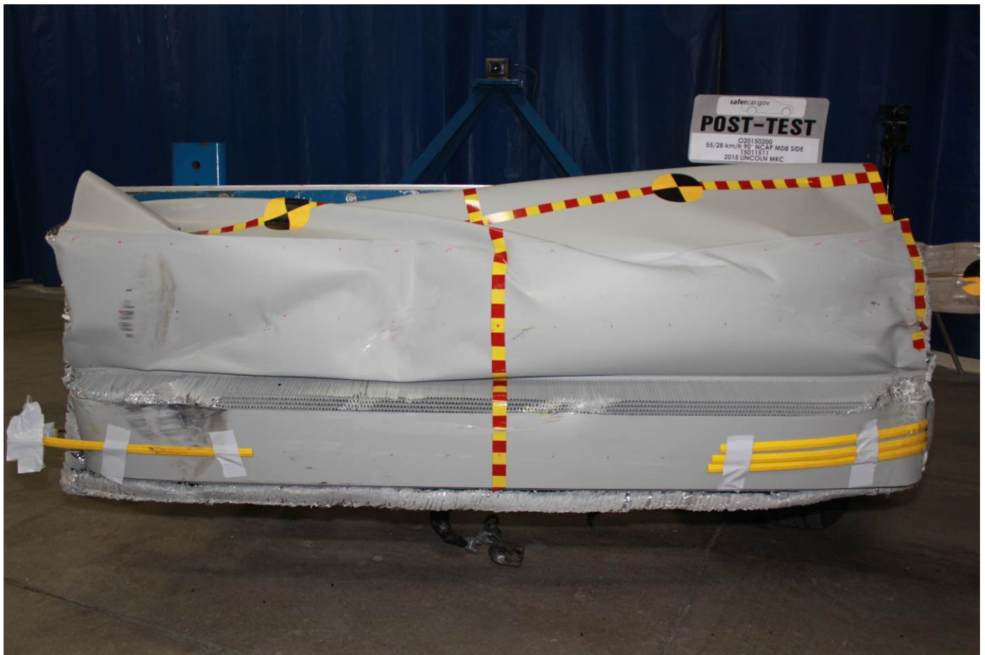
Post-Test Front View of MDB Impactor Face
