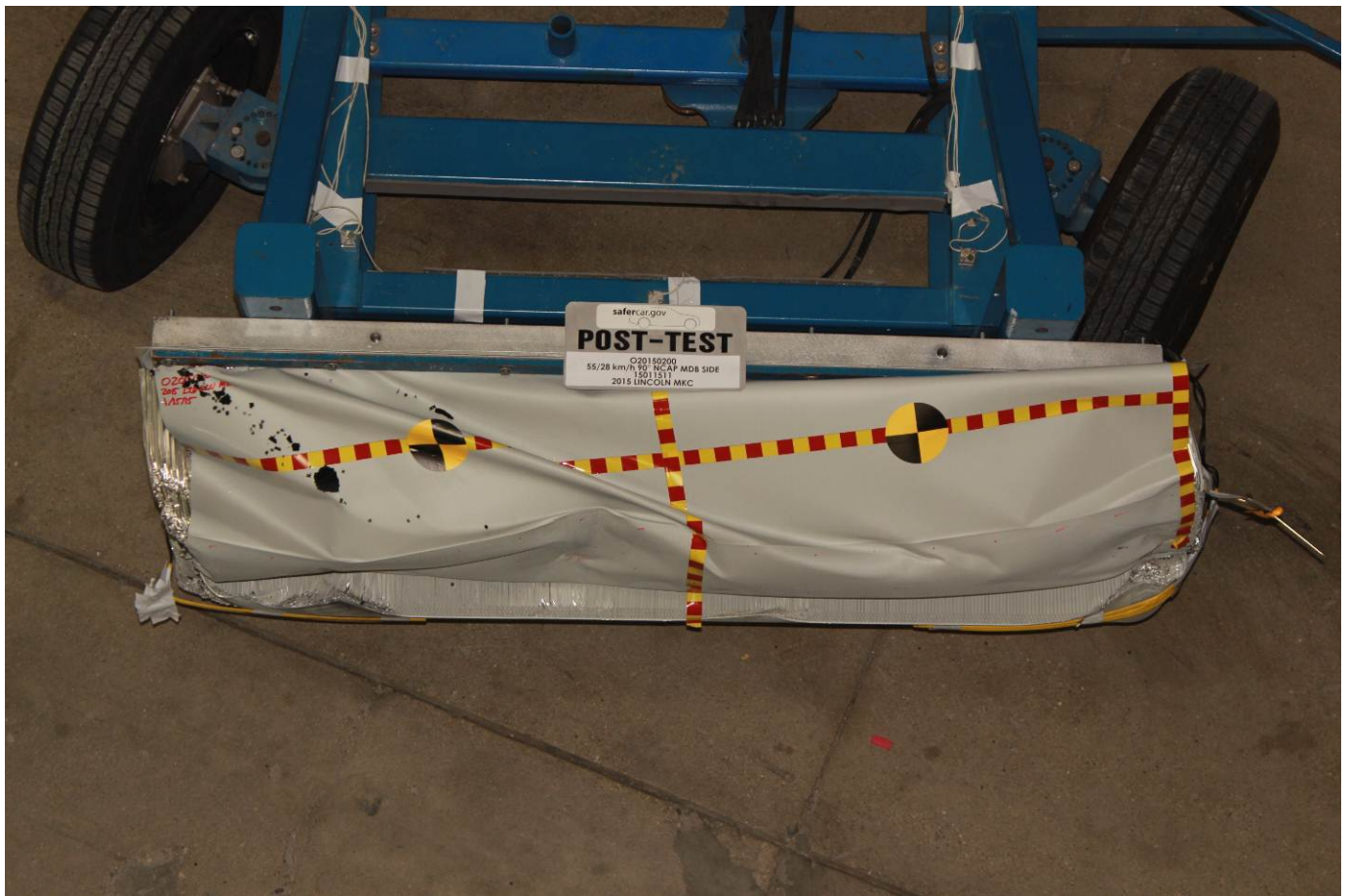
Post-Test Top View of MDB Impactor Face
