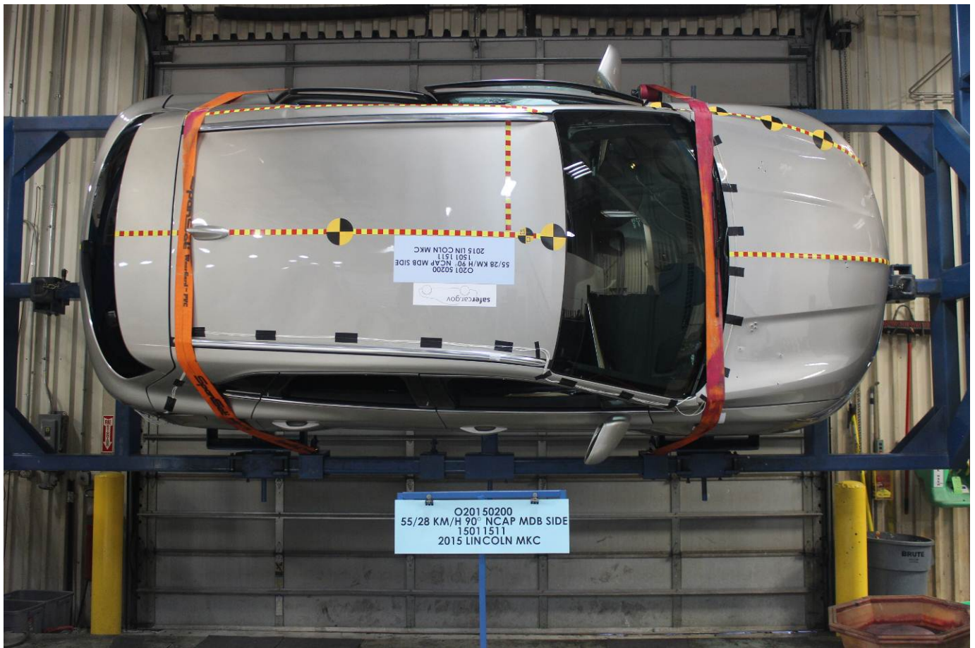
FMVSS No. 301 Static Rollover 90 Degrees
