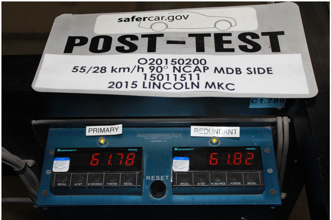
Post-Test Primary and Redundant Speed Trap Read-Out
