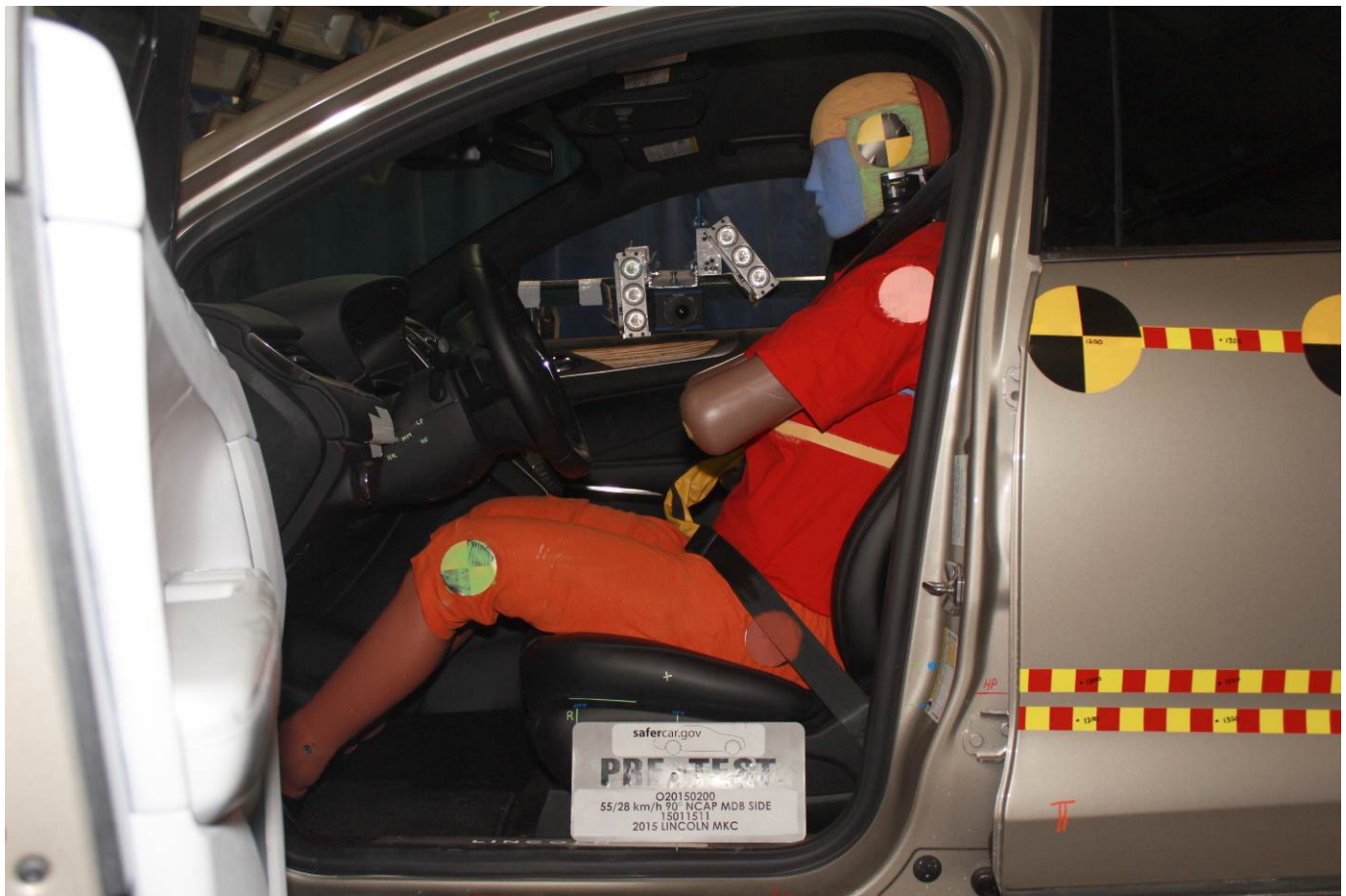
Pre-Test Left Side View of Driver Dummy Showing Belt and Chalking
