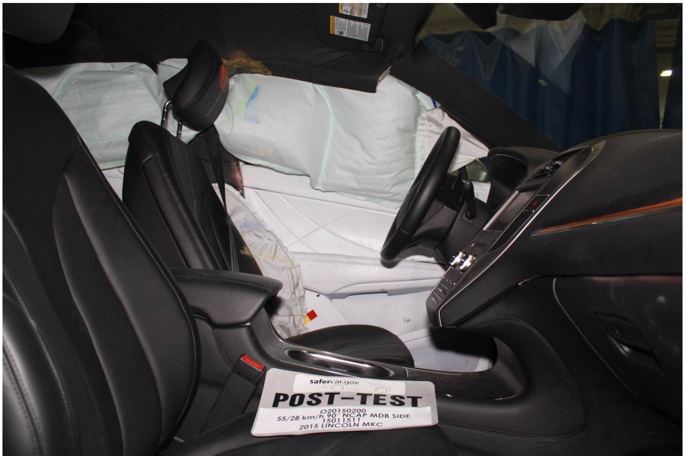
Post-Test Driver Inner Door Panel View
