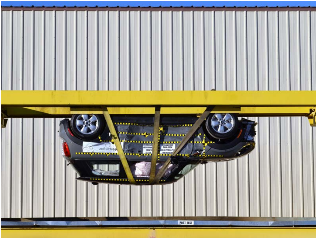
FIGURE 98. FMVSS No. 301 Static Rollover 180 Degrees
