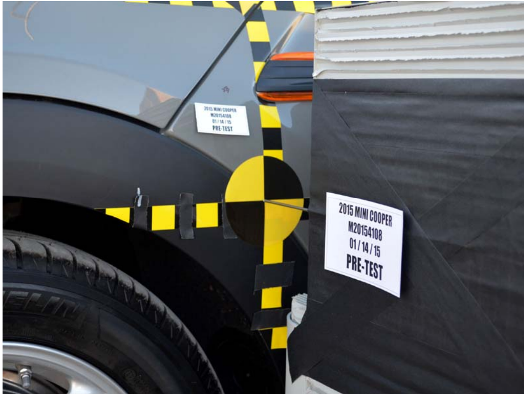
FIGURE 19. Pre-Test Close-Up View of Impact Point Target
