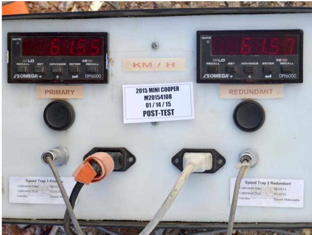
FIGURE 95. Post-Test Primary and Redundant Speed Trap Read-Out
