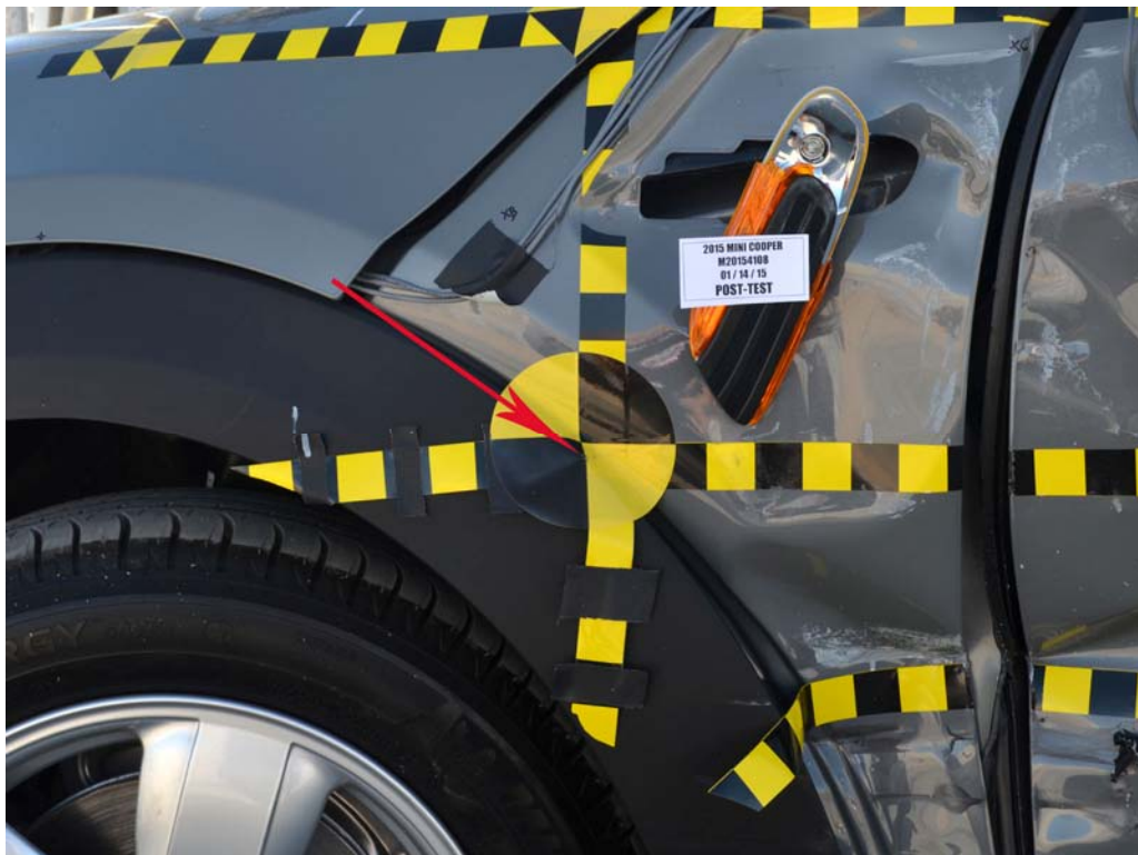
FIGURE 20. Post-Test Close-Up View of Impact Point Target
