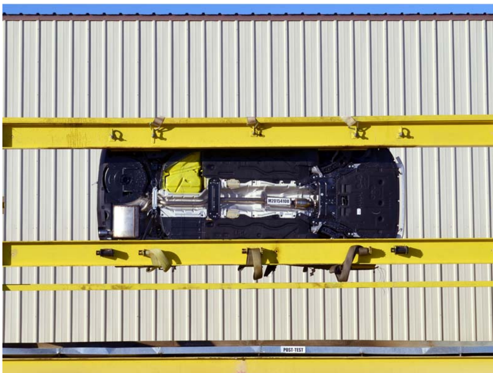
FIGURE 99. FMVSS No. 301 Static Rollover 270 Degrees
