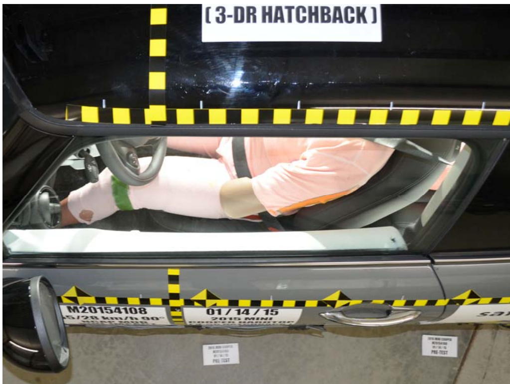
FIGURE 42. Pre-Test Driver Dummy and Door Clearance View
