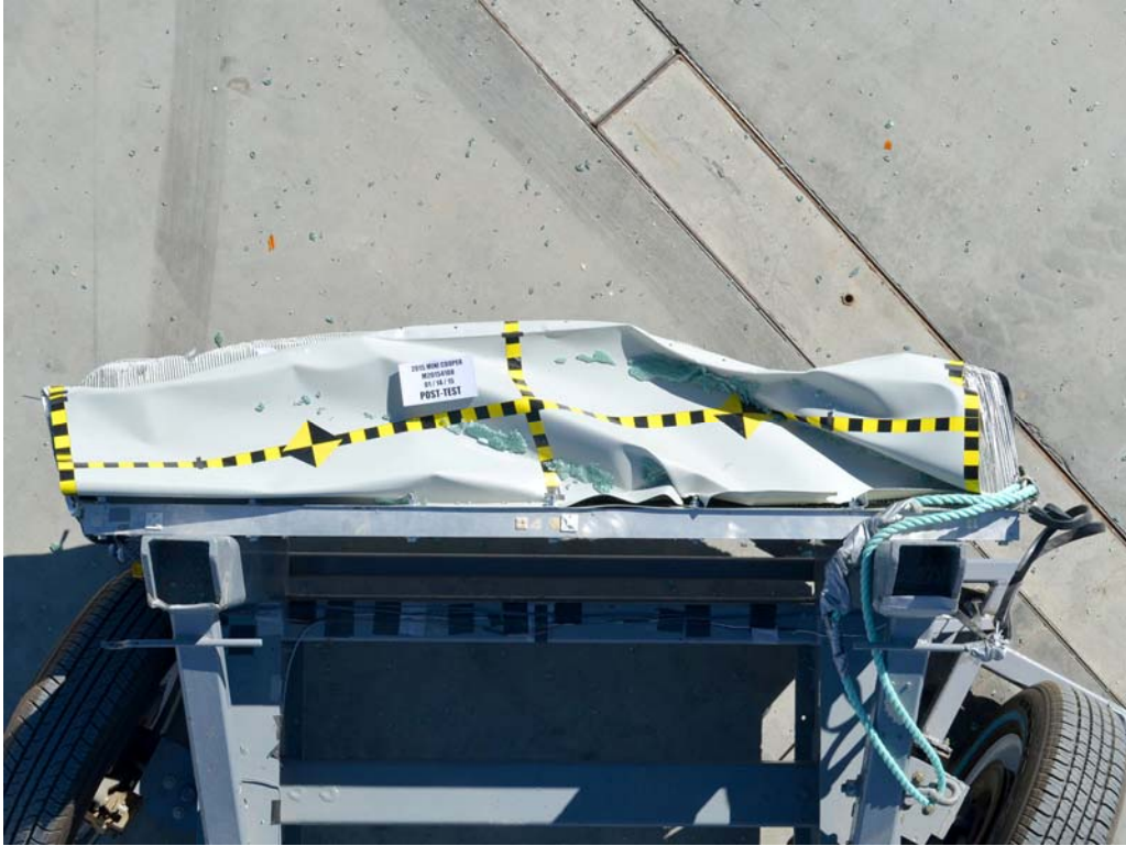
FIGURE 87. Post-Test Top View of MDB Impactor Face
