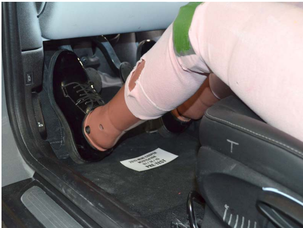
FIGURE 34. Pre-Test Placement of Driver Dummy's Feet
