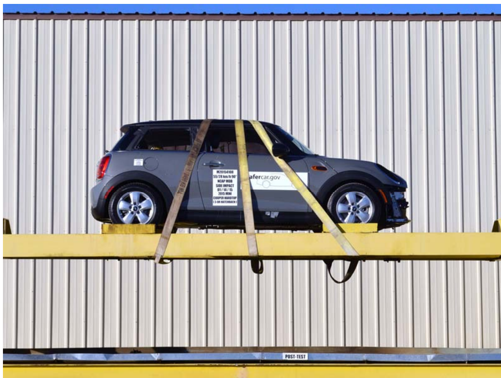
FIGURE 96. FMVSS No. 301 Static Rollover 0 Degrees
