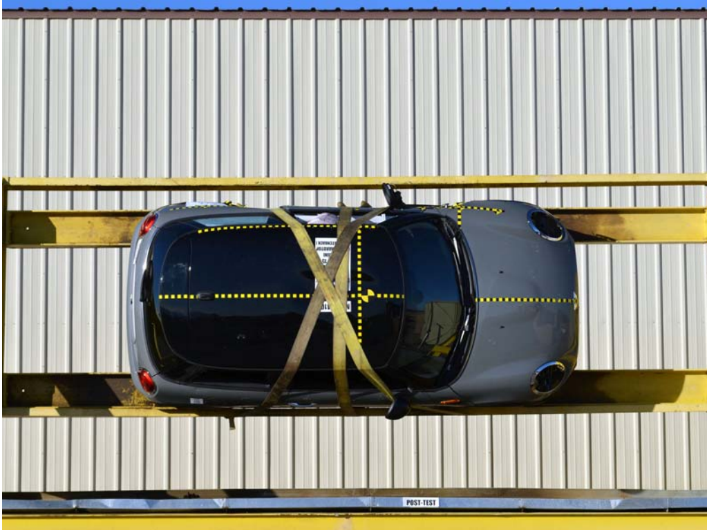
FIGURE 97. FMVSS No. 301 Static Rollover 90 Degrees
