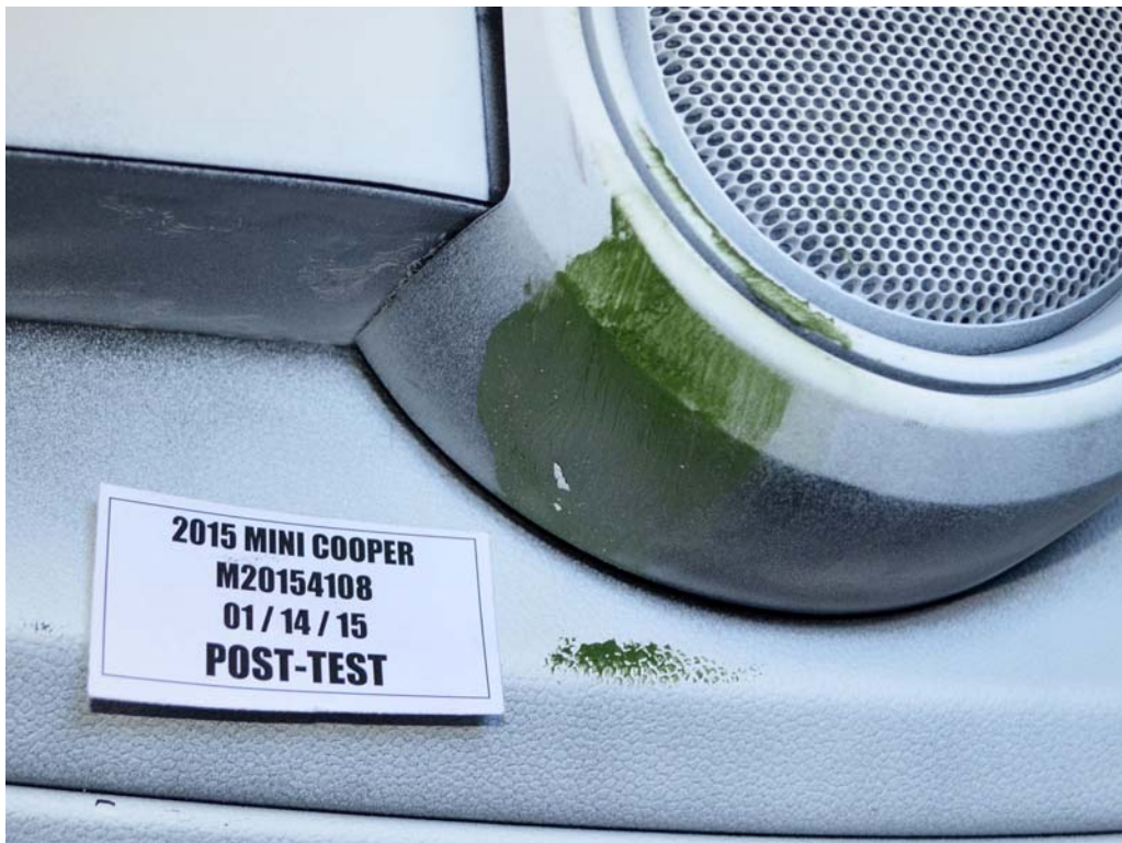
FIGURE 54. Post-Test Driver Dummy Close-Up Knee Contact View
