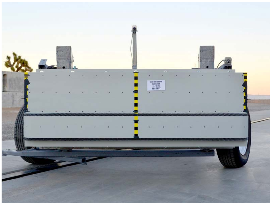
FIGURE 84. Pre-Test Front View of MDB Impactor Face
