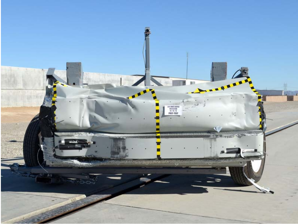
FIGURE 85. Post-Test Front View of MDB Impactor Face
