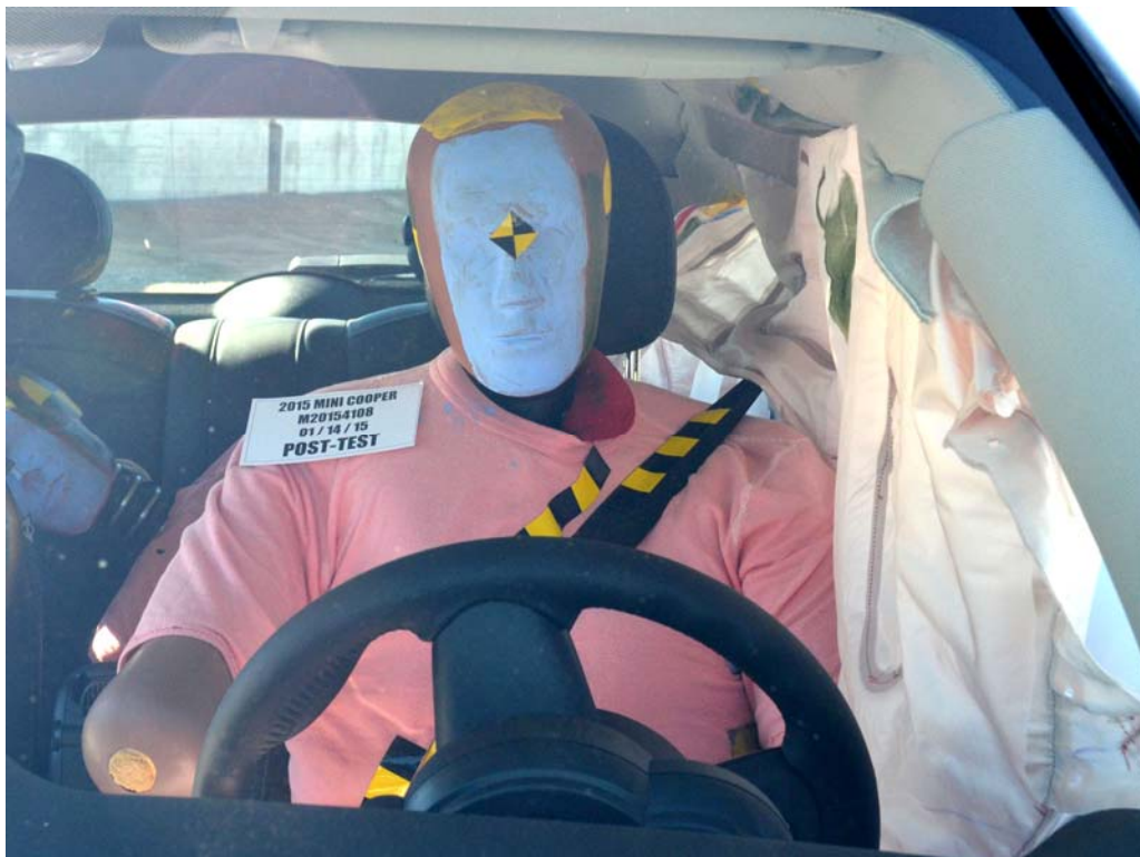
FIGURE 26. Post-Test Front Close-Up View of Driver Dummy
