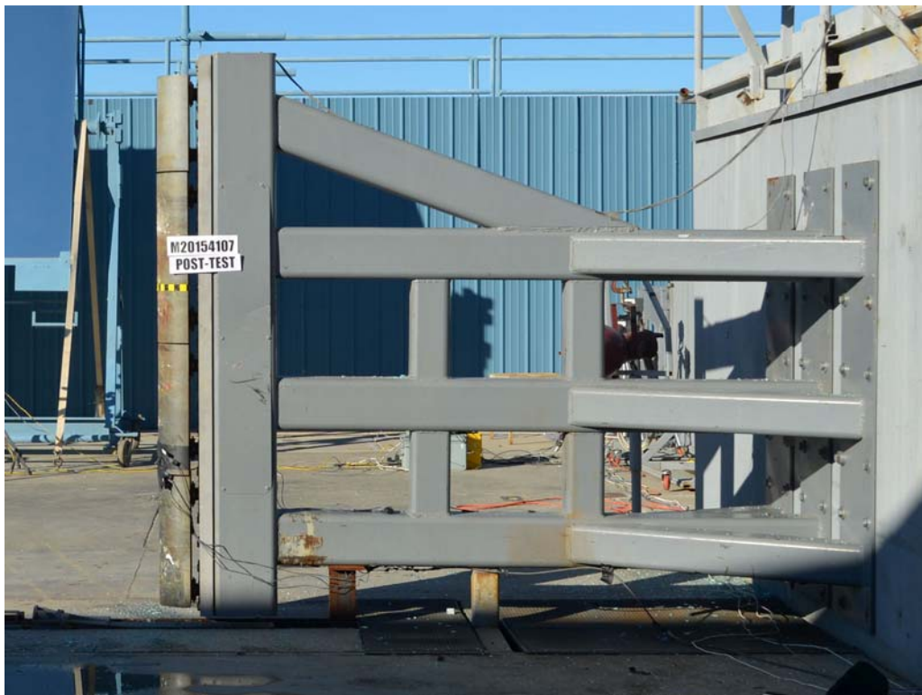
FIGURE 60. Post-Test Pole Barrier Side View
