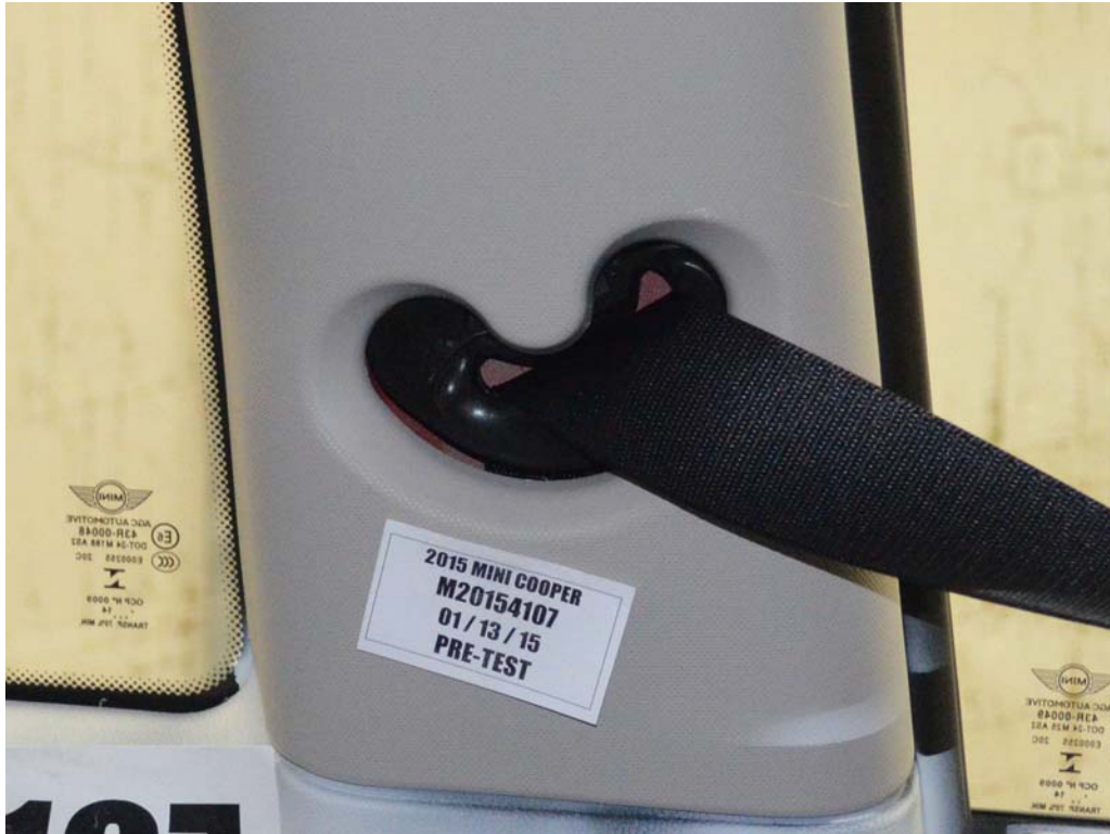
FIGURE 33. Pre-Test View of Belt Anchorage for Dummy
