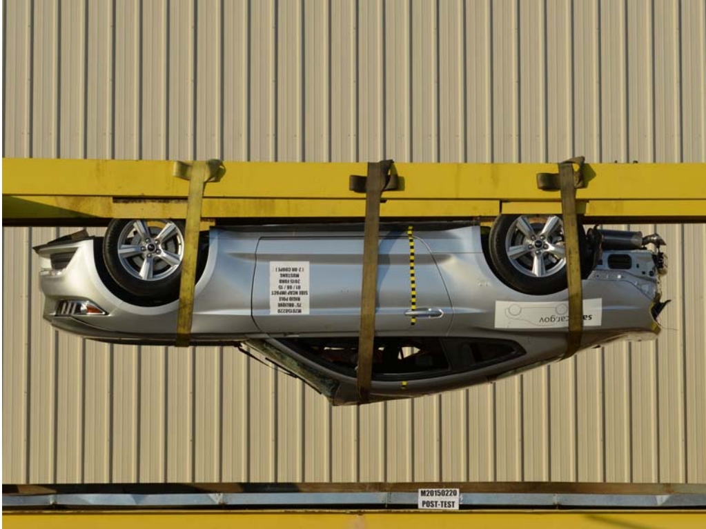
FIGURE 65. FMVSS No. 301 Static Rollover 180 Degrees
