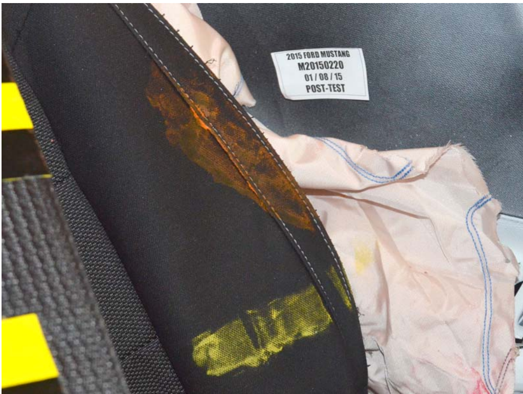
FIGURE 48. Post-Test Dummy Close-Up Torso Contact With Vehicle Interior View
