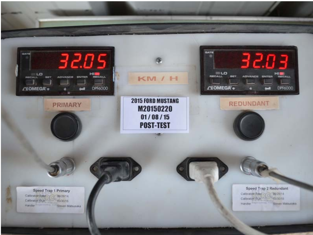
FIGURE 62. Post-Test Primary and Redundant Speed Trap Read-Out
