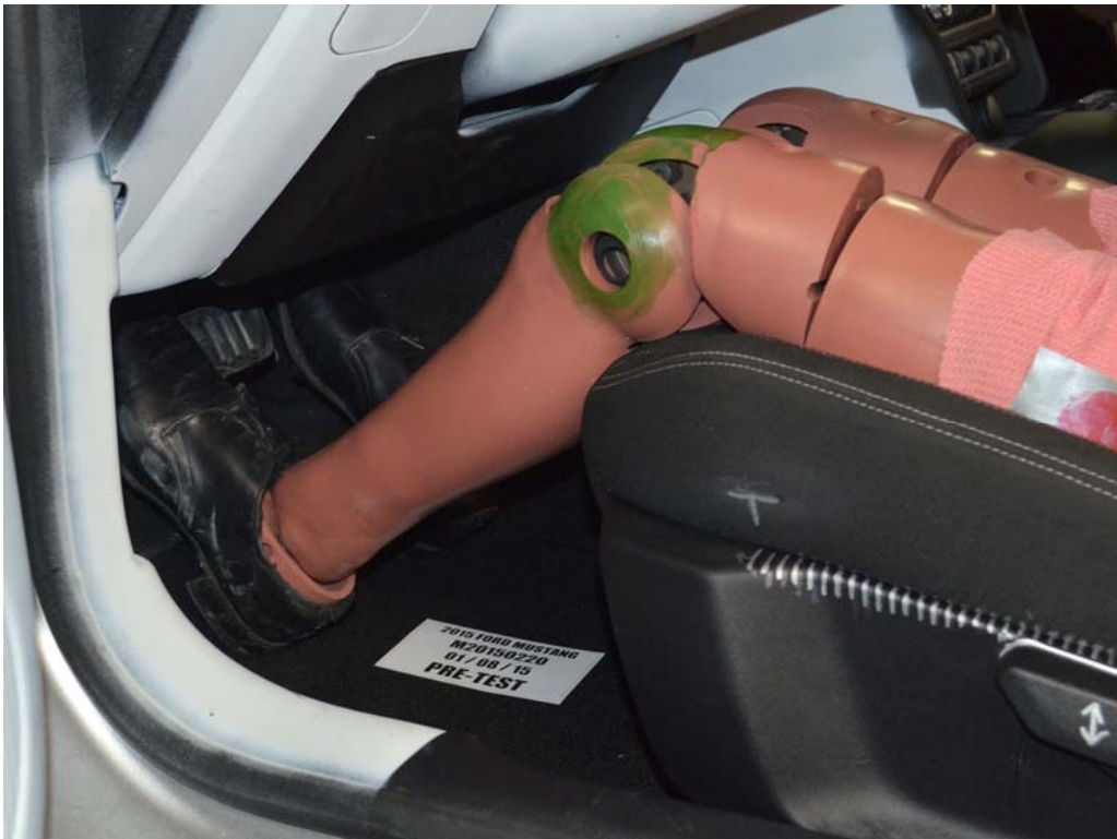
FIGURE 32. Pre-Test Placement of Dummy's Feet
