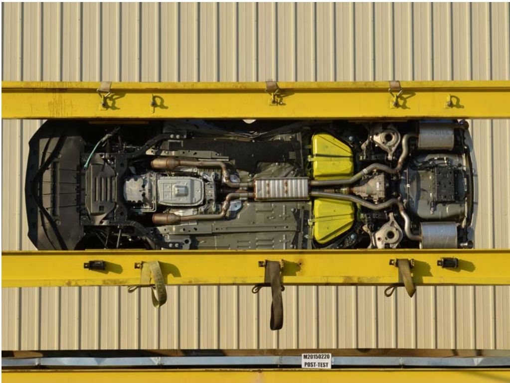
FIGURE 66. FMVSS No. 301 Static Rollover 270 Degrees
