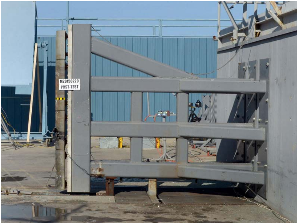
FIGURE 60. Post-Test Pole Barrier Side View
