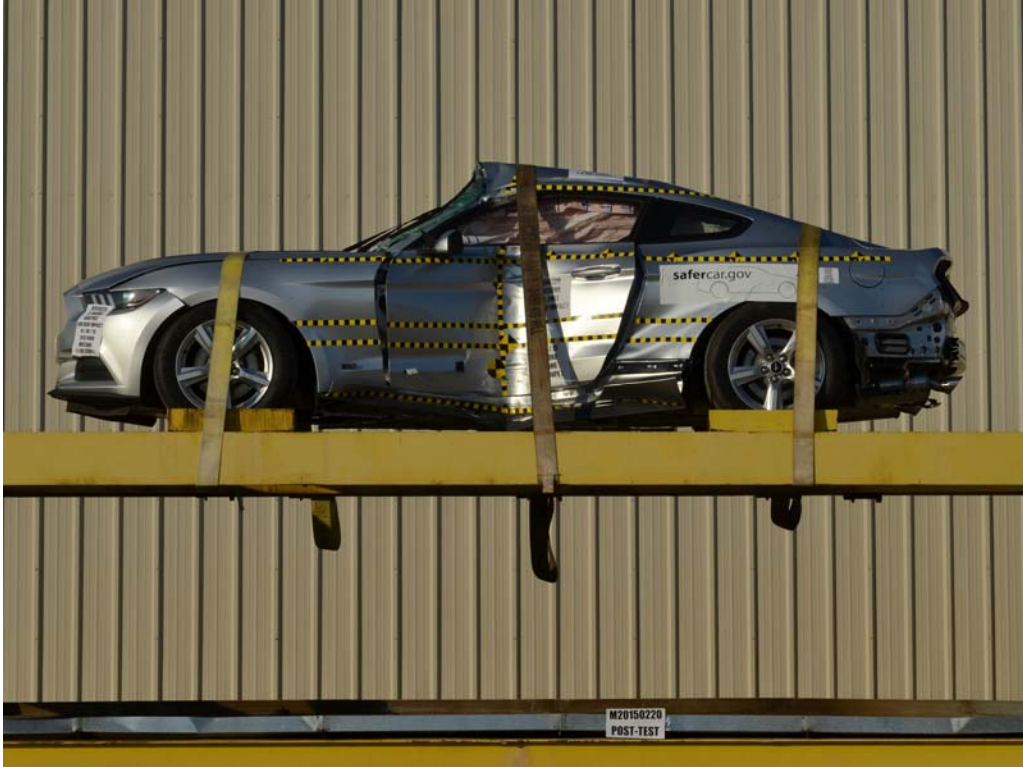
FIGURE 63. FMVSS No. 301 Static Rollover 0 Degrees
