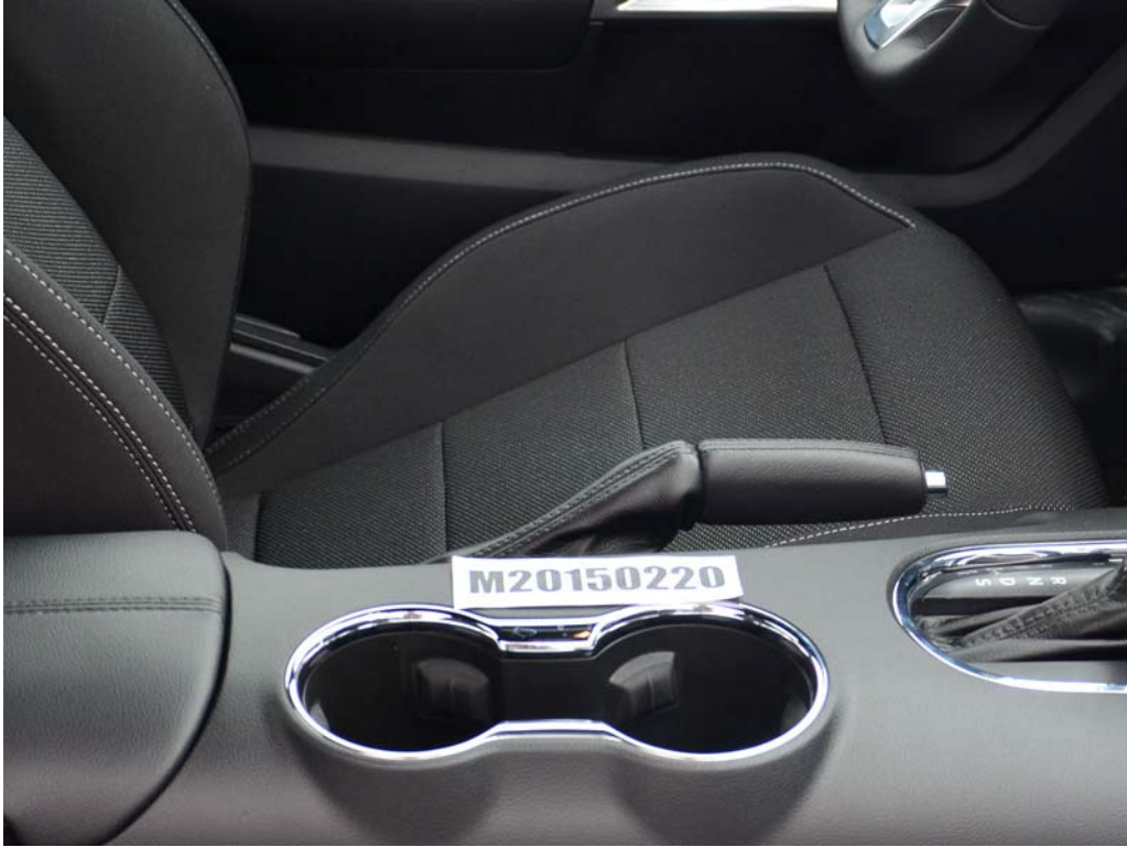
FIGURE 35. View of Disengaged Parking Brake
