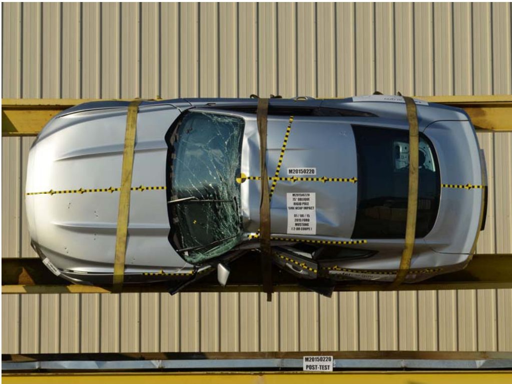
FIGURE 64. FMVSS No. 301 Static Rollover 90 Degrees
