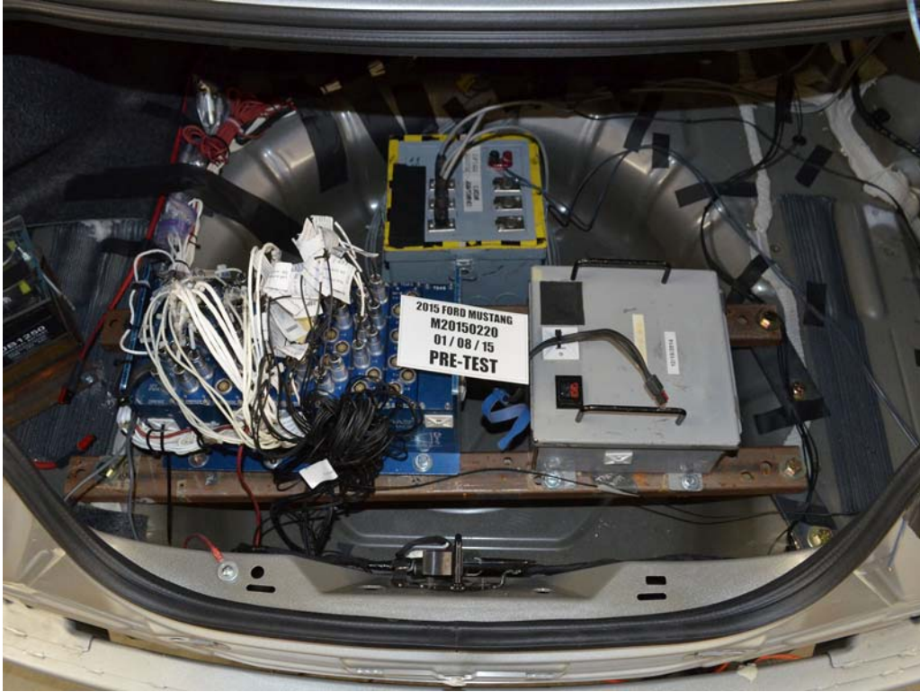
FIGURE 61. Pre-Test Ballast View
