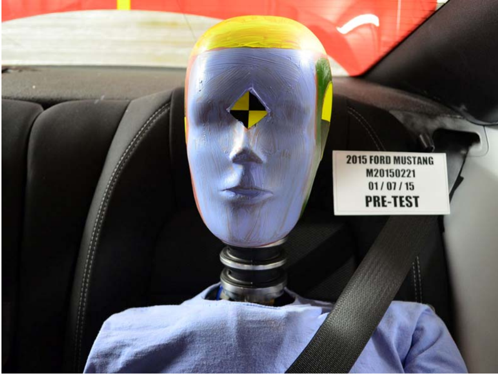
FIGURE 59. Pre-Test Frontal View of Rear Passenger Dummy Head and Shoulders in Relation to Head Restraint
