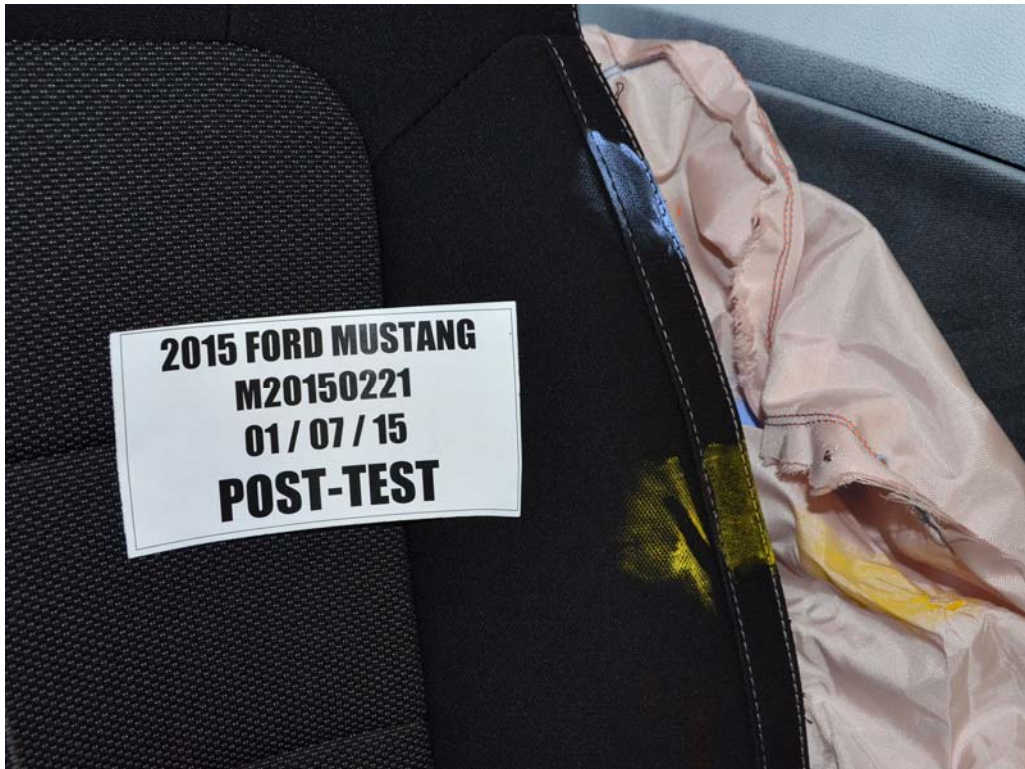
FIGURE 50. Post-Test Driver Dummy Close-Up Torso Contact with Vehicle Interior View
