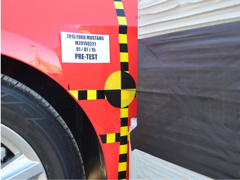
FIGURE 19. Pre-Test Close-Up View of Impact Point Target
