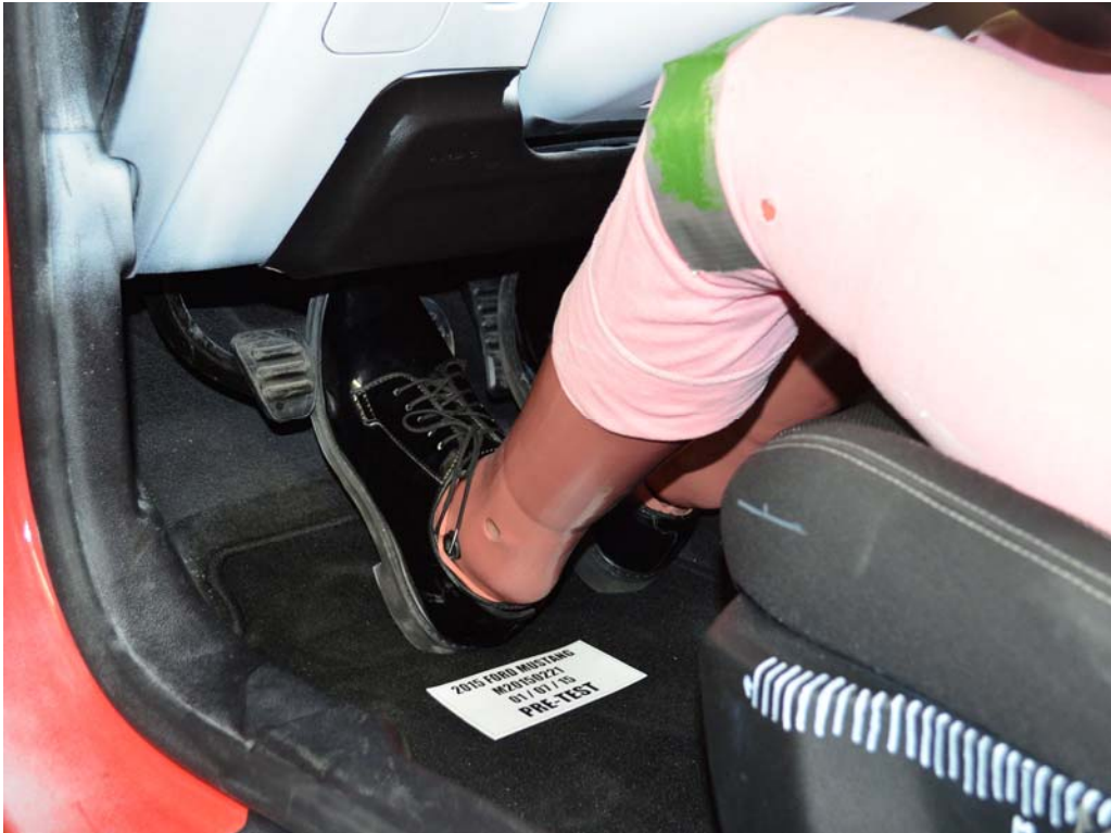
FIGURE 34. Pre-Test Placement of Driver Dummy's Feet
