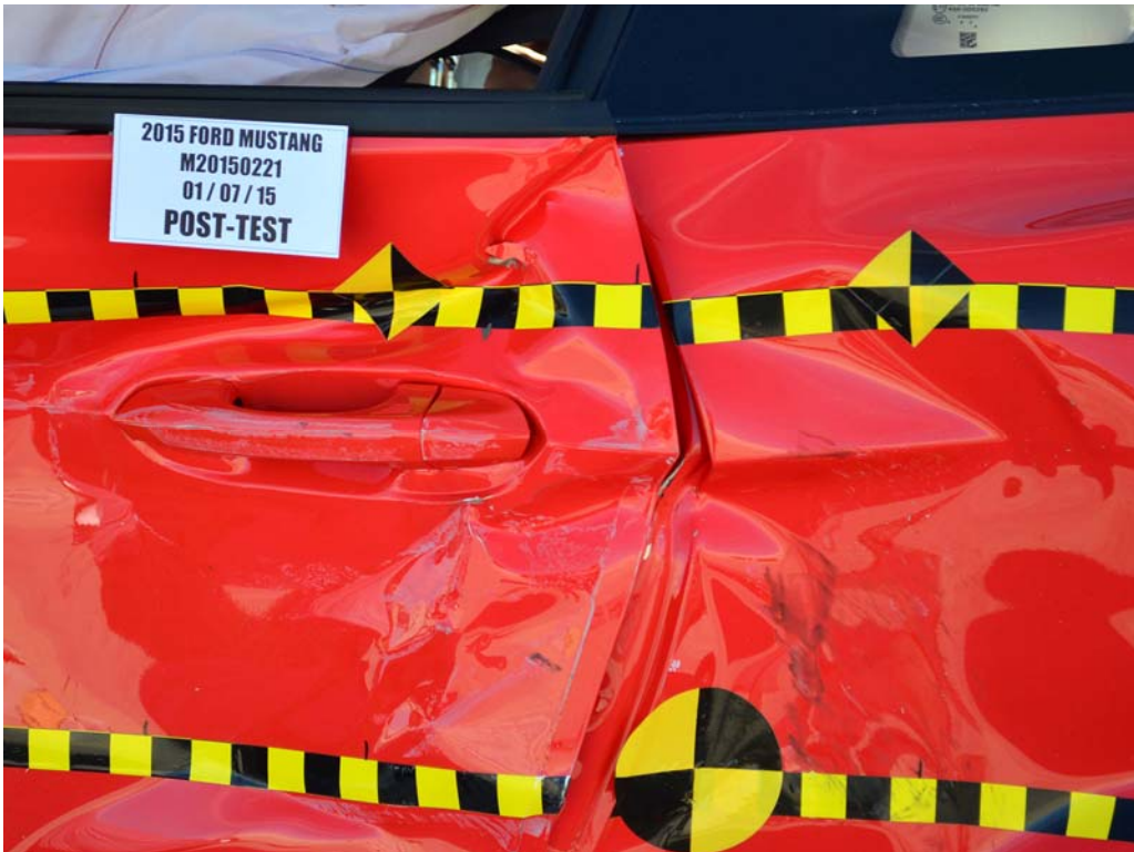
FIGURE 22. Post-Test Left Front Door Latch Close-Up
