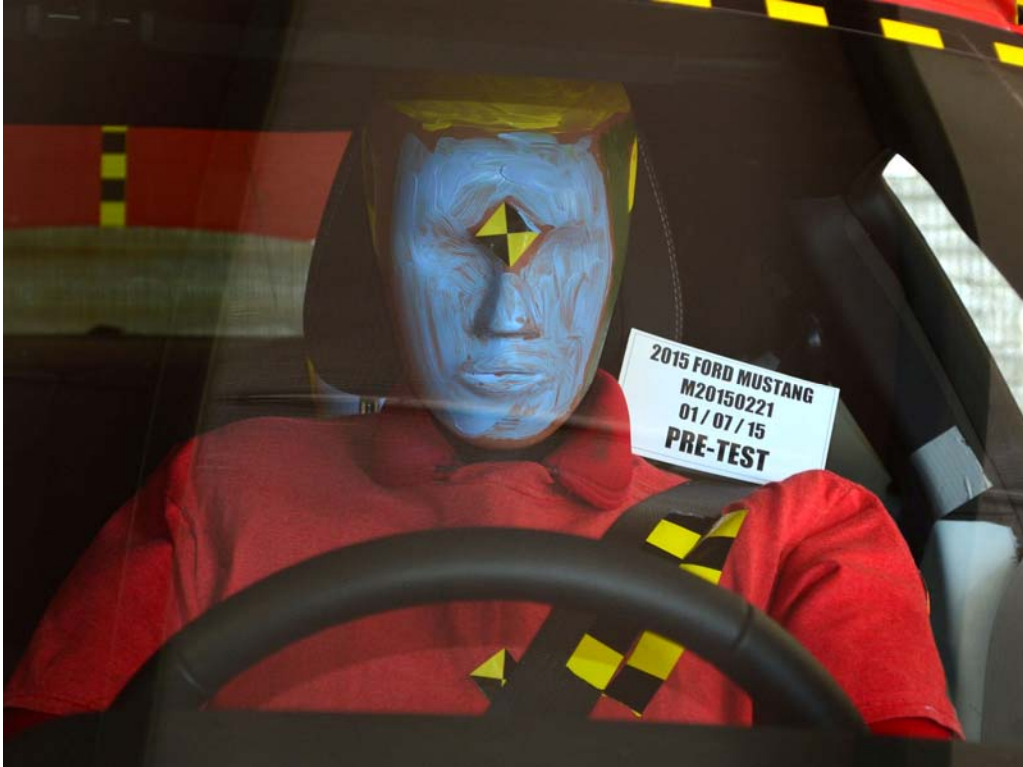
FIGURE 31. Pre-Test Frontal View of Driver Dummy Head and Shoulders in Relation to Head Restraint
