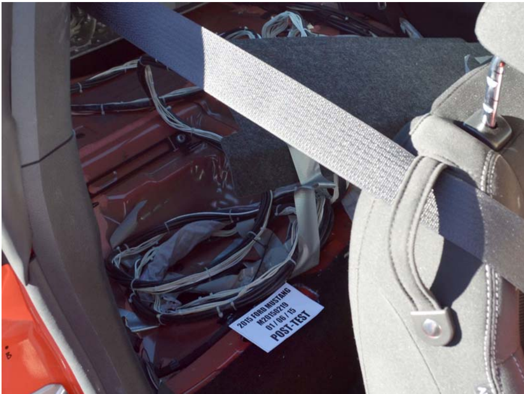
FIGURE 28. Post-Test Dummy Cable Routing
