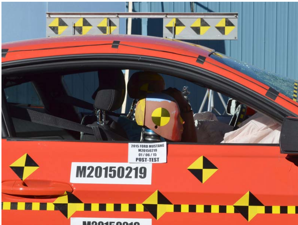
FIGURE 53. Post-Test Passenger Dummy Window View
