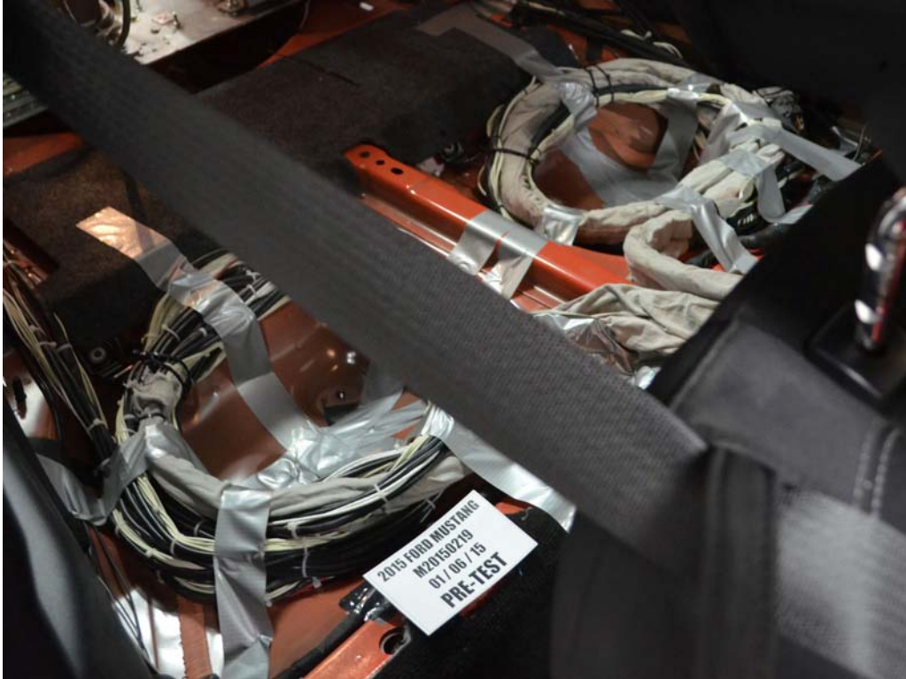
FIGURE 27. Pre-Test Dummy Cable Routing
