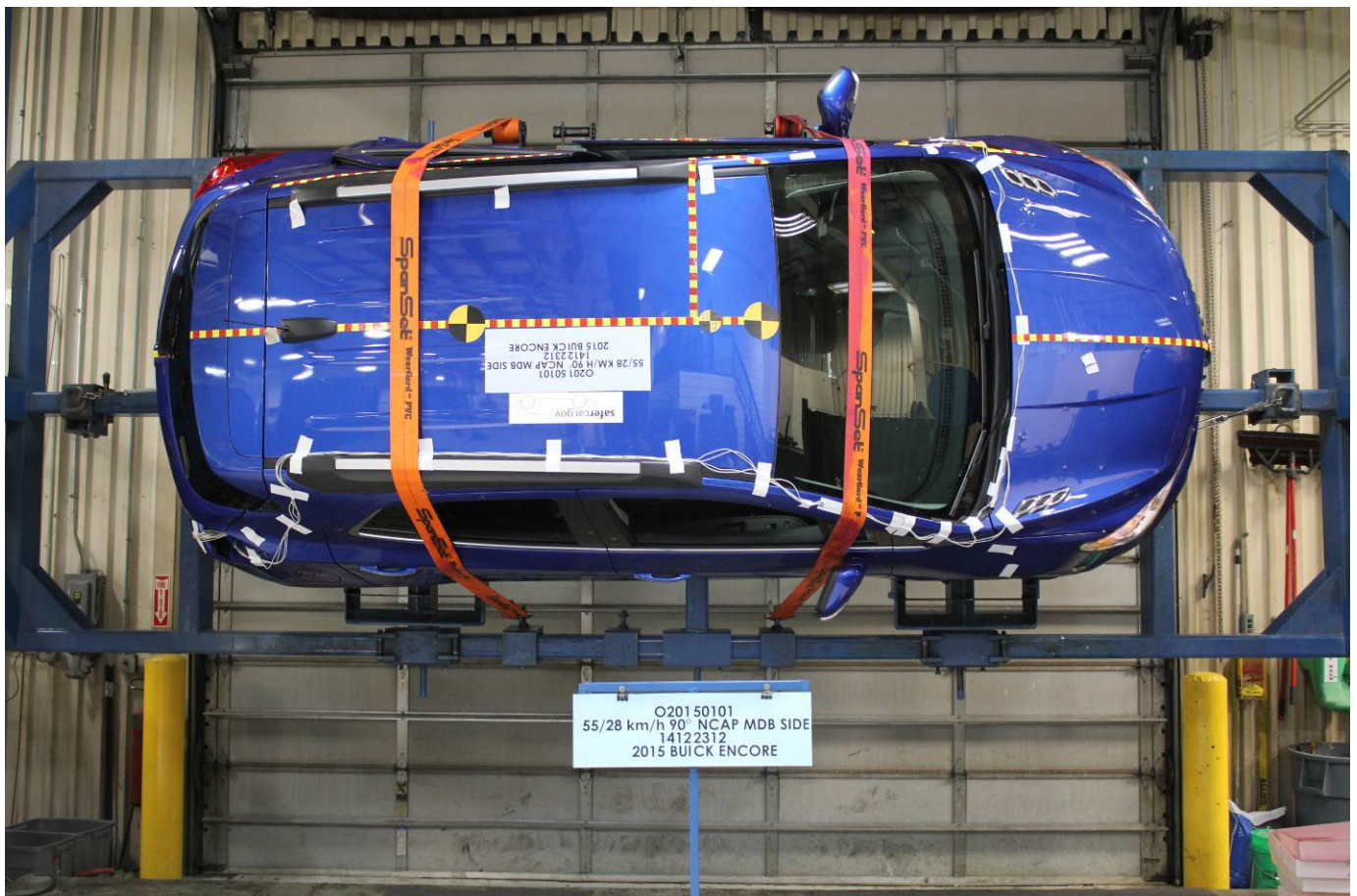
FMVSS No. 301 Static Rollover 90 Degrees
