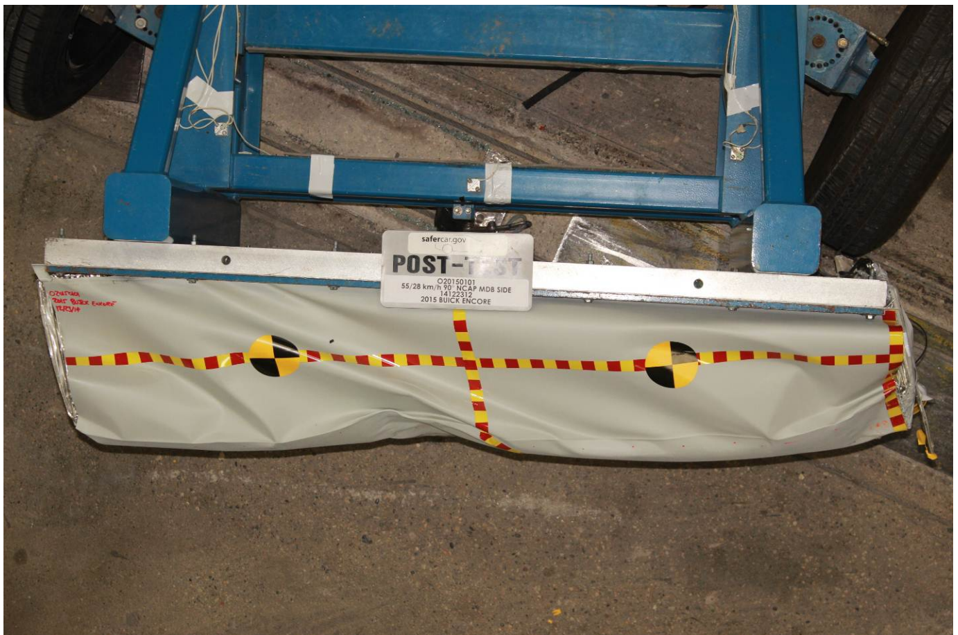
Post-Test Top View of MDB Impactor Face
