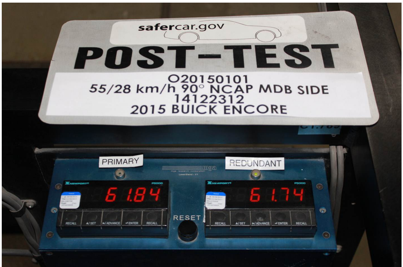
Post-Test Primary and Redundant Speed Trap Read-Out
