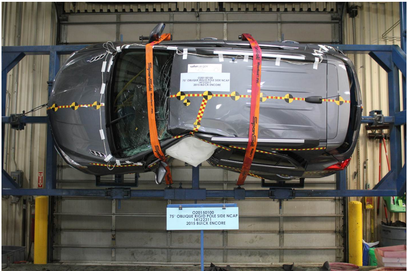
FMVSS No. 301 Static Rollover 270 Degrees
