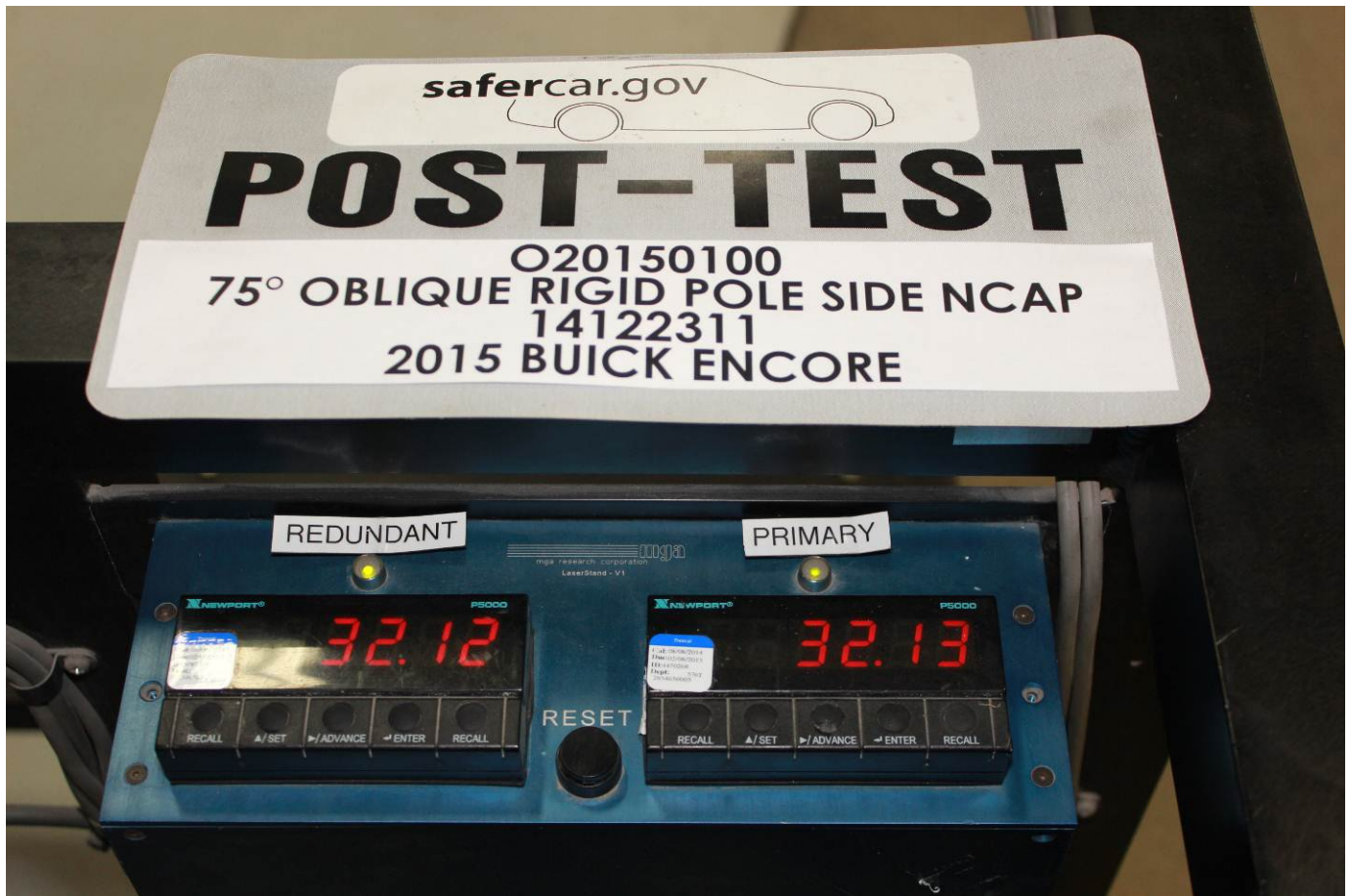
Post-Test Primary and Redundant Speed Trap Read-Out
