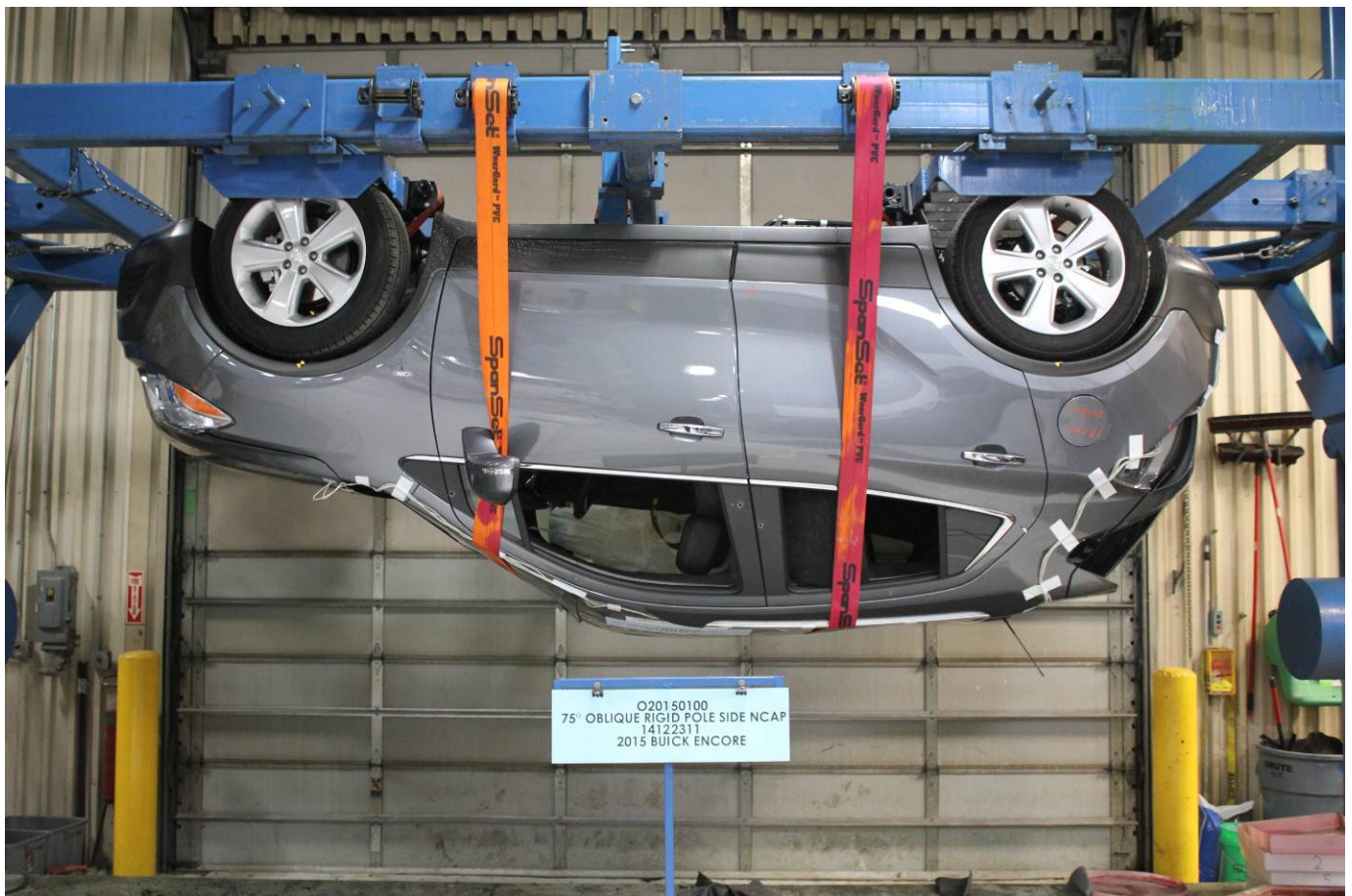
FMVSS No. 301 Static Rollover 180 Degrees
