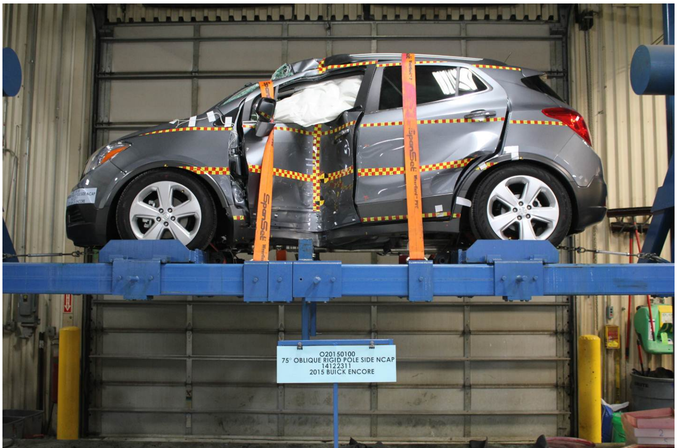
FMVSS No. 301 Static Rollover 360 Degrees
