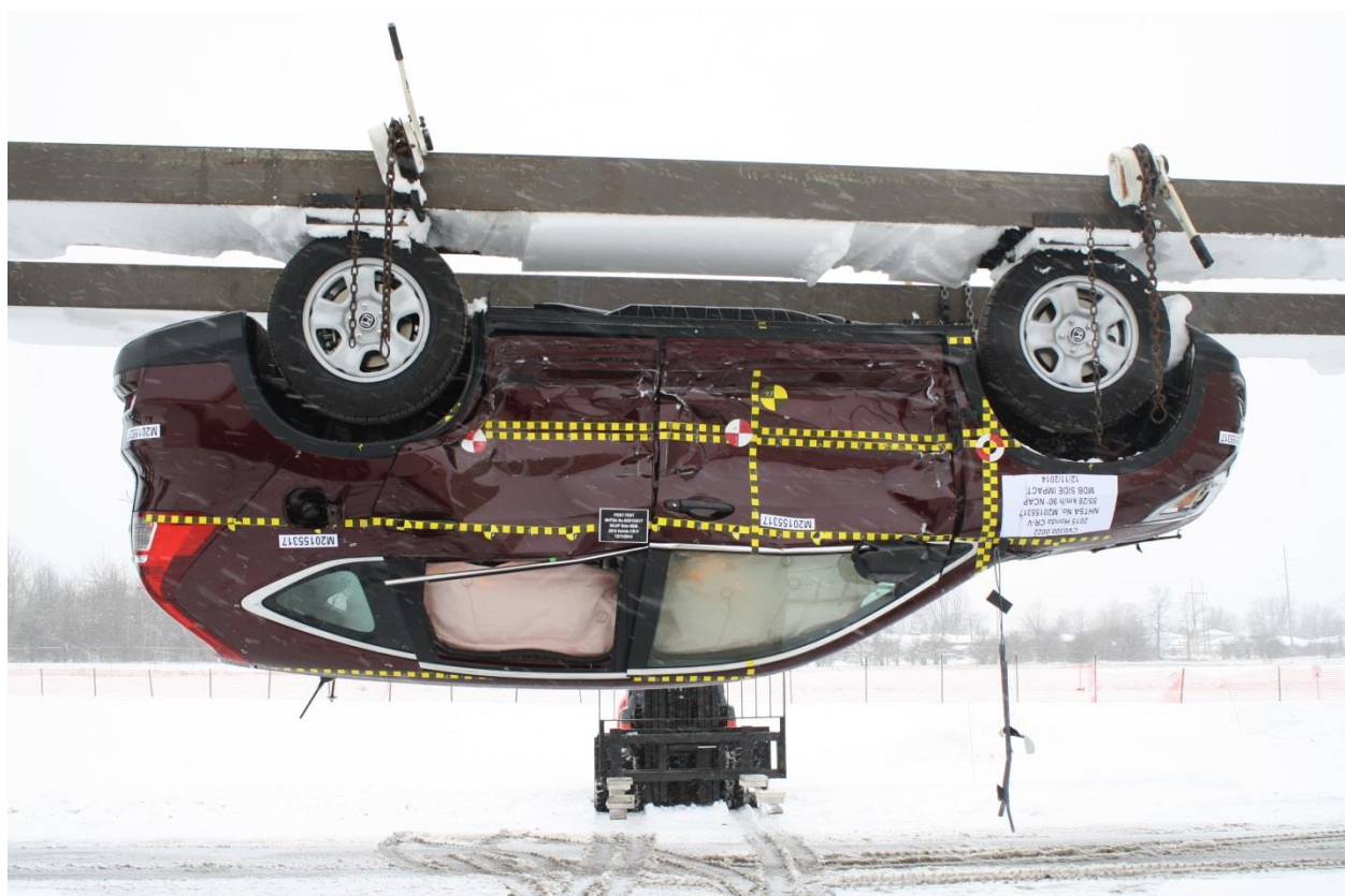
Figure A-98: FMVSS No. 301 Static Rollover 180 Degrees
