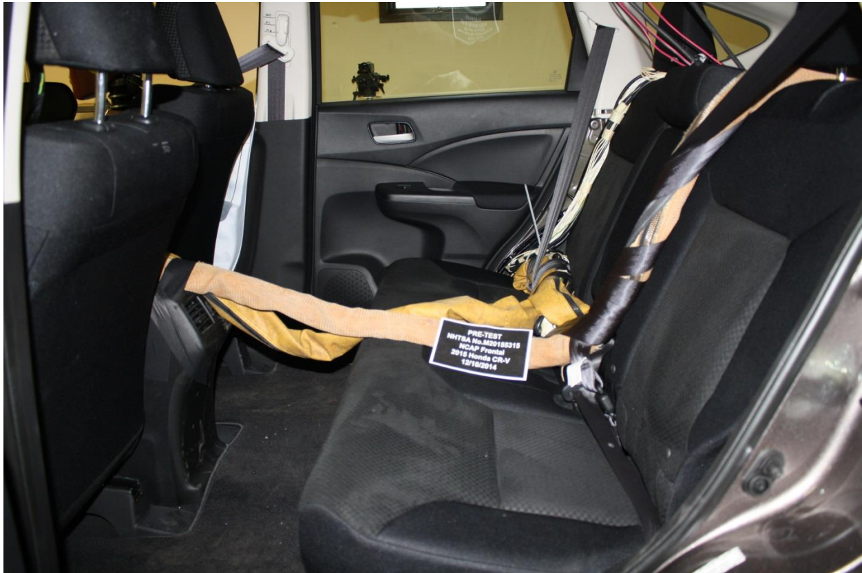
Figure A-27: Pre-Test Dummy Cable Routing
