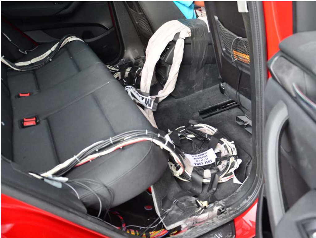
FIGURE 28. Post-Test Dummy Cable Routing
