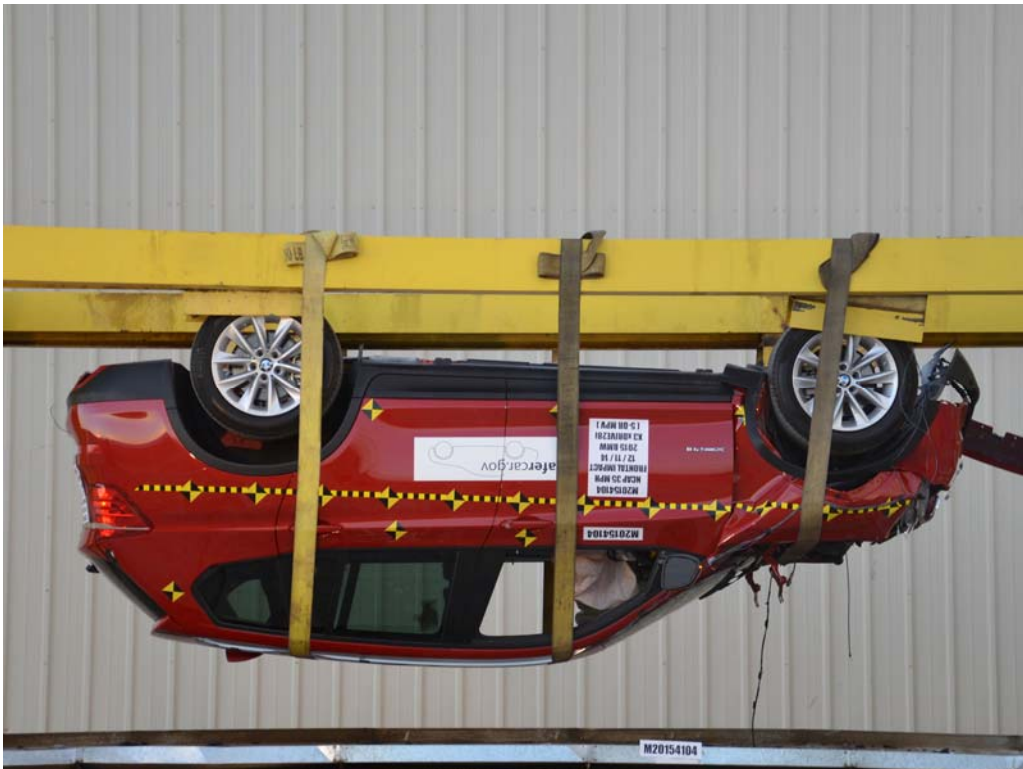
FIGURE 74. Vehicle at 180° on Static Rollover Device
