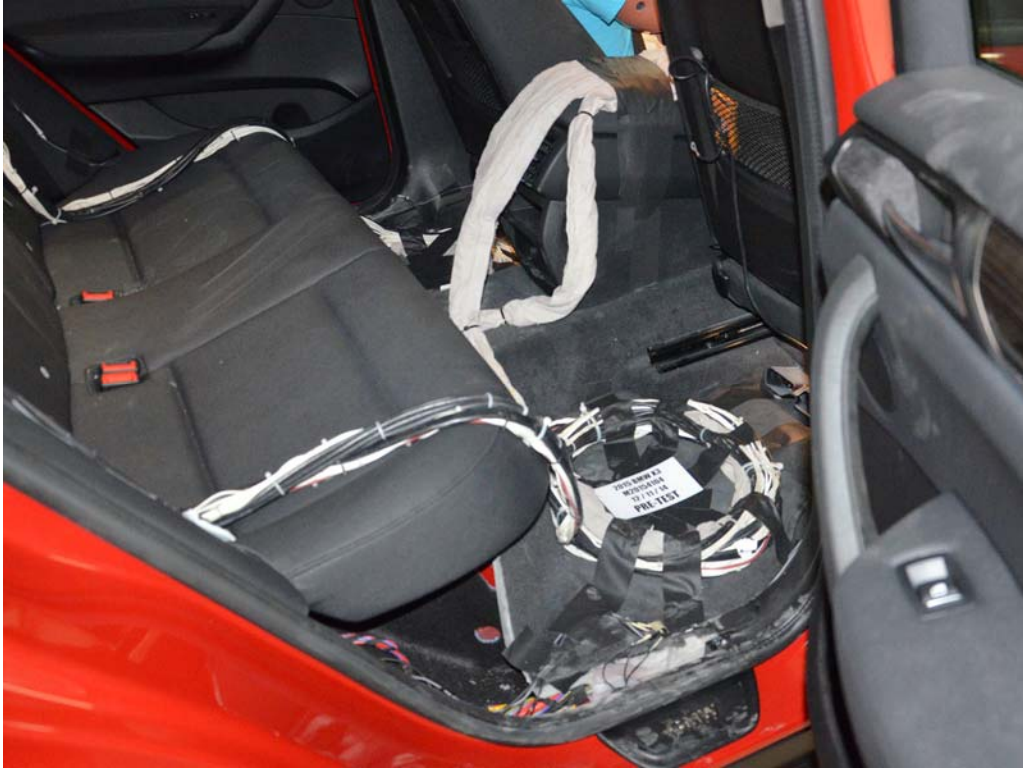
FIGURE 27. Pre-Test Dummy Cable Routing
