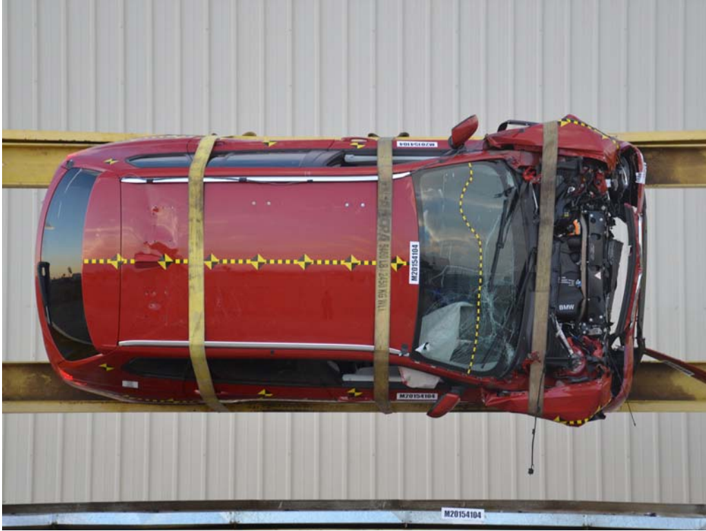
FIGURE 73. Vehicle at 90° on Static Rollover Device
