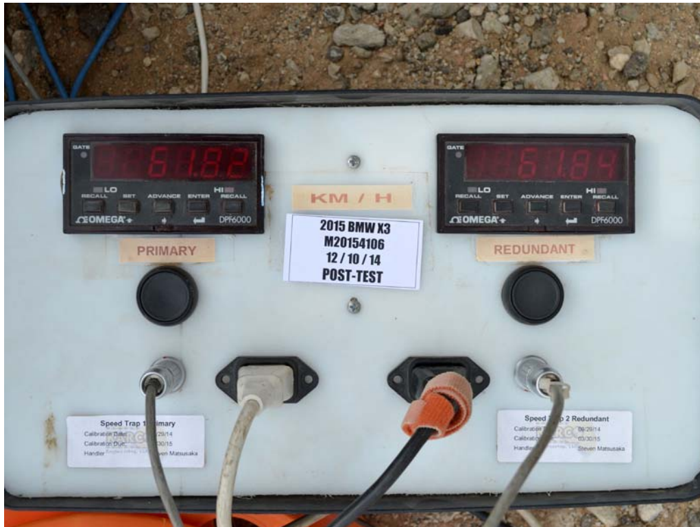
FIGURE 95. Post-Test Primary and Redundant Speed Trap Read-Out
