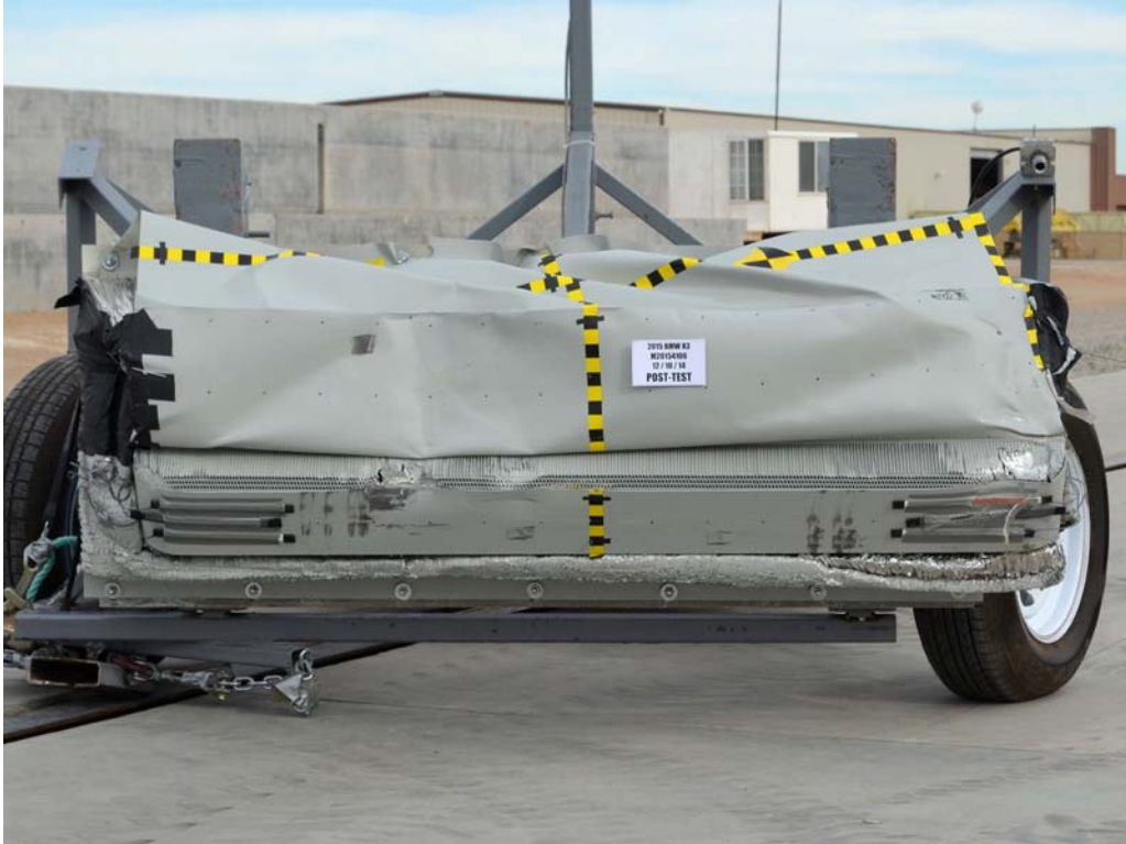
FIGURE 85. Post-Test Front View of MDB Impactor Face
