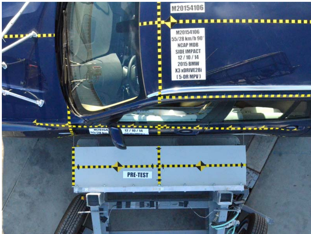
FIGURE 15. Pre-Test Overhead View of Test Area
