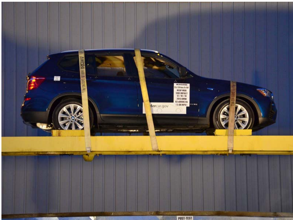
FIGURE 100. FMVSS No. 301 Static Rollover 360 Degrees
