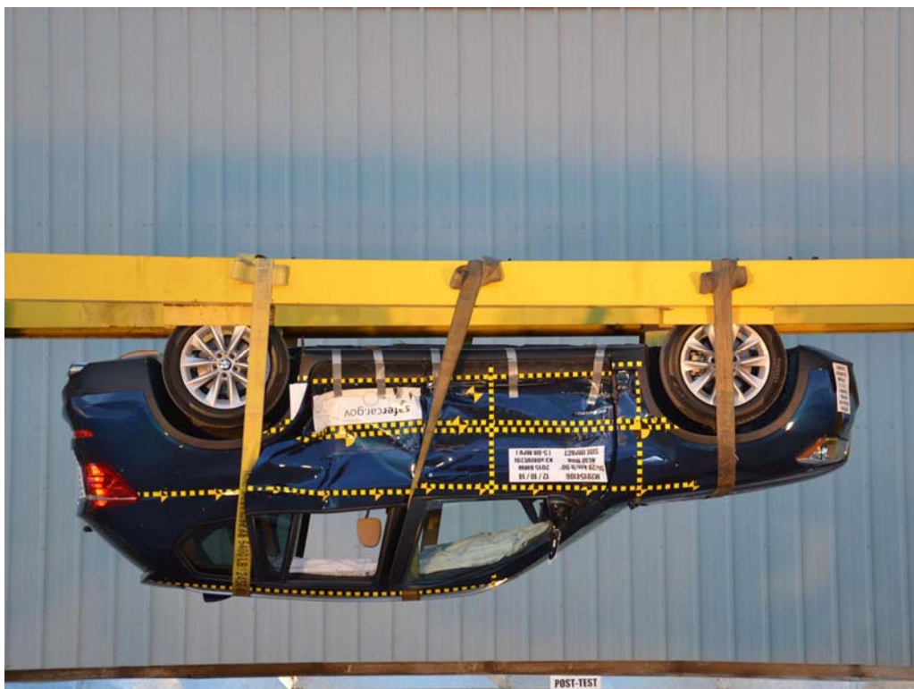
FIGURE 98. FMVSS No. 301 Static Rollover 180 Degrees
