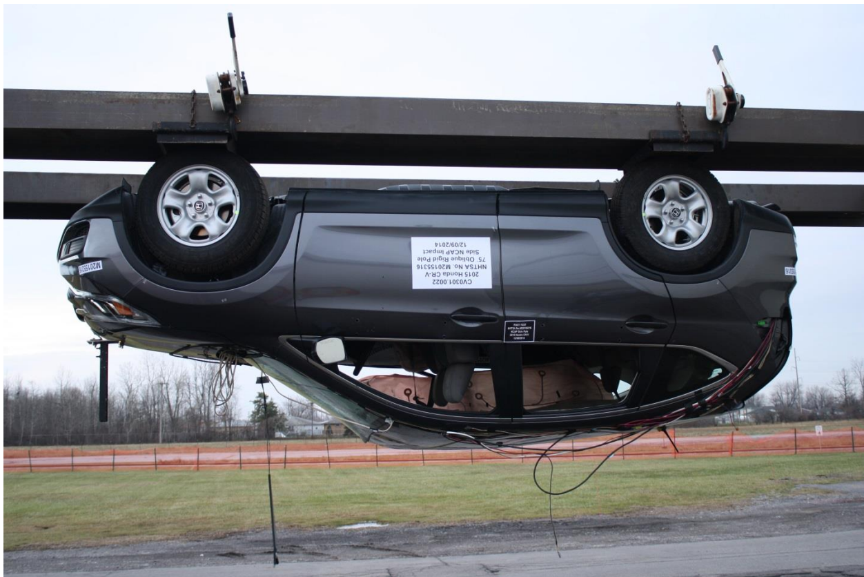
Figure A-65: FMVSS No. 301 Static Rollover 180 Degrees
