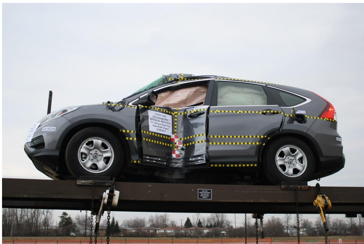
Figure A-63: FMVSS No. 301 Static Rollover 0 Degrees
