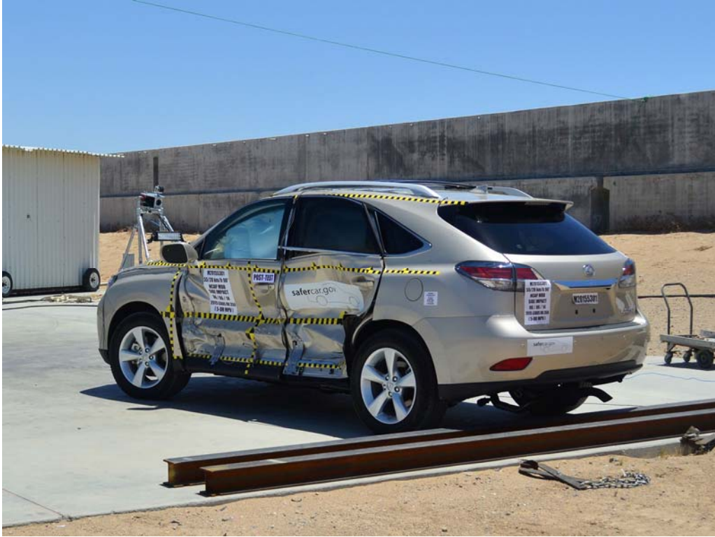
FIGURE 5. Post-Test Left Rear \frac{3}{4} View of NCAP Side Impact Test
