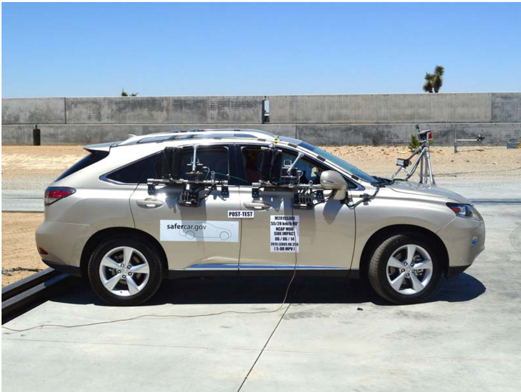
FIGURE 6. Post-Test Right Side View of NCAP Side Impact Test
