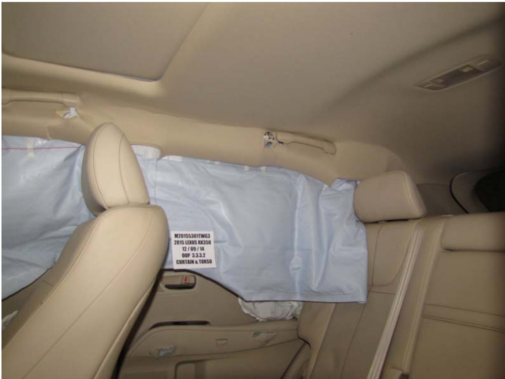
FIGURE 14. Post-Test Airbags, Left Front \frac{3}{4} View
