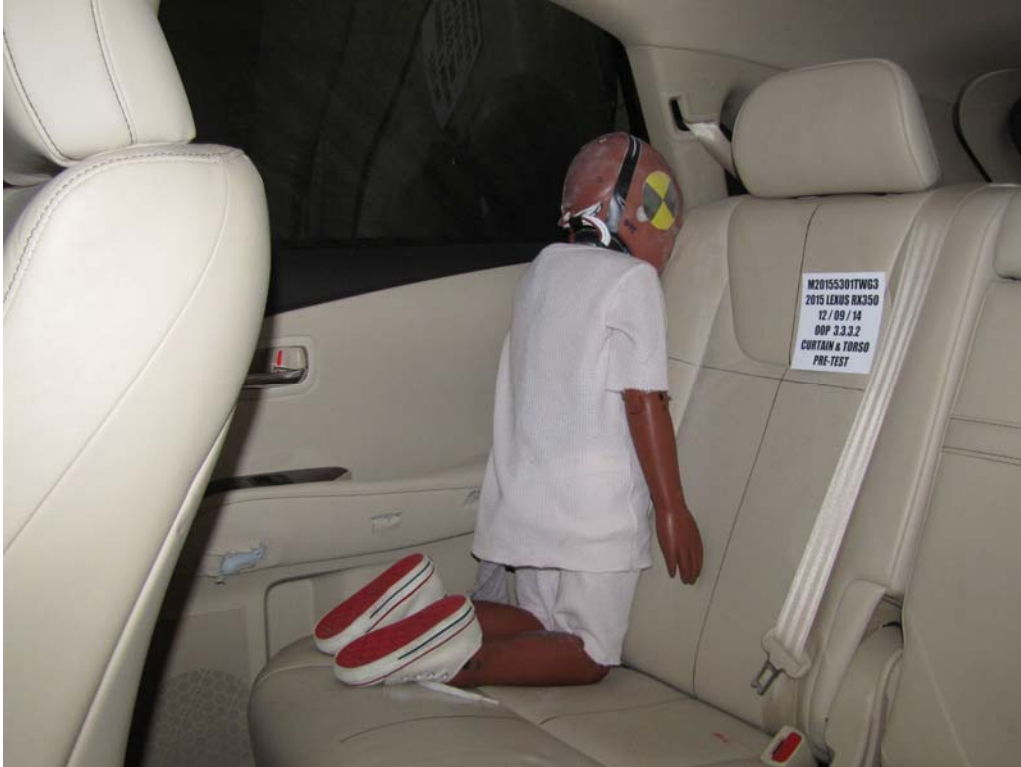
FIGURE 9. Pre-Test Dummy Position, \frac{3}{4} View
