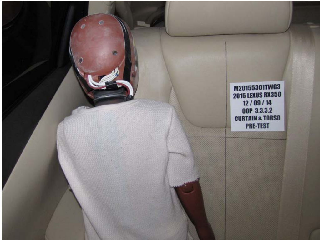
FIGURE 11. Pre-Test Dummy Position, Front View
