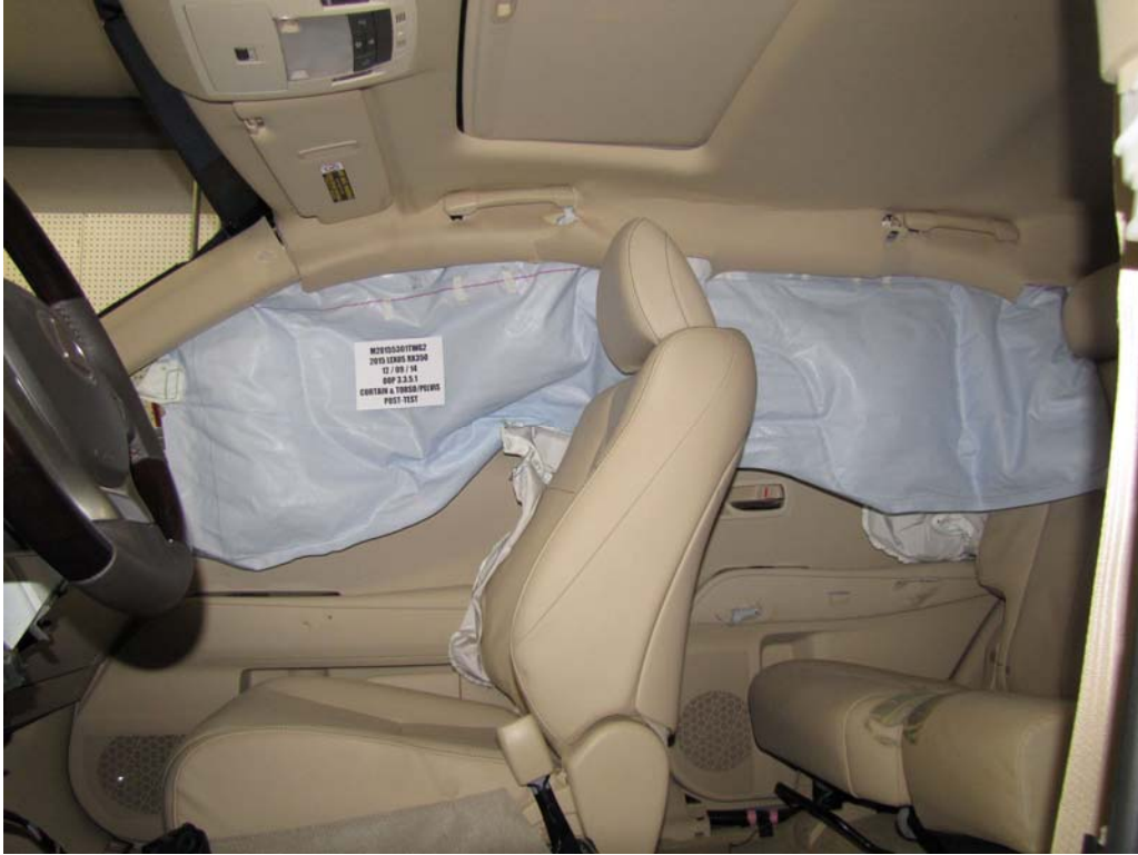
FIGURE 13. Post-Test Airbags, Left Side View
