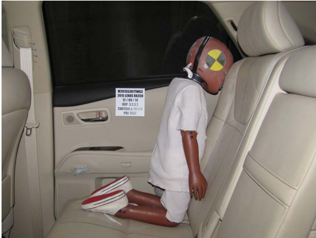
FIGURE 7. Pre-Test Dummy Position, Left Side View
