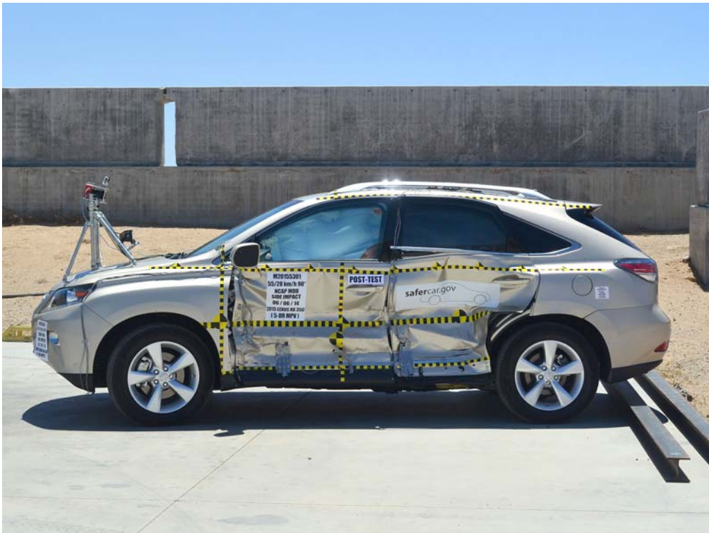
FIGURE 4. Post-Test Left Side View of NCAP Side Impact Test
