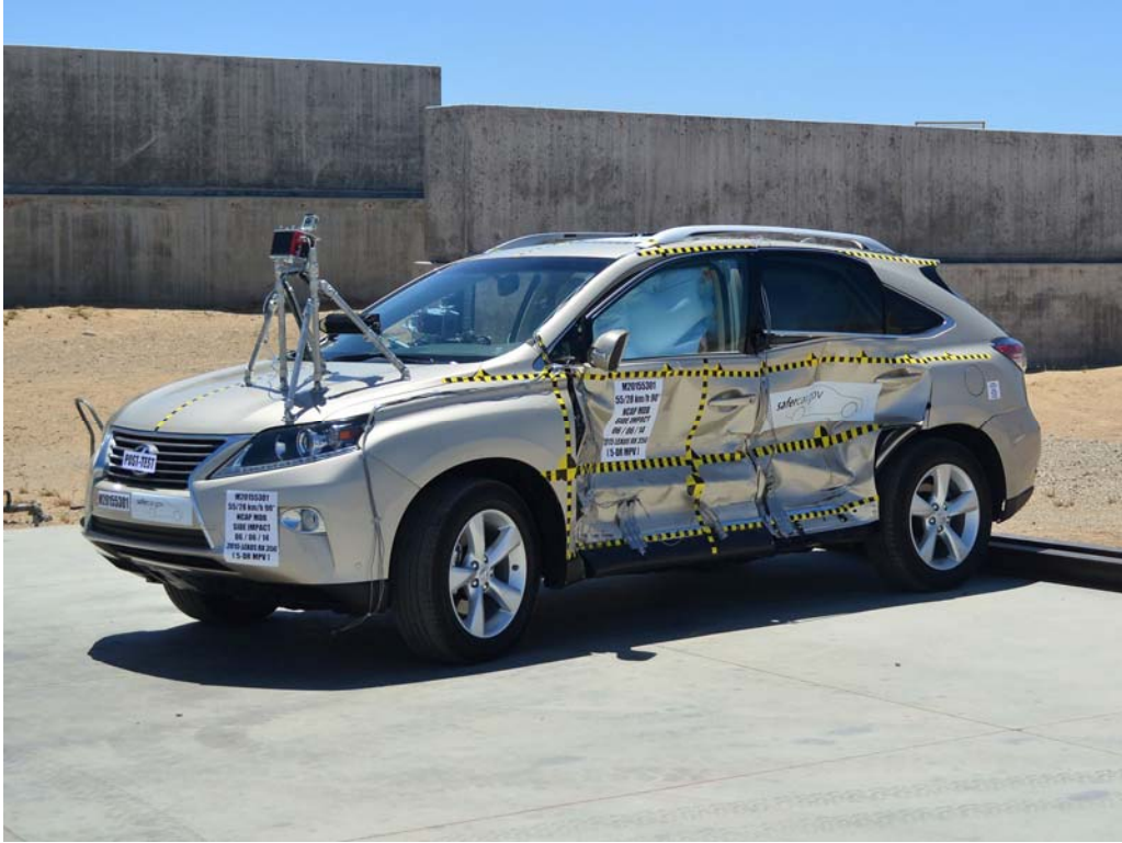
FIGURE 3. Post-Test Left Front \frac{3}{4} View of NCAP Side Impact Test
