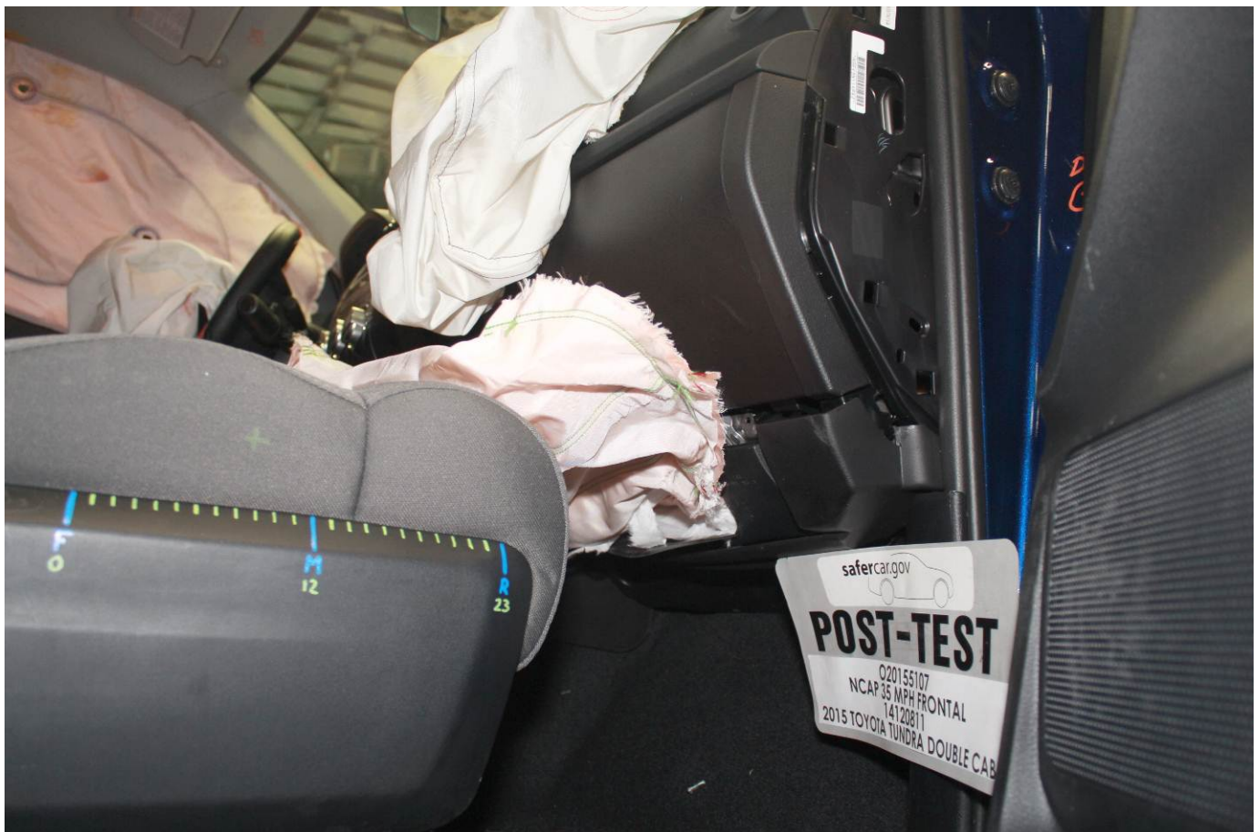
Post-Test Passenger's Side Knee Bolster (without dummy)
