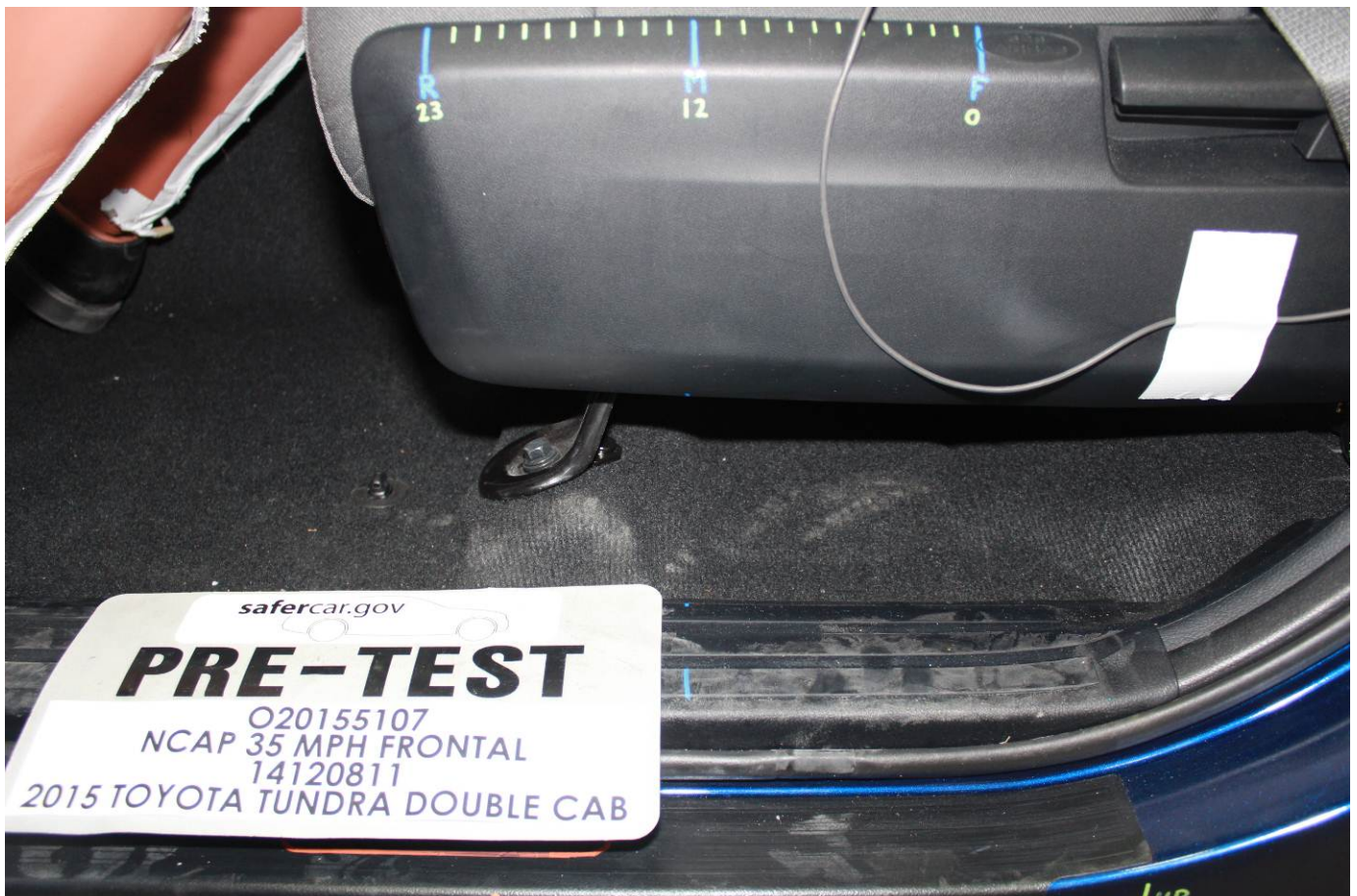
Pre-Test Driver's Seat Fore-Aft Markings
