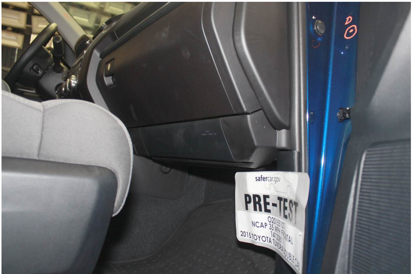
Pre-Test Passenger's Side Knee Bolster (without dummy)
