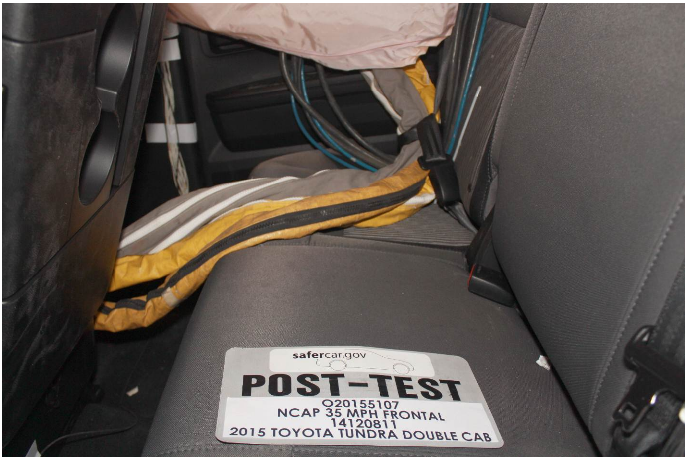
Post-Test Dummy Cable Routing
