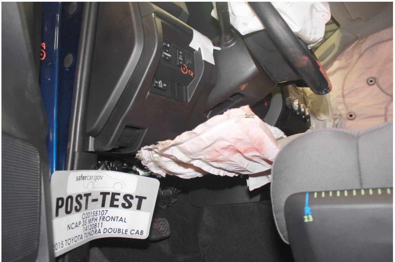
Post-Test Driver's Side Knee Bolster (without dummy)
