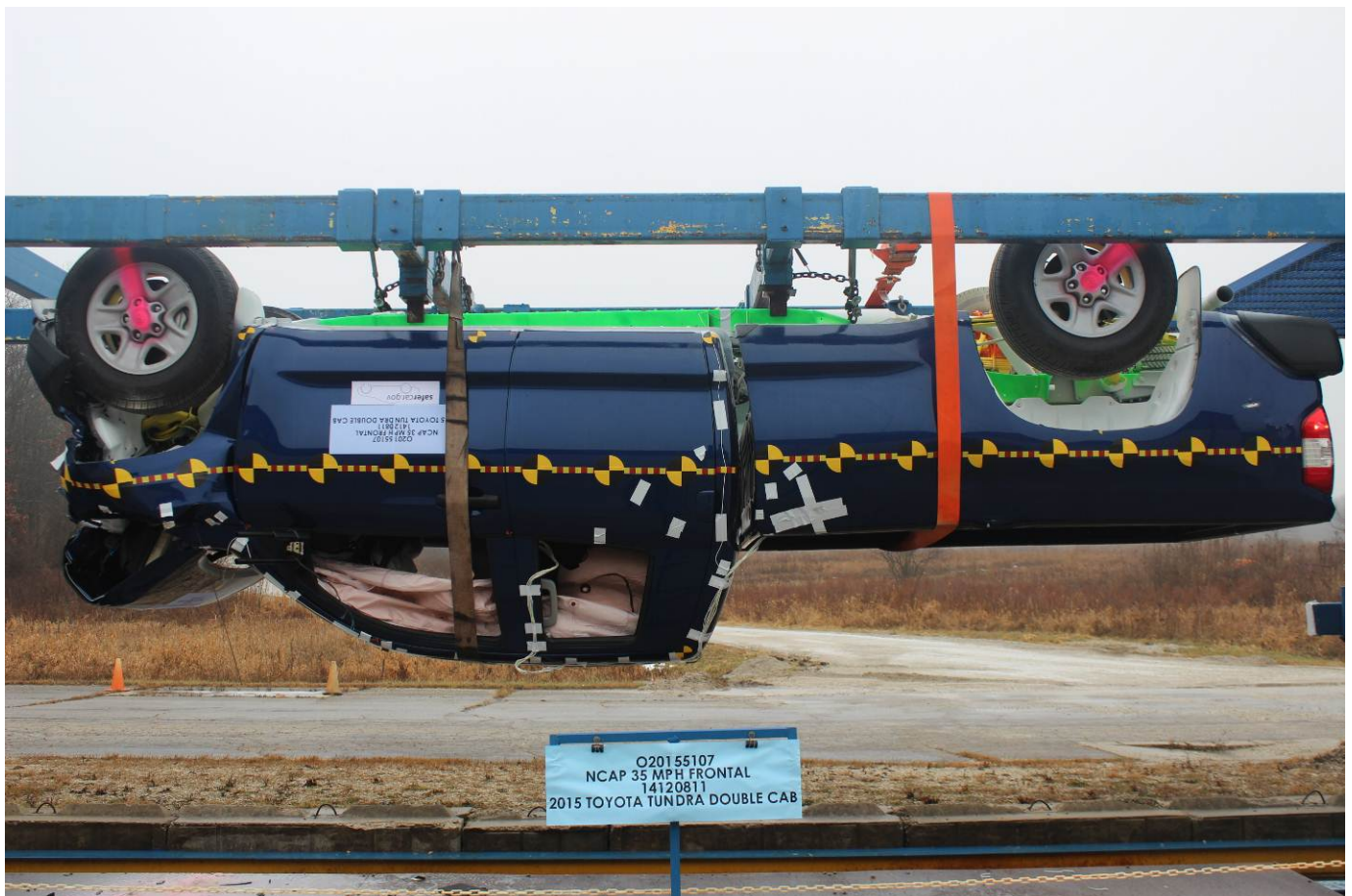
Vehicle at 180 Degrees on Static Rollover Device
