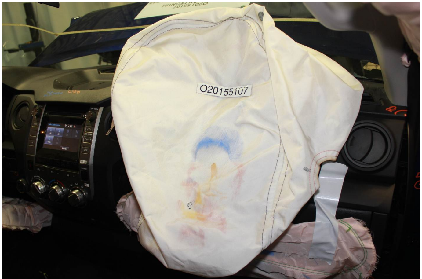
Post-Test Passenger Dummy Contact with Airbag
