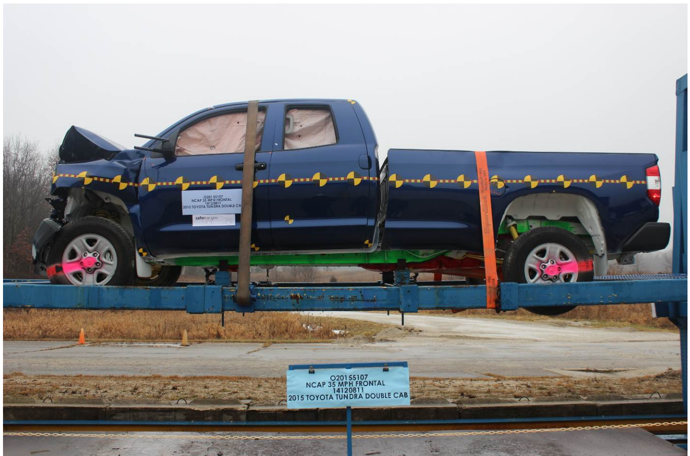
Vehicle at 0 Degree on Static Rollover Device
