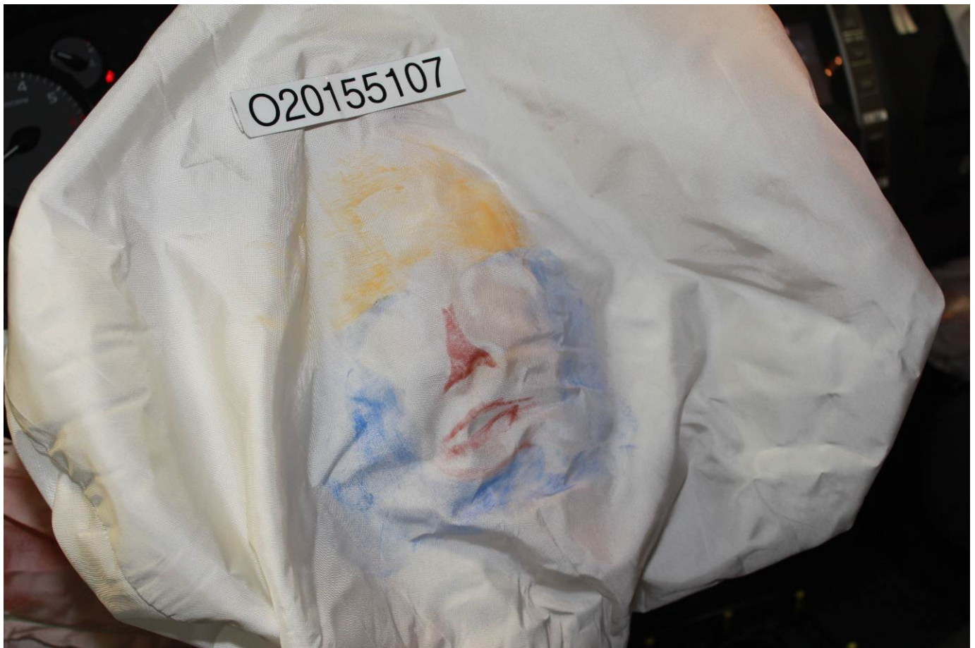
Post-Test Driver Dummy Contact with Airbag
