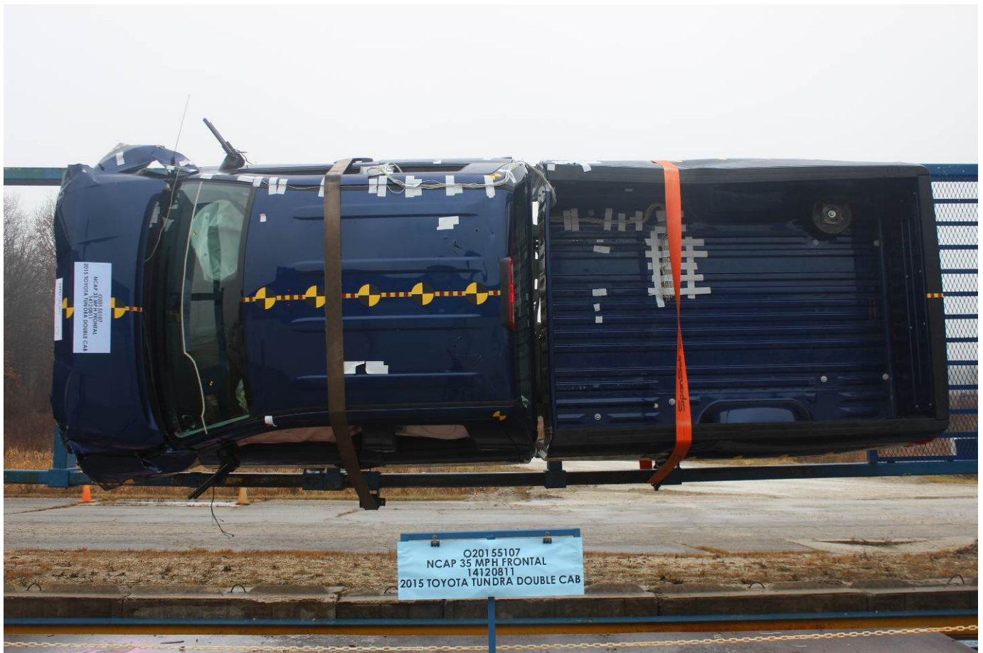
Vehicle at 90 Degrees on Static Rollover Device
