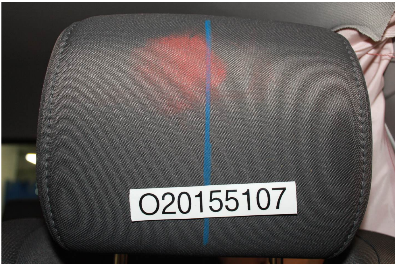
Post-Test Driver Dummy Contact with Headrest
