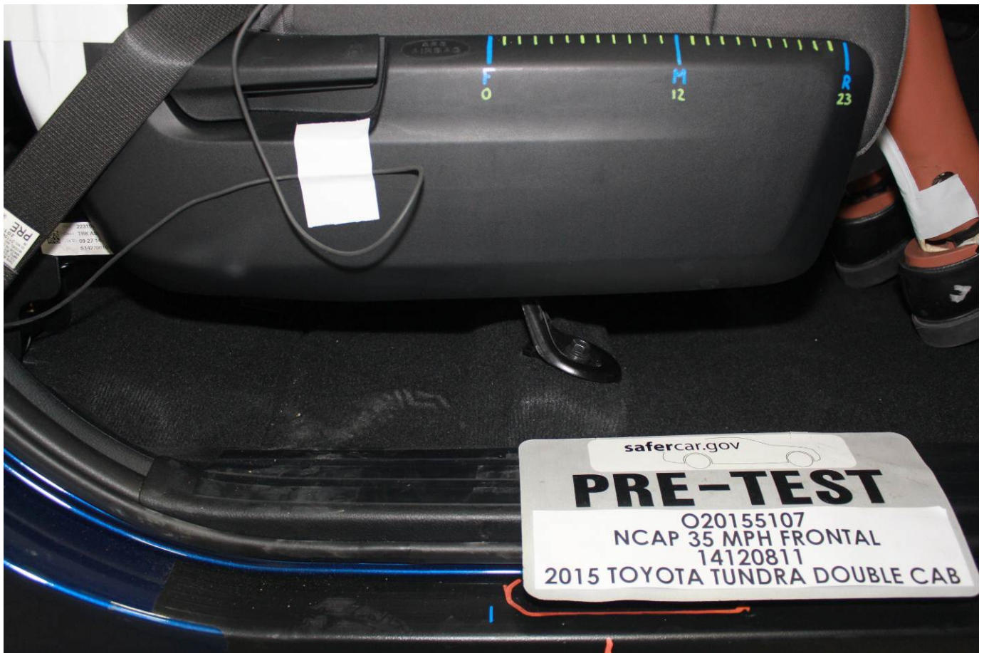
Pre-Test Passenger's Seat Fore-Aft Markings
