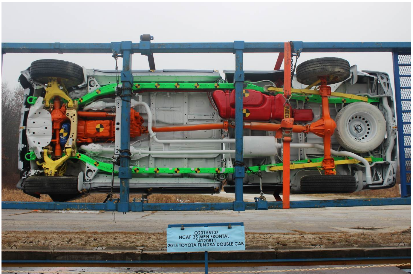
Vehicle at 270 Degrees on Static Rollover Device
