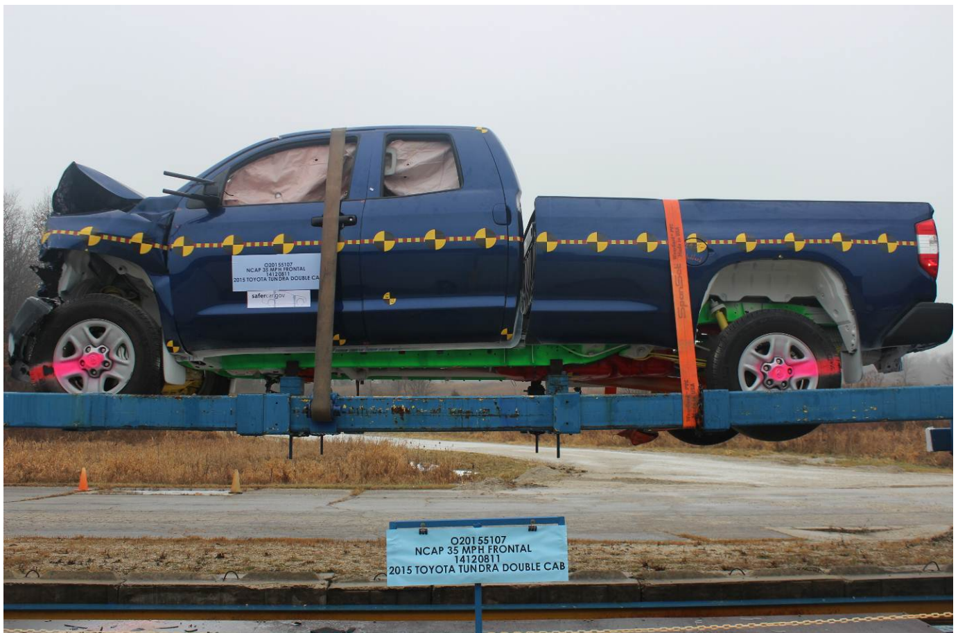
Vehicle at 360 Degrees on Static Rollover Device
