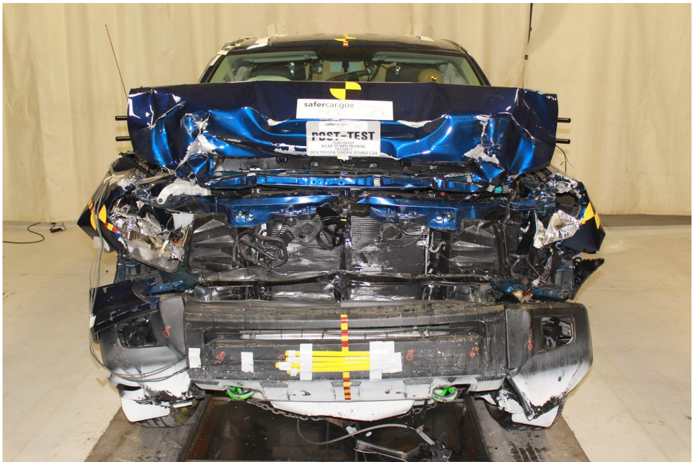
Post-Test Front View of Test Vehicle
