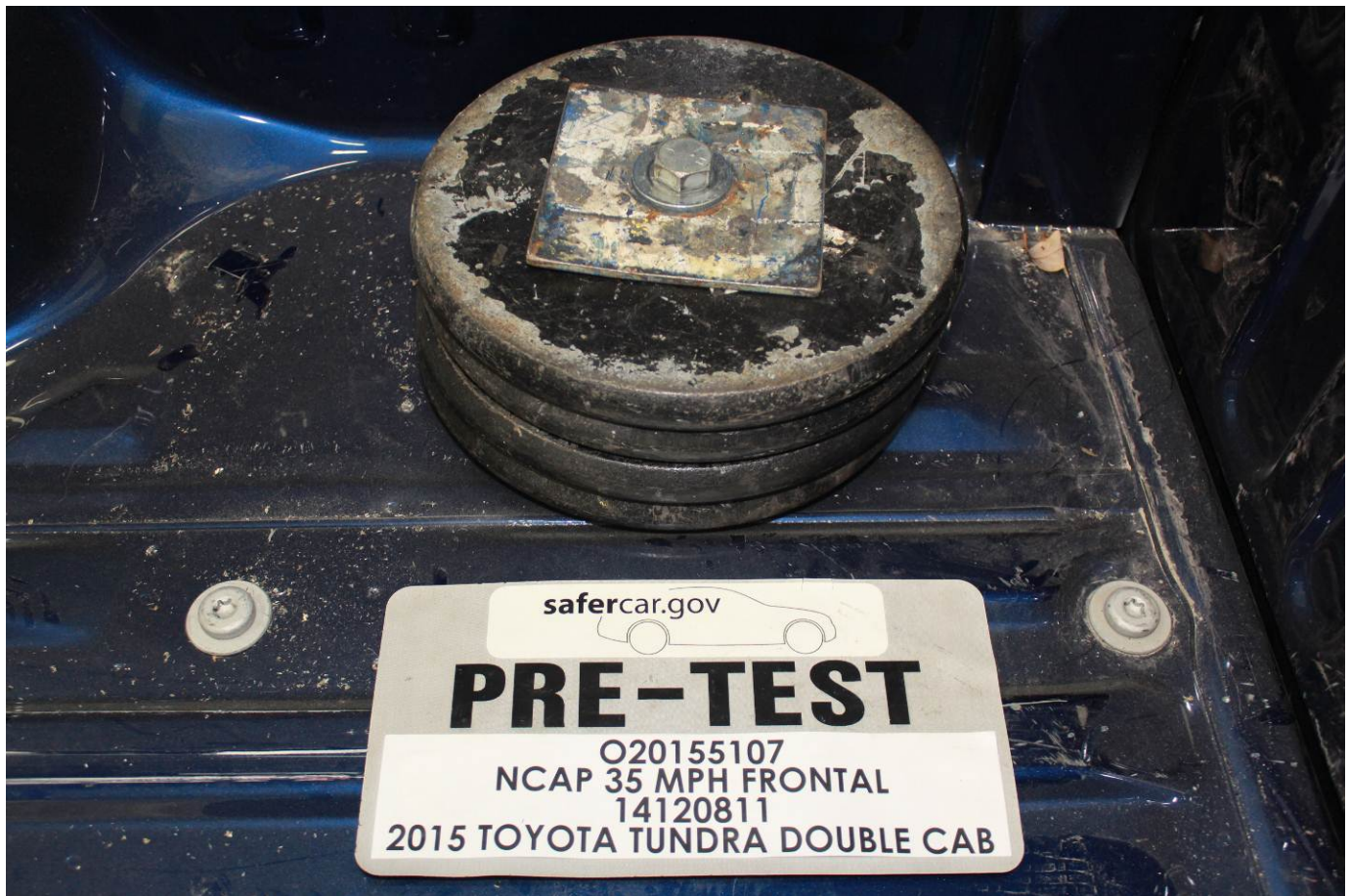
Ballast Installed in Vehicle
