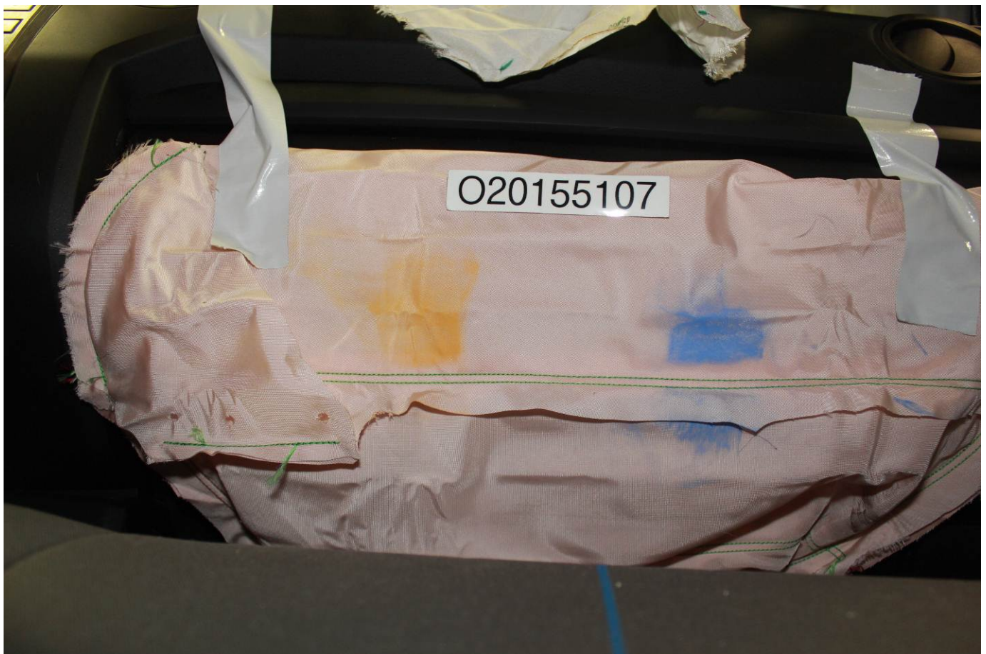
Post-Test Passenger Dummy Contact with Knee Airbag
