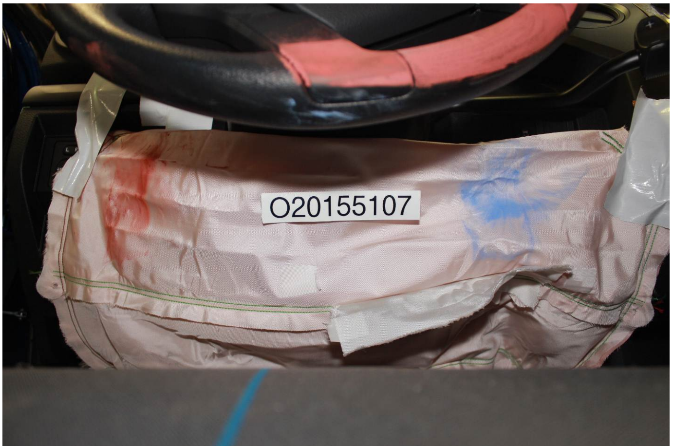
Post-Test Driver Dummy Contact with Knee Airbag
