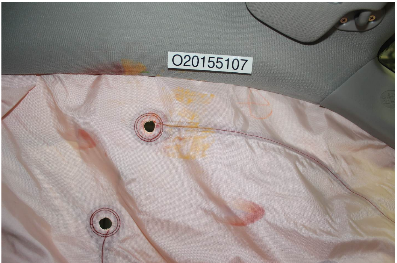
Post-Test Driver Dummy Contact with Airbag
