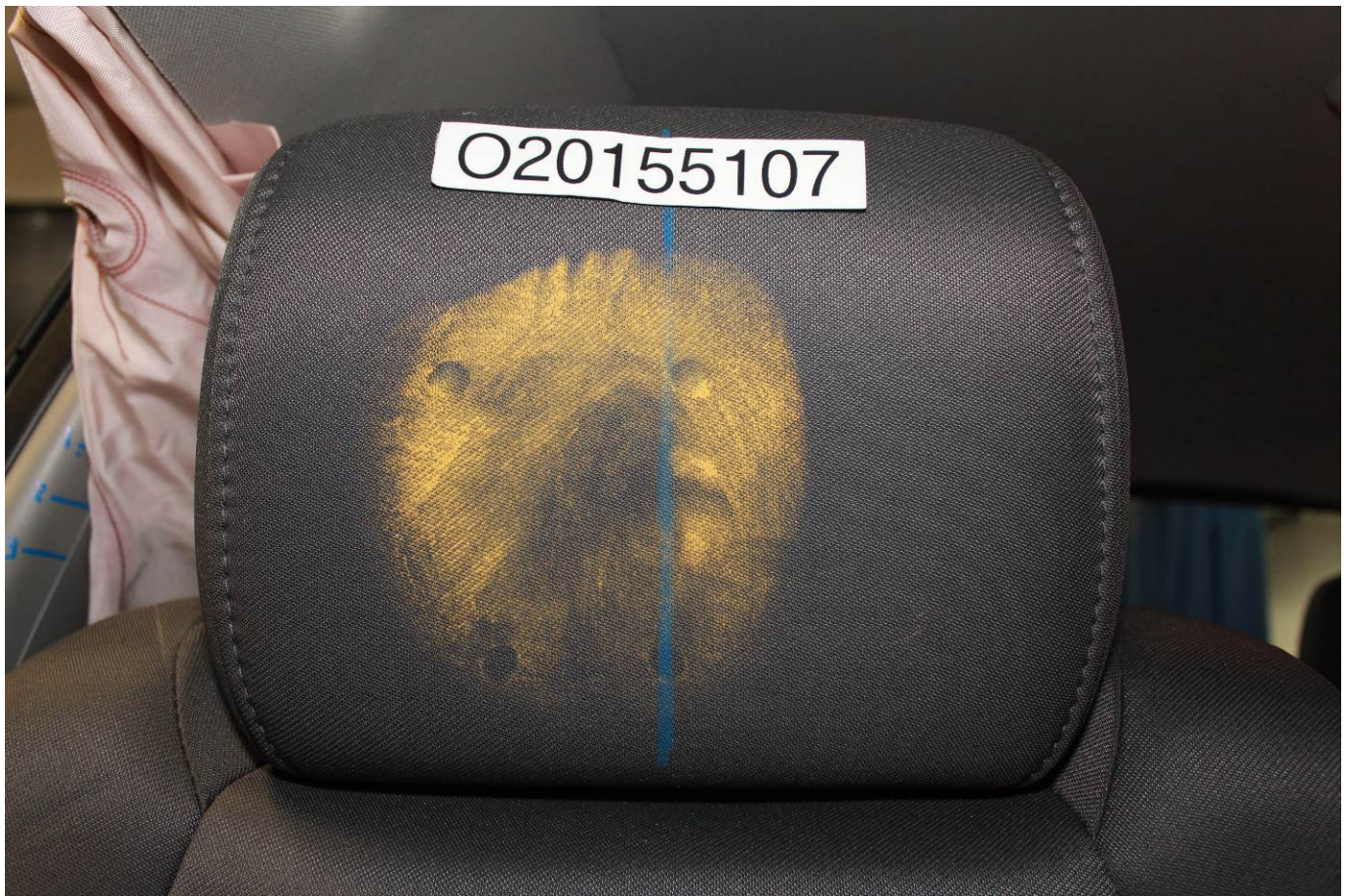
Post-Test Passenger Dummy Contact with Headrest
