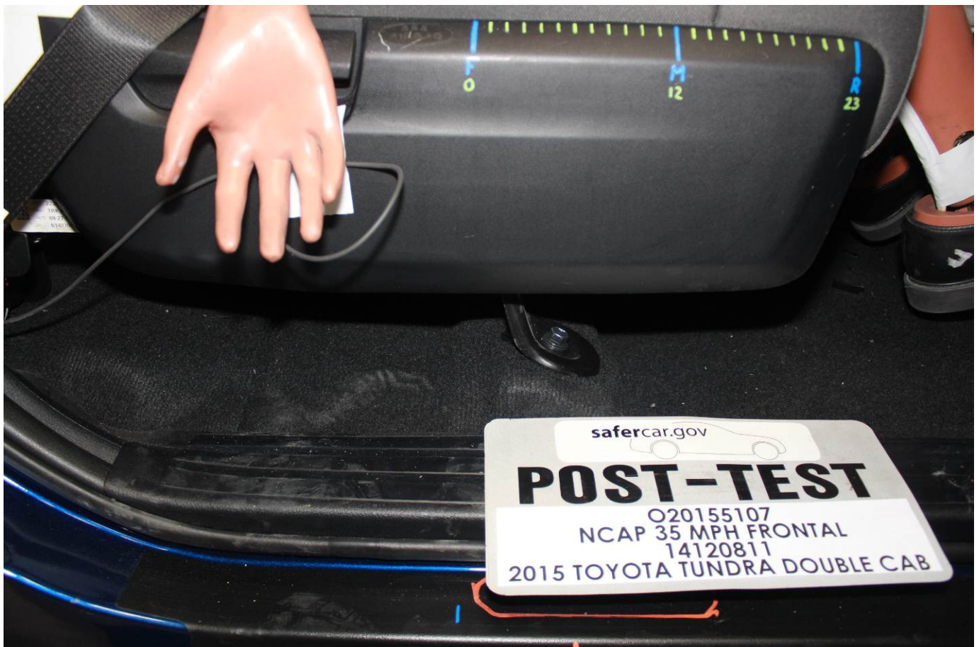
Post-Test Passenger's Seat Fore-Aft Markings
