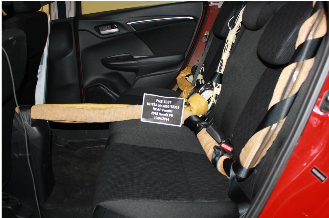
Figure A-27: Pre-Test Dummy Cable Routing
