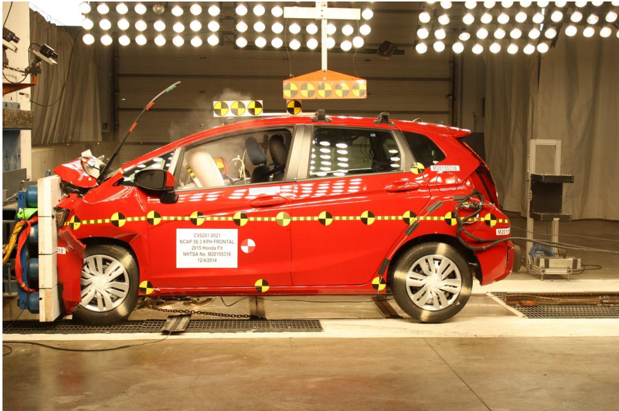
Figure A-77: 2015 Honda Fit Frontal Impact Event
