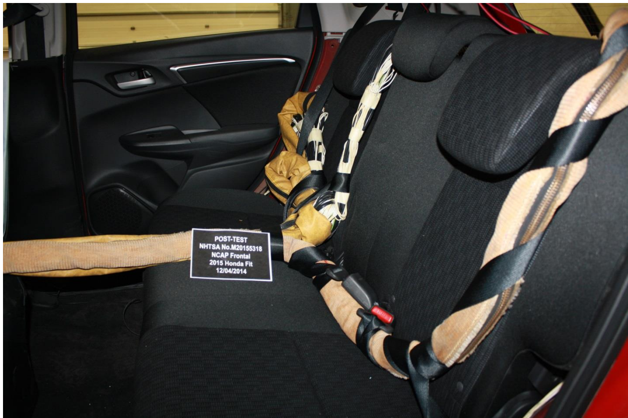
Figure A-28: Post-Test Dummy Cable Routing
