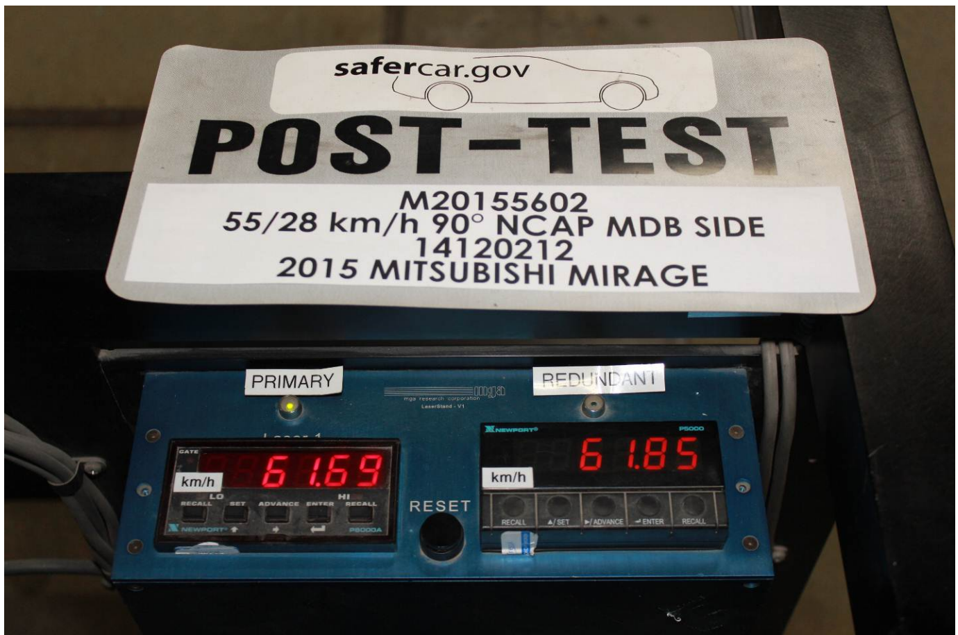
Post-Test Primary and Redundant Speed Trap Read-Out
