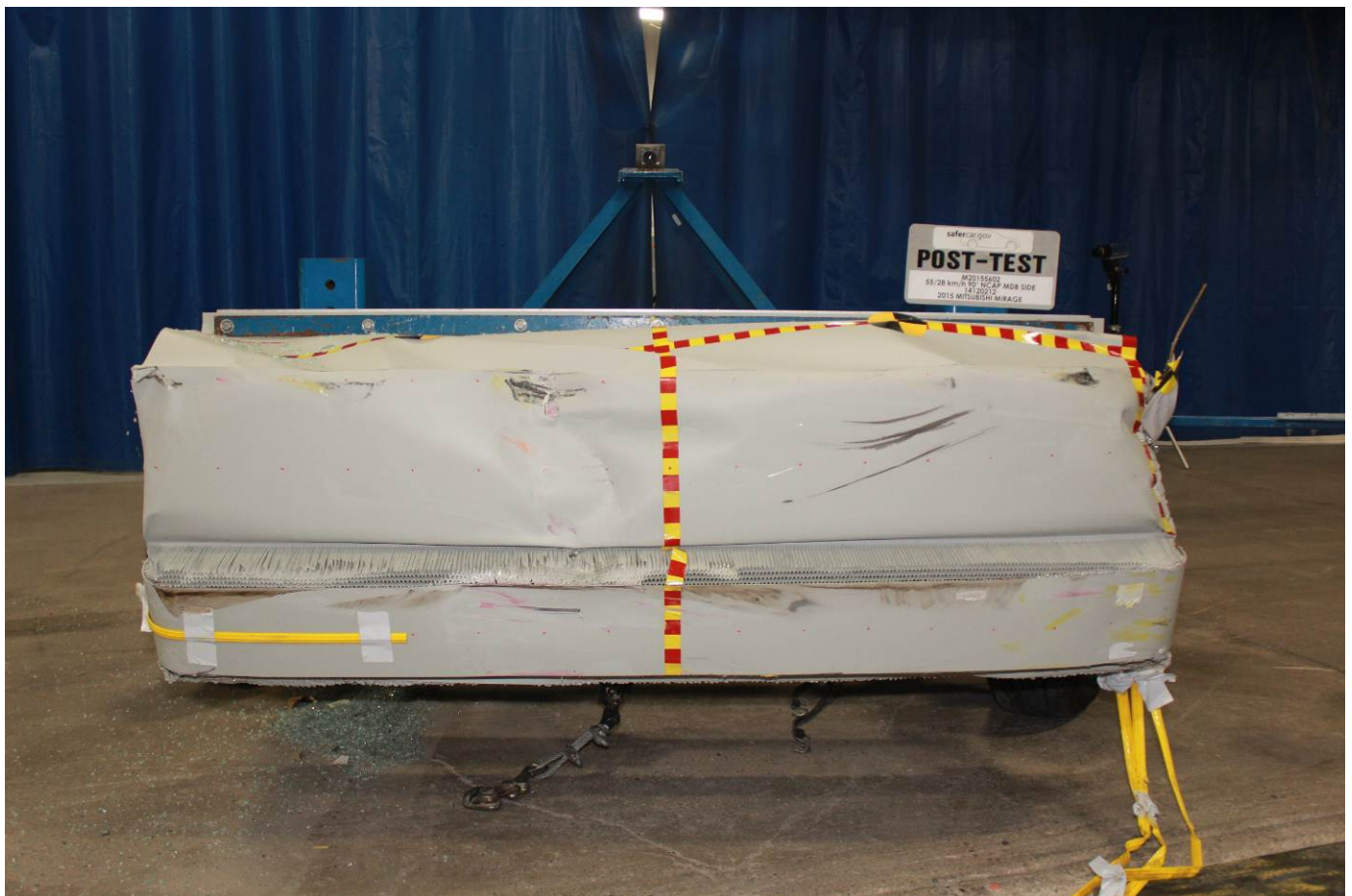
Post-Test Front View of MDB Impactor Face
