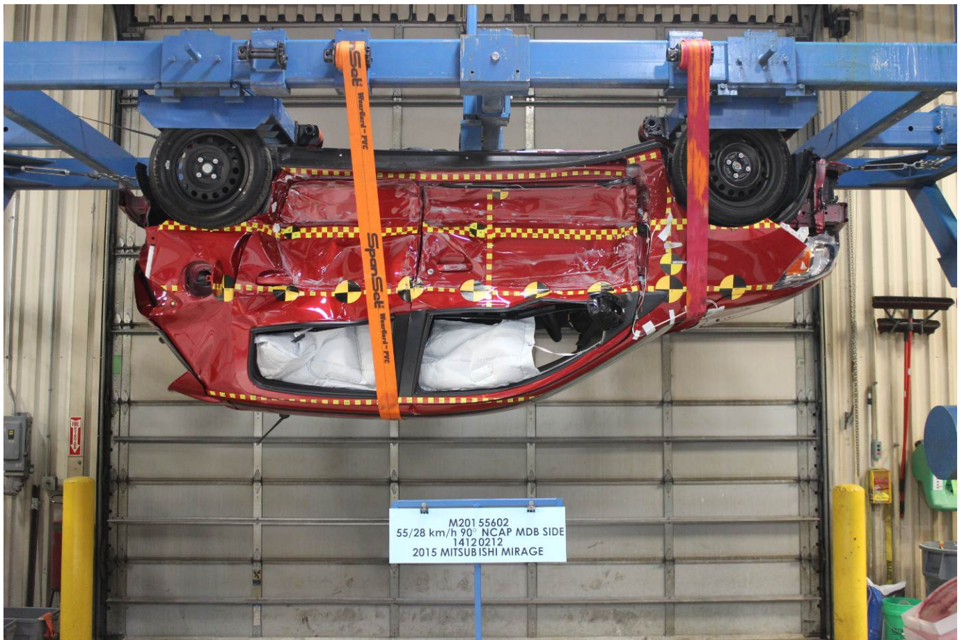
FMVSS No. 301 Static Rollover 180 Degrees
