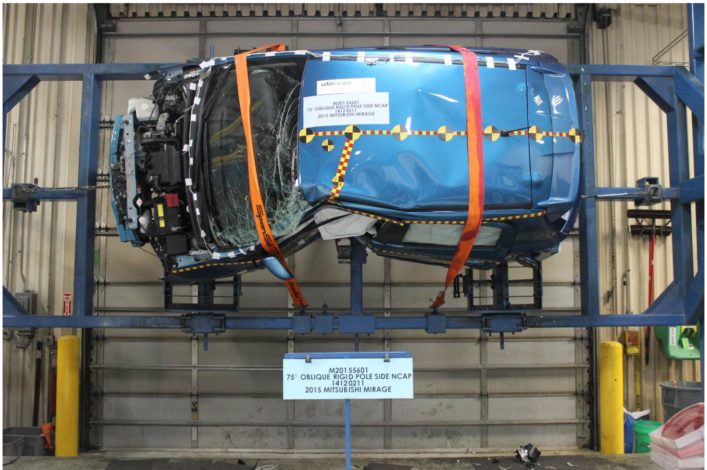
FMVSS No. 301 Static Rollover 90 Degrees
