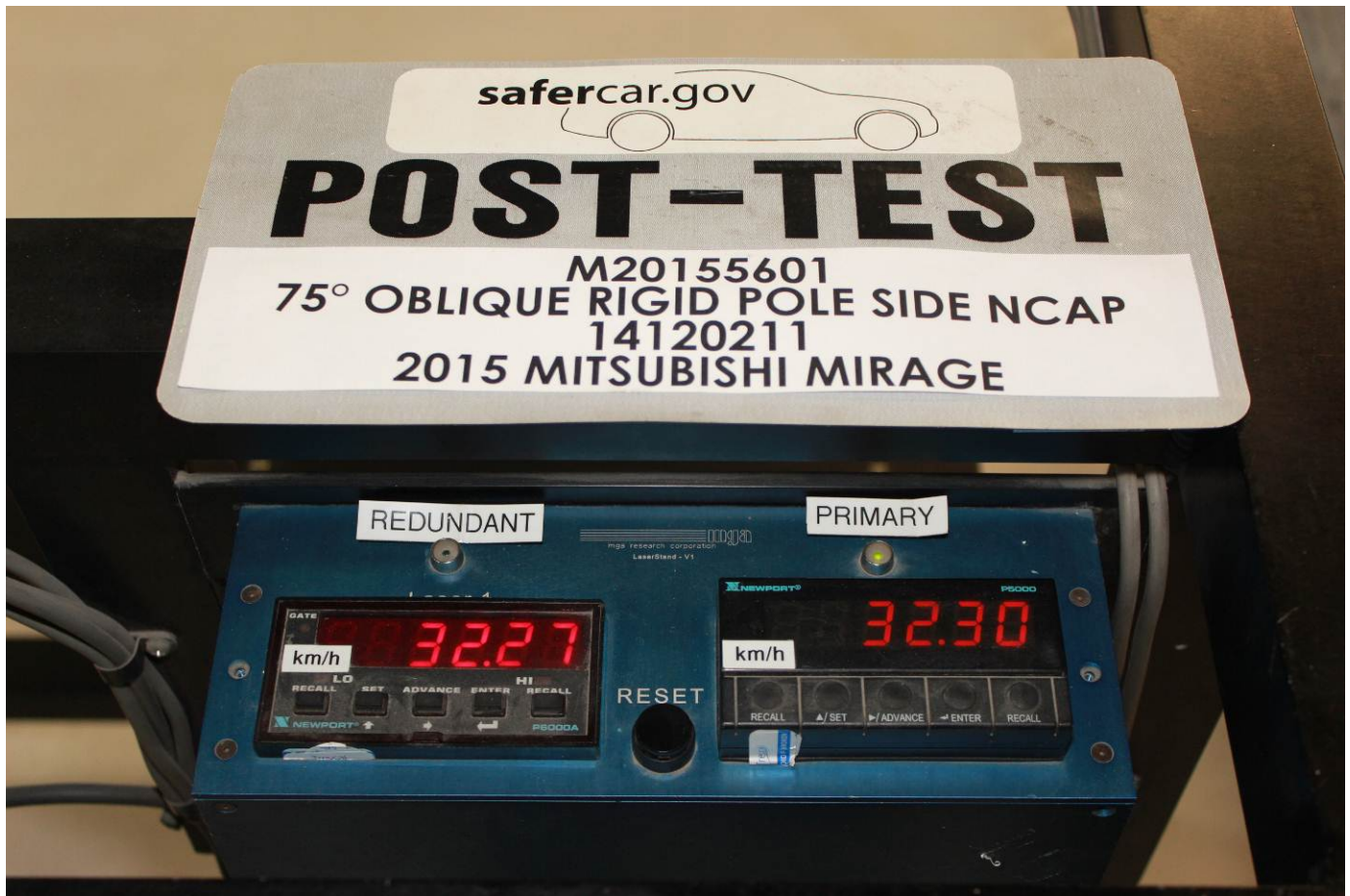
Post-Test Primary and Redundant Speed Trap Read-Out
