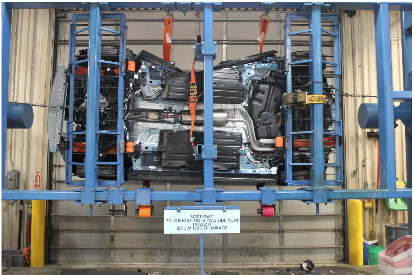
FMVSS No. 301 Static Rollover 270 Degrees
