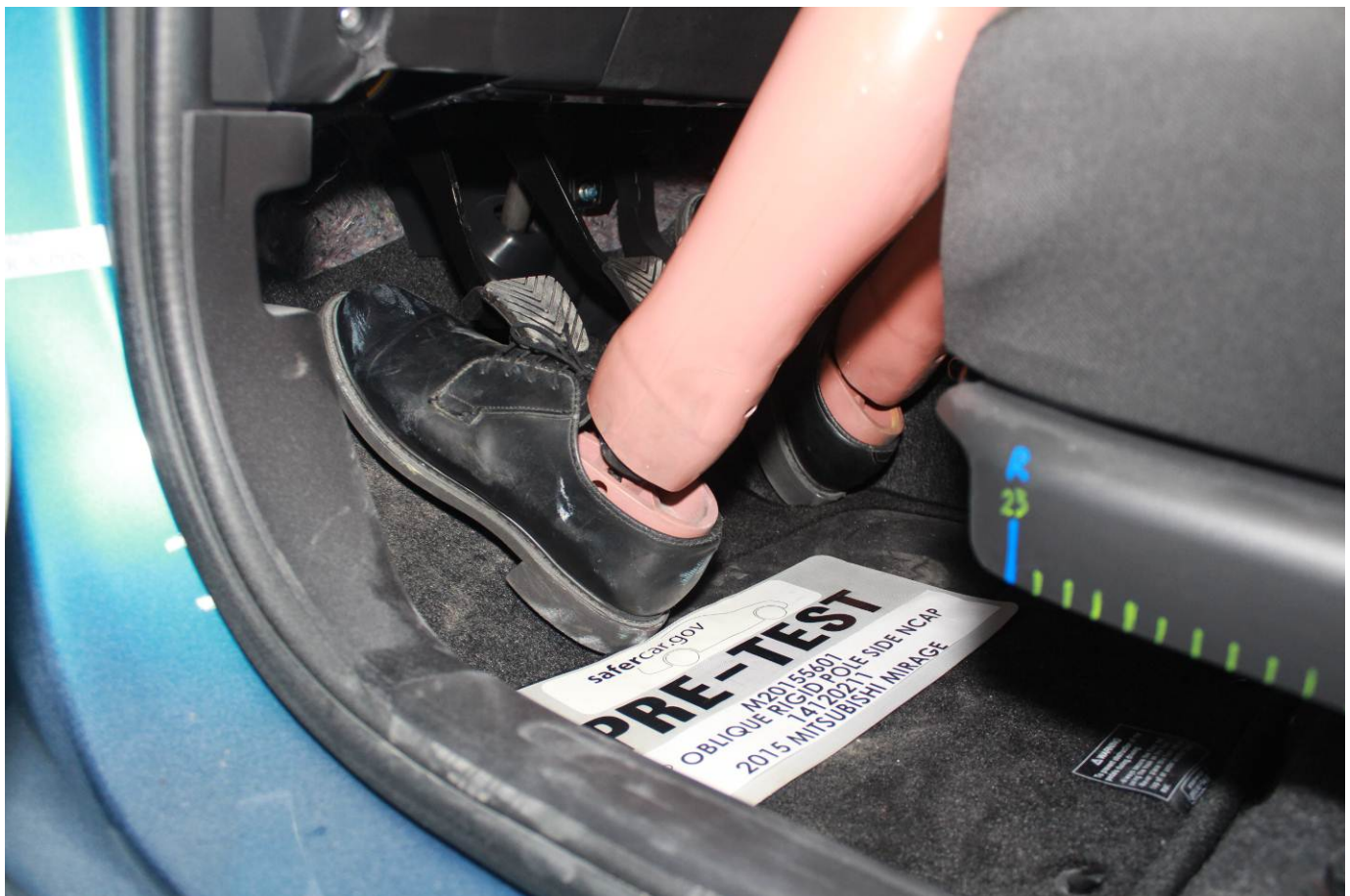
Pre-Test Placement of Dummy's Feet
