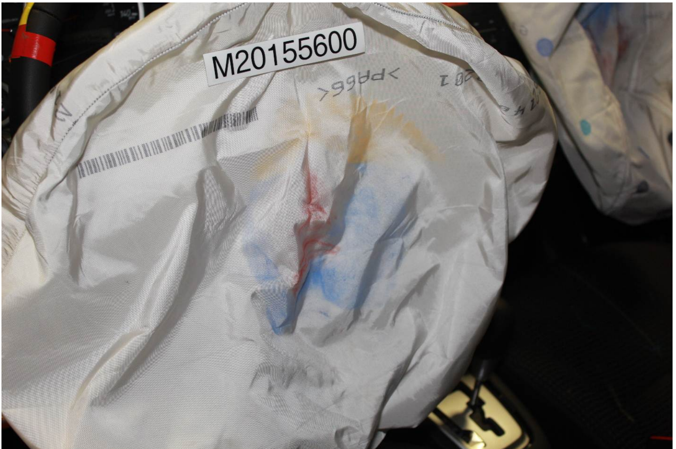
Post-Test Driver Dummy Contact with Airbag
