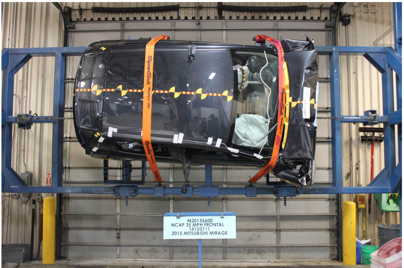
Vehicle at 270 Degrees on Static Rollover Device
