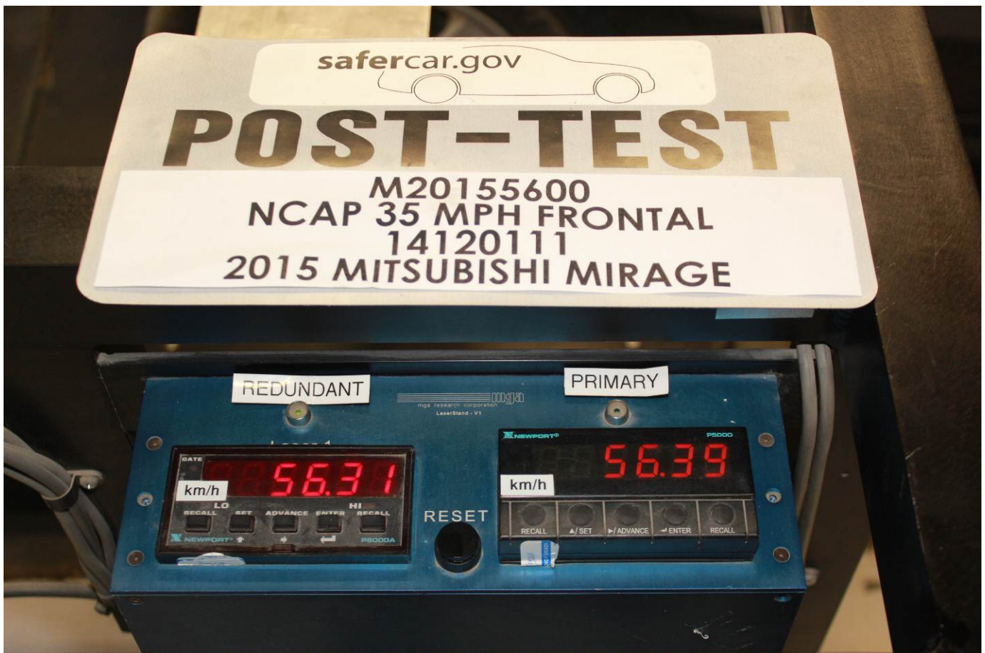
Post-Test Speed Trap Read-Out
