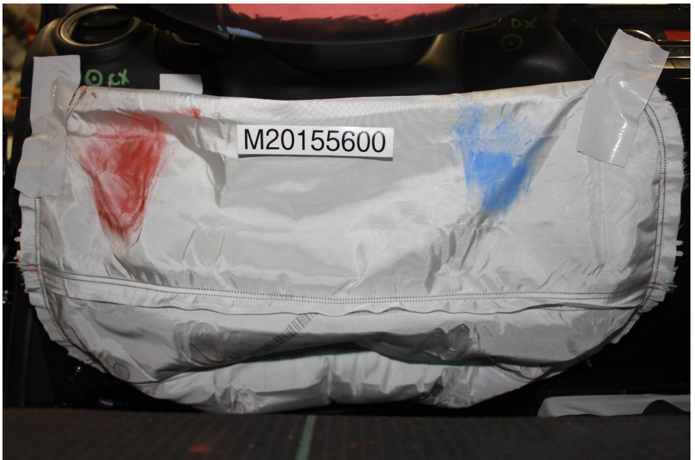
Post-Test Driver Dummy Contact with Knee Airbag
