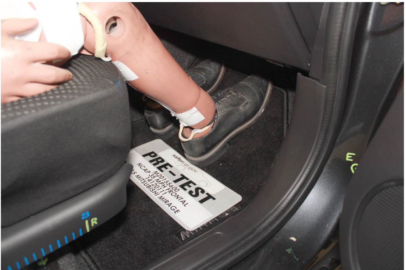
Pre-Test Passenger Dummy Feet
