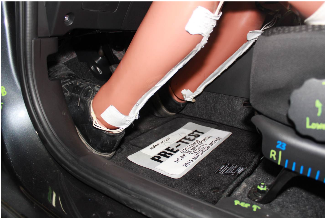
Pre-Test Driver Dummy Feet
