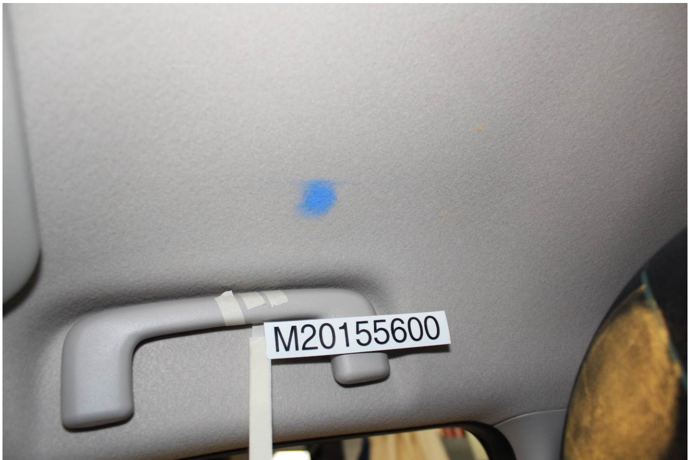
Post-Test Passenger Dummy Contact with Headliner
