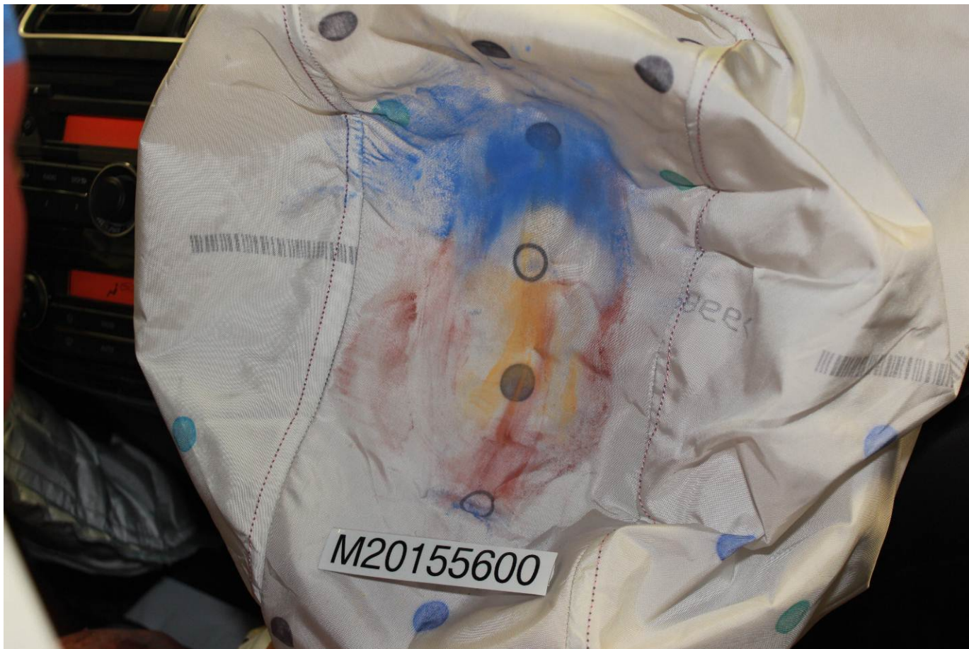
Post-Test Passenger Dummy Contact with Airbag
