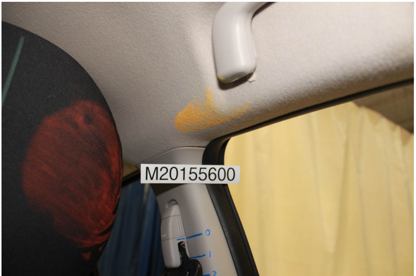
Post-Test Driver Dummy Contact with Headliner
