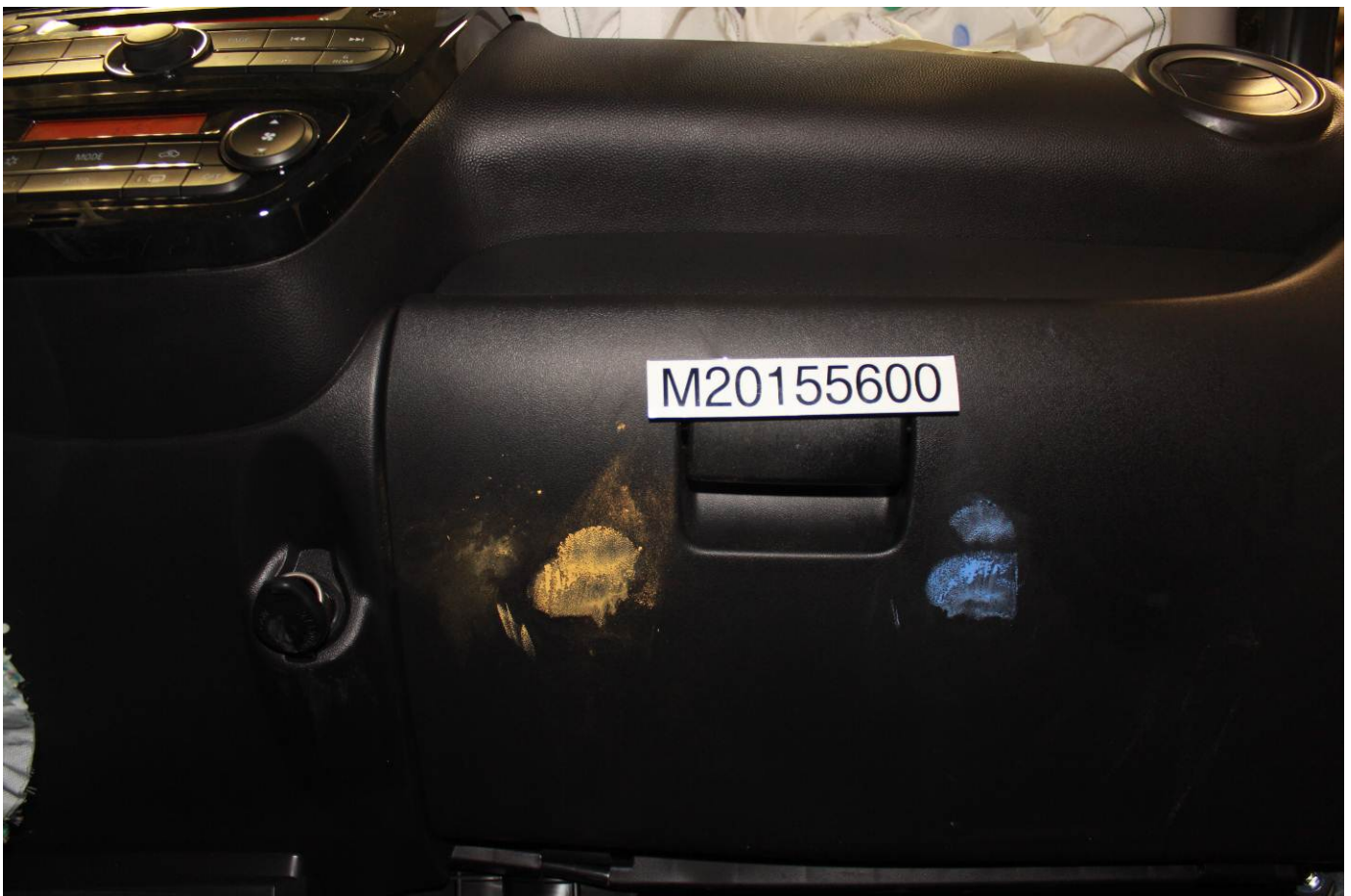
Post-Test Passenger Dummy Contact with Glovebox
