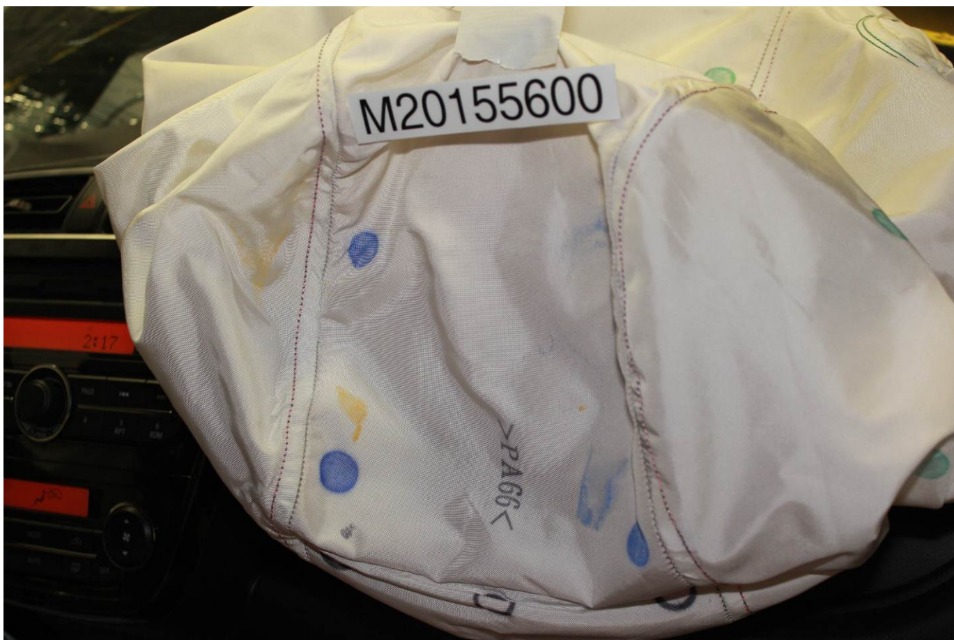
Post-Test Passenger Dummy Contact with Airbag
