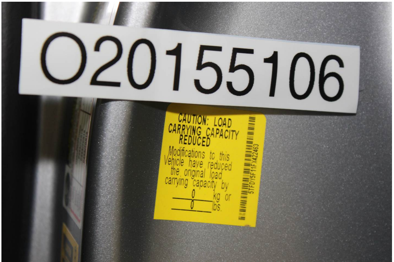
Load Carrying Capacity Reduced Label
