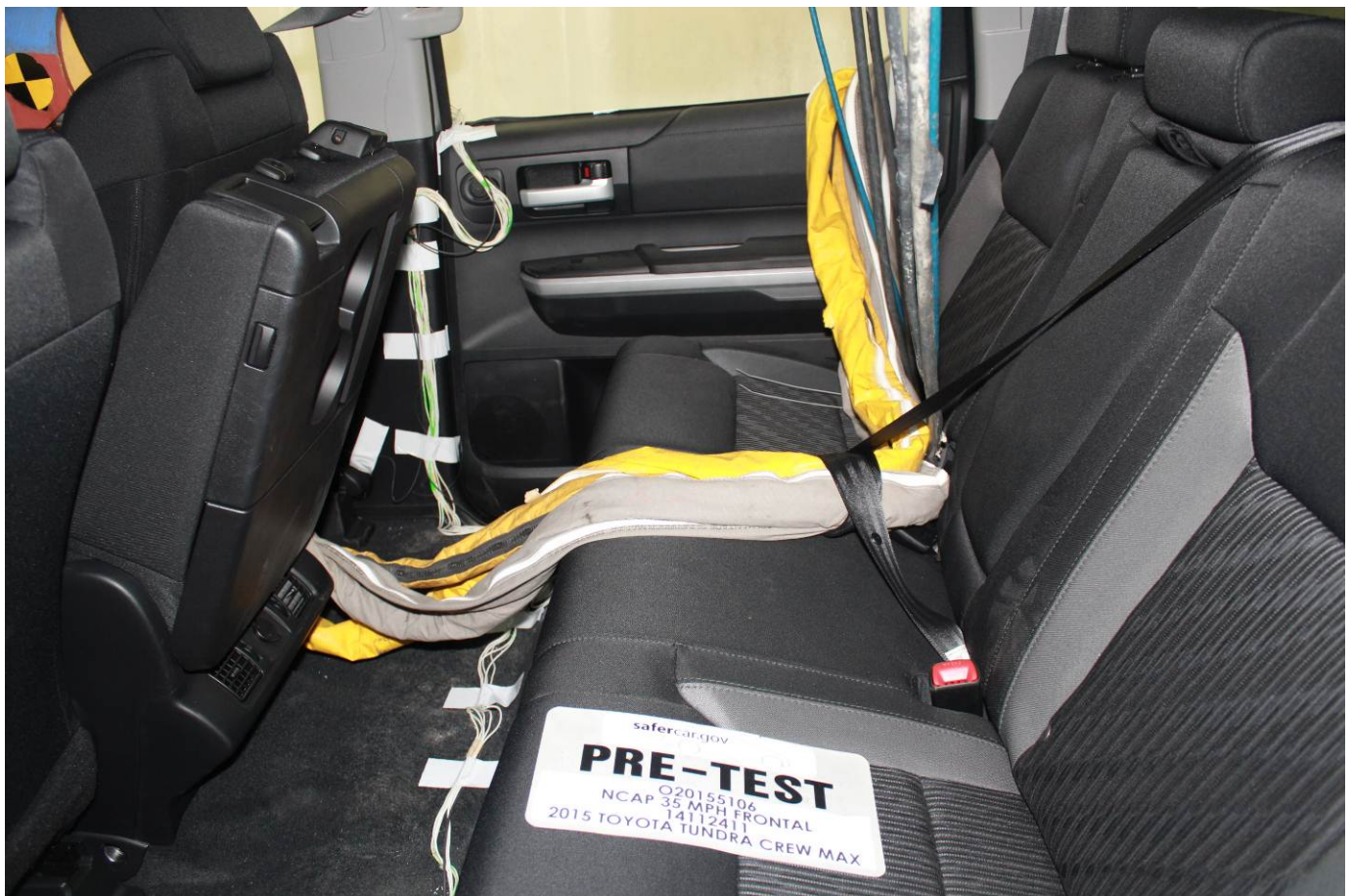
Pre-Test Dummy Cable Routing
