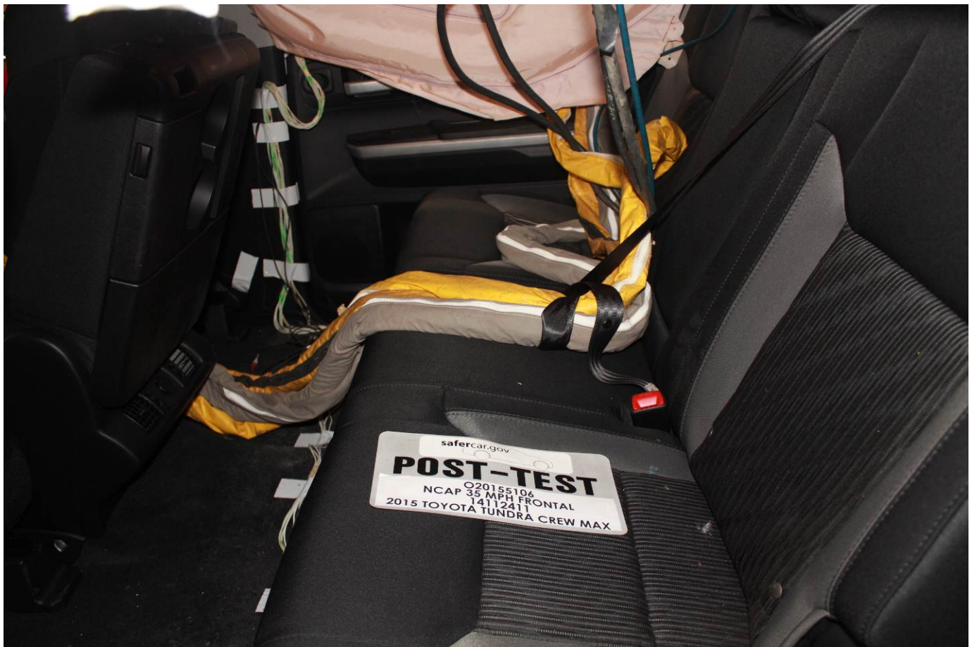
Post-Test Dummy Cable Routing
