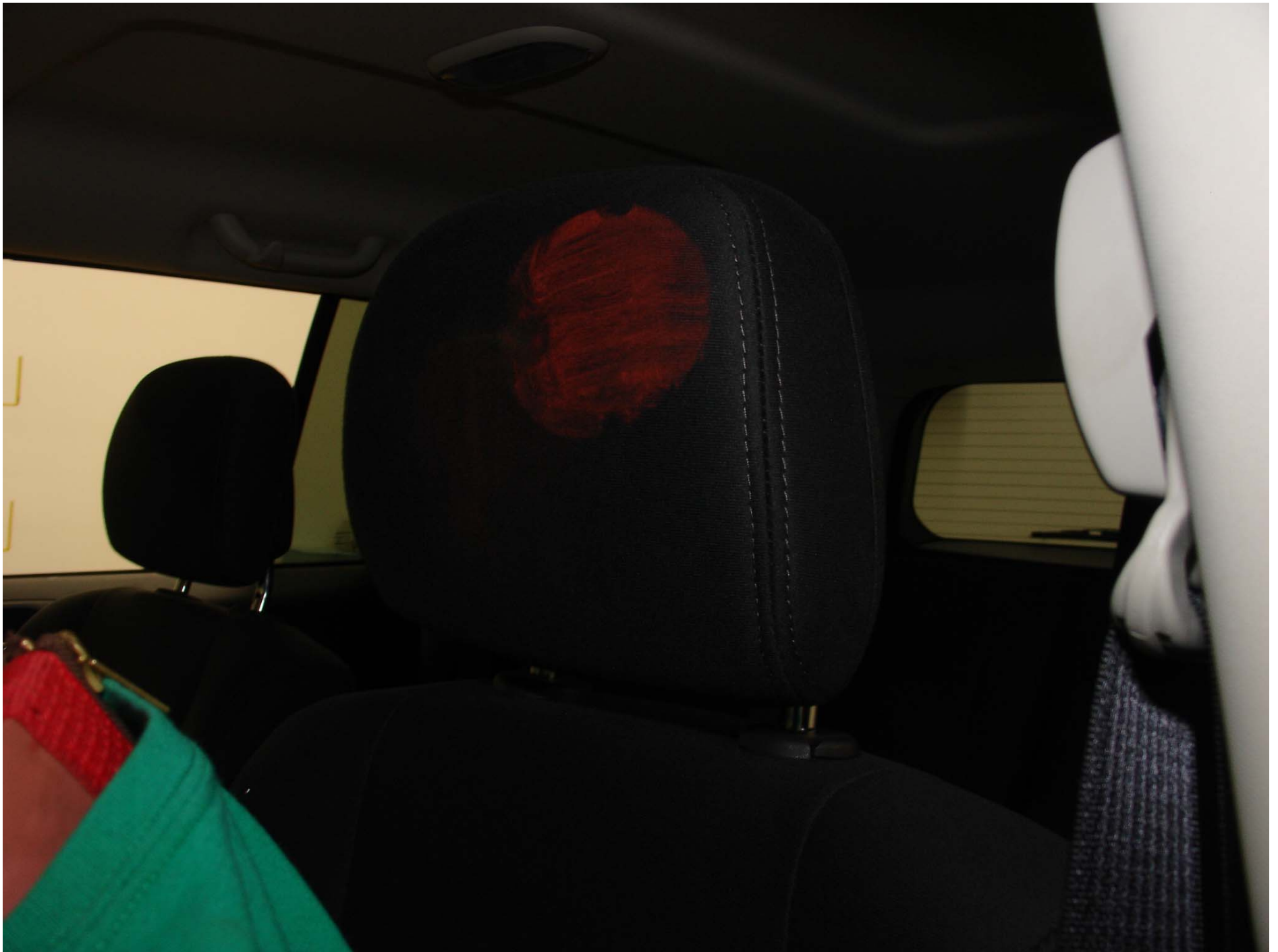
Photo No. 14 - Post-Test 5th Fem. P2 Driver Dummy Head Contact (headrest)
