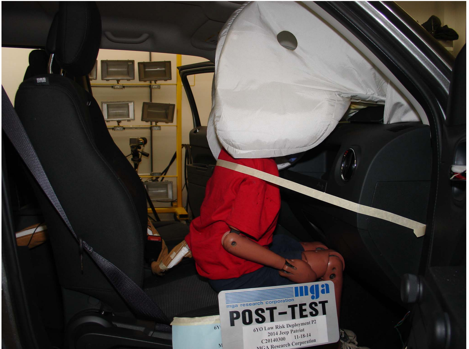
Photo No. 39 - Post-Test 6YO P2 Passenger Dummy Right Side View
