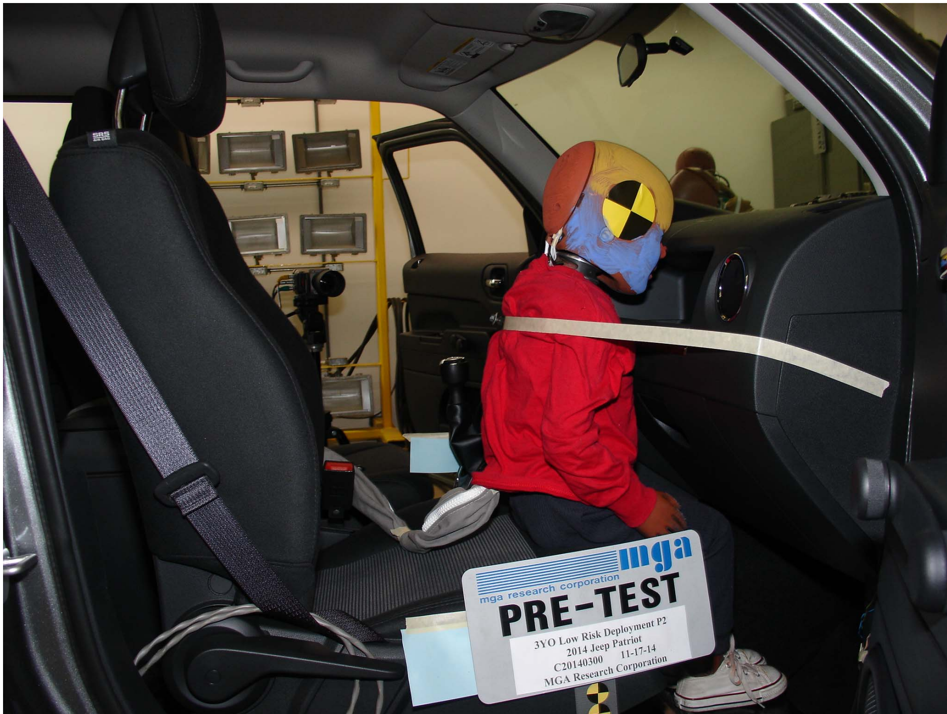
Photo No. 24 - Pre-Test 3YO P2 Passenger Dummy Right Side View
