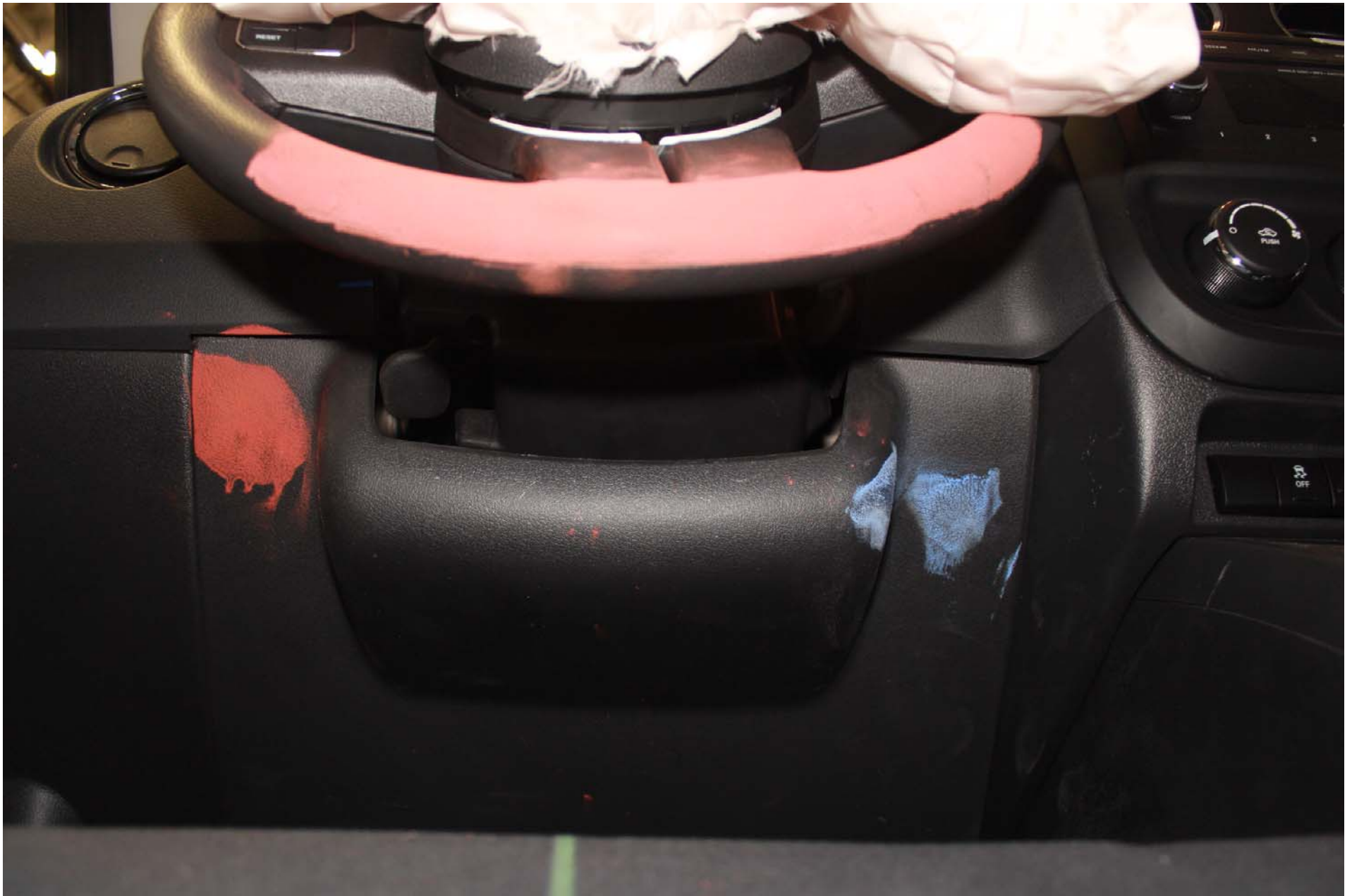
Photo No. 47 - Post-Test Driver Dummy Knee Contact (knee bolster)
