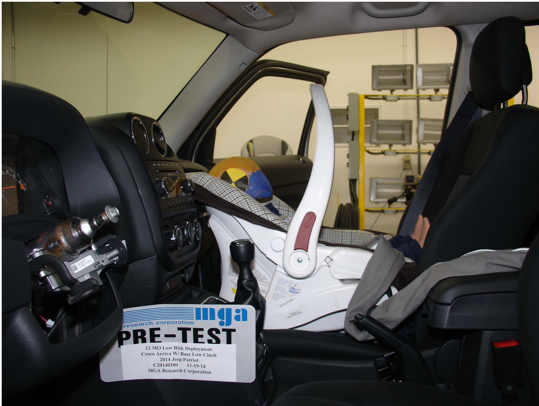
Photo No. 60 - Pre-Test 12 Mo Pass. Dummy Left Side View (Cosco Arriva W- Base Low Cinch)
