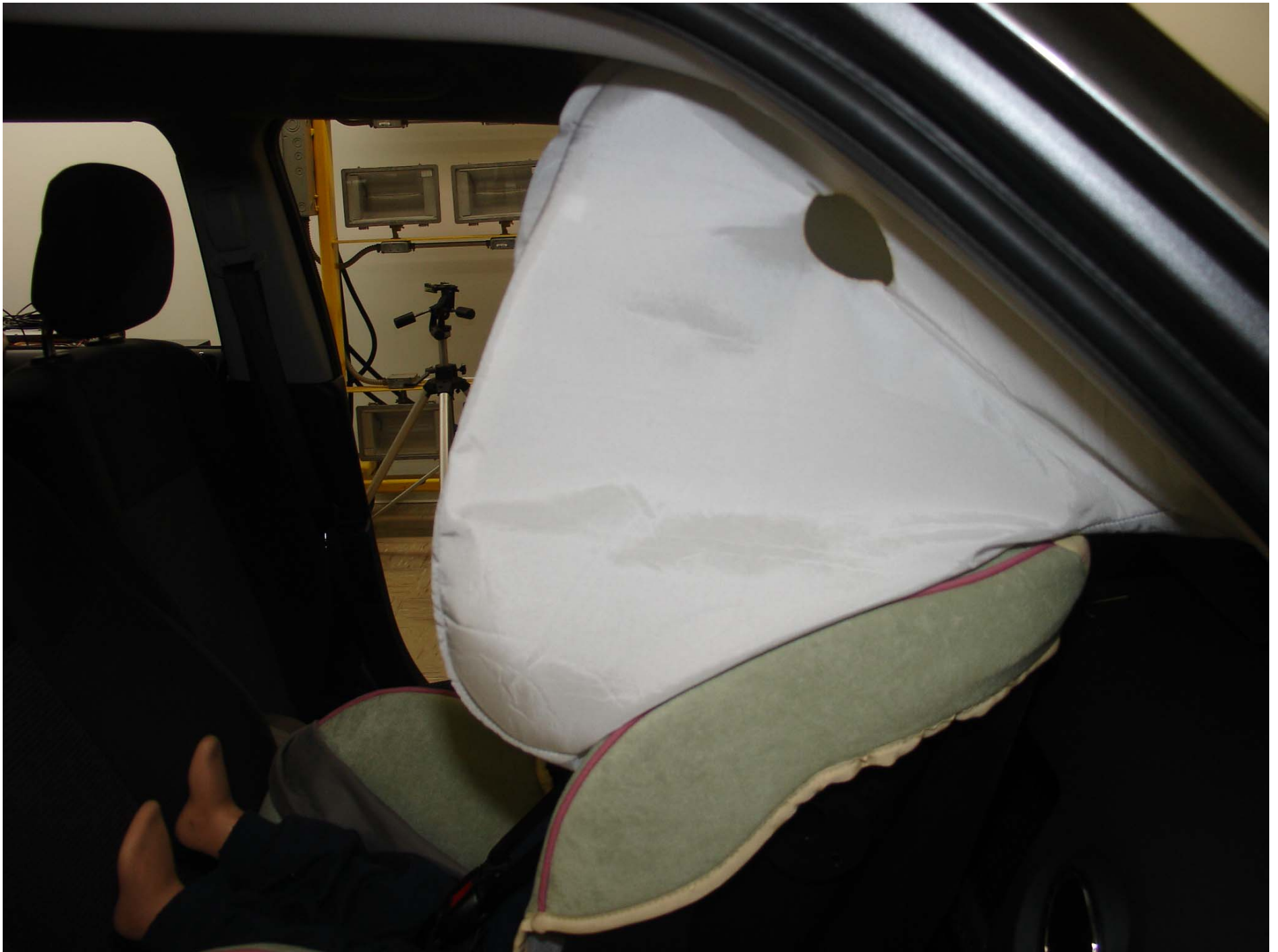
Photo No. 71 - Post-Test 12 Mo Pass. Dummy Airbag Right Side View (Evenflo Tribute Low Cinch)
