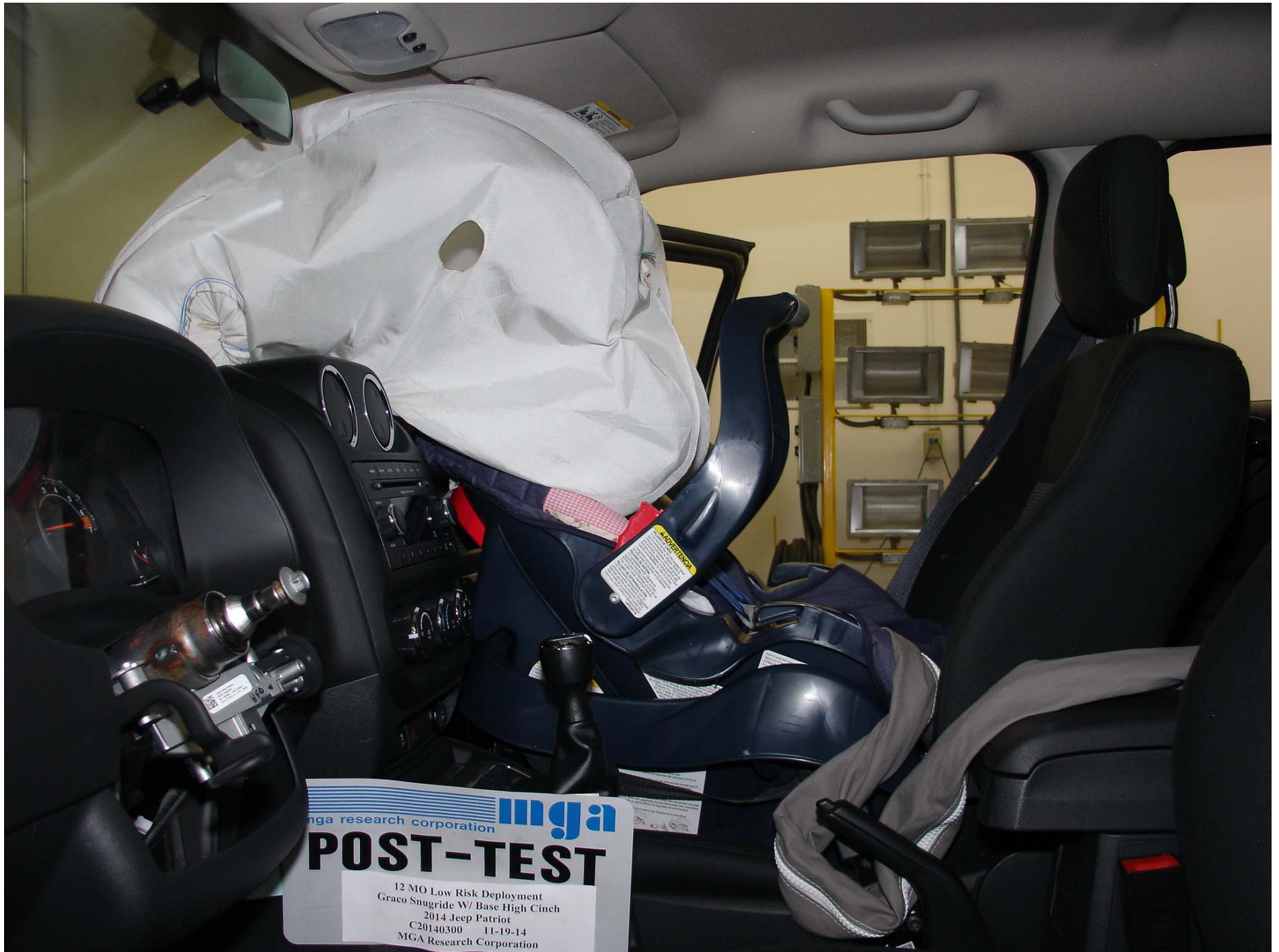
Photo No. 49 - Post-Test 12 Mo Pass. Dummy Left Side View (Graco Snugride W- Base High Cinch)
