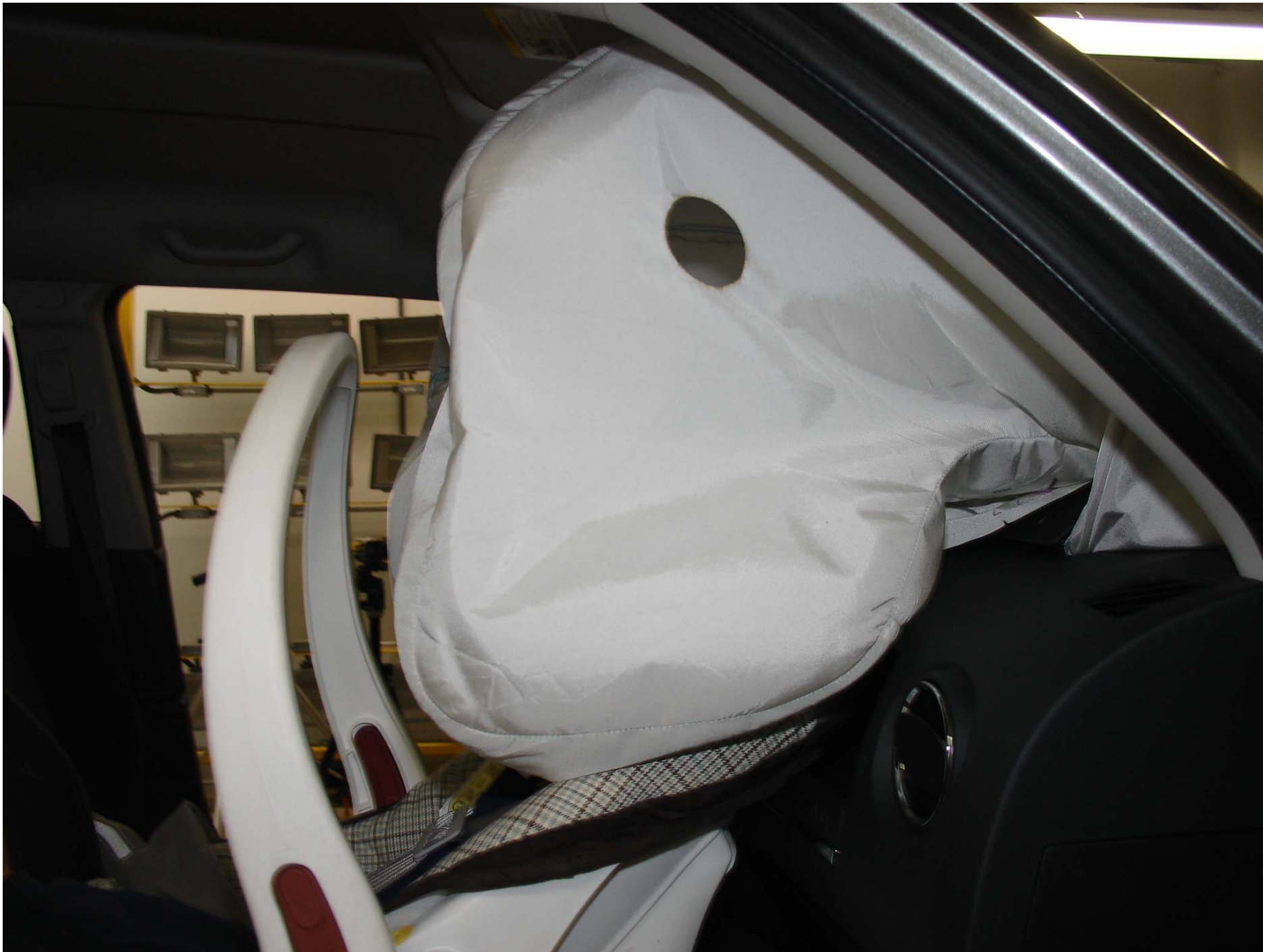
Photo No. 65 - Post-Test 12 Mo Pass. Dummy Airbag Right Side View (Cosco Arriva W- Base Low Cinch)
