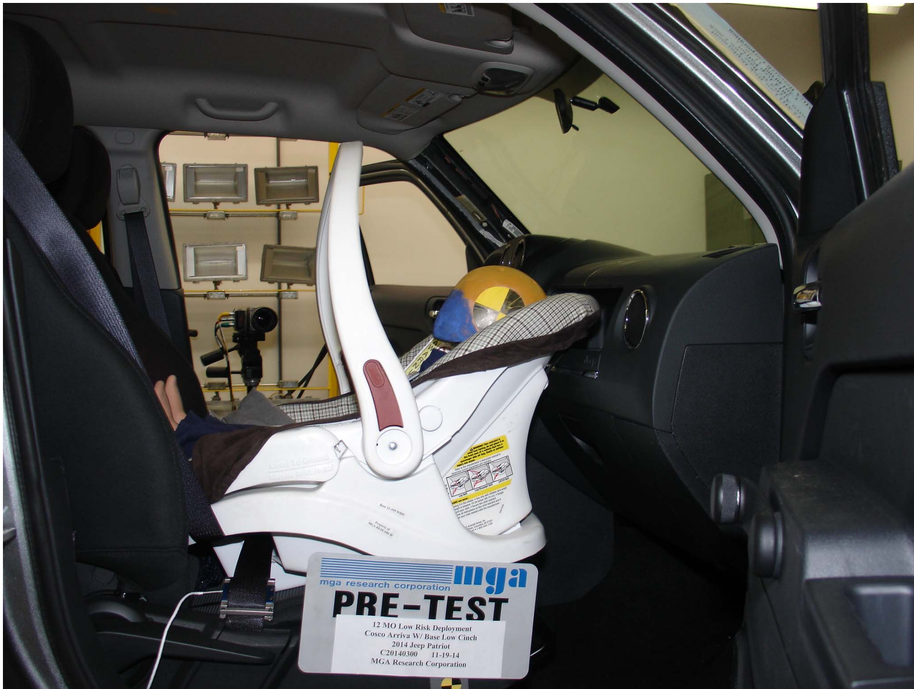
Photo No. 62 - Pre-Test 12 Mo Pass. Dummy Right Side View (Cosco Arriva W- Base Low Cinch)
