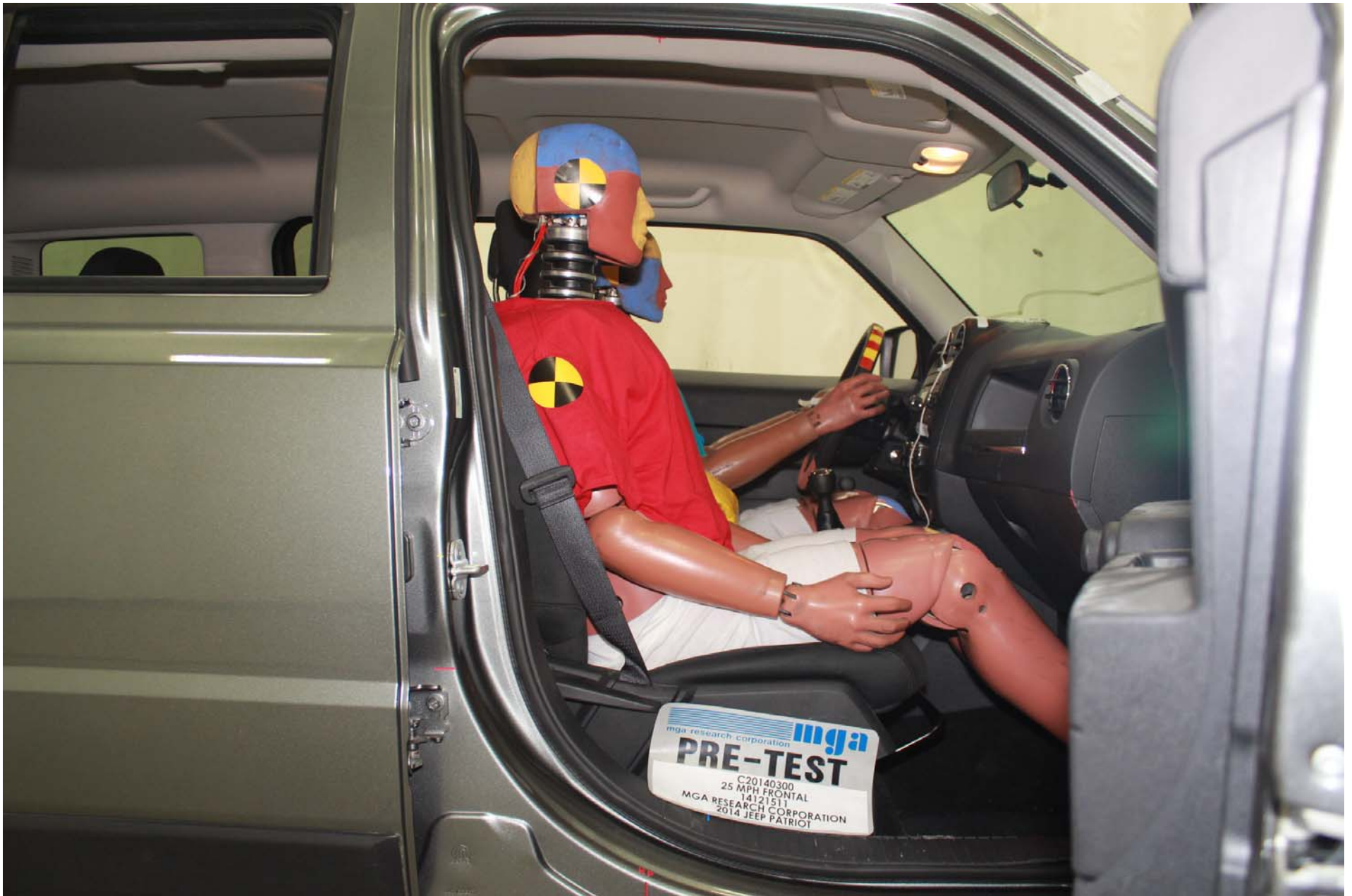
Photo No. 52 - Pre-Test Passenger Dummy Position Right Side View (door open)
