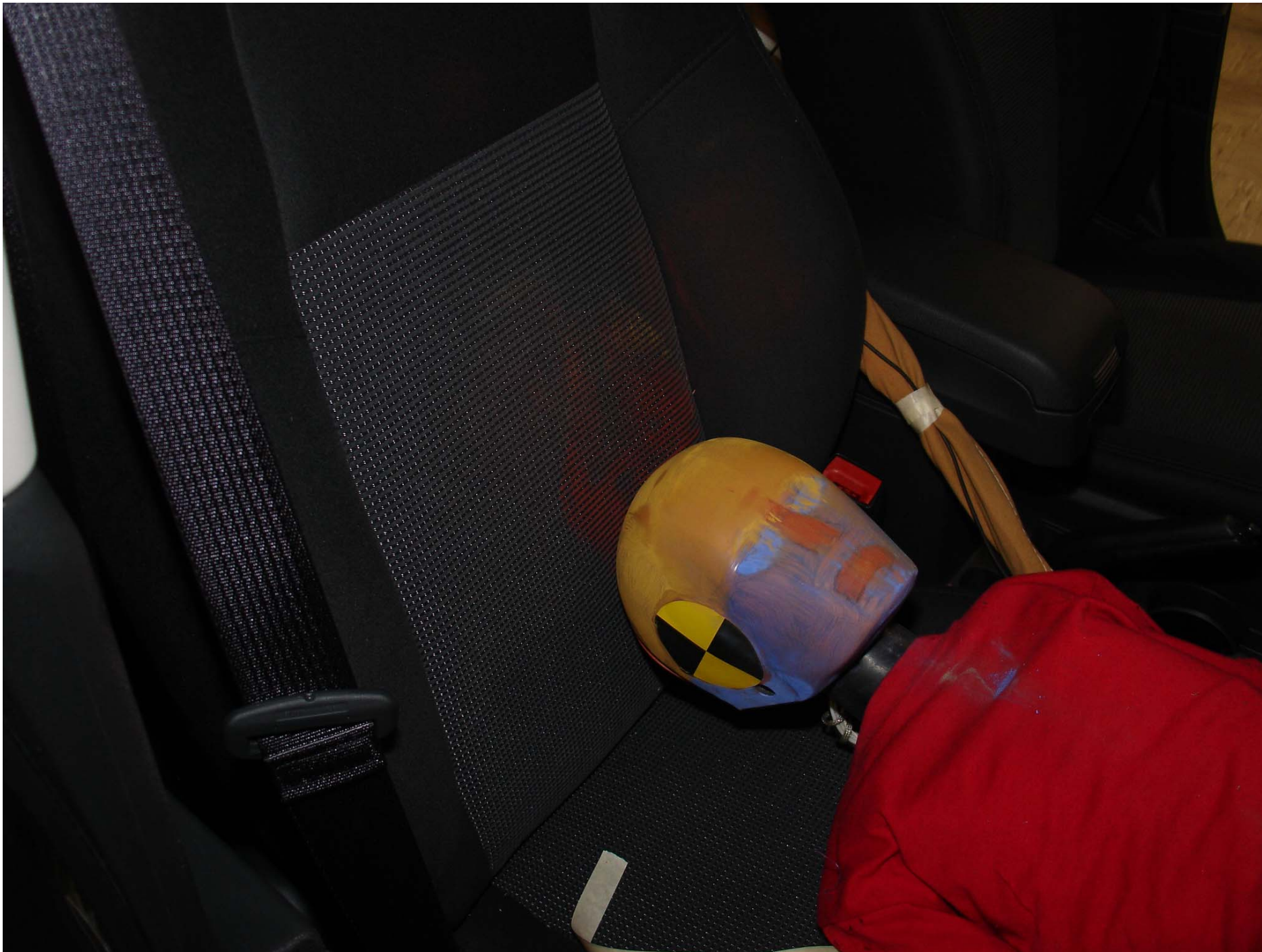
Photo No. 35 - Post-Test 6YO P1 Passenger Dummy Head Contact (seat back)
