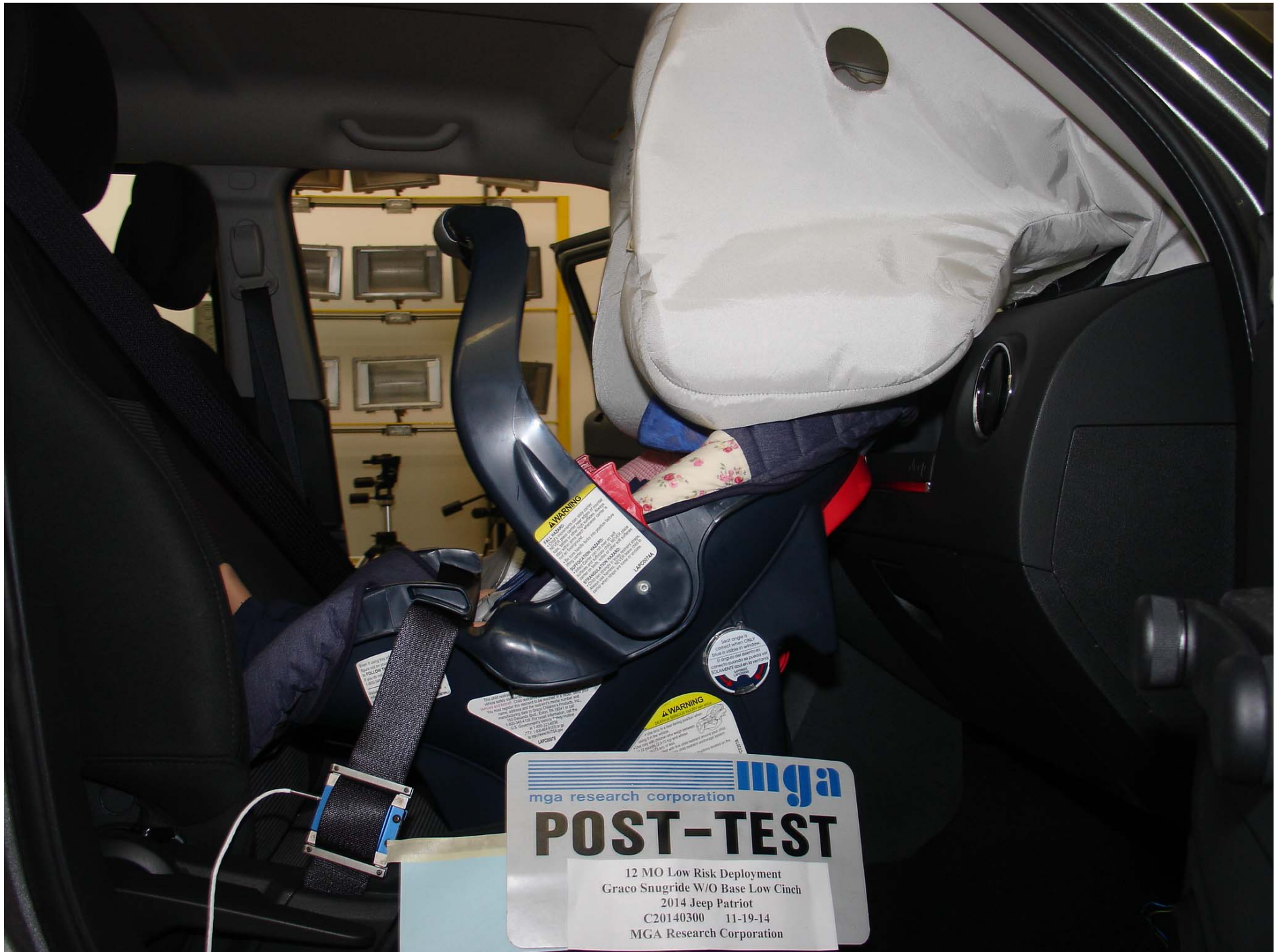
Photo No. 45 - Post-Test 12 Mo Pass. Dummy Right Side View (Graco Snugride W-O Base Low Cinch)
