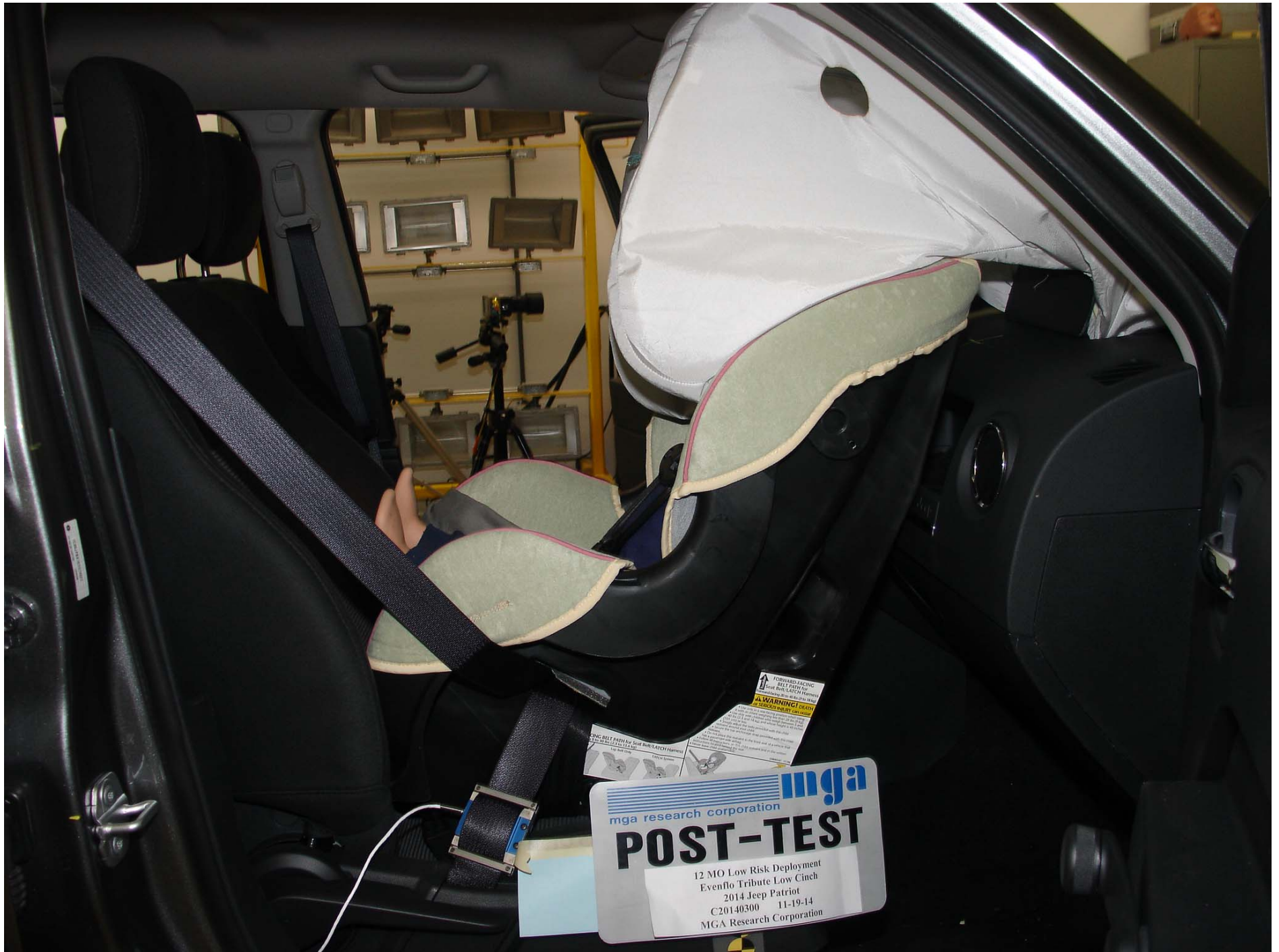
Photo No. 69 - Post-Test 12 Mo Pass. Dummy Right Side View (Evenflo Tribute Low Cinch)
