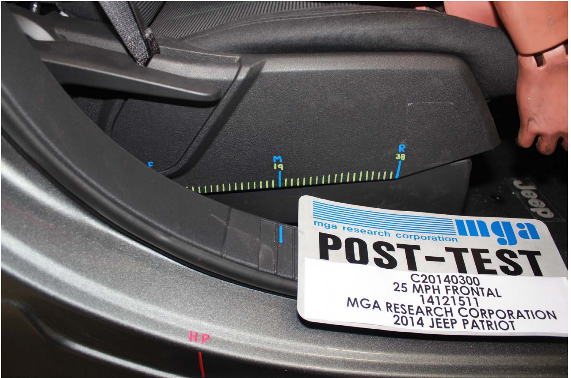
Photo No. 55 - Post-Test Passenger Dummy Seat Position
