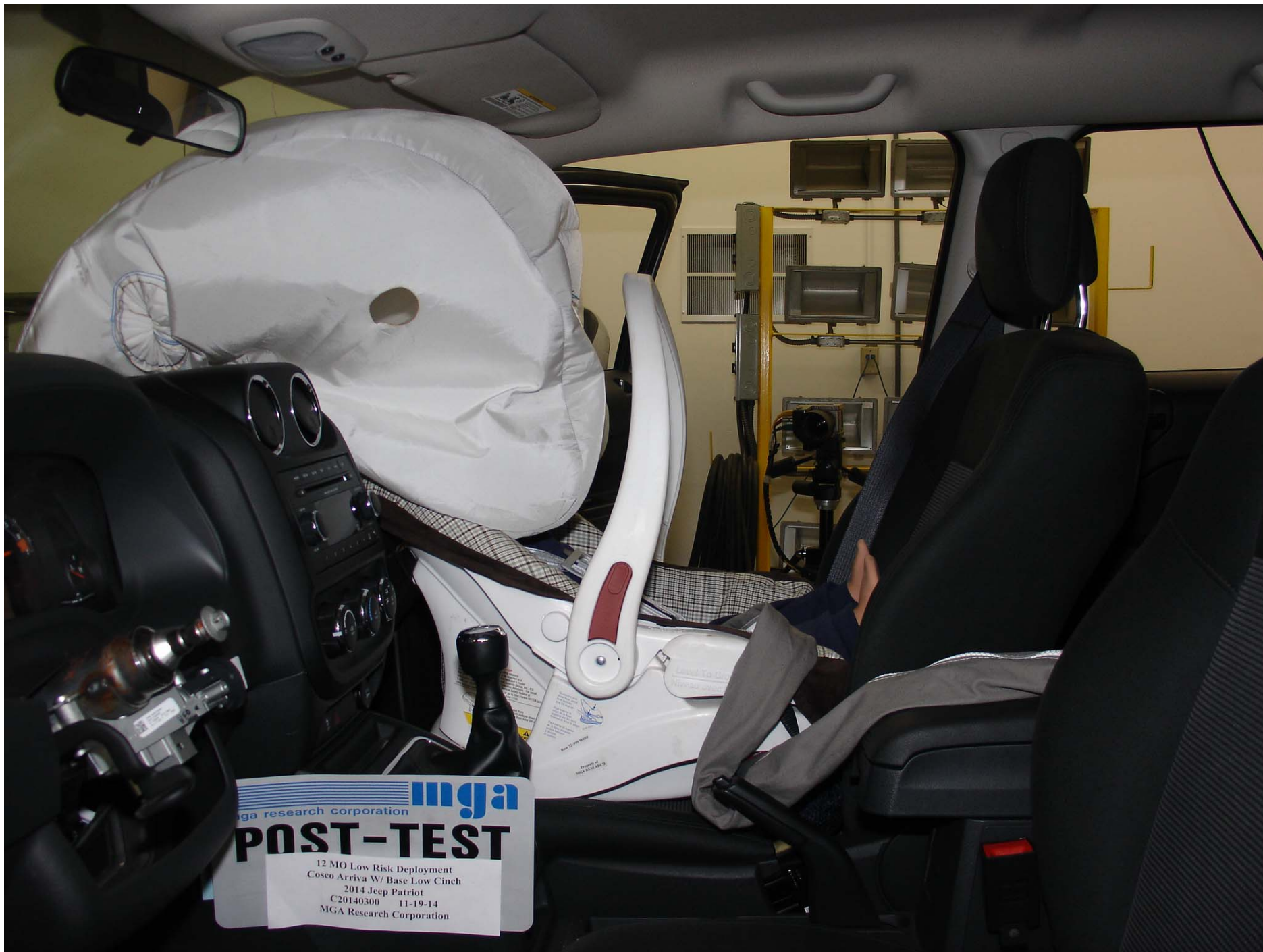
Photo No. 61 - Post-Test 12 Mo Pass. Dummy Left Side View (Cosco Arriva W- Base Low Cinch)
