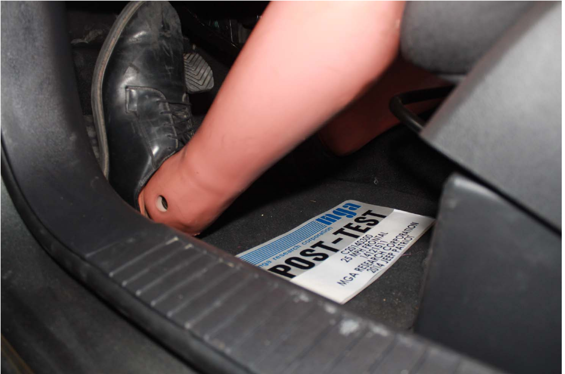
Photo No. 42 - Post-Test Driver Dummy Feet Position
