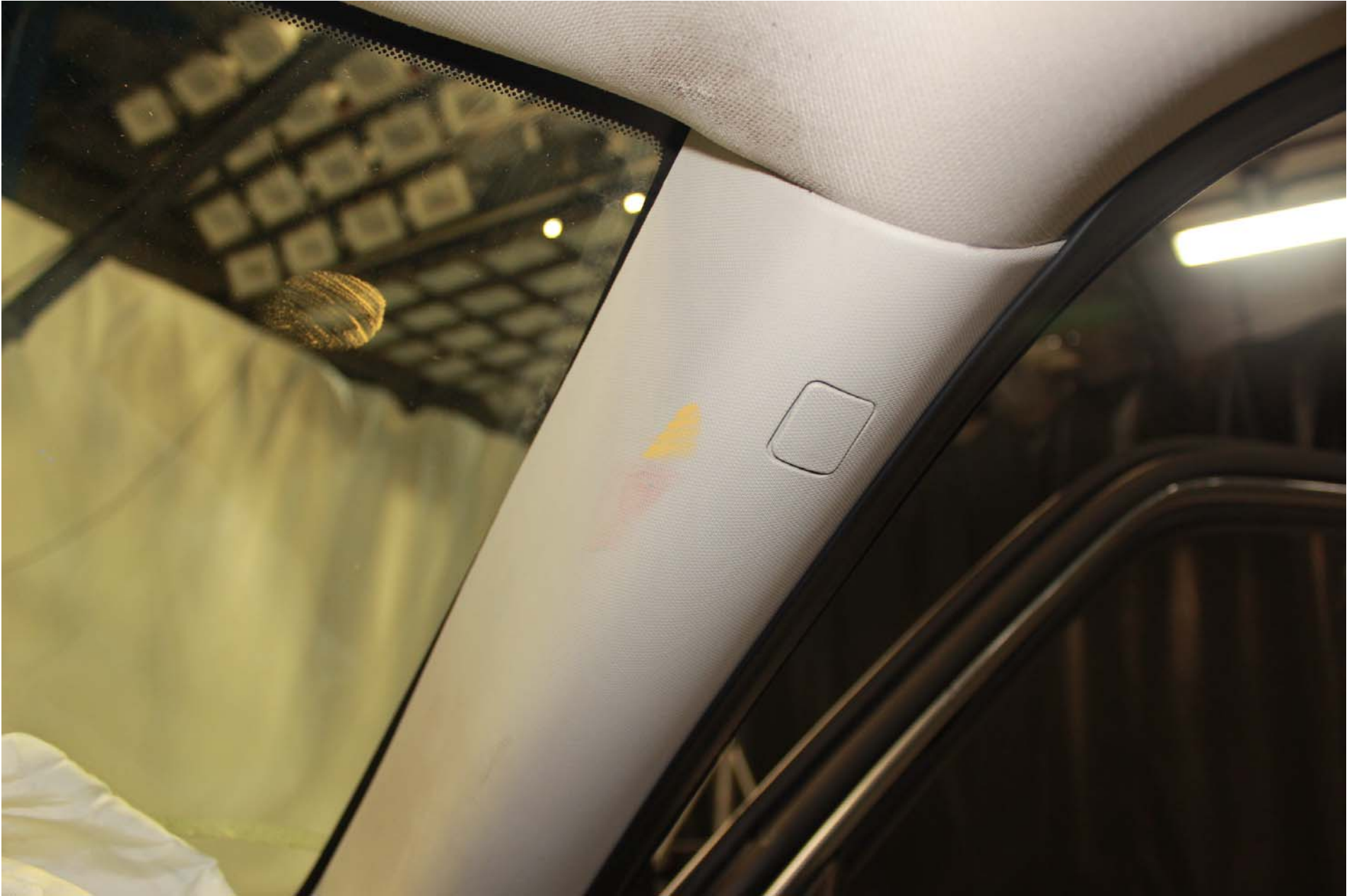
Photo No. 61 - Post-Test Passenger Dummy Head Contact (A-pillar, windshield)
