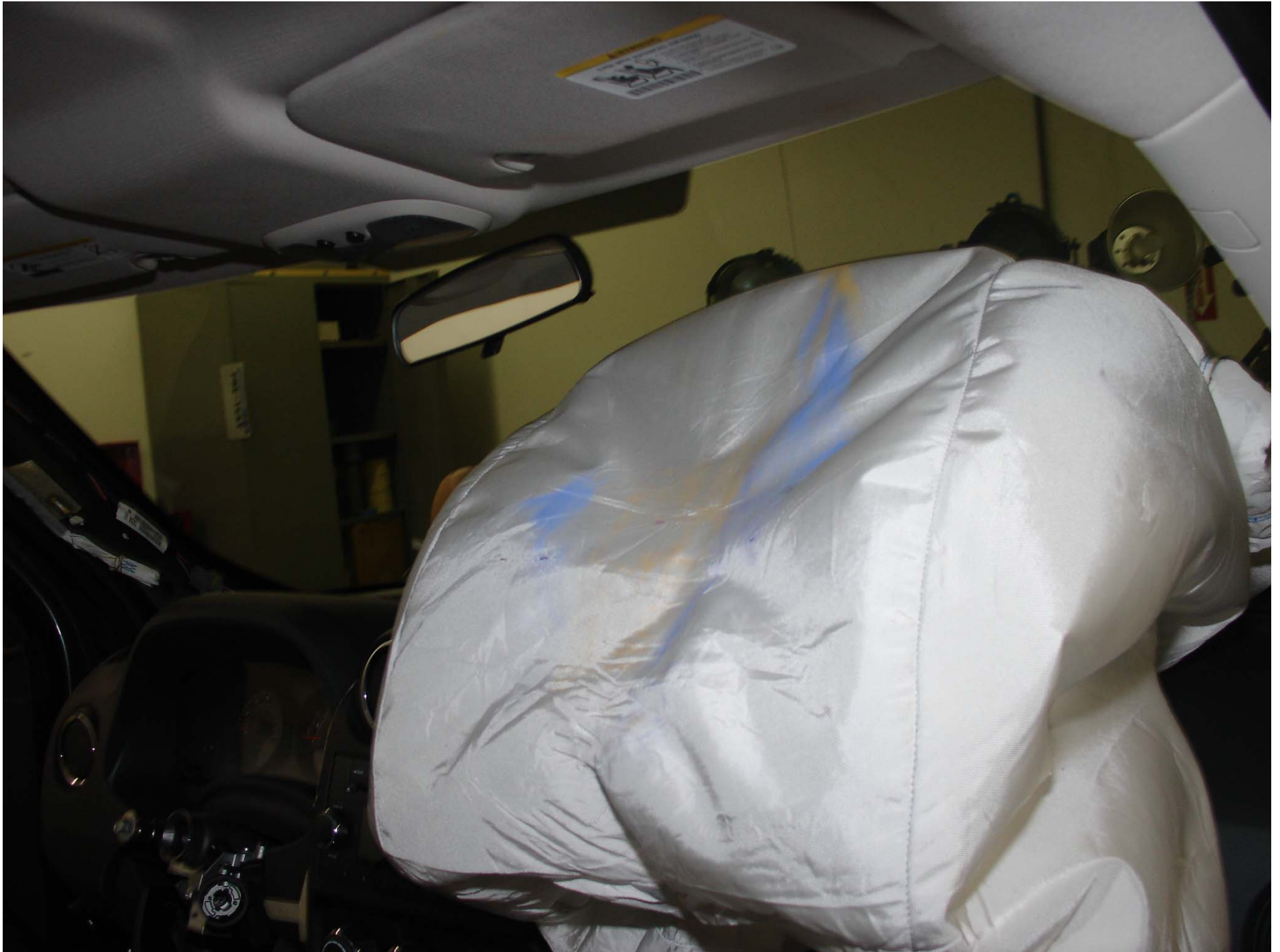
Photo No. 34 - Post-Test 6YO P1 Passenger Dummy Airbag Right Side View
