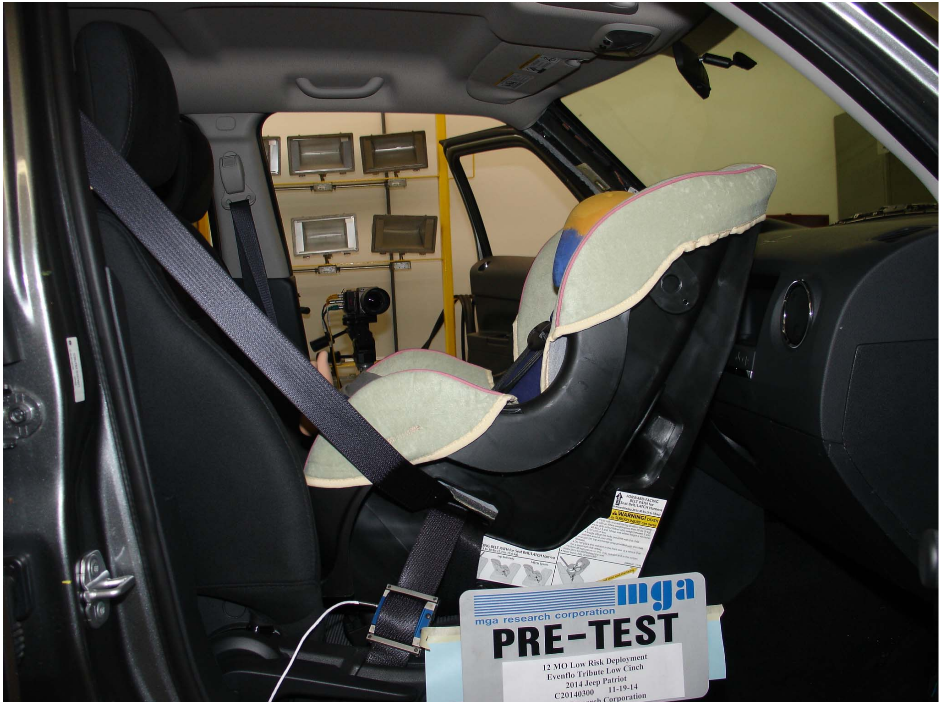
Photo No. 68 - Pre-Test 12 Mo Pass. Dummy Right Side View (Evenflo Tribute Low Cinch)
