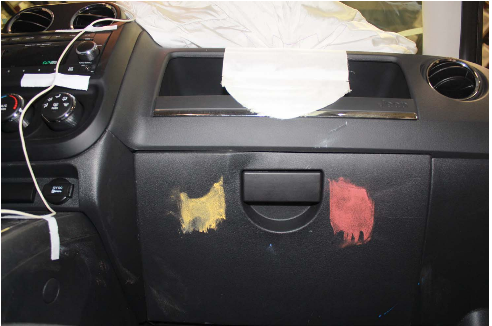
Photo No. 62 - Post-Test Passenger Dummy Knee Contact
