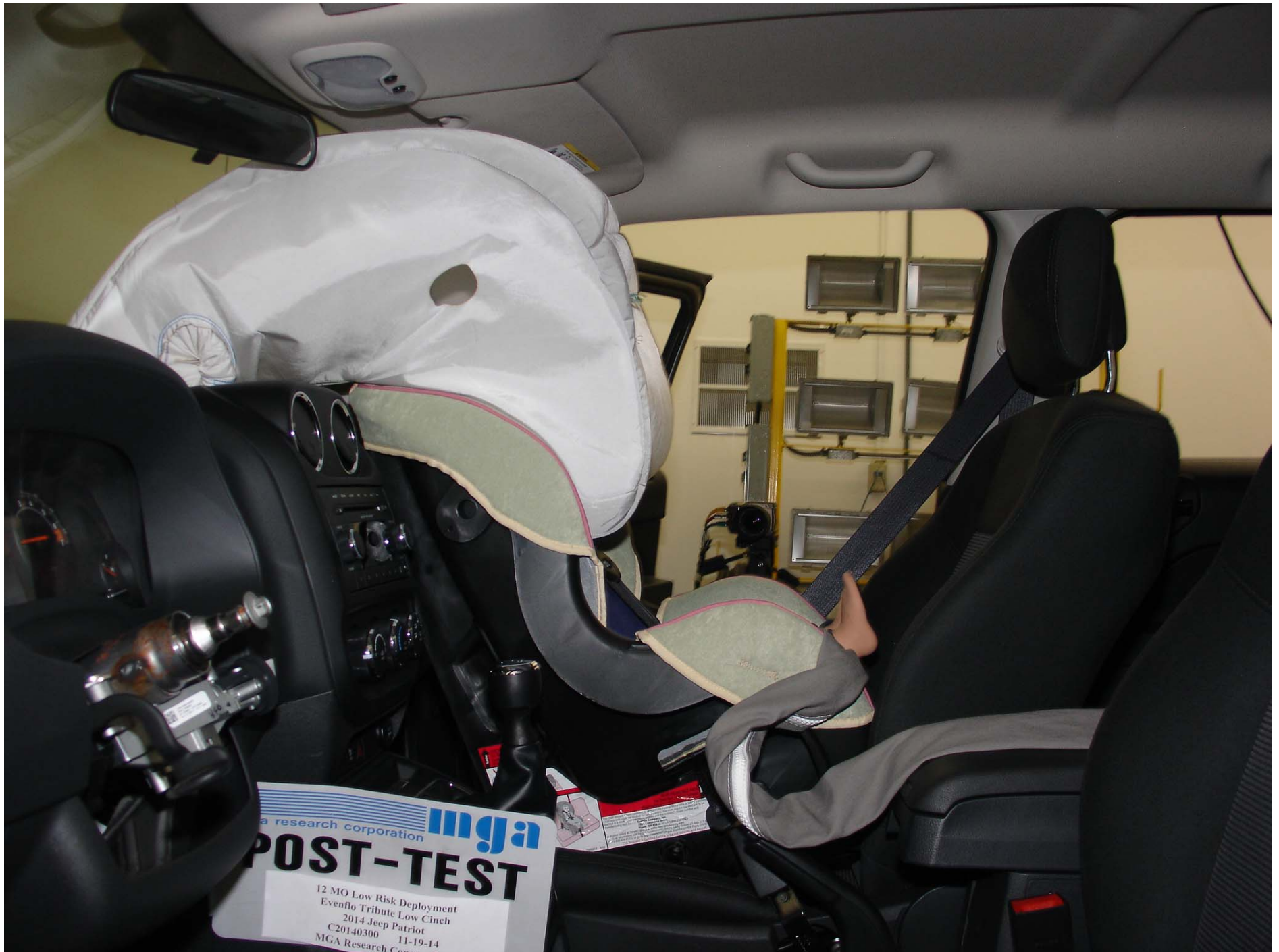
Photo No. 67 - Post-Test 12 Mo Pass. Dummy Left Side View (Evenflo Tribute Low Cinch)
