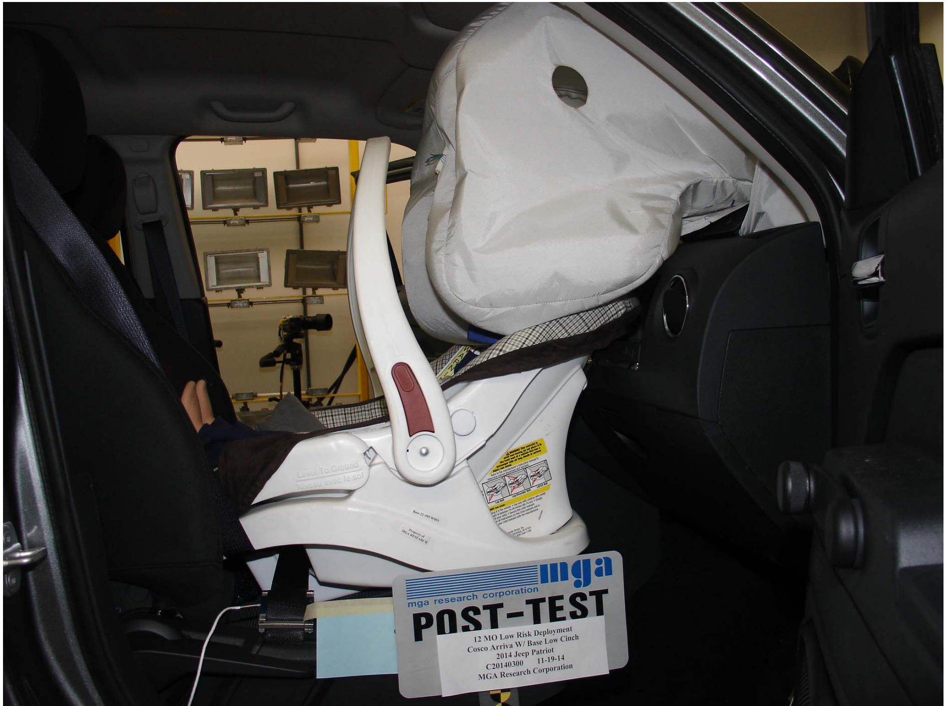
Photo No. 63 - Post-Test 12 Mo Pass. Dummy Right Side View (Cosco Arriva W- Base Low Cinch)
