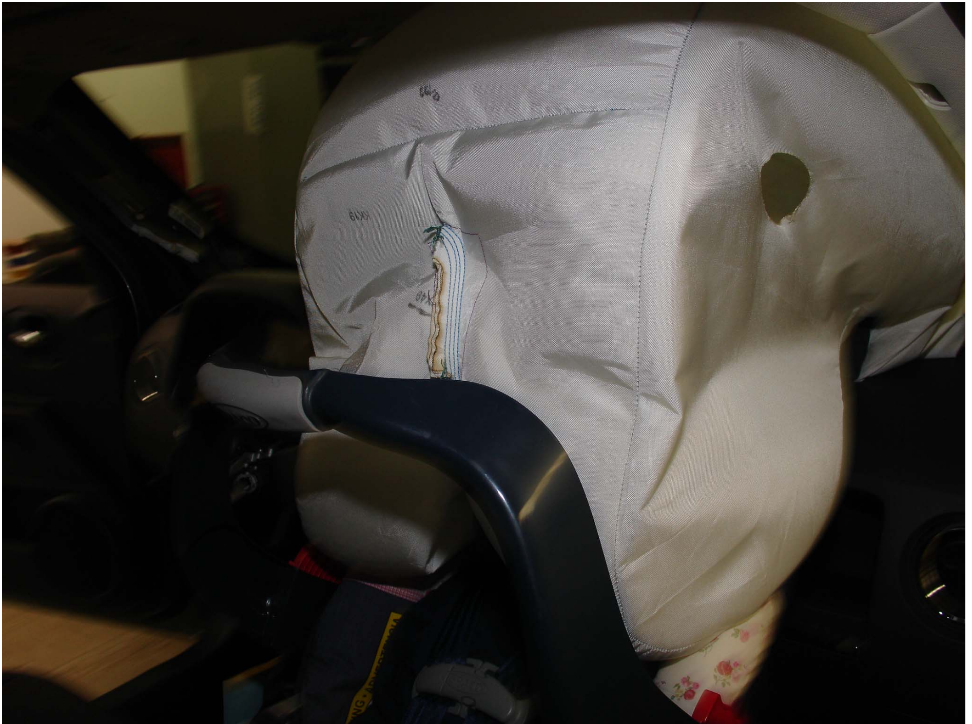
Photo No. 53 - Post-Test 12 Mo Pass. Dummy Airbag Right Side View (Graco Snugride W- Base High Cinch)
