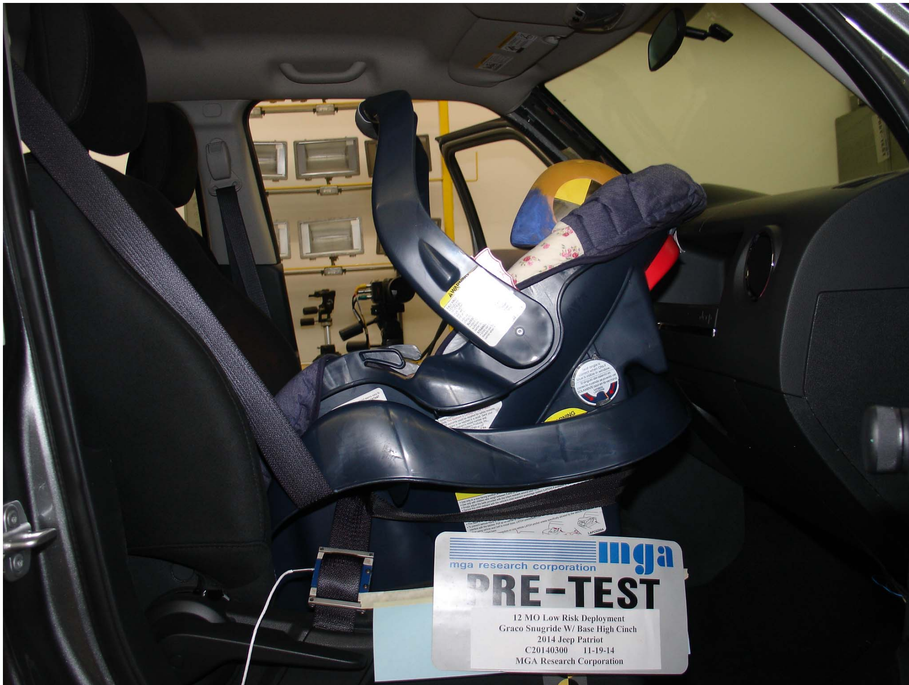
Photo No. 50 - Pre-Test 12 Mo Pass. Dummy Right Side View (Graco Snugride W- Base High Cinch)
