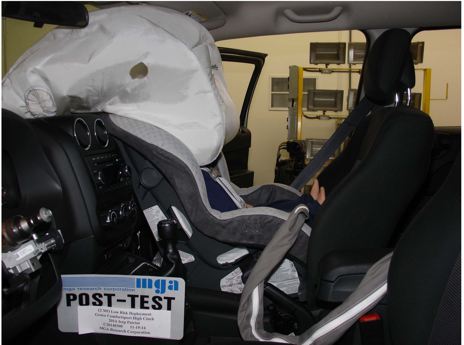
Photo No. 73 - Post-Test 12 Mo Pass. Dummy Left Side View (Graco ComfortSport High Cinch)
