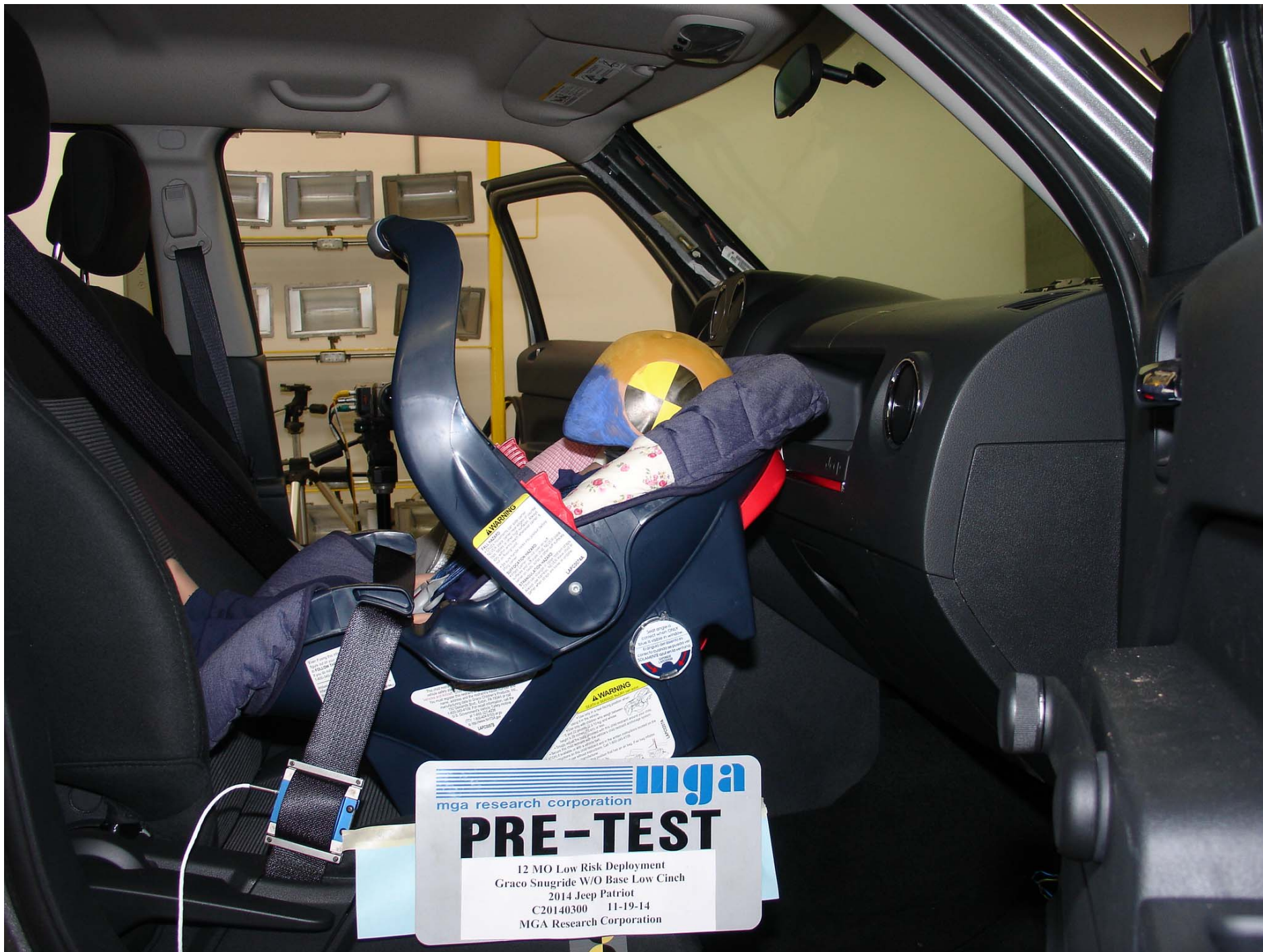
Photo No. 44 - Pre-Test 12 Mo Pass. Dummy Right Side View (Graco Snugride W-O Base Low Cinch)
