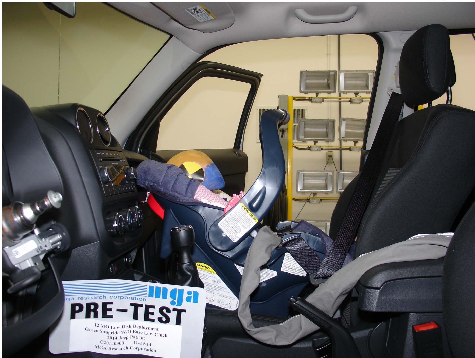
Photo No. 42 - Pre-Test 12 Mo Pass. Dummy Left Side View (Graco Snugride W-O Base Low Cinch)
