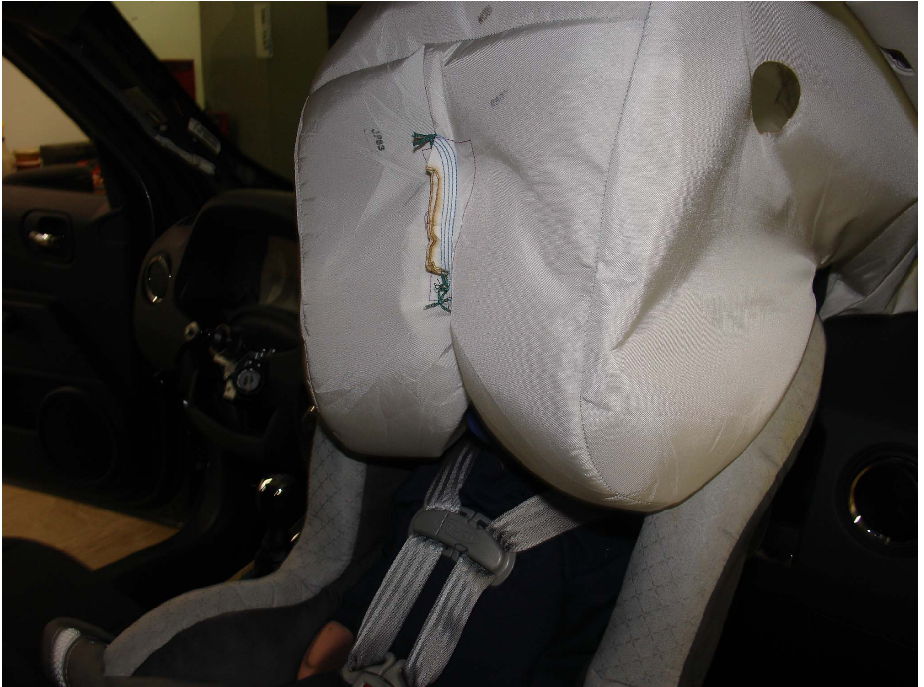
Photo No. 77 - Post-Test 12 Mo Pass. Dummy Airbag Right Side View (Graco ComfortSport High Cinch)
