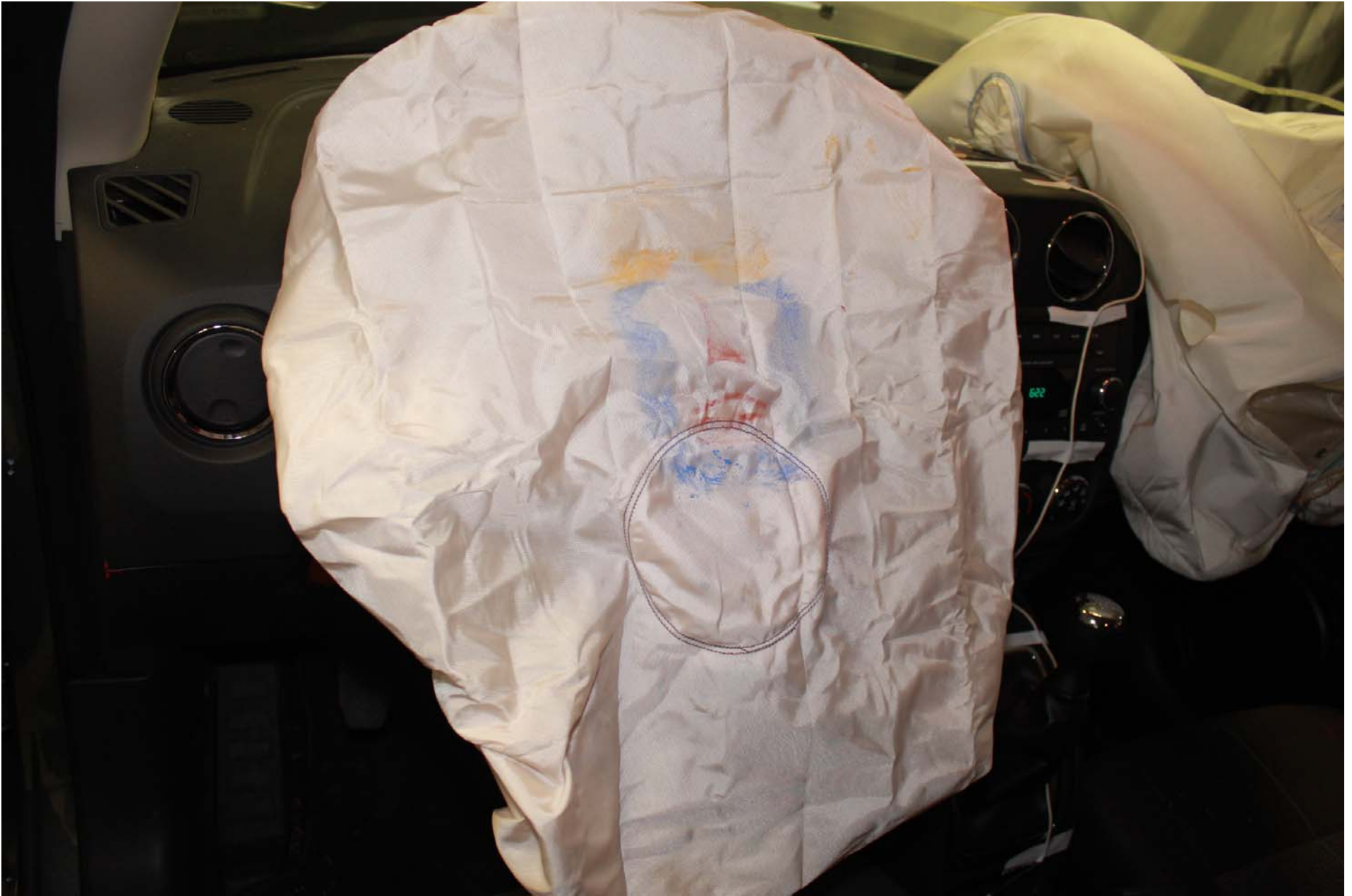
Photo No. 45 - Post-Test Driver Dummy Airbag Contact
