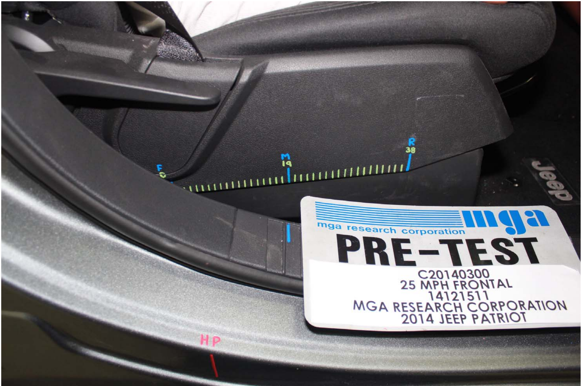
Photo No. 54 - Pre-Test Passenger Dummy Seat Position
