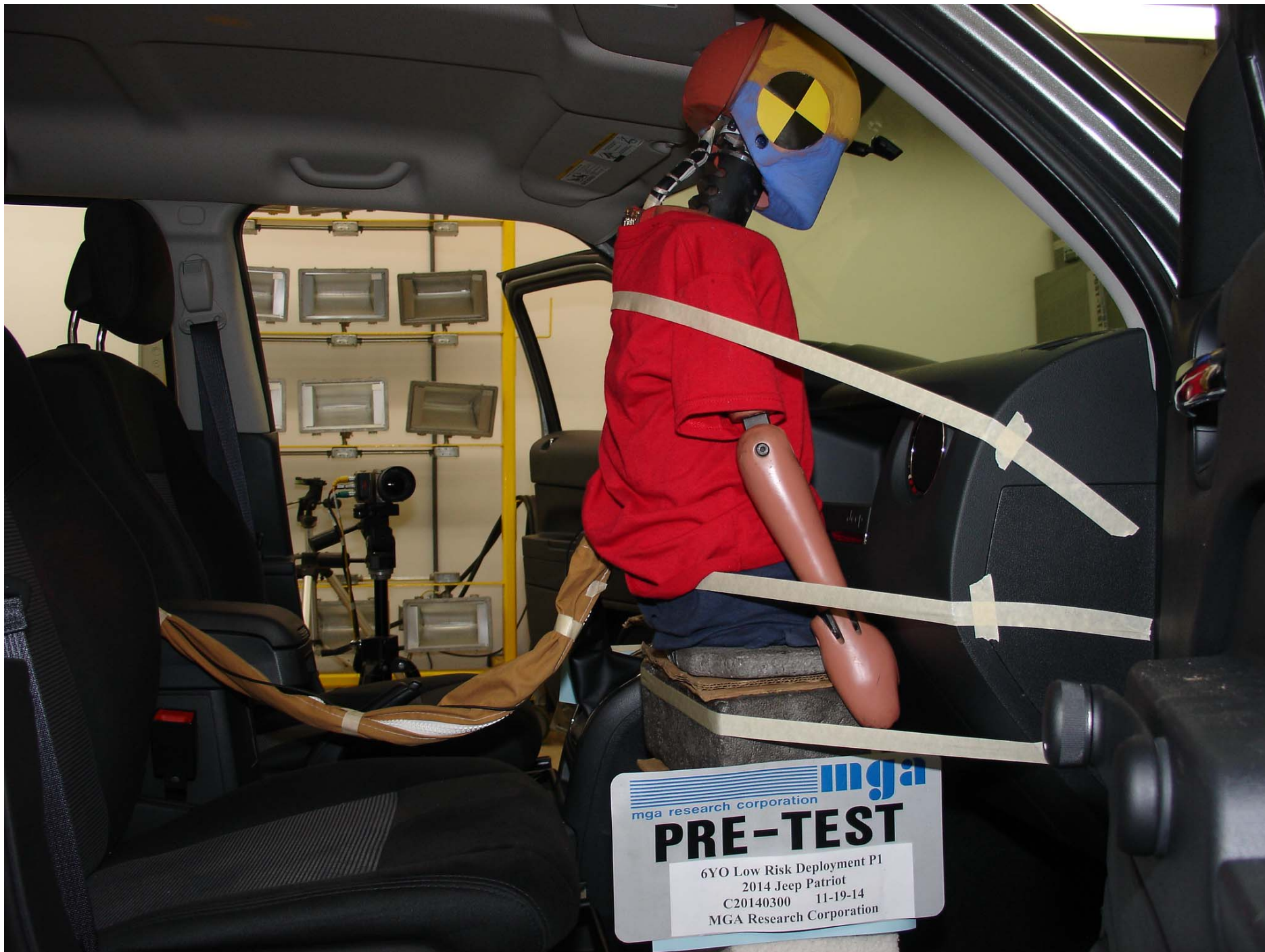
Photo No. 31 - Pre-Test 6YO P1 Passenger Dummy Right Side View
