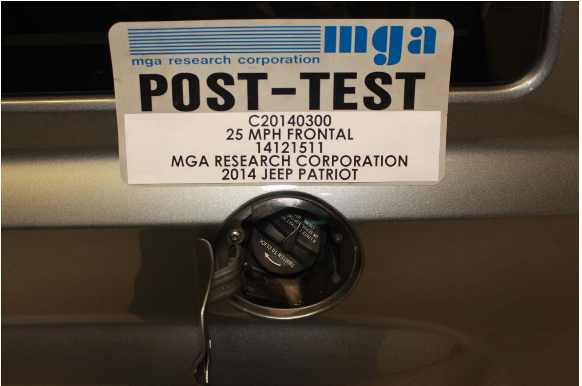
Photo No. 24 - Post-Test Fuel Filler Cap View
