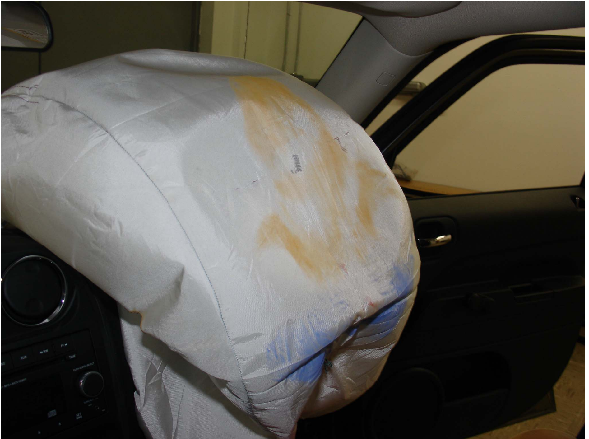
Photo No. 26 - Post-Test 3YO P2 Passenger Dummy Airbag Left Side View
