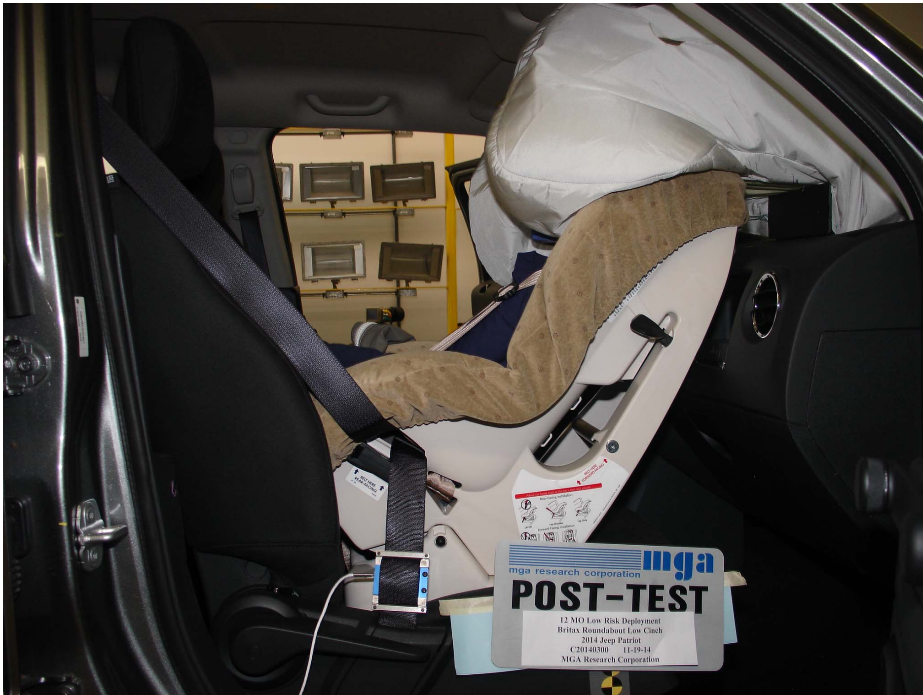
Photo No. 57 - Post-Test 12 Mo Pass. Dummy Right Side View (Britax Roundabout Low Cinch)
