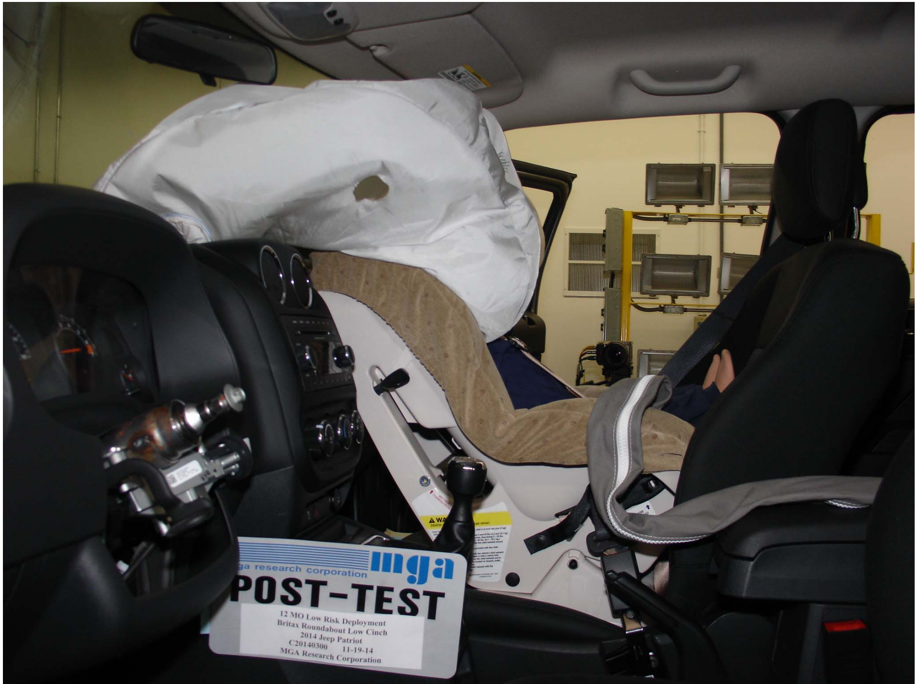
Photo No. 55 - Post-Test 12 Mo Pass. Dummy Left Side View (Britax Roundabout Low Cinch)
