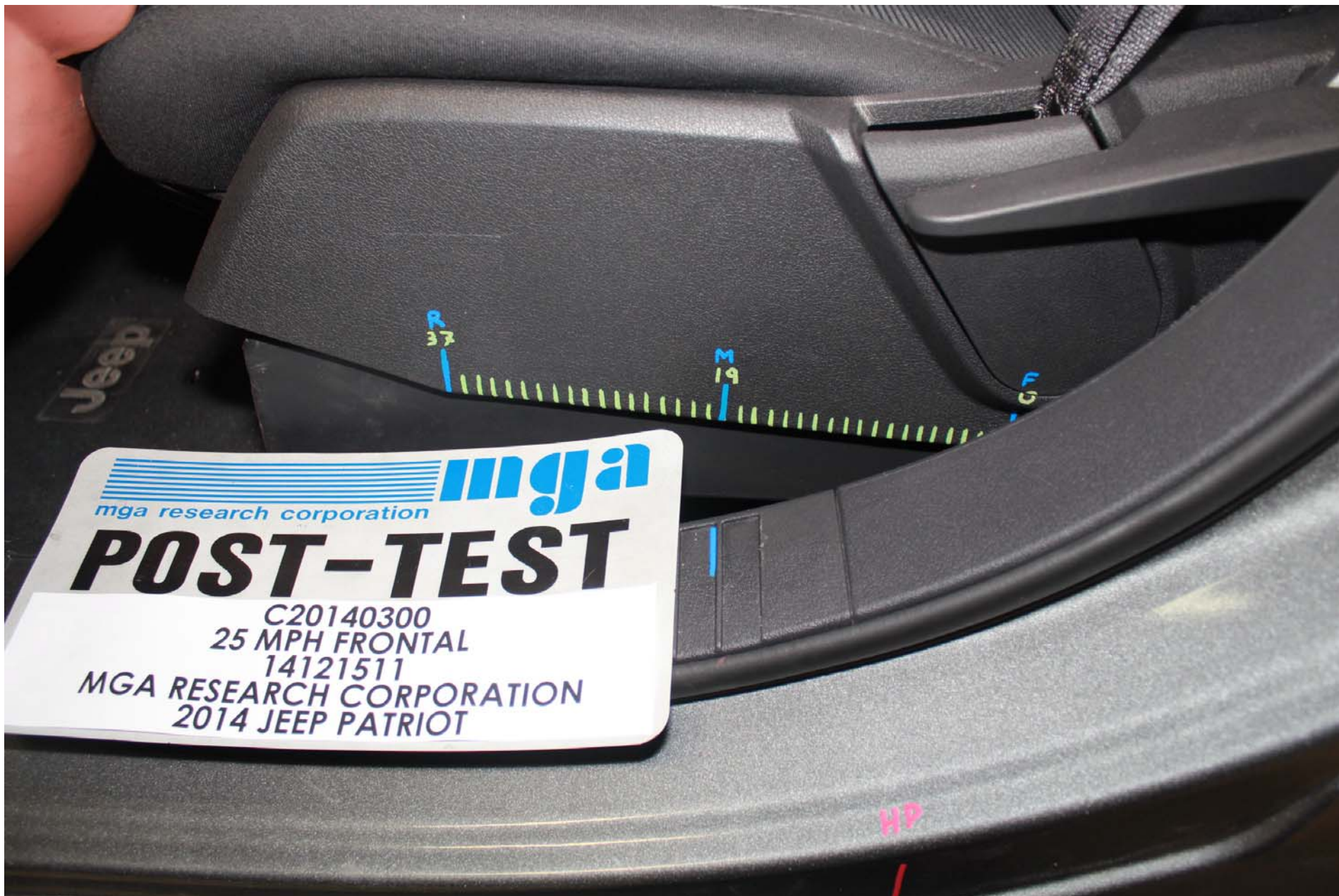
Photo No. 40 - Post-Test Driver Dummy Seat Position
