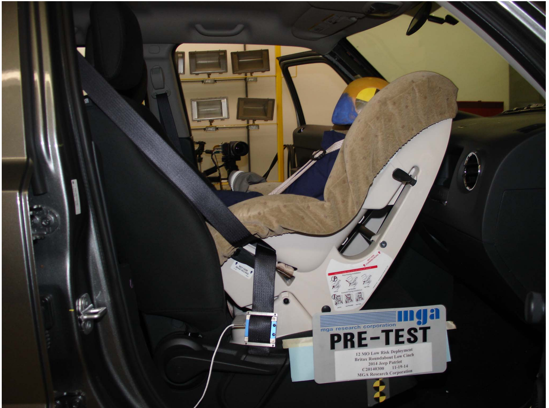
Photo No. 56 - Pre-Test 12 Mo Pass. Dummy Right Side View (Britax Roundabout Low Cinch)
