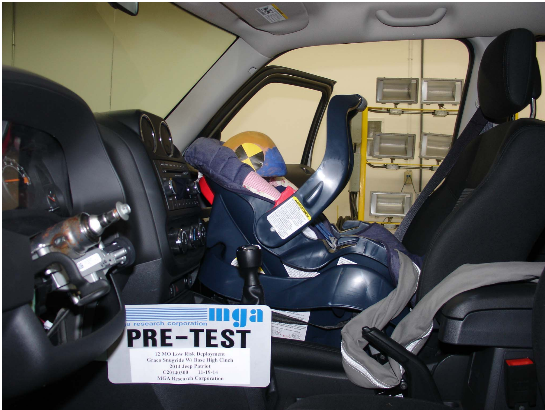
Photo No. 48 - Pre-Test 12 Mo Pass. Dummy Left Side View (Graco Snugride W- Base High Cinch)
