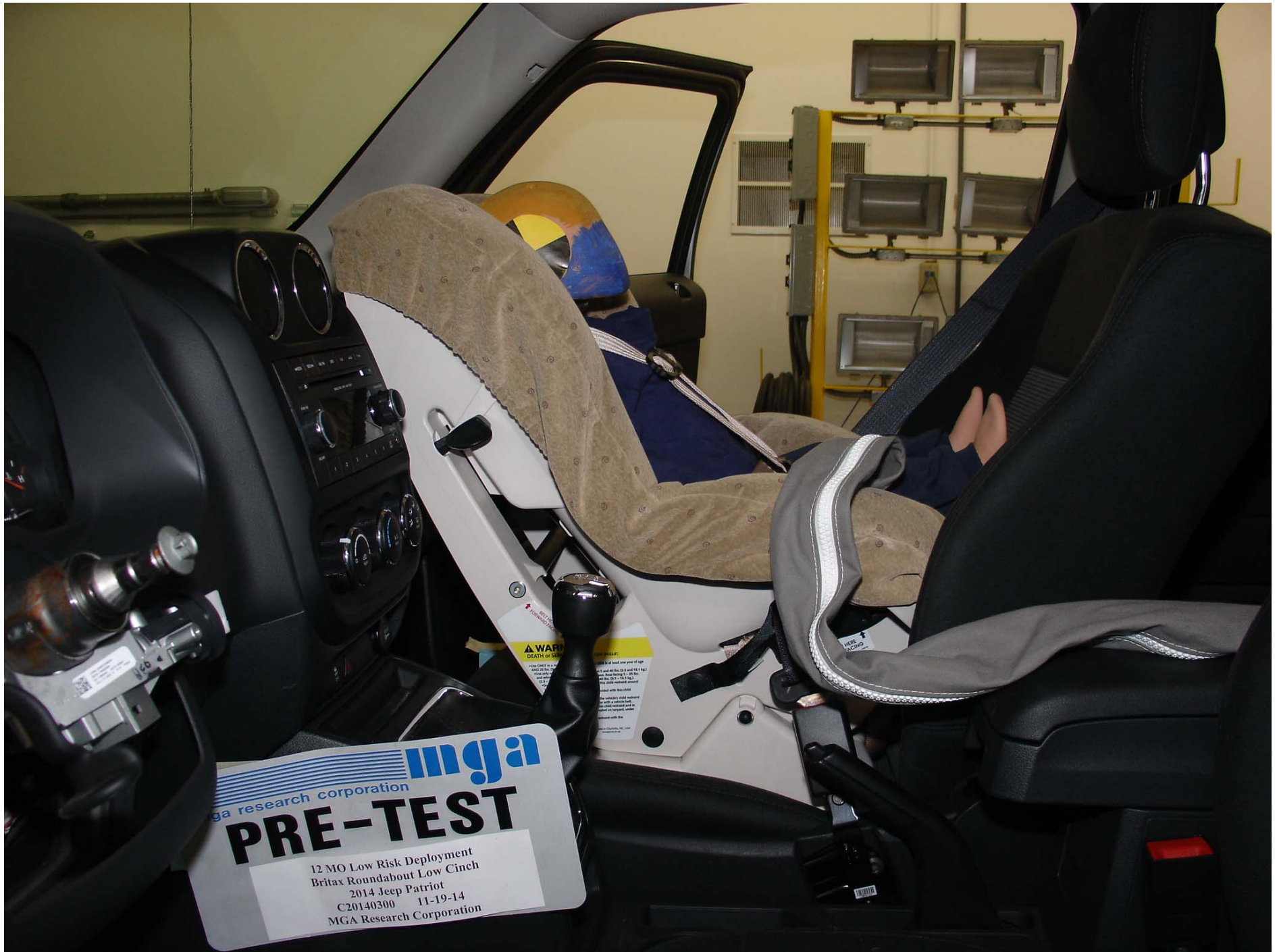
Photo No. 54 - Pre-Test 12 Mo Pass. Dummy Left Side View (Britax Roundabout Low Cinch)
