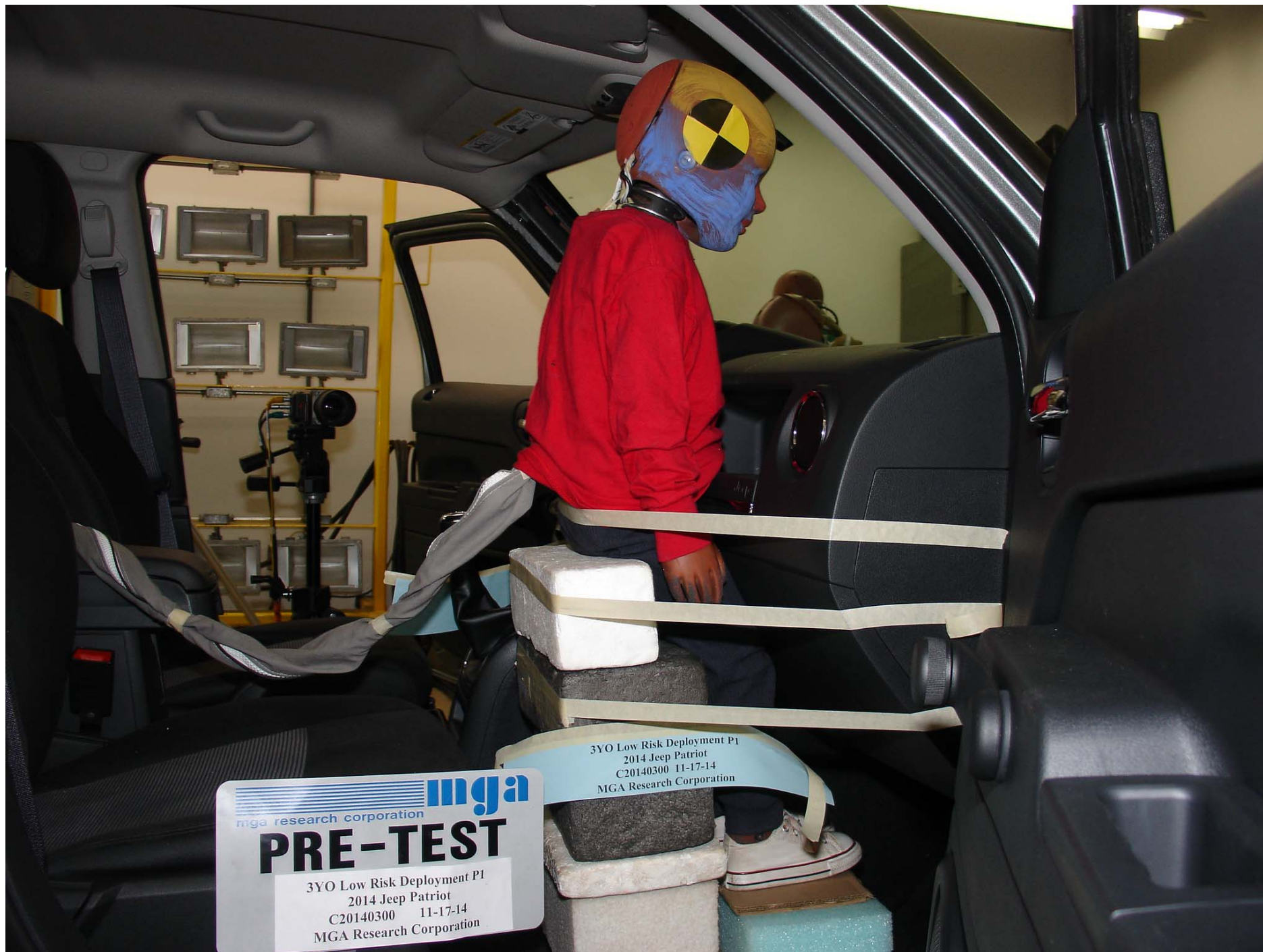
Photo No. 17 - Pre-Test 3YO P1 Passenger Dummy Right Side View
