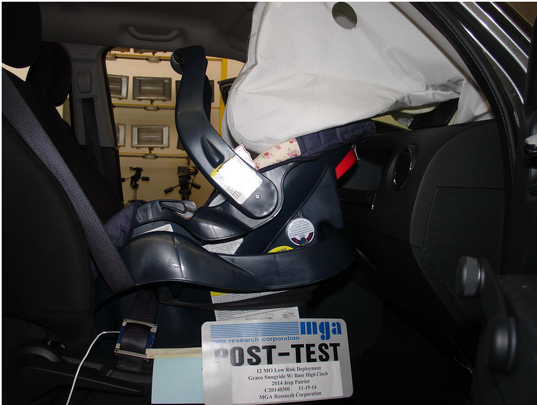
Photo No. 51 - Post-Test 12 Mo Pass. Dummy Right Side View (Graco Snugride W- Base High Cinch)
