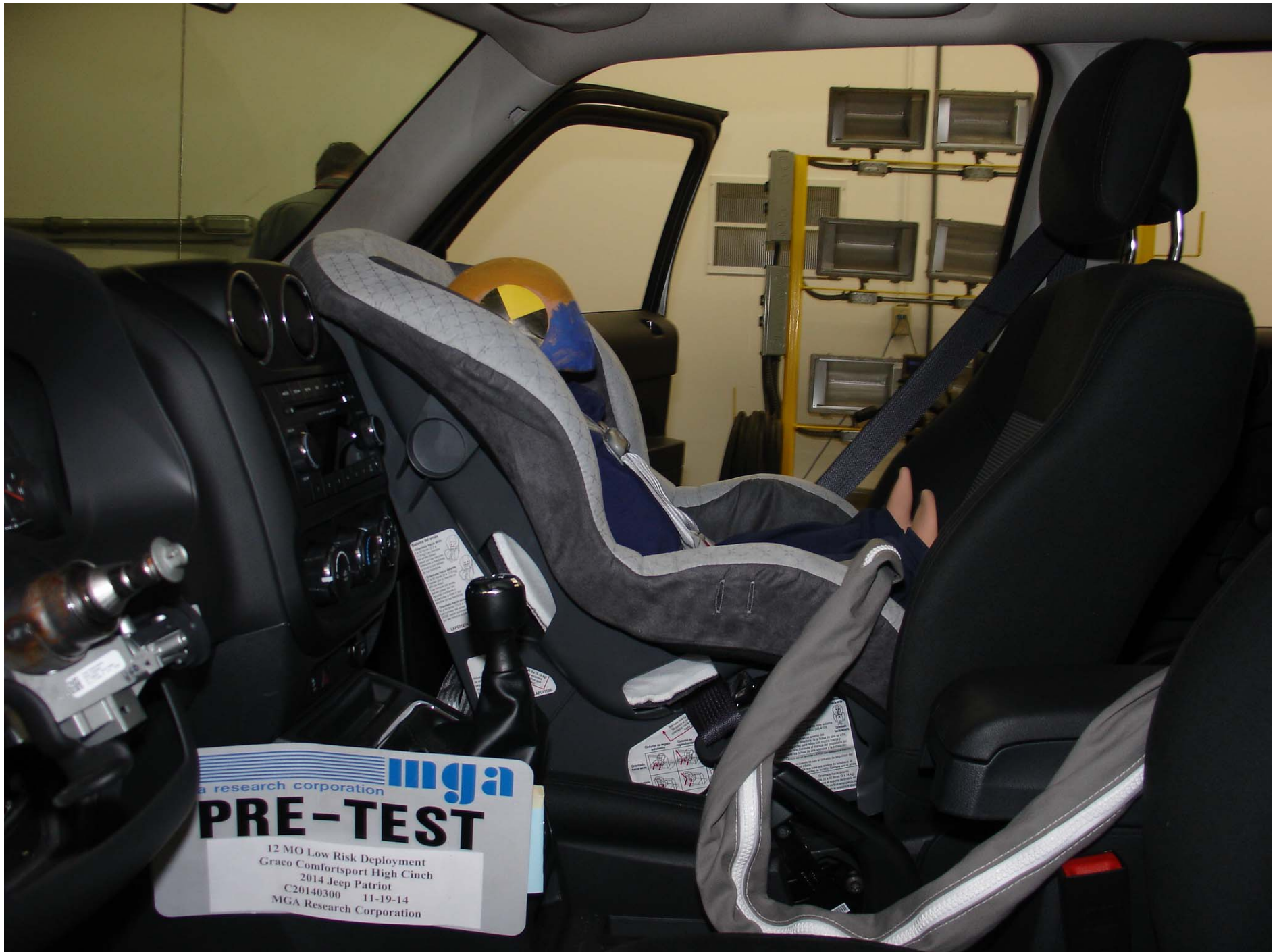
Photo No. 72 - Pre-Test 12 Mo Pass. Dummy Left Side View (Graco ComfortSport High Cinch)
