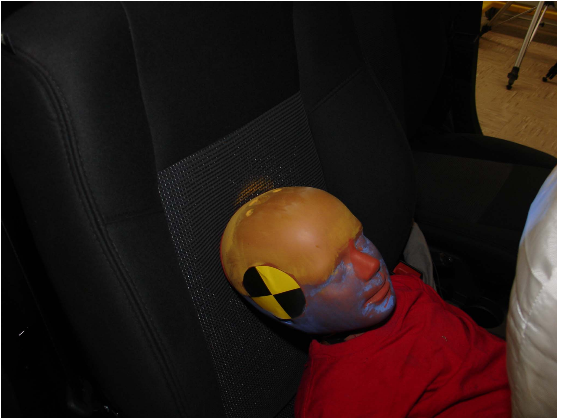
Photo No. 28 - Post-Test 3YO P2 Passenger Dummy Head Contact (seat back)
