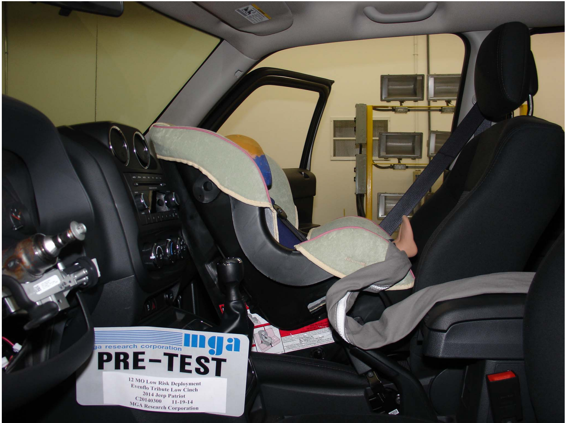
Photo No. 66 - Pre-Test 12 Mo Pass. Dummy Left Side View (Evenflo Tribute Low Cinch)
