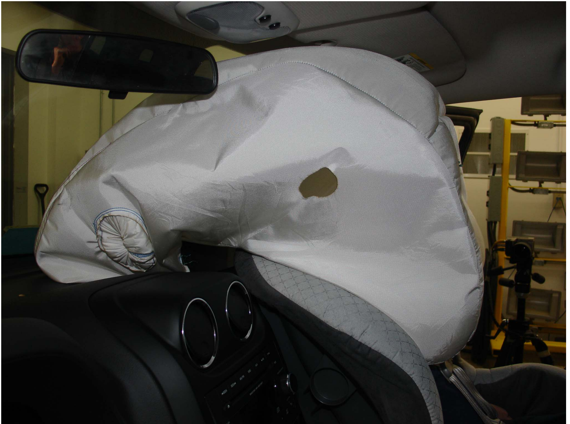
Photo No. 76 - Post-Test 12 Mo Pass. Dummy Airbag Left Side View (Graco ComfortSport High Cinch)
