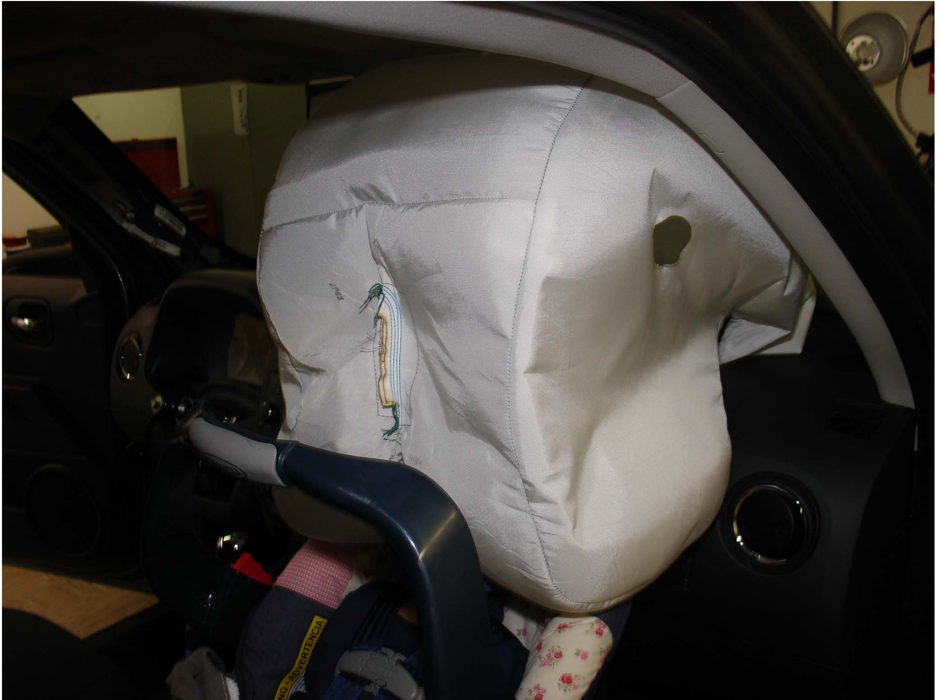
Photo No. 47 - Post-Test 12 Mo Pass. Dummy Airbag Right Side View (Graco Snugride W-O Base Low Cinch)
