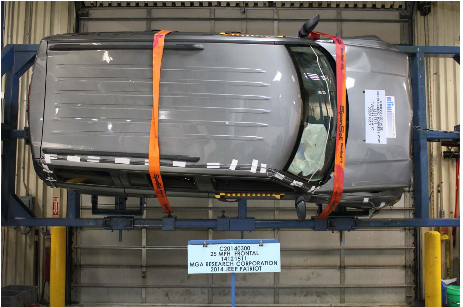
Photo No. 65 - Rollover 270 Degrees
