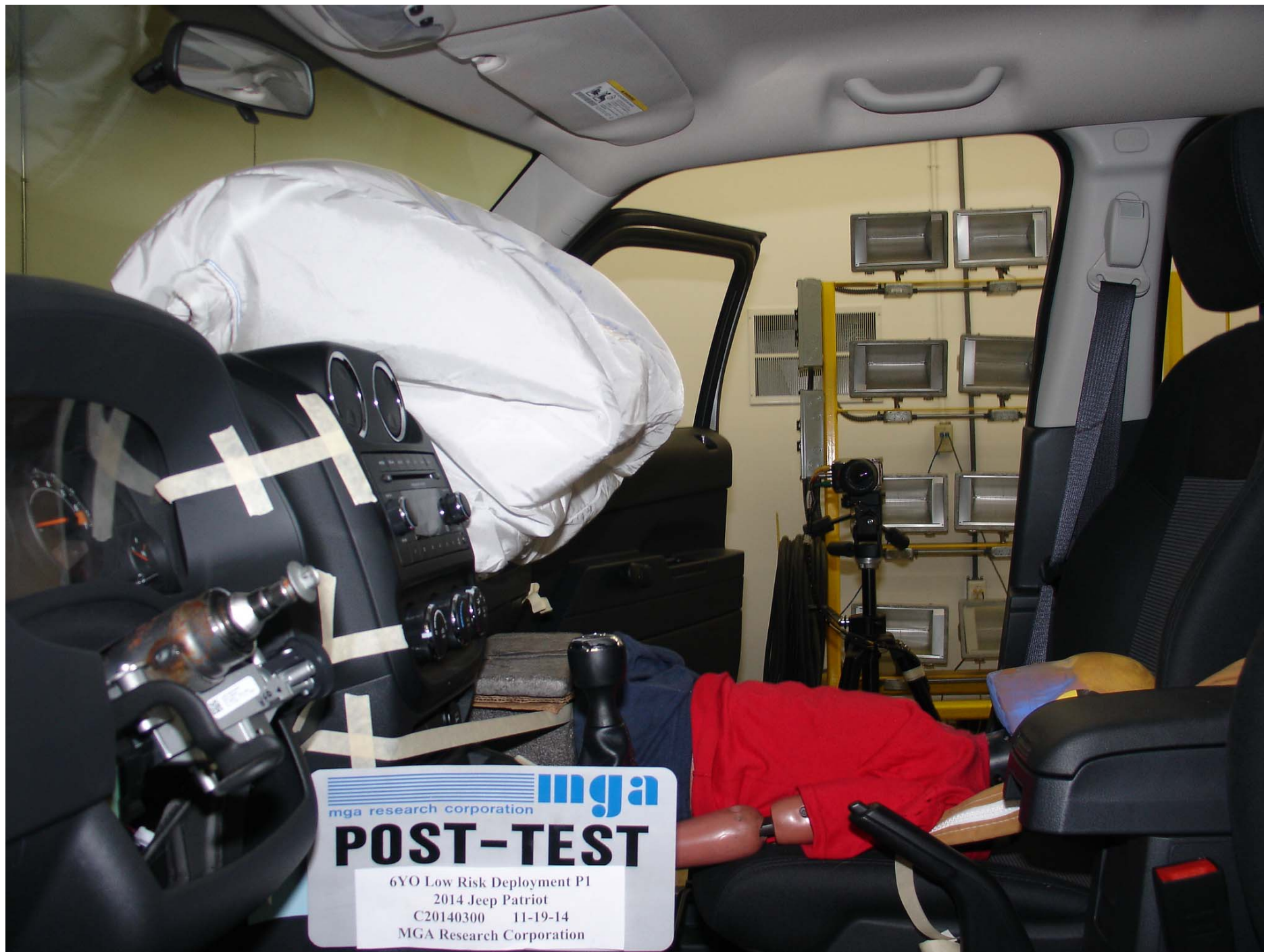
Photo No. 30 - Post-Test 6YO P1 Passenger Dummy Left Side View
