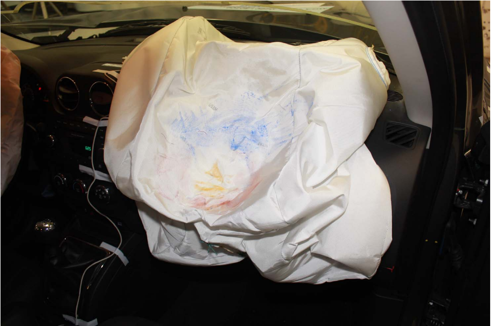
Photo No. 60 - Post-Test Passenger Dummy Airbag Contact
