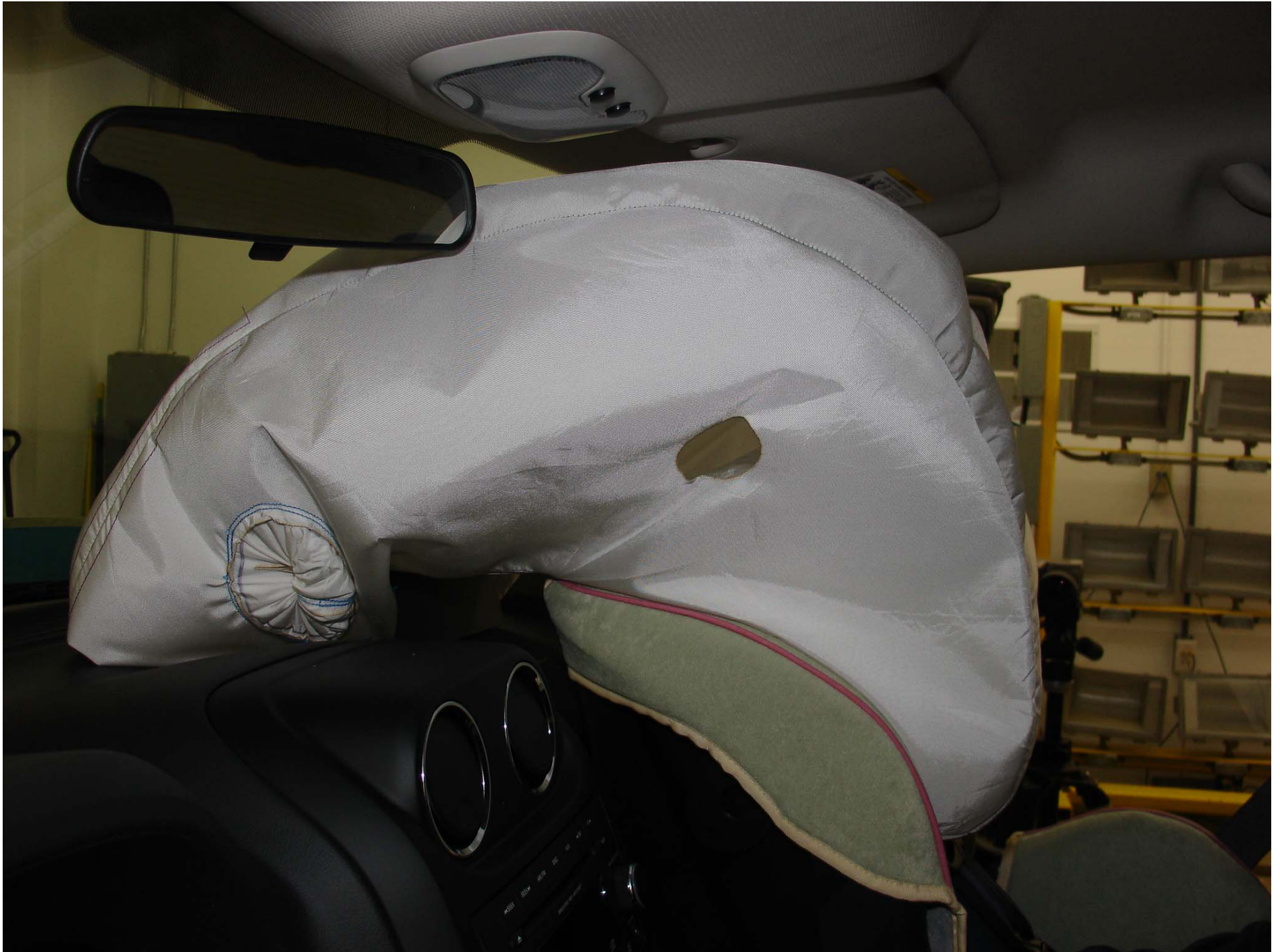
Photo No. 70 - Post-Test 12 Mo Pass. Dummy Airbag Left Side View (Evenflo Tribute Low Cinch)
