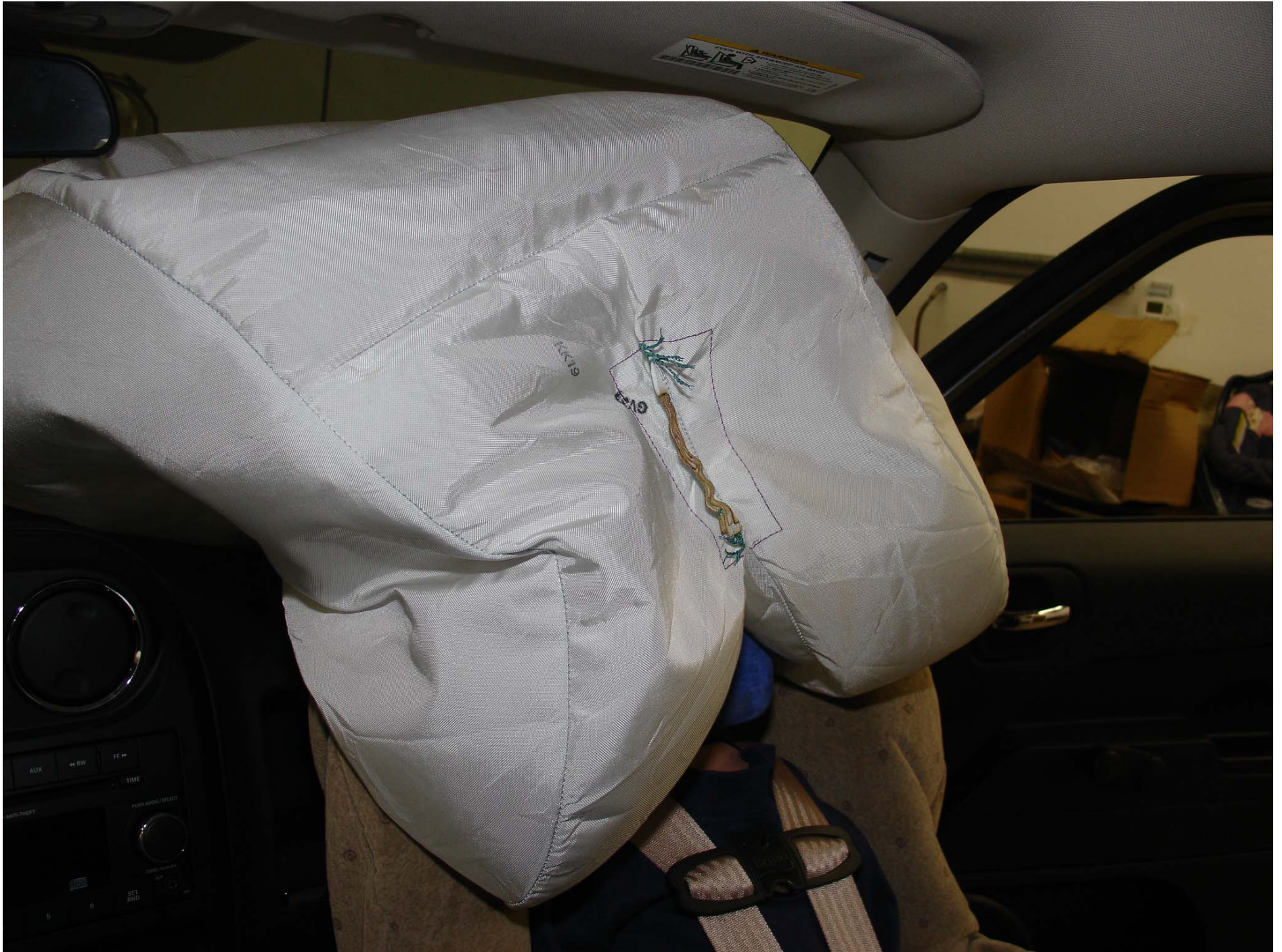
Photo No. 58 - Post-Test 12 Mo Pass. Dummy Airbag Left Side View (Britax Roundabout Low Cinch)
