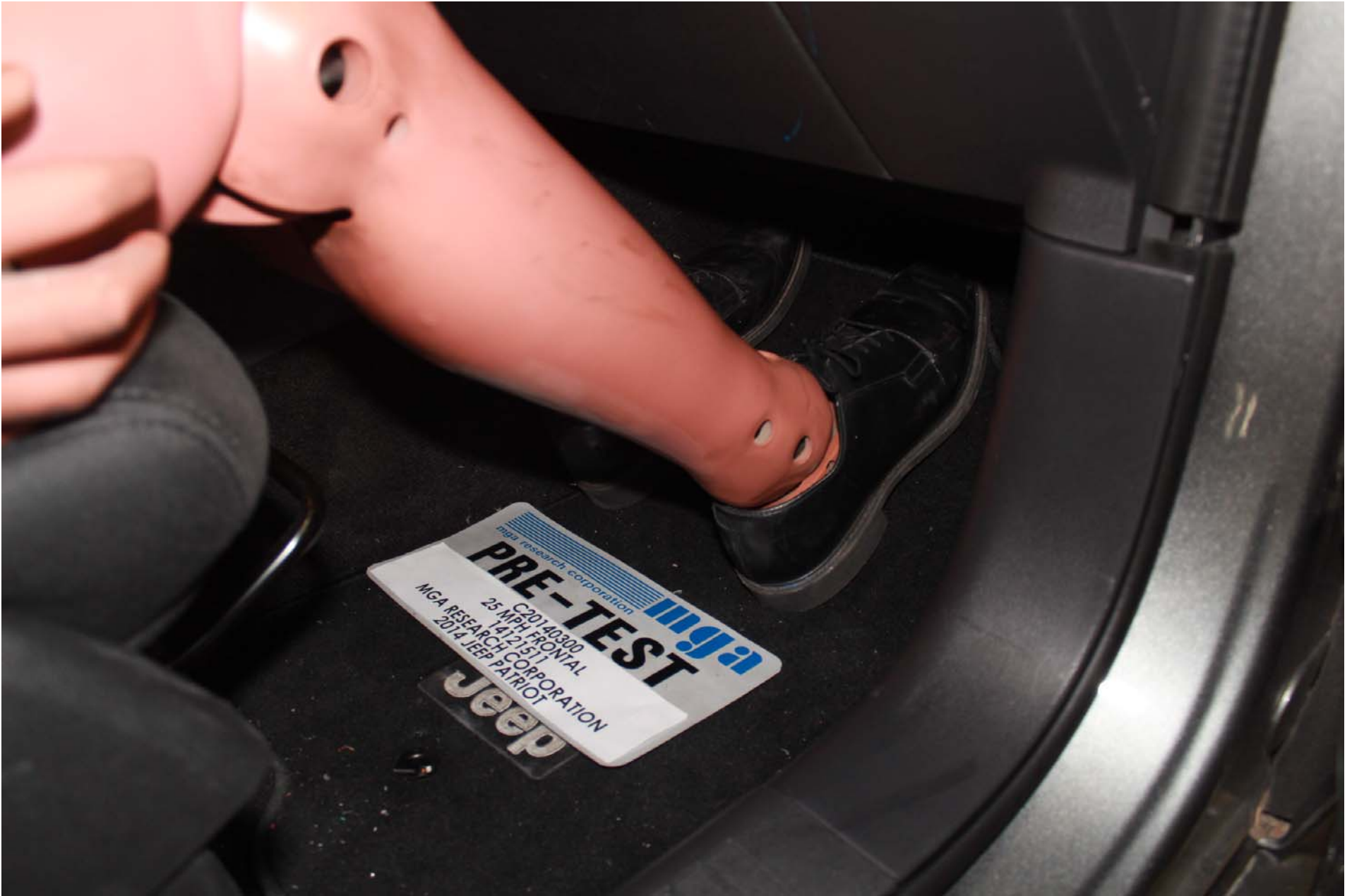
Photo No. 56 - Pre-Test Passenger Dummy Feet Position
