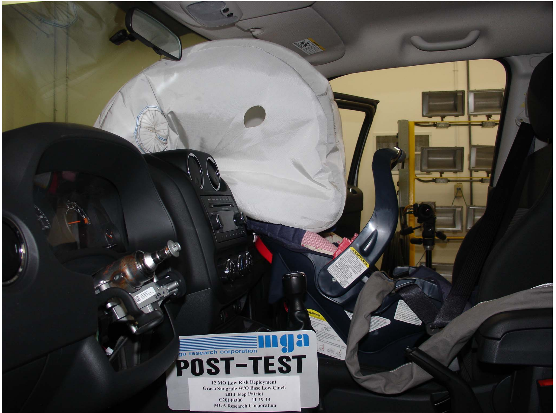
Photo No. 43 - Post-Test 12 Mo Pass. Dummy Left Side View (Graco Snugride W-O Base Low Cinch)
