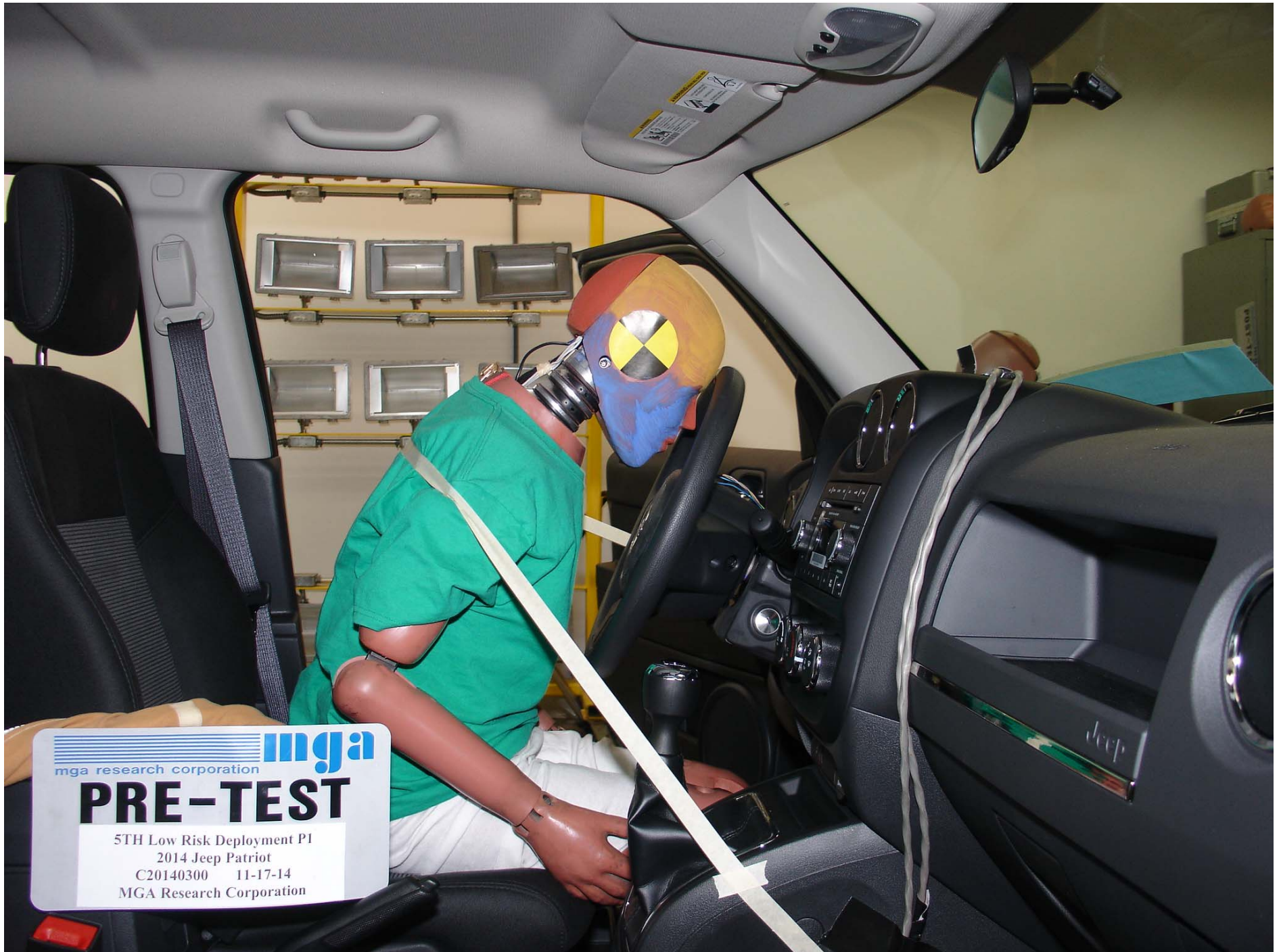
Photo No. 3 - Pre-Test 5th Fem. P1 Driver Dummy Right Side View
