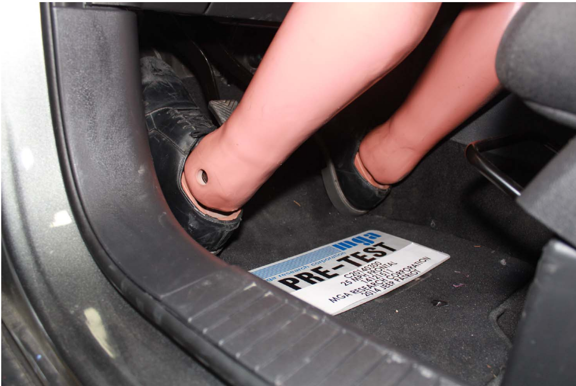
Photo No. 41 - Pre-Test Driver Dummy Feet Position
