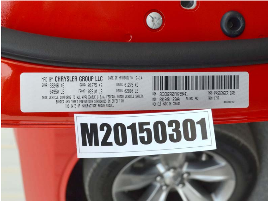
FIGURE 55. Close-Up View of Vehicle's Certification Label
