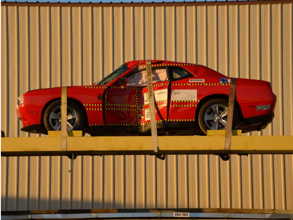
FIGURE 63. FMVSS No. 301 Static Rollover 0 Degrees
