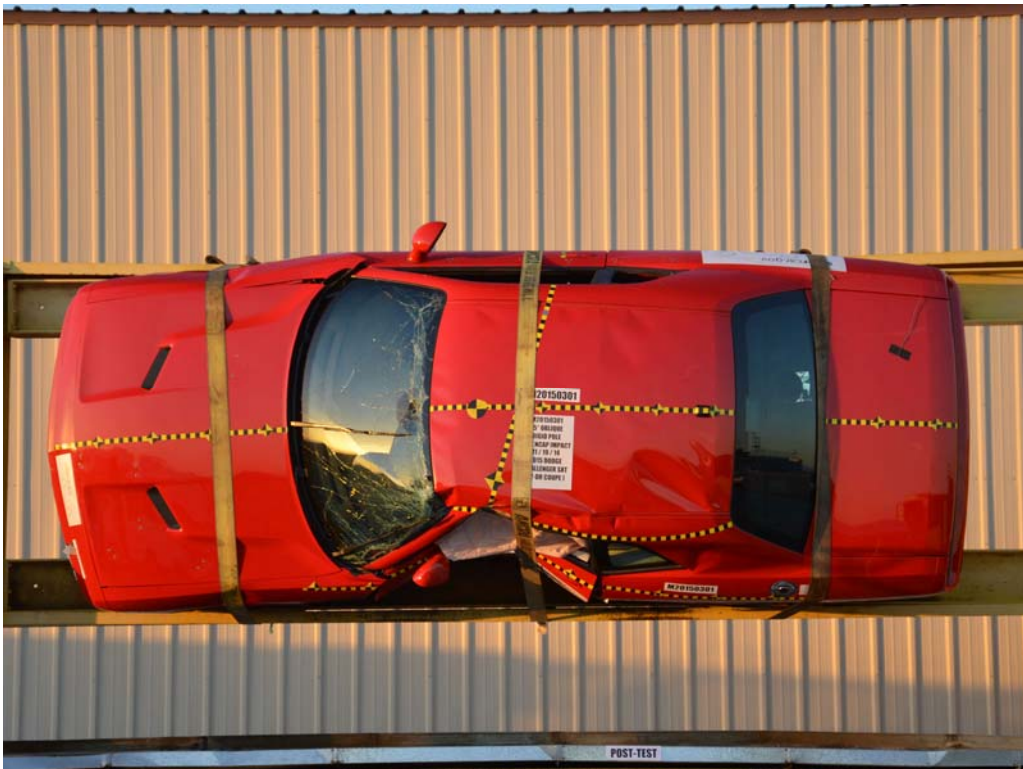
FIGURE 64. FMVSS No. 301 Static Rollover 90 Degrees
