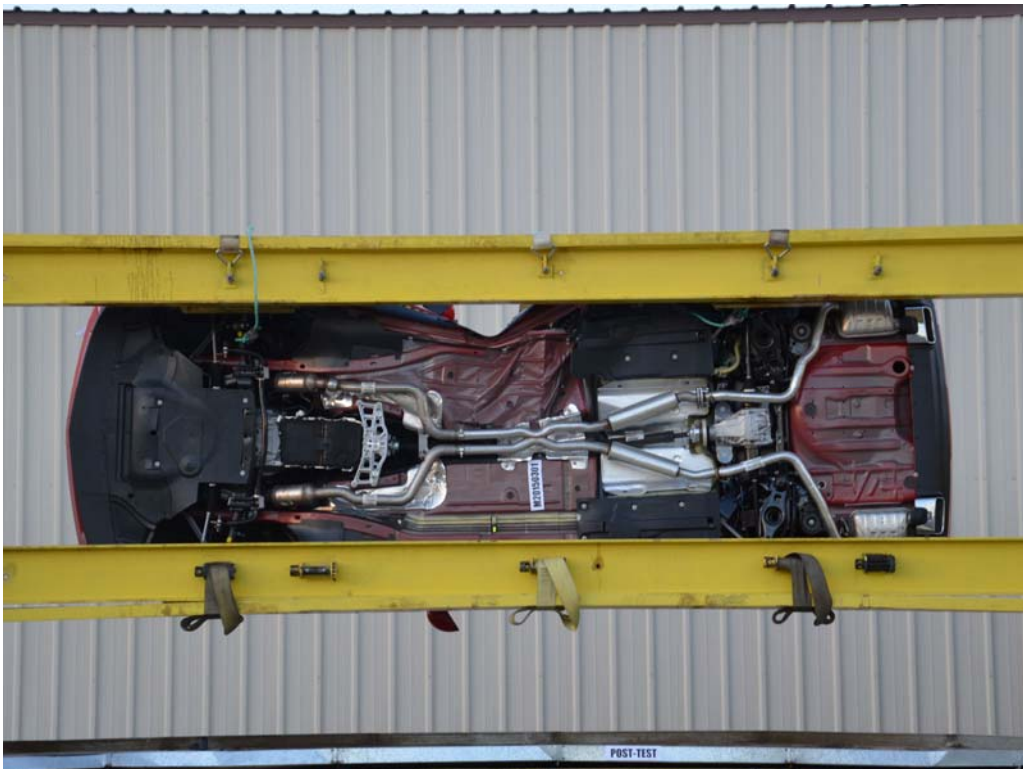
FIGURE 66. FMVSS No. 301 Static Rollover 270 Degrees
