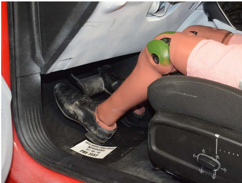
FIGURE 32. Pre-Test Placement of Dummy's Feet
