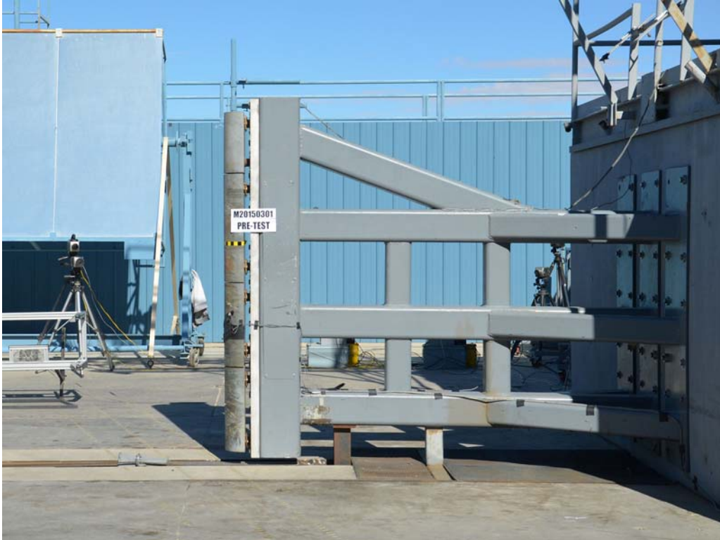
FIGURE 59. Pre-Test Pole Barrier Side View
