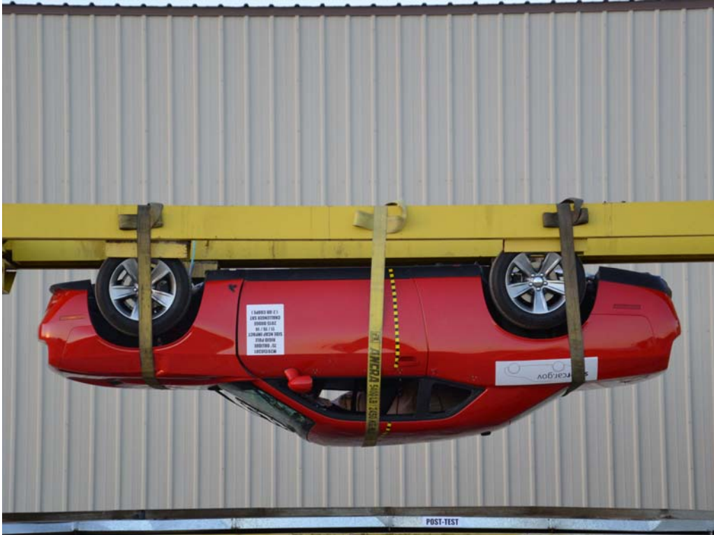
FIGURE 65. FMVSS No. 301 Static Rollover 180 Degrees
