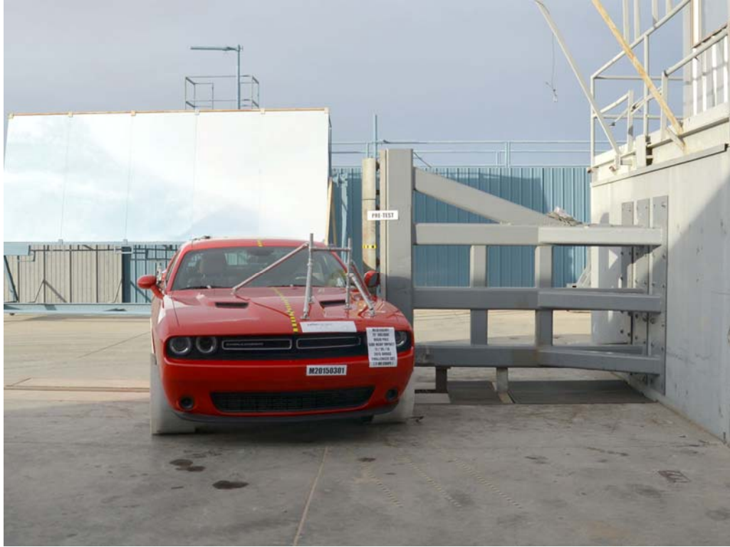
FIGURE 17. Pre-Test Left Side View of Pole Positioned Against Side of Vehicle
