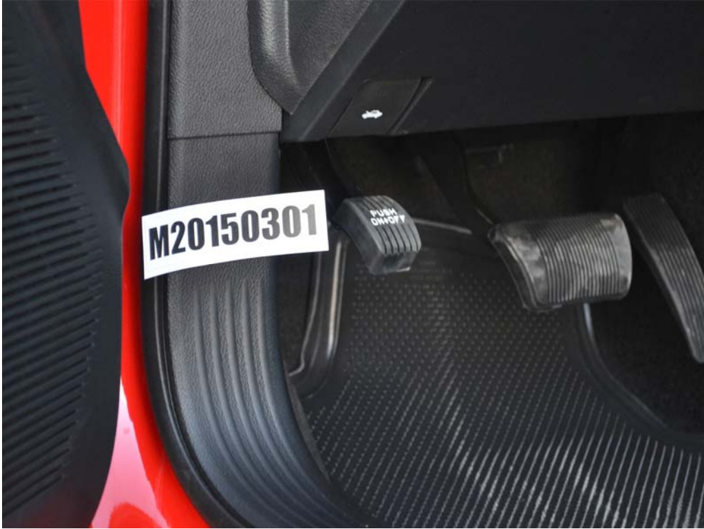
FIGURE 35. View of Disengaged Parking Brake
