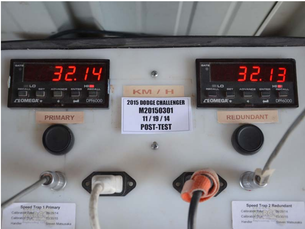
FIGURE 62. Post-Test Primary and Redundant Speed Trap Read-Out
