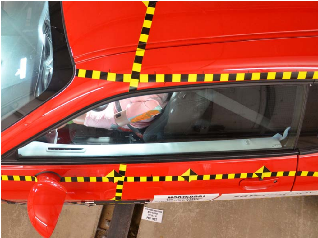
FIGURE 40. Pre-Test Dummy and Door Clearance View
