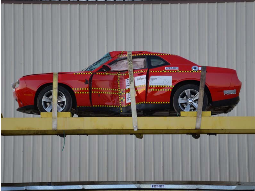
FIGURE 67. FMVSS No. 301 Static Rollover 360 Degrees
