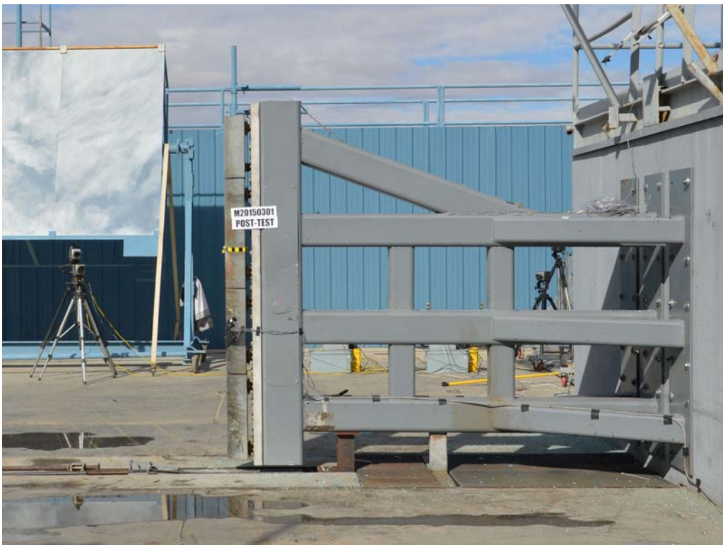
FIGURE 60. Post-Test Pole Barrier Side View
