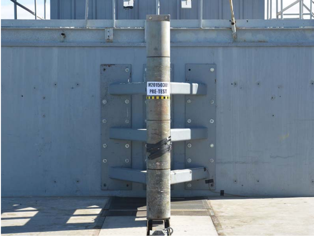
FIGURE 57. Pre-Test Pole Barrier Front View
