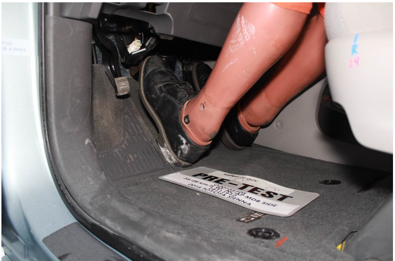
Pre-Test Placement of Driver Dummy's Feet
