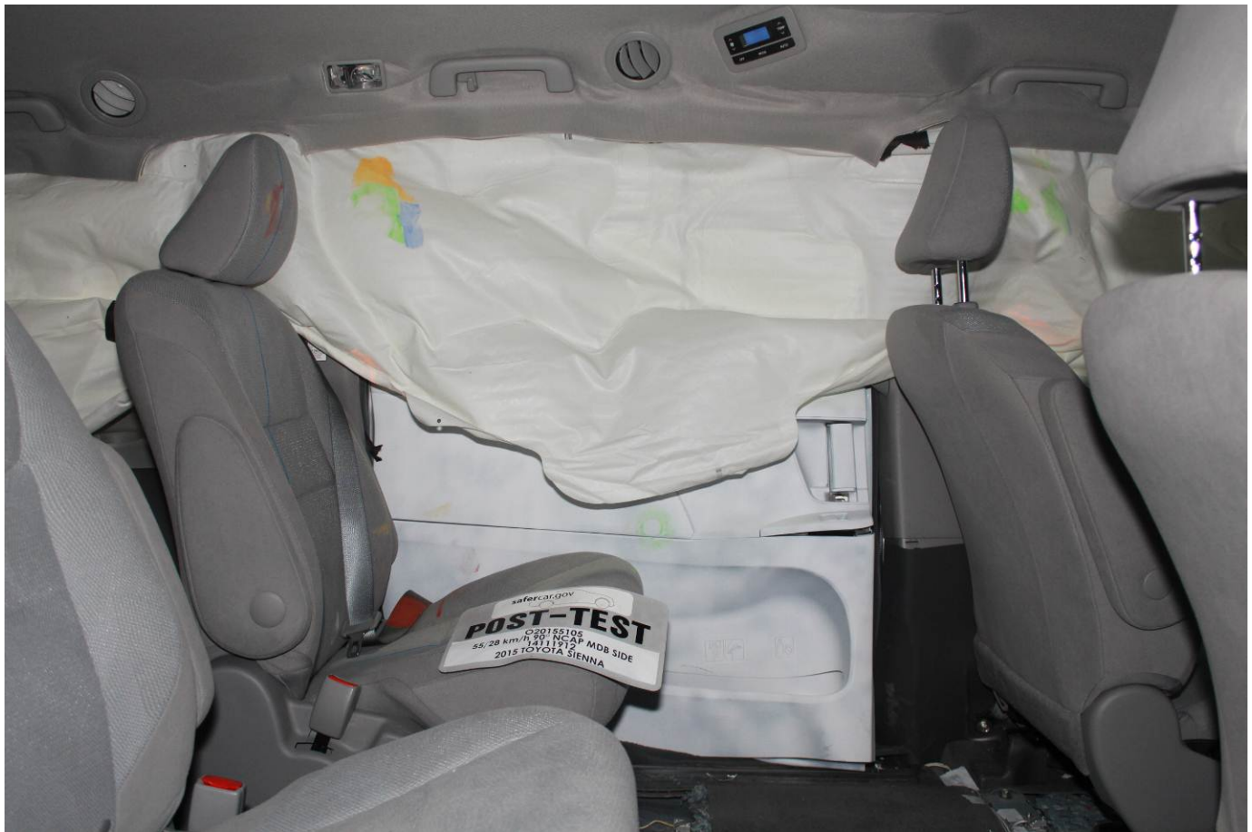
Post-Test Rear Passenger Inner Door Panel View
