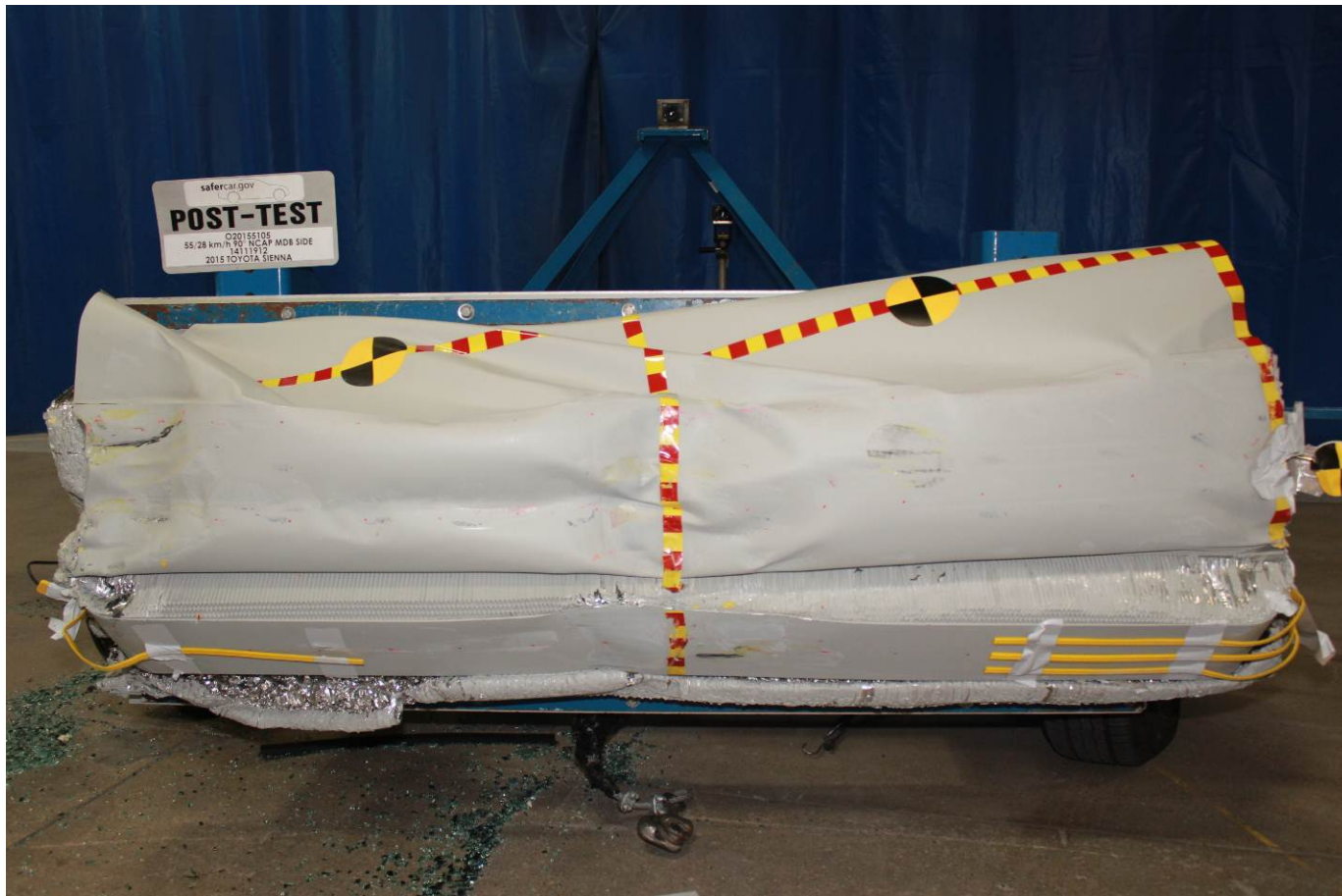
Post-Test Front View of MDB Impactor Face
