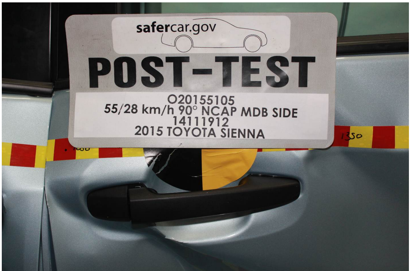
Post-Test Left Rear Door Latch Close-Up
