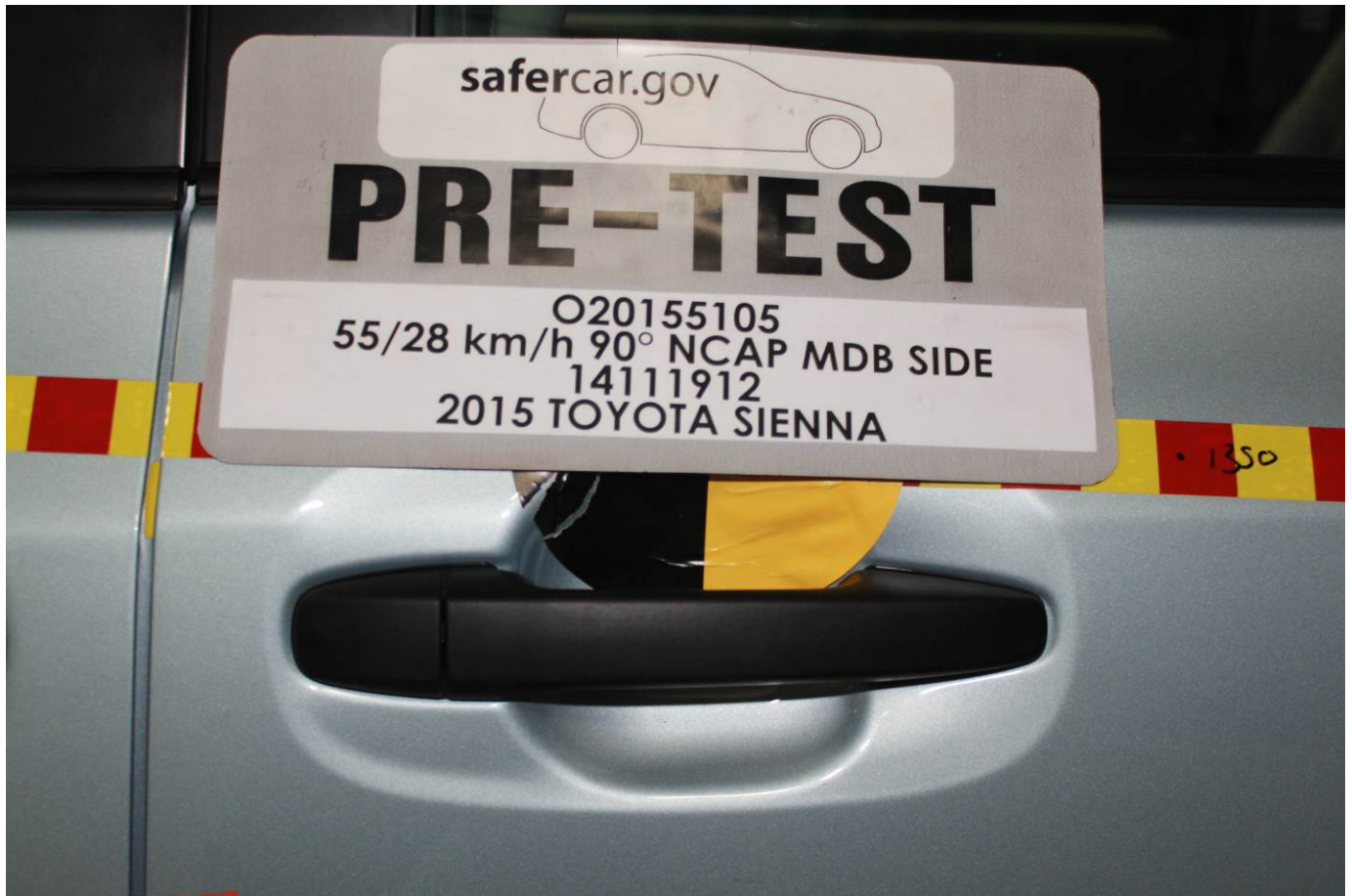
Pre-Test Left Rear Door Latch Close-Up
