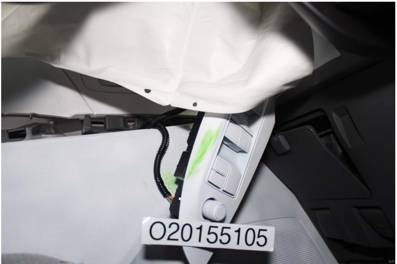
Post-Test Driver Dummy Close-up Knee Contact View
