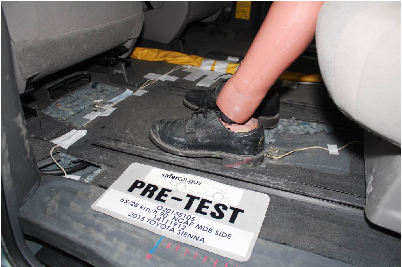
Pre-Test Placement of Rear Passenger Dummy's Feet
