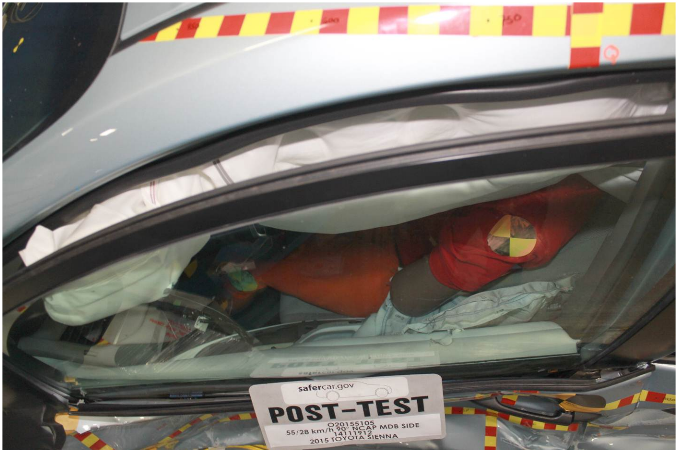
Post-Test Driver Dummy and Door Clearance View
