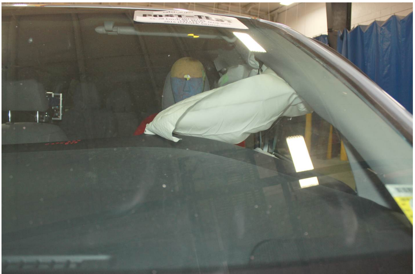
Post-Test Front Close-Up View of Driver Dummy
