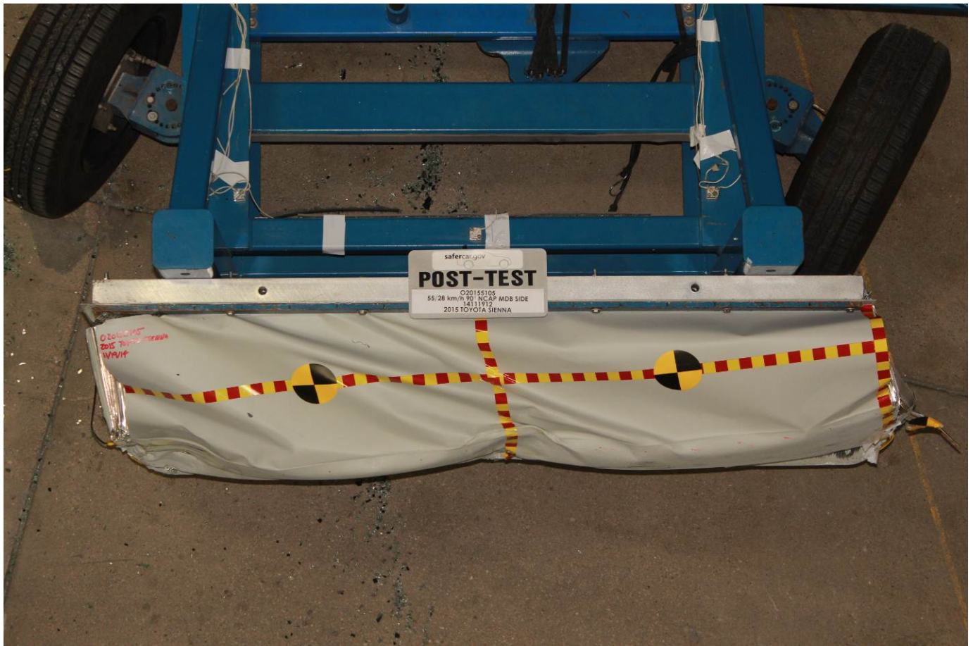
Post-Test Top View of MDB Impactor Face
