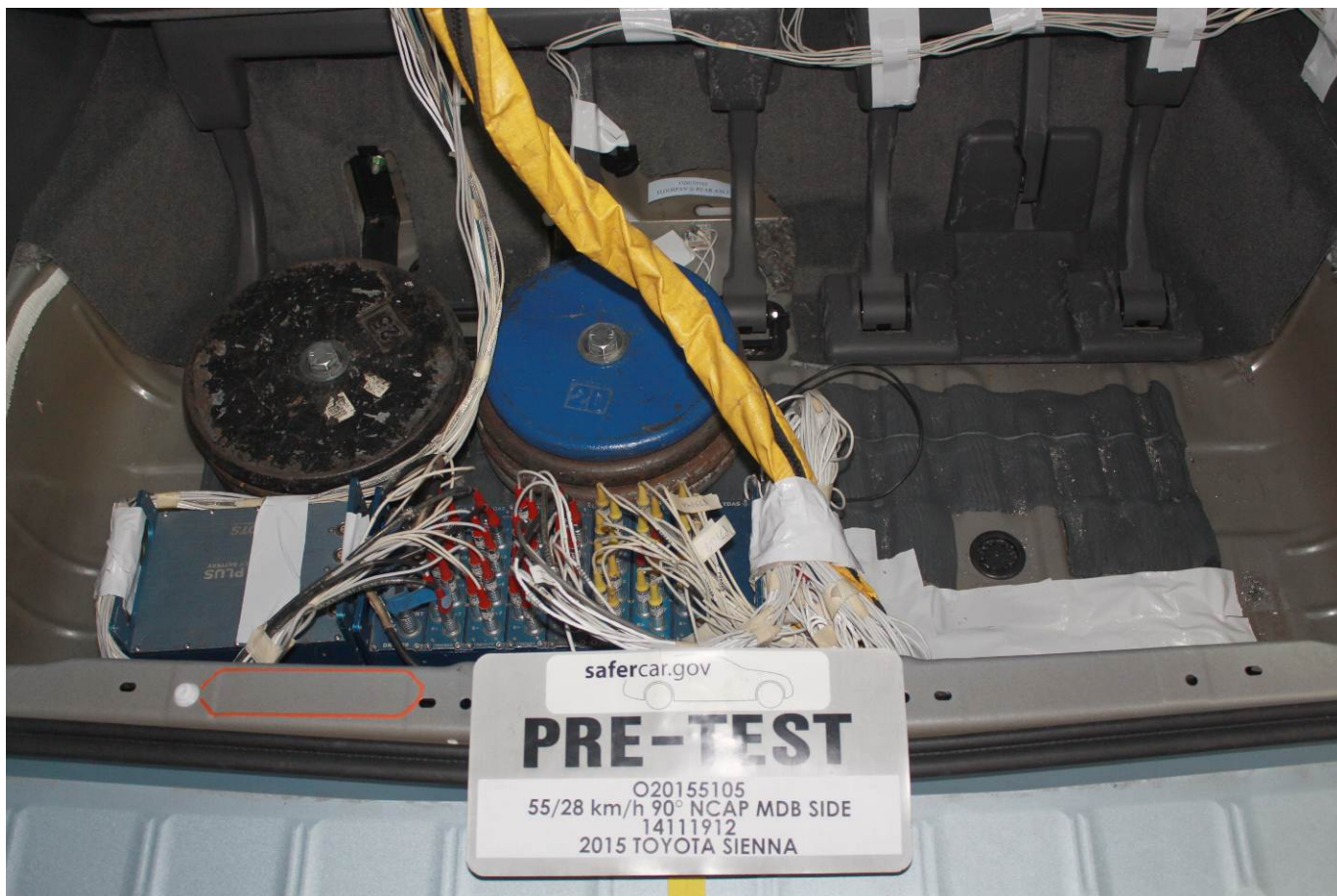
Pre-Test Ballast View
