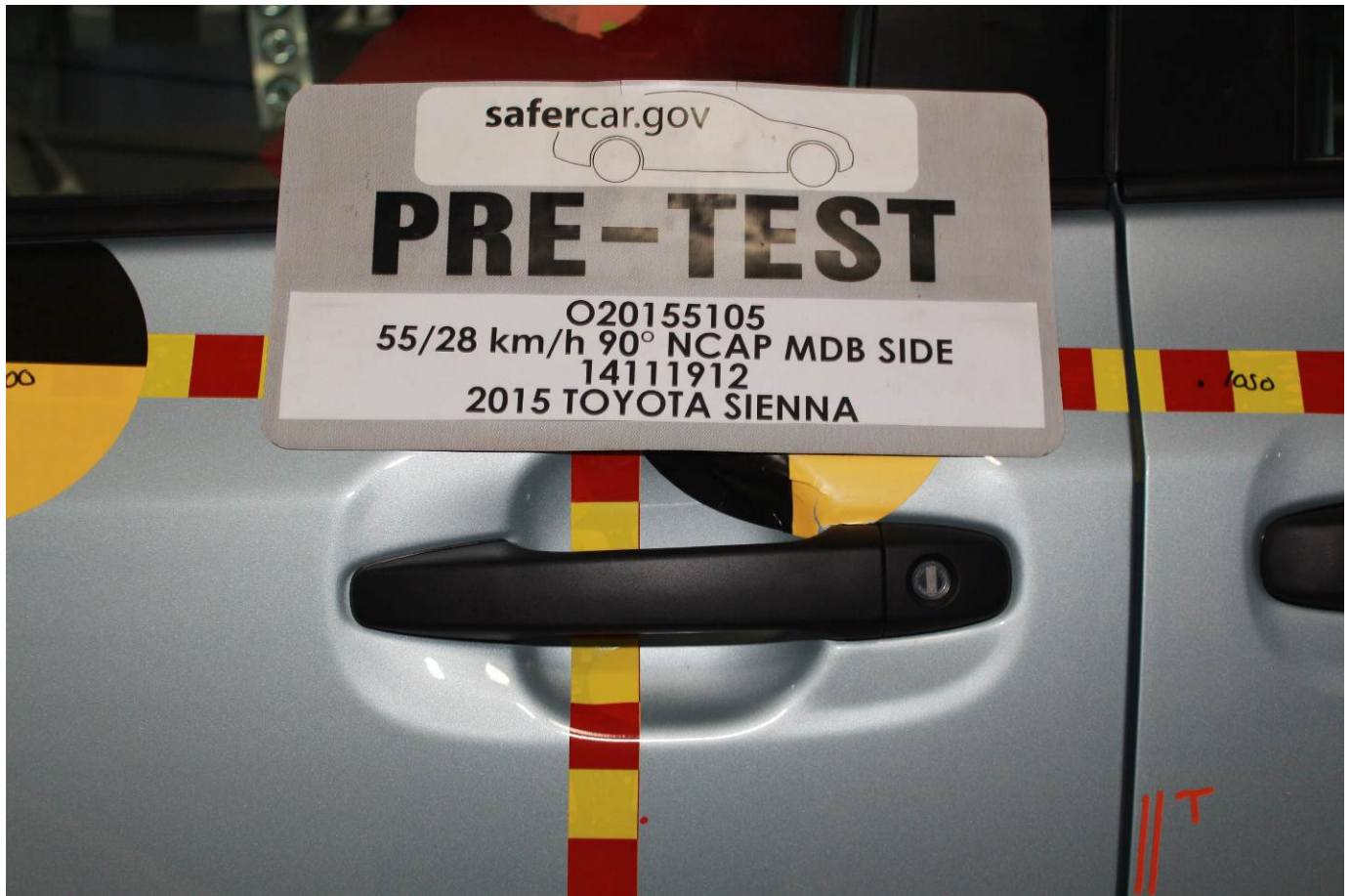
Pre-Test Left Front Door Latch Close-Up
