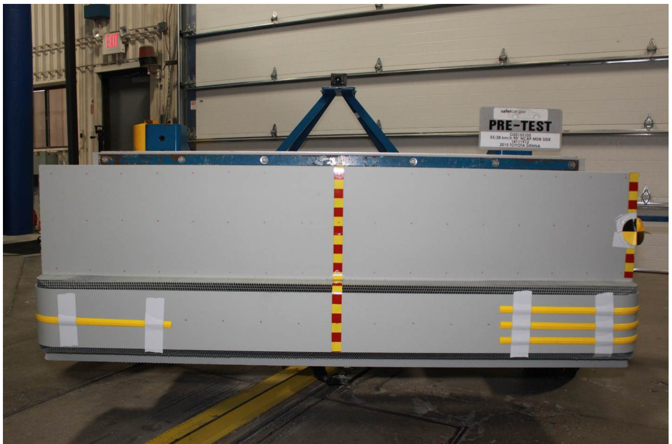
Pre-Test Front View of MDB Impactor Face
