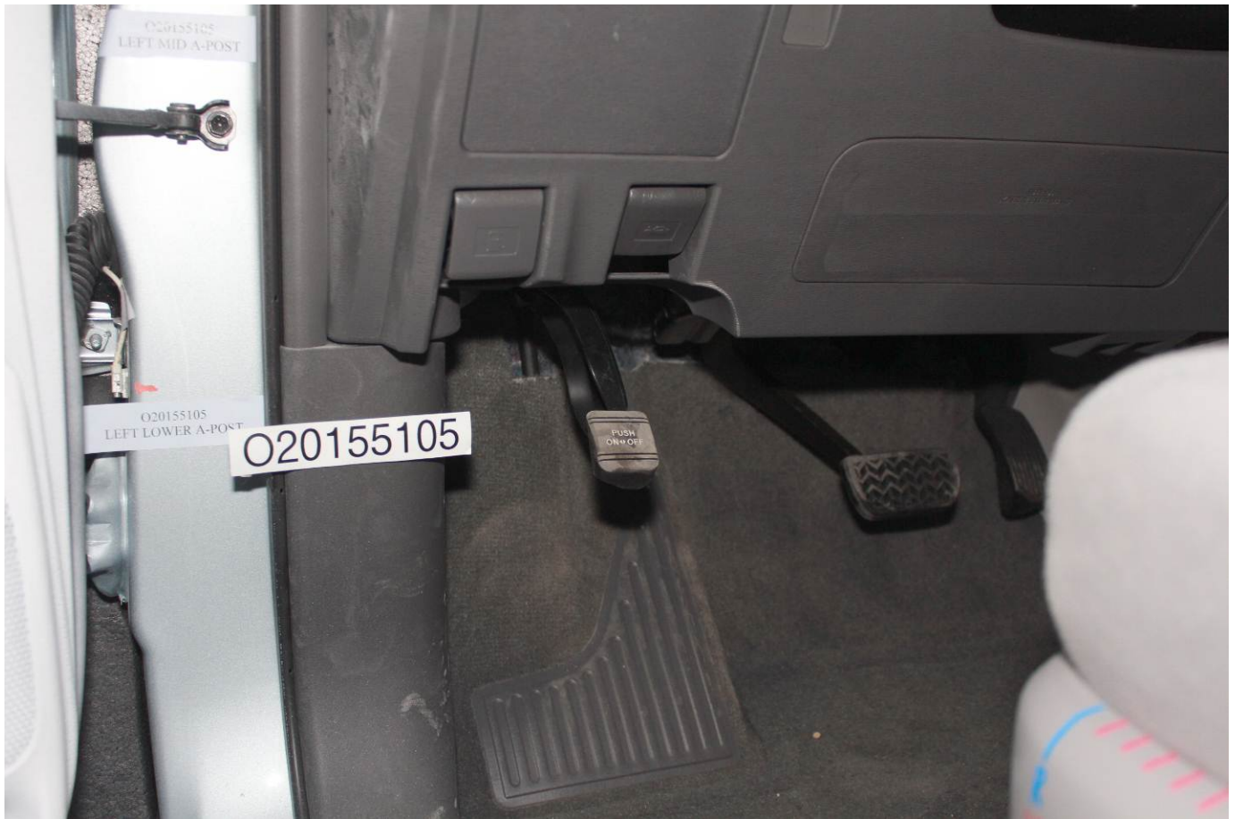
Pre-Test View of Disengaged Parking Brake
