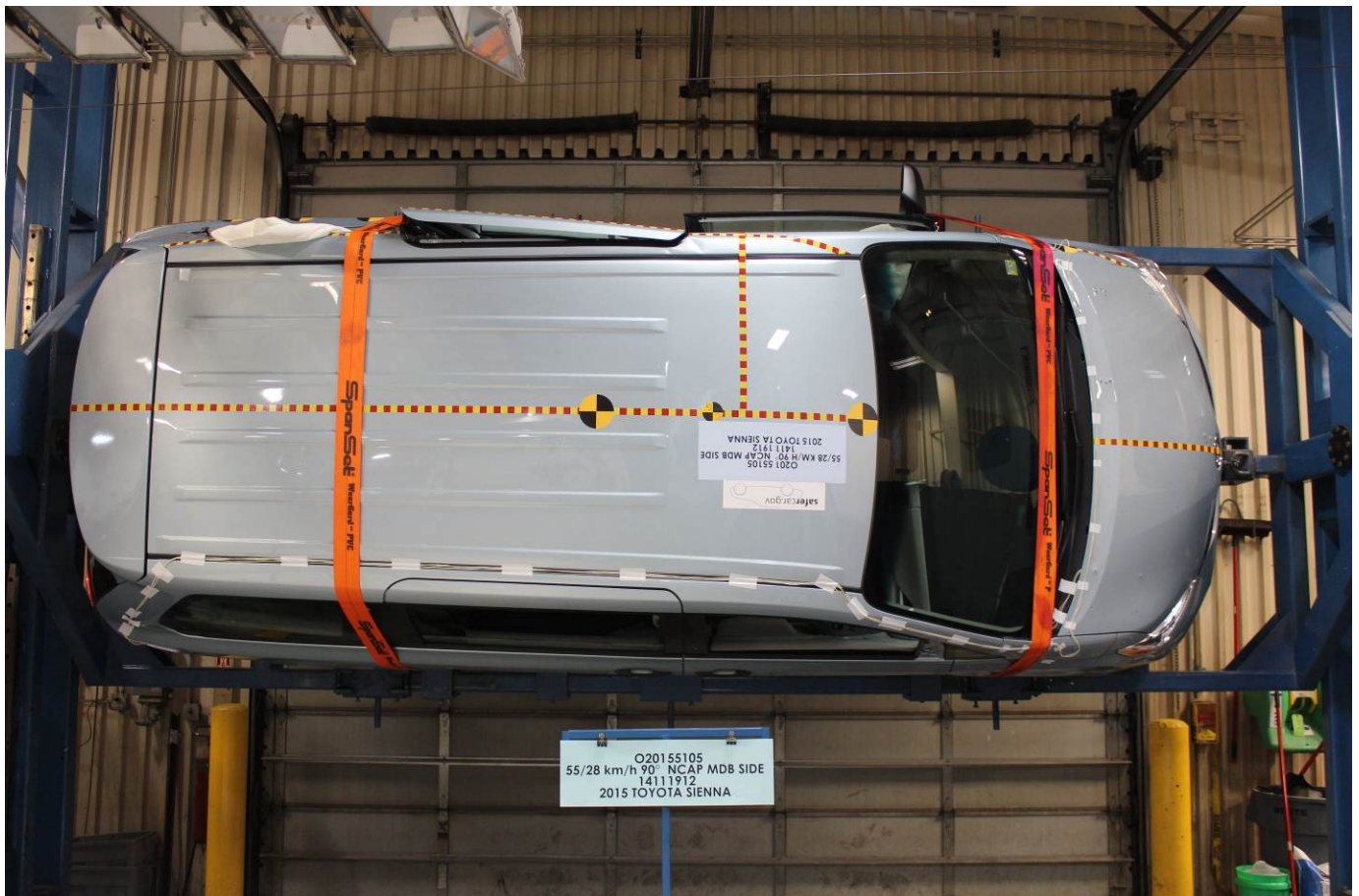
FMVSS No. 301 Static Rollover 270 Degrees
