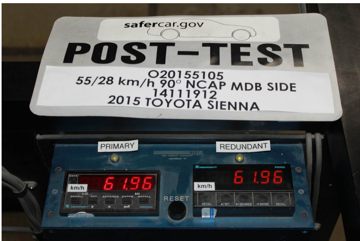
Post-Test Primary and Redundant Speed Trap Read-Out
