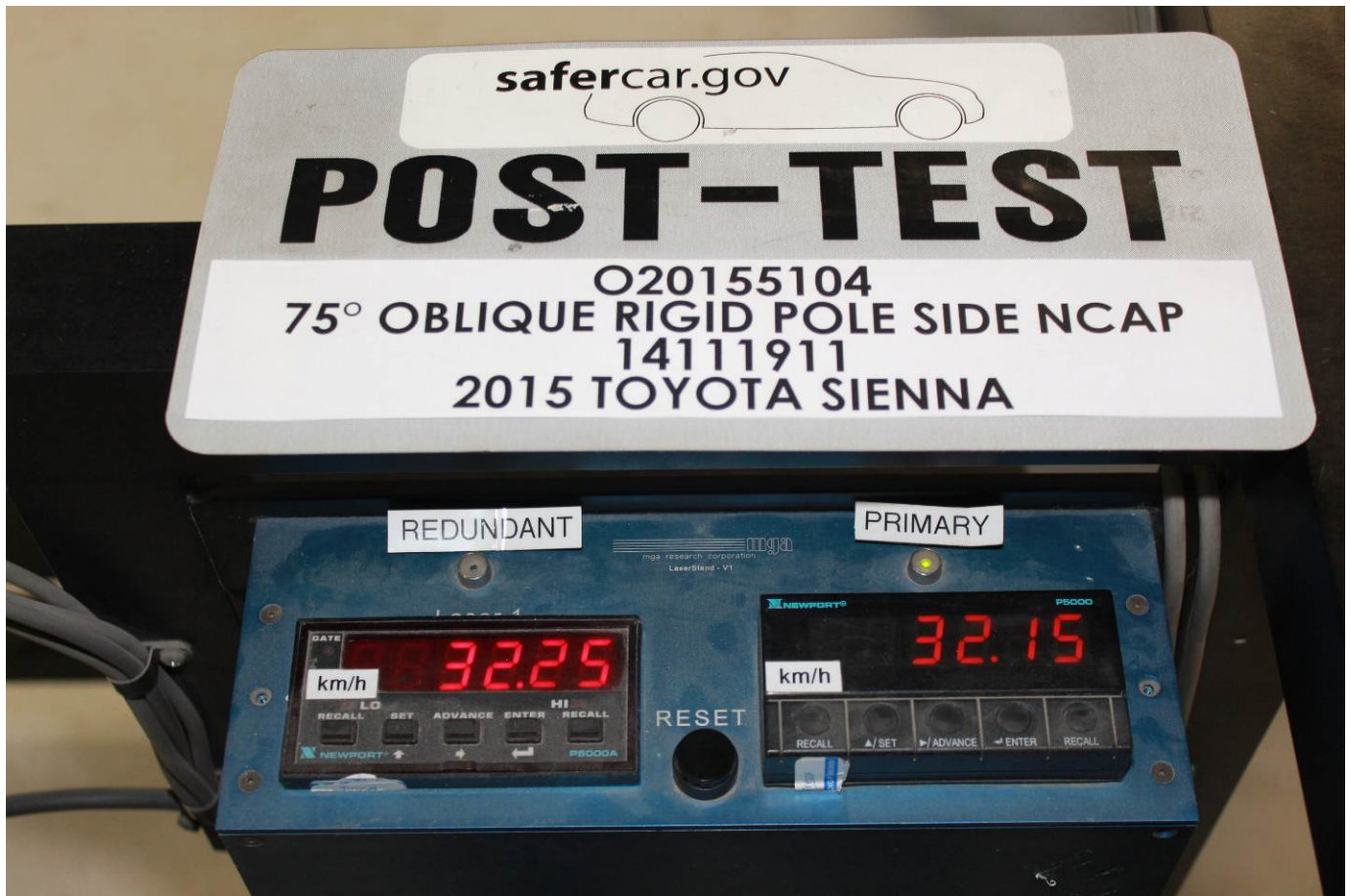
Post-Test Primary and Redundant Speed Trap Read-Out
