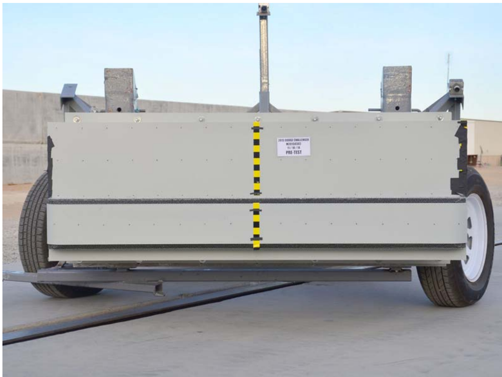
FIGURE 84. Pre-Test Front View of MDB Impactor Face
