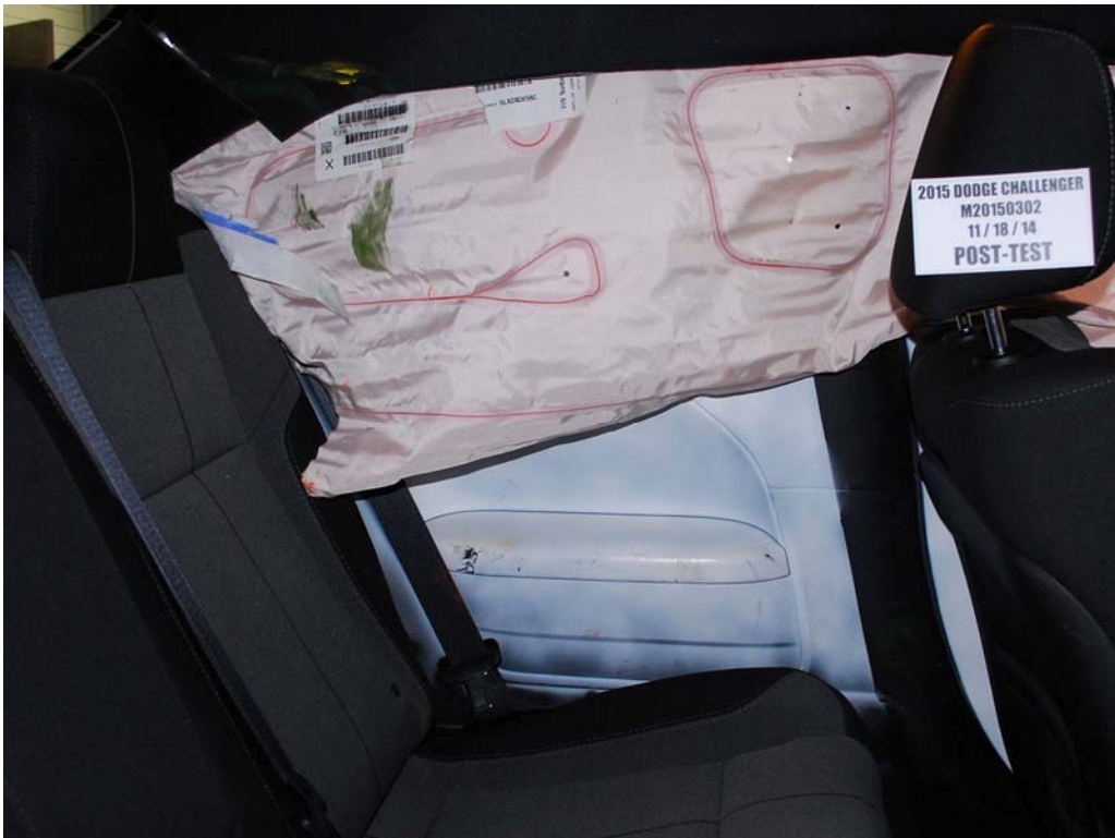
FIGURE 74. Post-Test Rear Passenger Inner Door Panel View Showing Rear Passenger Dummy Contact Locations
