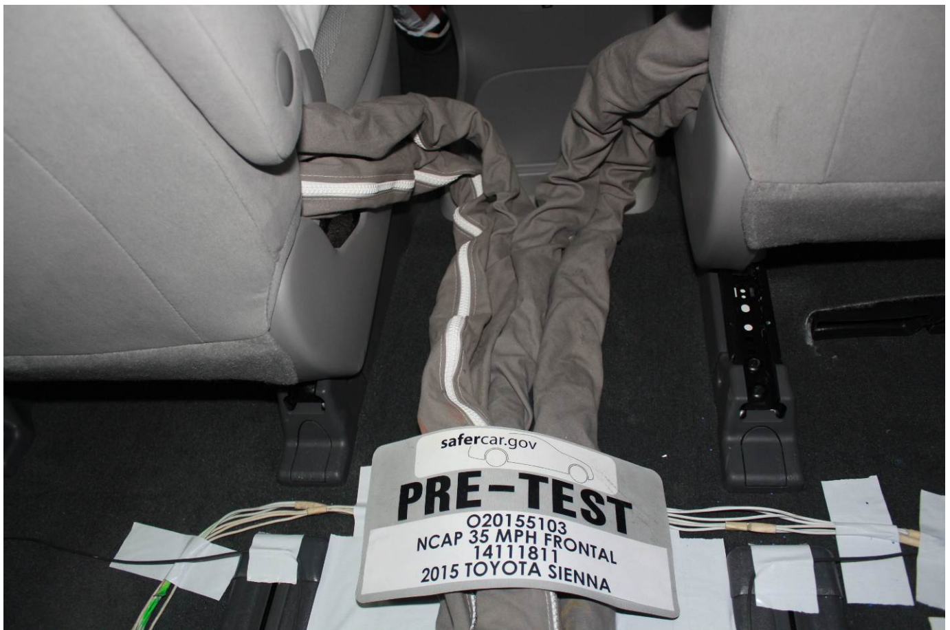
Pre-Test Dummy Cable Routing
