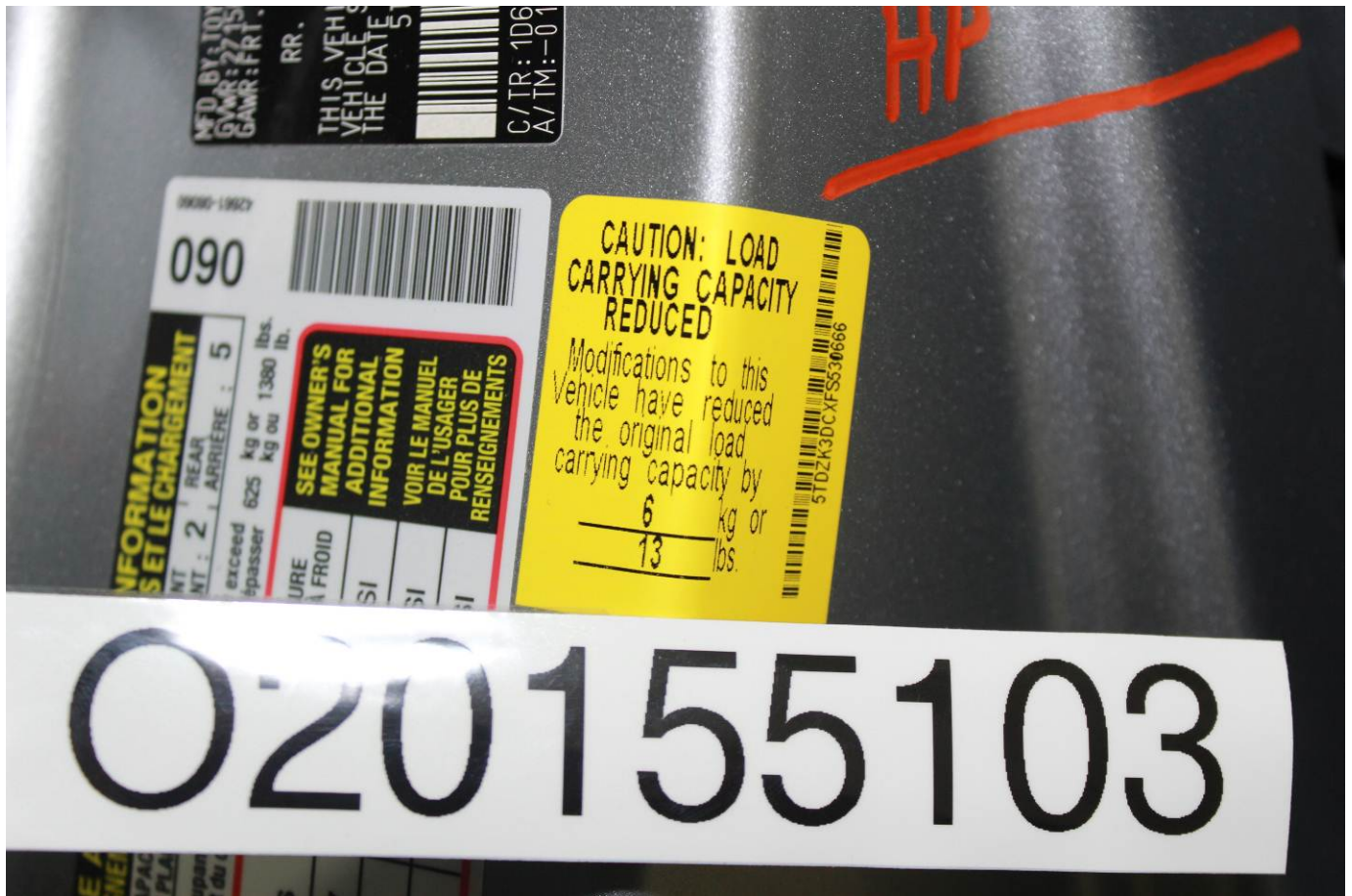
Load Carrying Capacity Reduced Label
