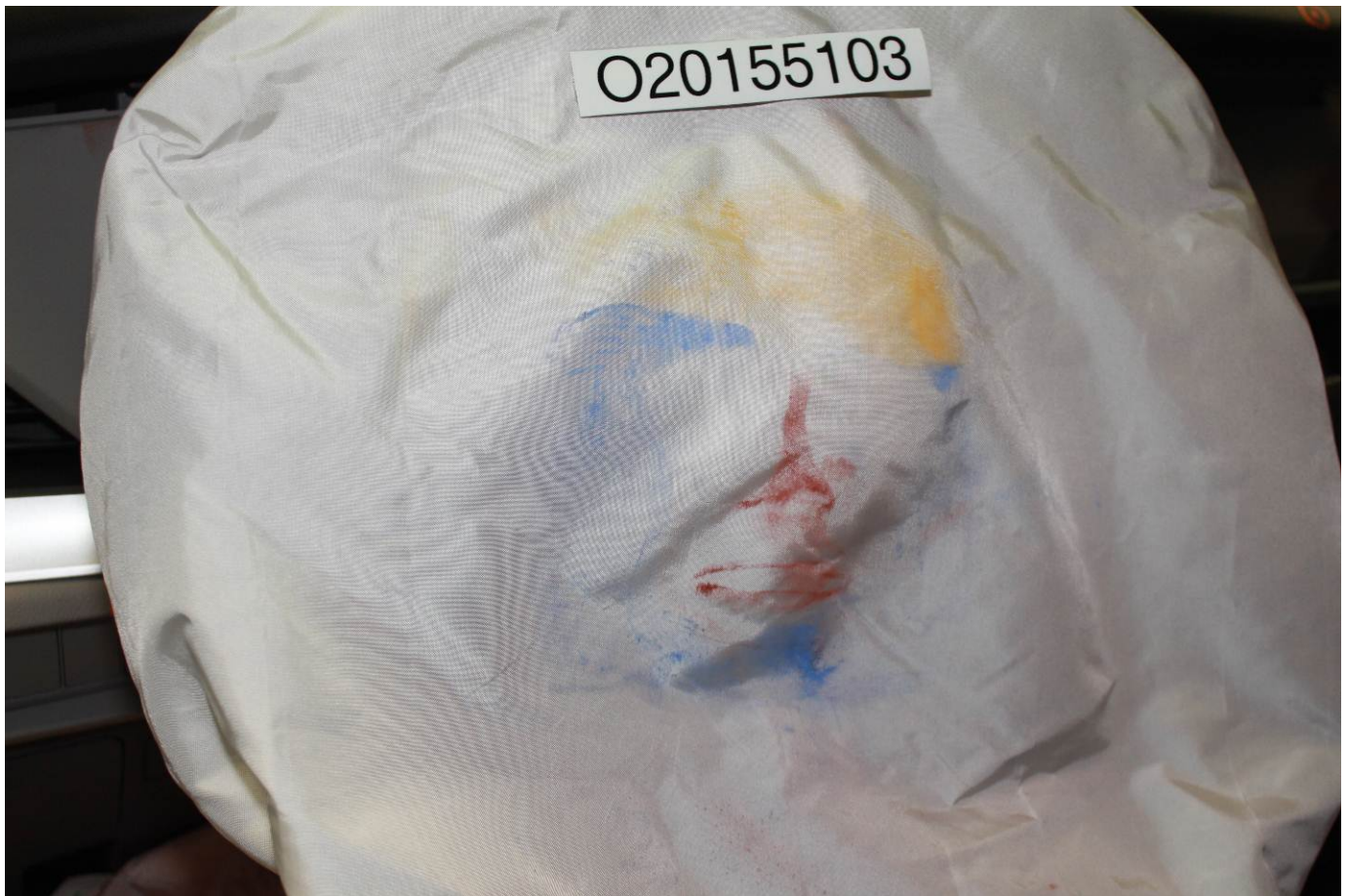
Post-Test Driver Dummy Contact with Airbag
