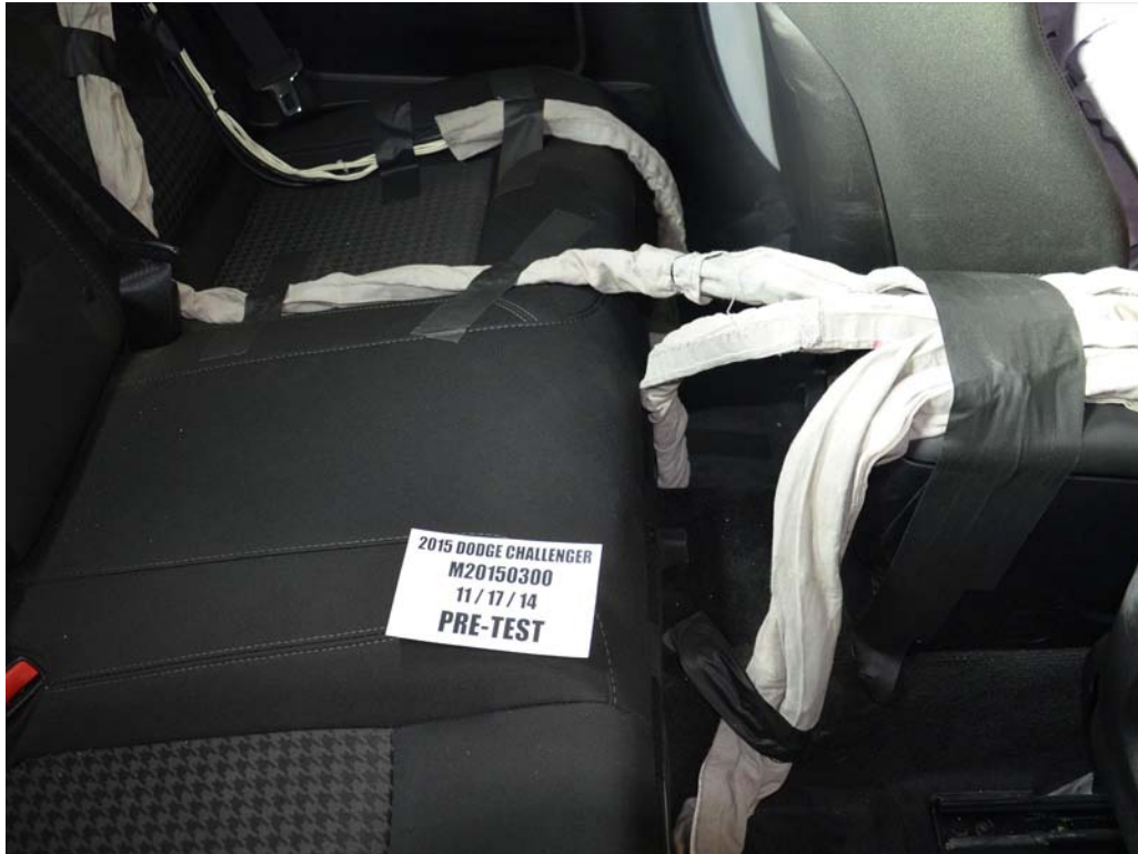
FIGURE 27. Pre-Test Dummy Cable Routing
