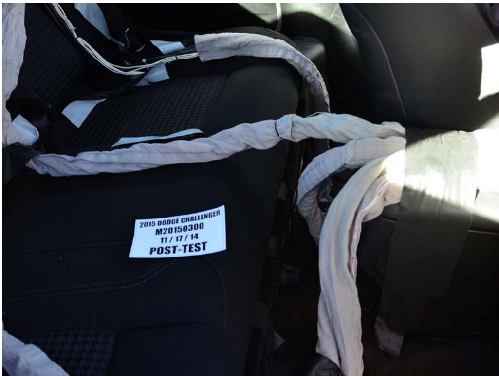
FIGURE 28. Post-Test Dummy Cable Routing
