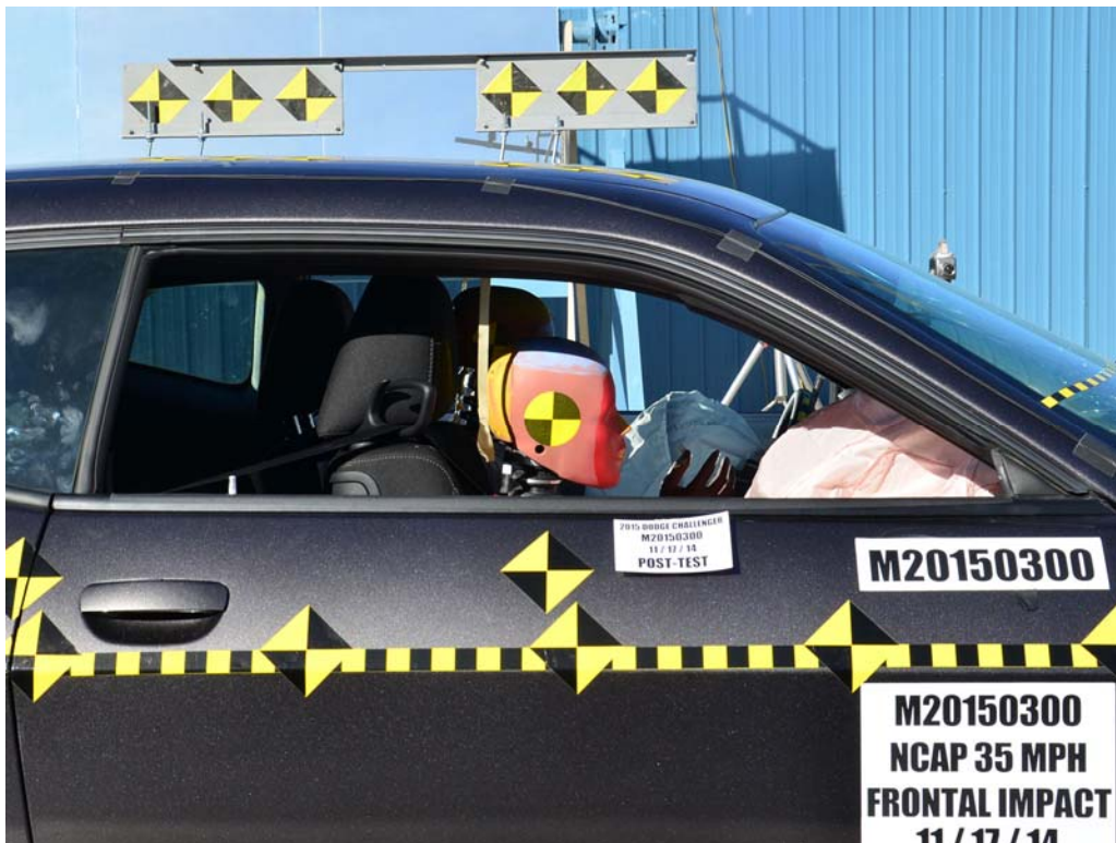
FIGURE 53. Post-Test Passenger Dummy Window View
