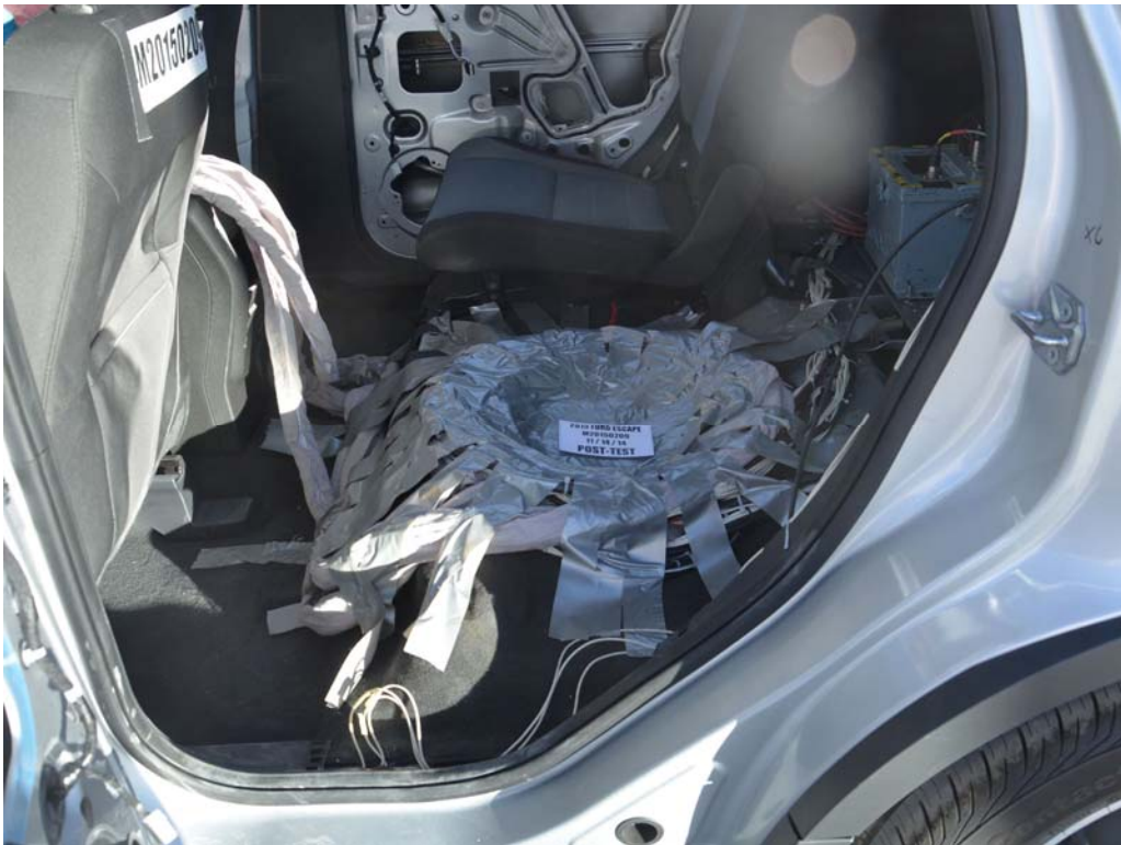
FIGURE 28. Post-Test Dummy Cable Routing
