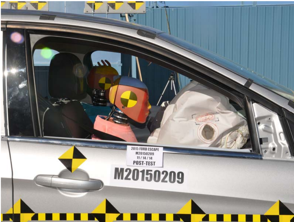
FIGURE 53. Post-Test Passenger Dummy Window View
