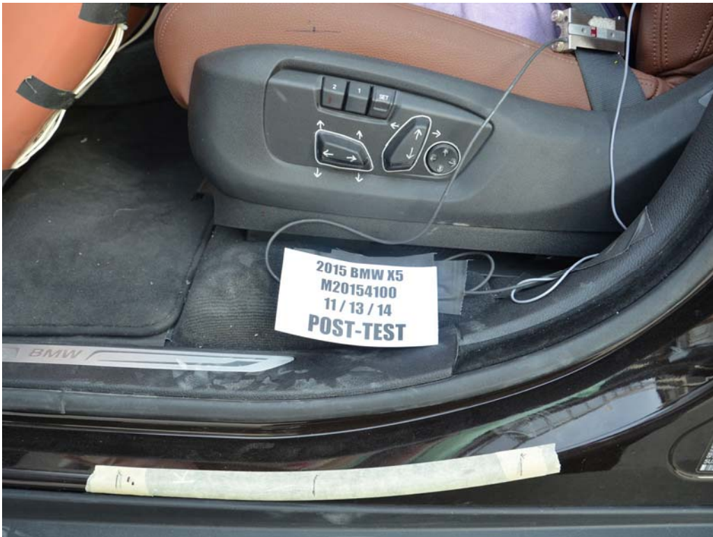
FIGURE 36. Post-Test Driver's Seat Fore-Aft Markings
