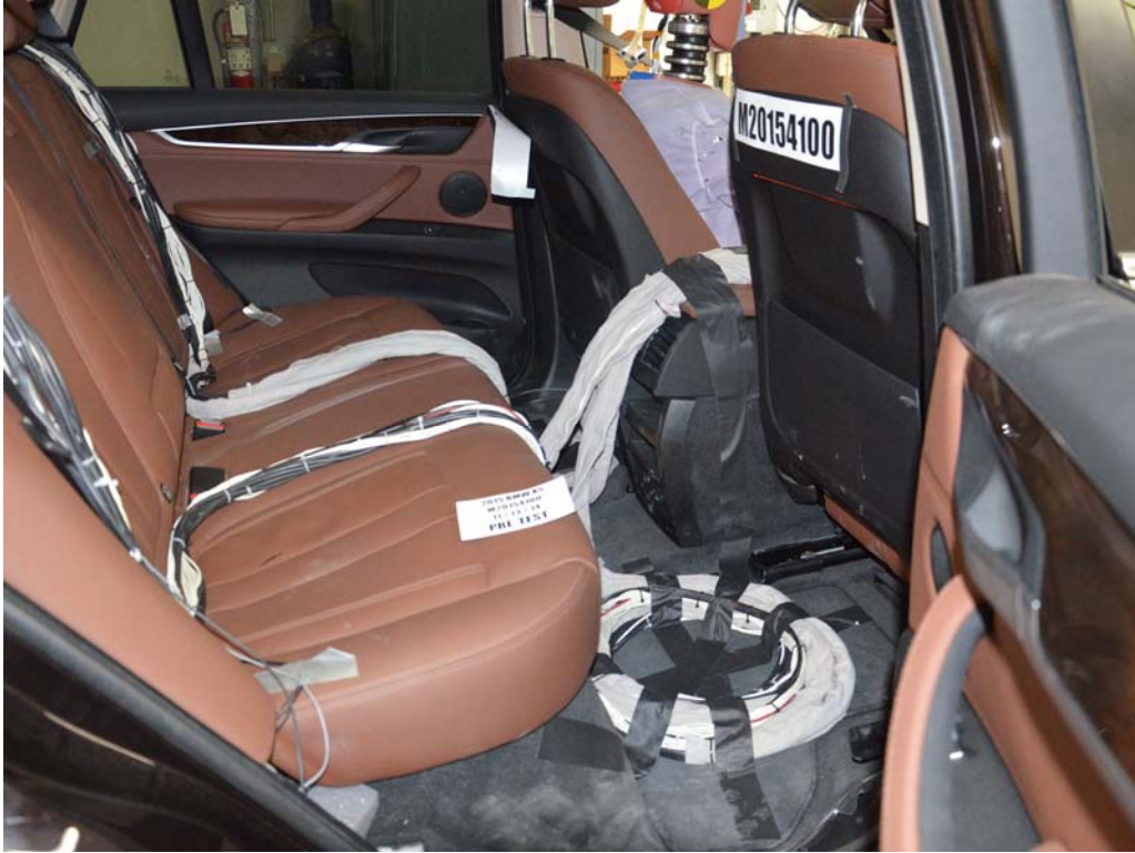
FIGURE 27. Pre-Test Dummy Cable Routing
