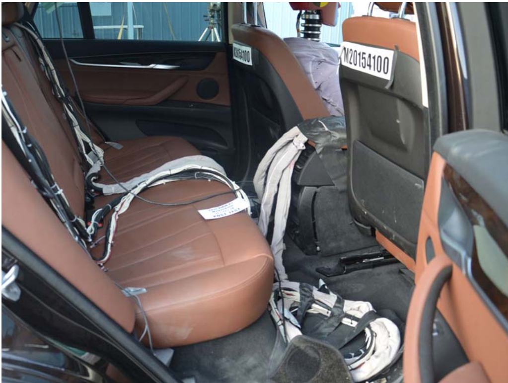
FIGURE 28. Post-Test Dummy Cable Routing
