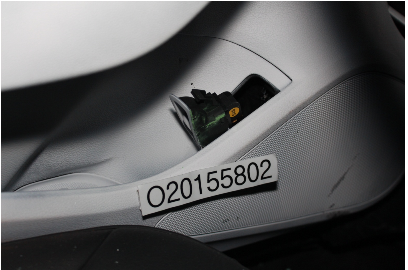
Post-Test Driver Dummy Close-up Knee Contact View
