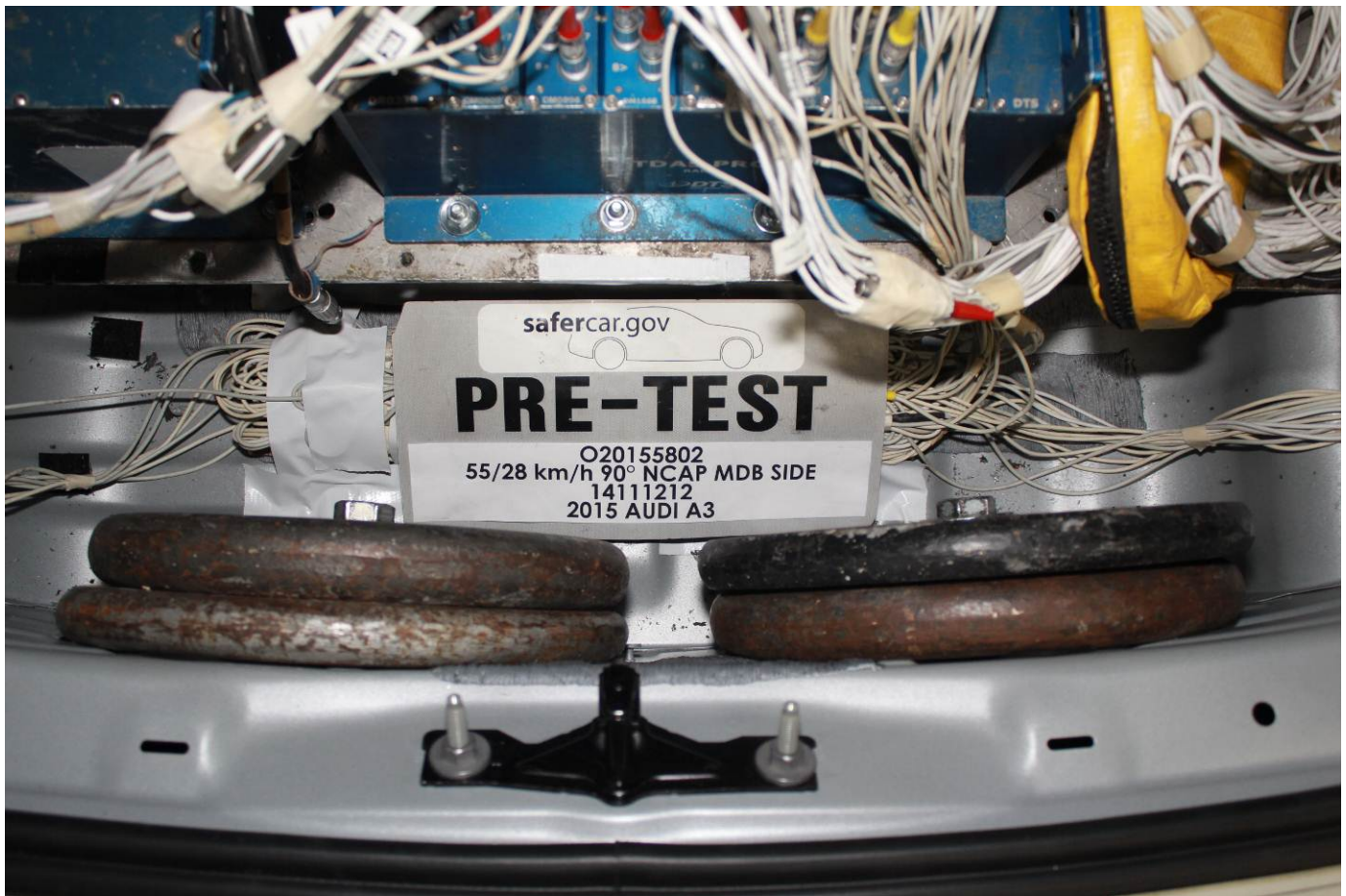
Pre-Test Ballast View
