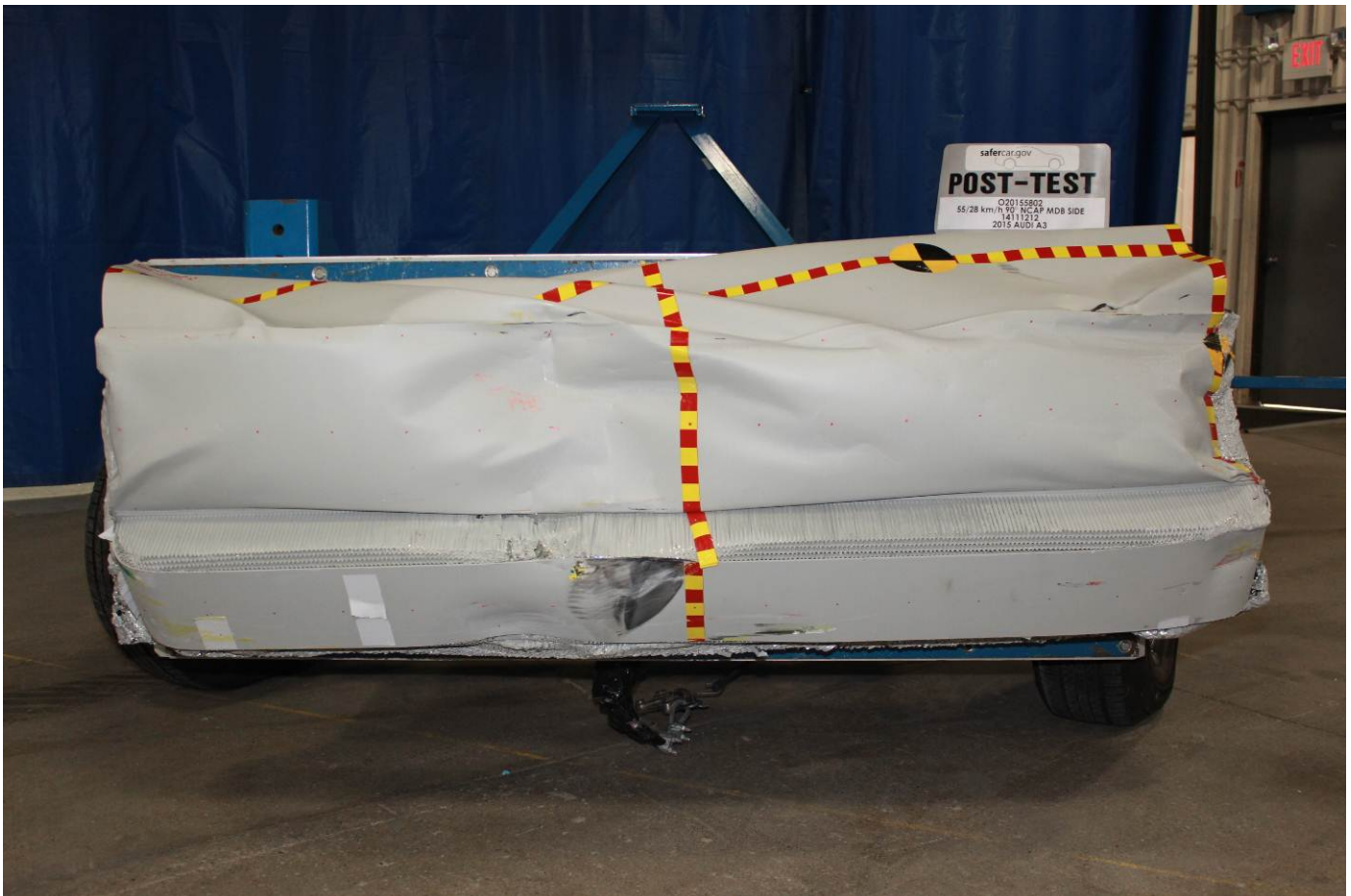
Post-Test Front View of MDB Impactor Face
