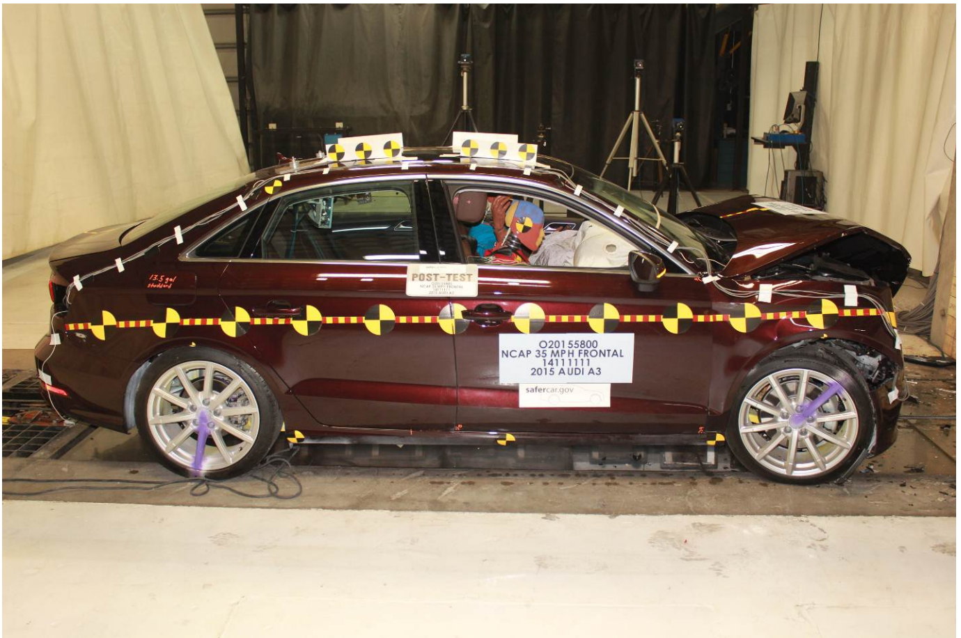
Post-Test Right View of Test Vehicle
