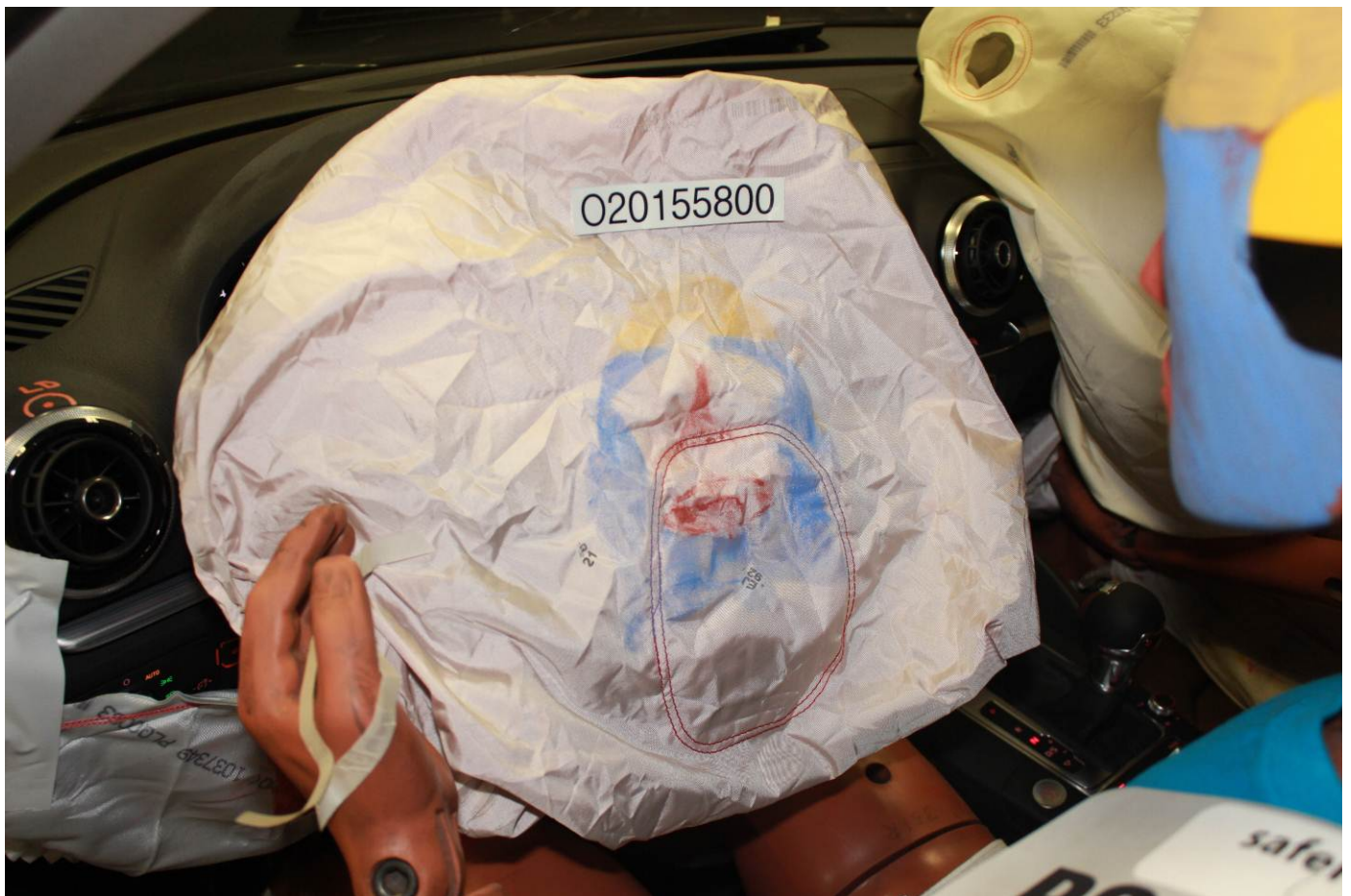
Post-Test Driver Dummy Contact with Airbag
