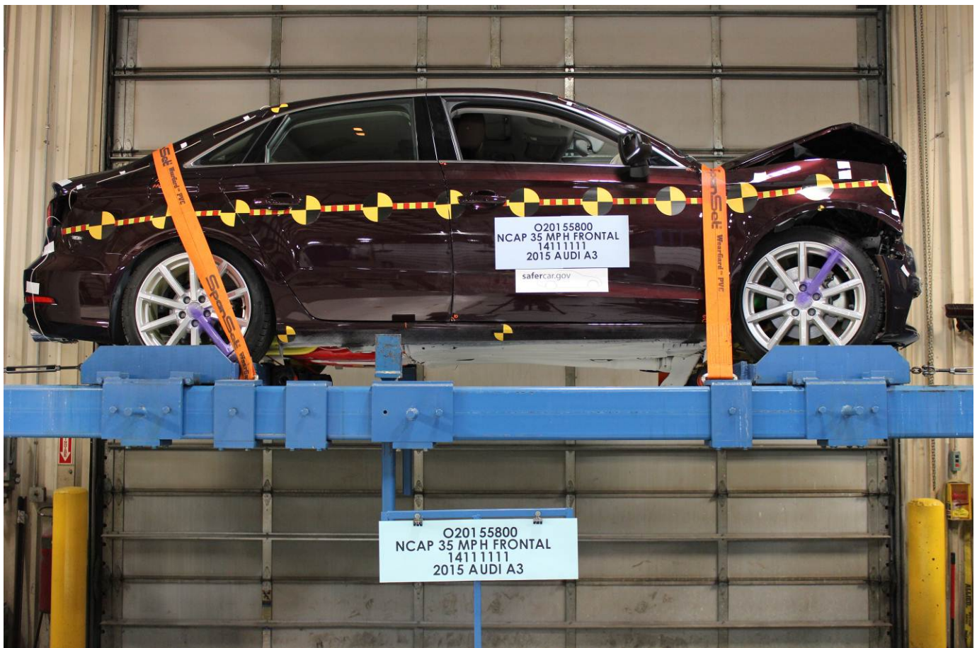
Vehicle at 0 Degree on Static Rollover Device
