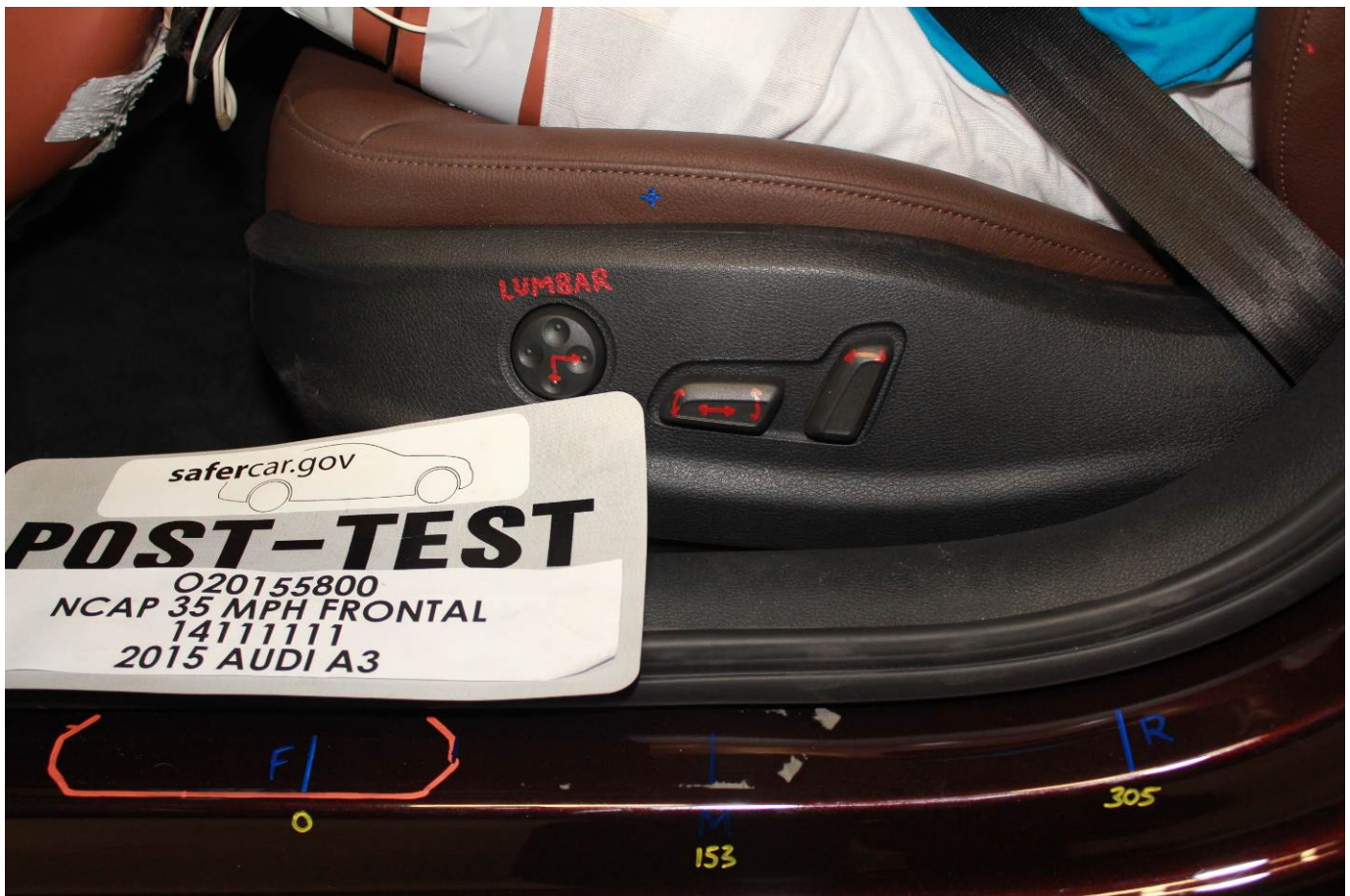
Post-Test Driver's Seat Fore-Aft Markings
