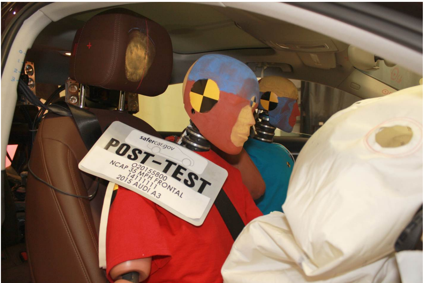
Post-Test Passenger Dummy Face
