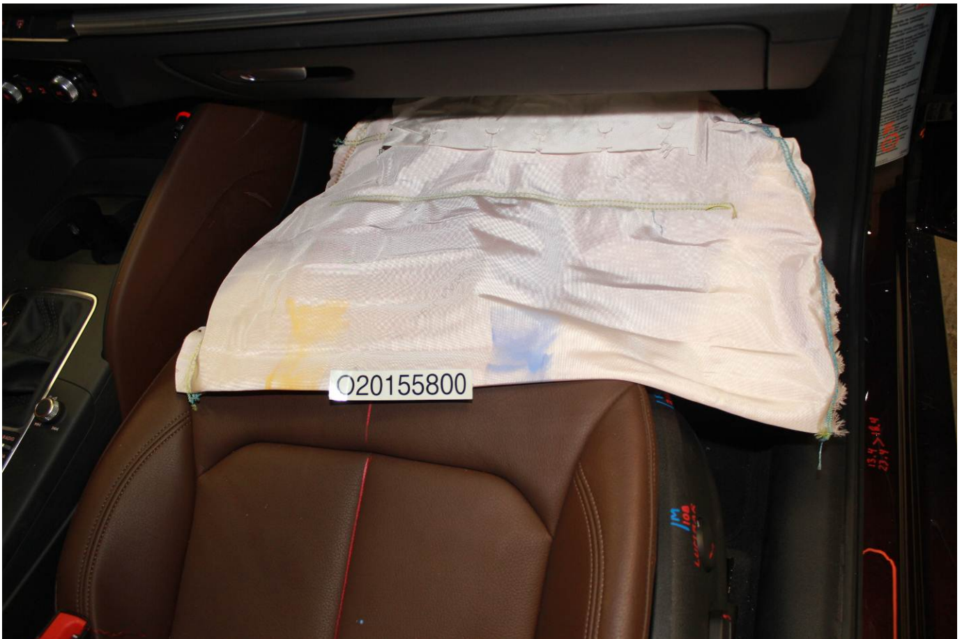
Post-Test Passenger Dummy Contact with Knee Airbag
