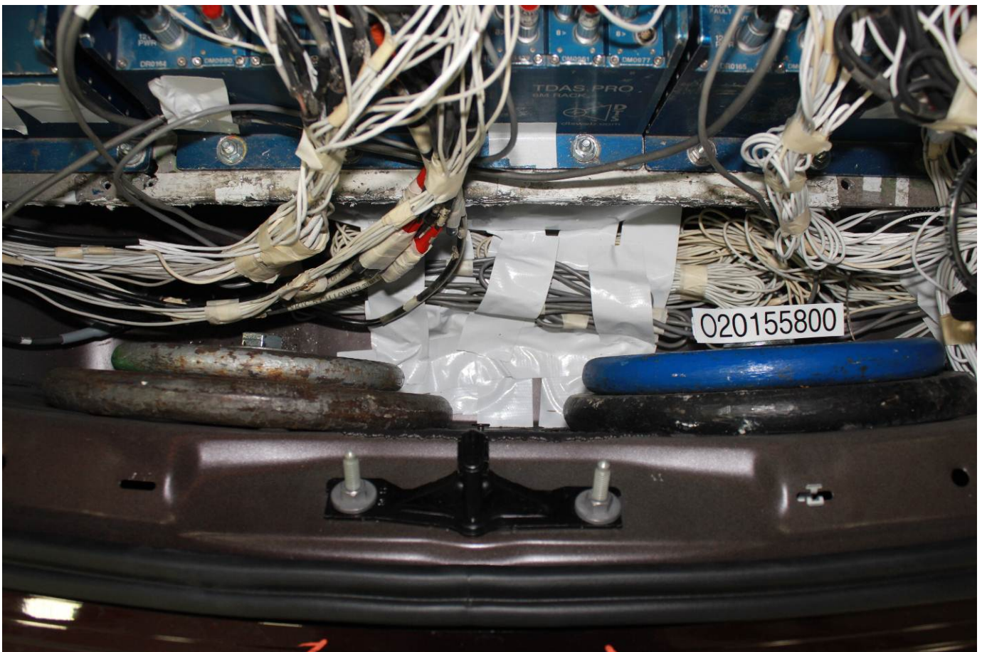
Ballast Installed in Vehicle
