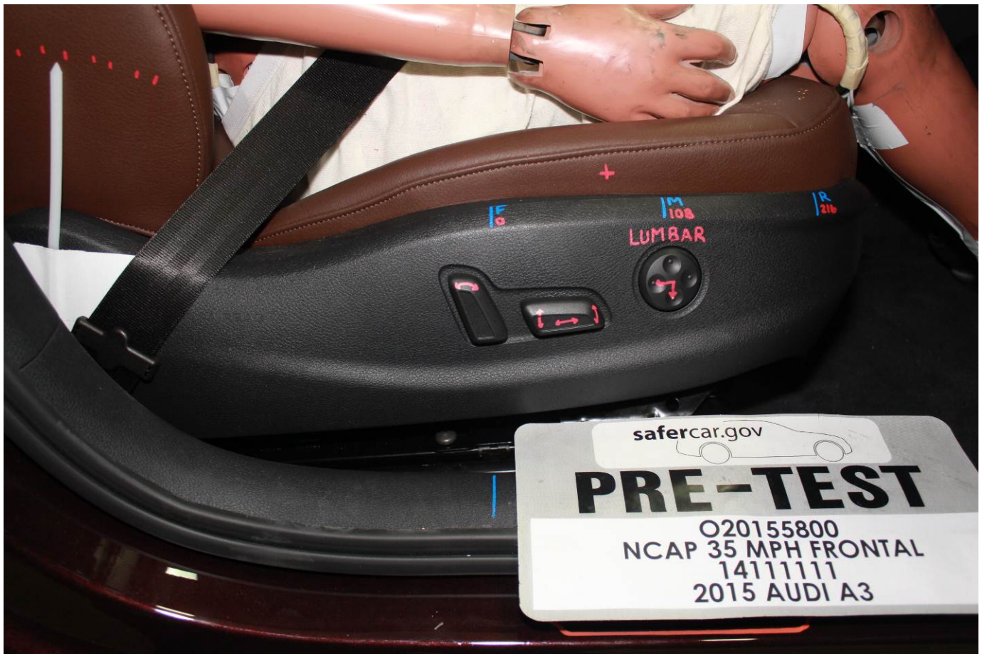
Pre-Test Passenger's Seat Fore-Aft Markings
