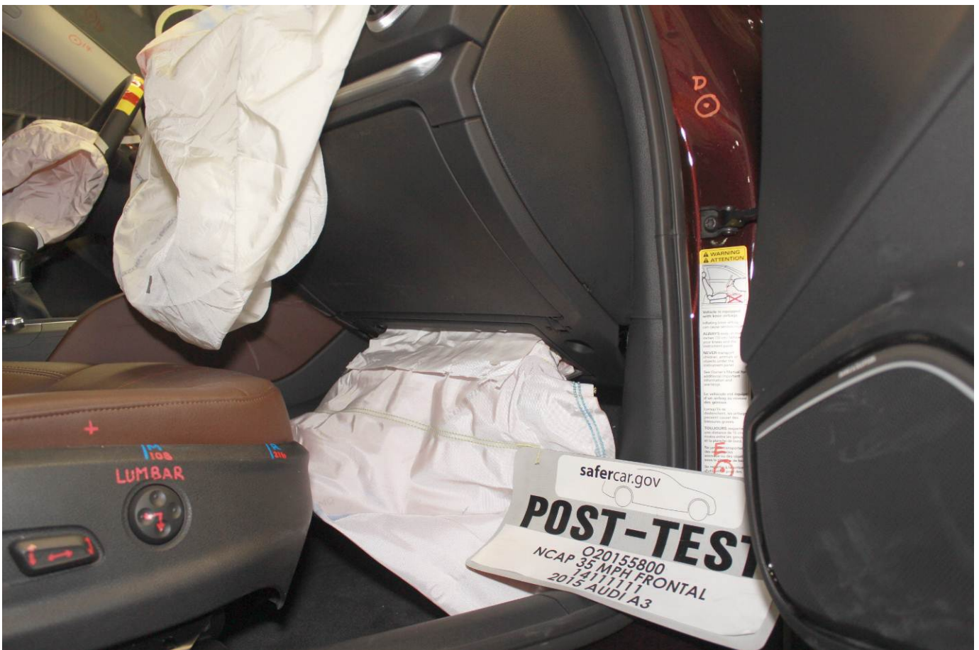
Post-Test Passenger's Side Knee Bolster (without dummy)
