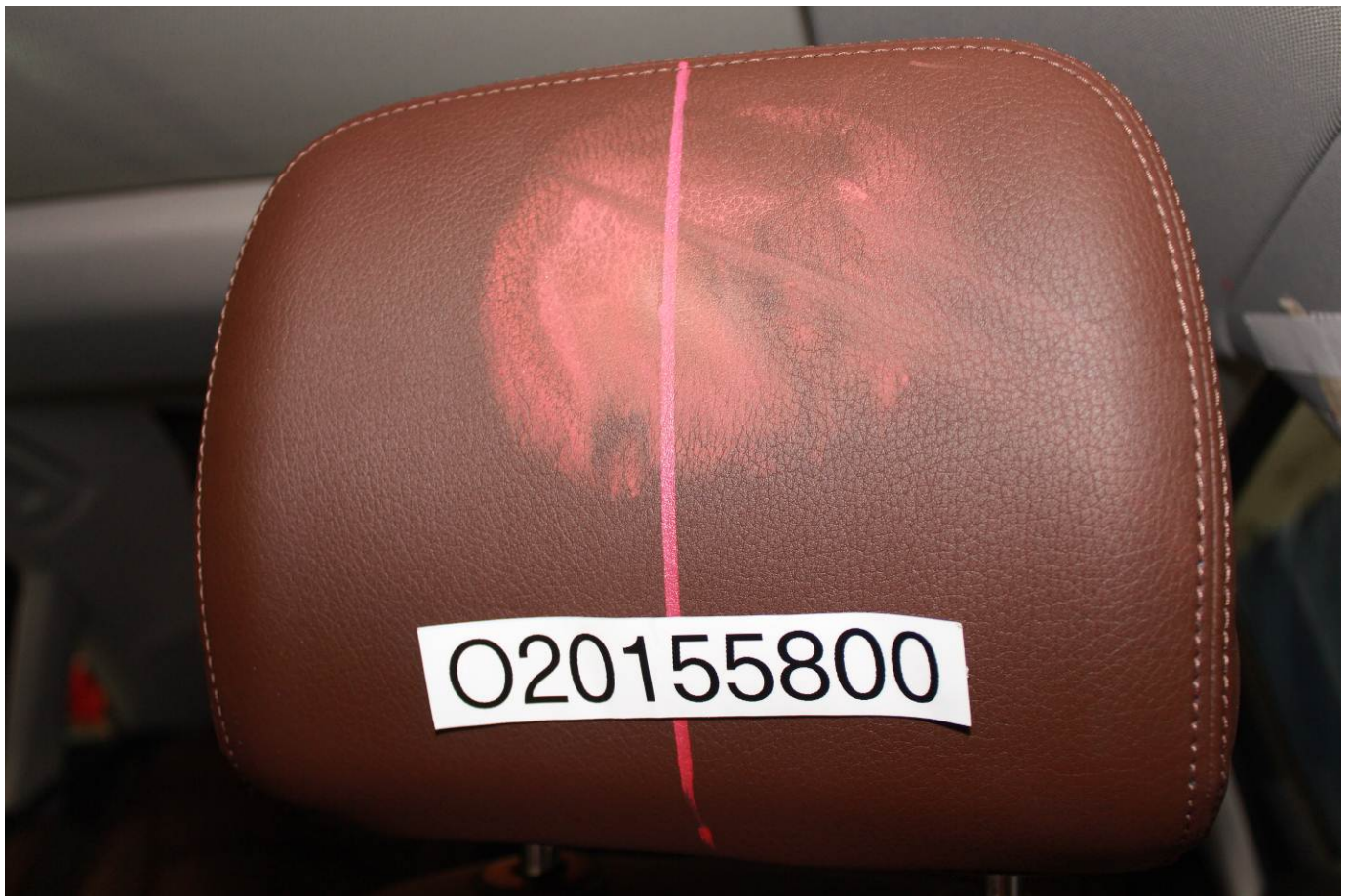
Post-Test Driver Dummy Contact with Headrest
