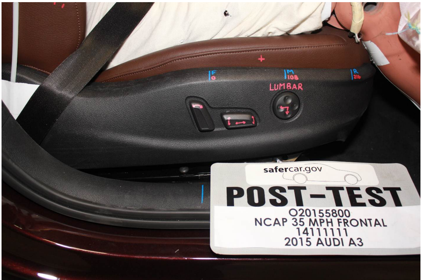
Post-Test Passenger's Seat Fore-Aft Markings
