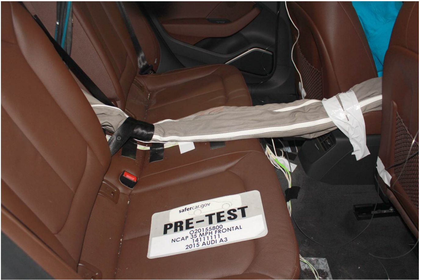
Pre-Test Dummy Cable Routing
