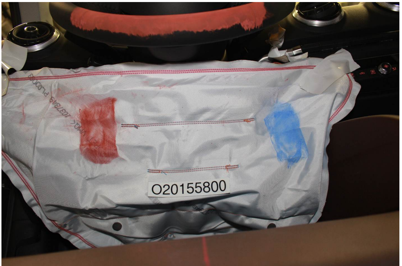
Post-Test Driver Dummy Contact with Knee Airbag
