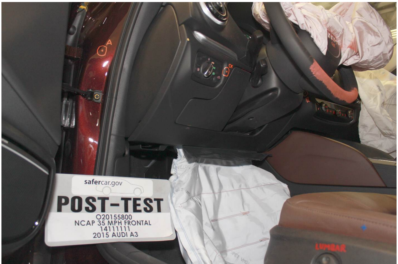
Post-Test Driver's Side Knee Bolster (without dummy)
