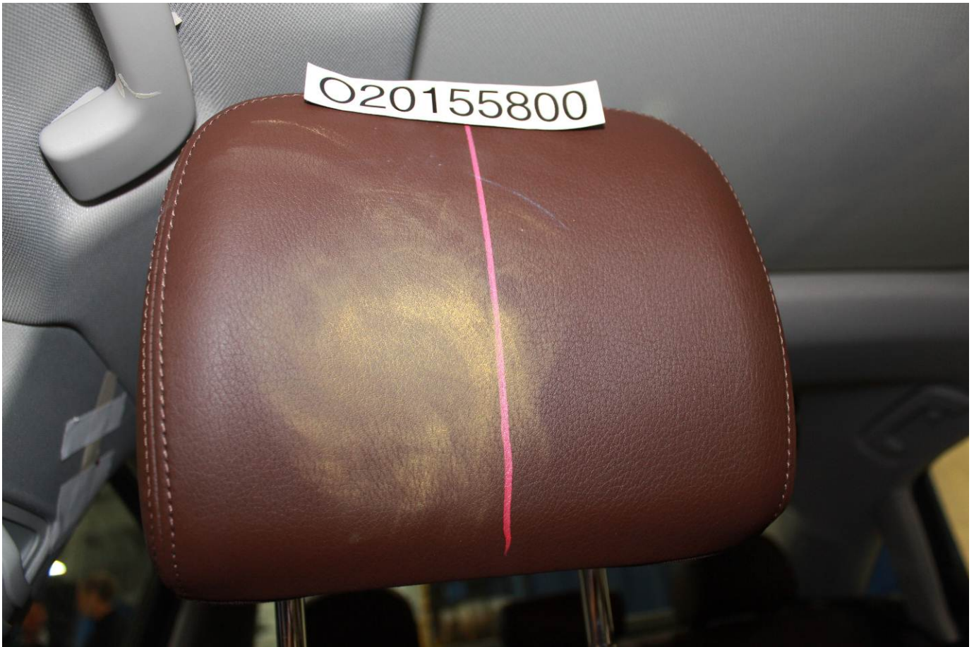
Post-Test Passenger Dummy Contact with Headrest
