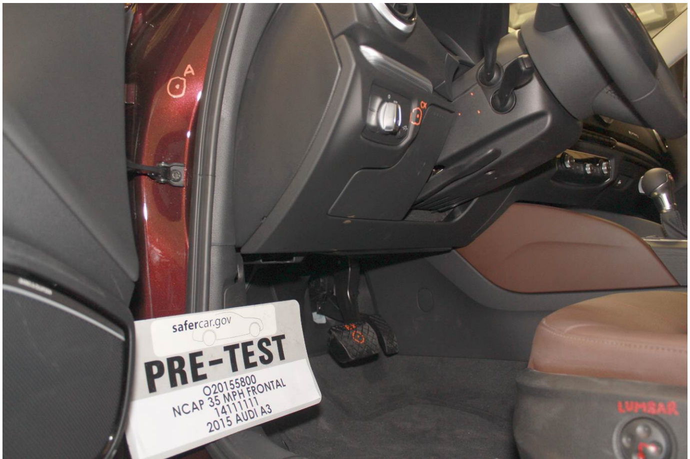
Pre-Test Driver's Side Knee Bolster (without dummy)
