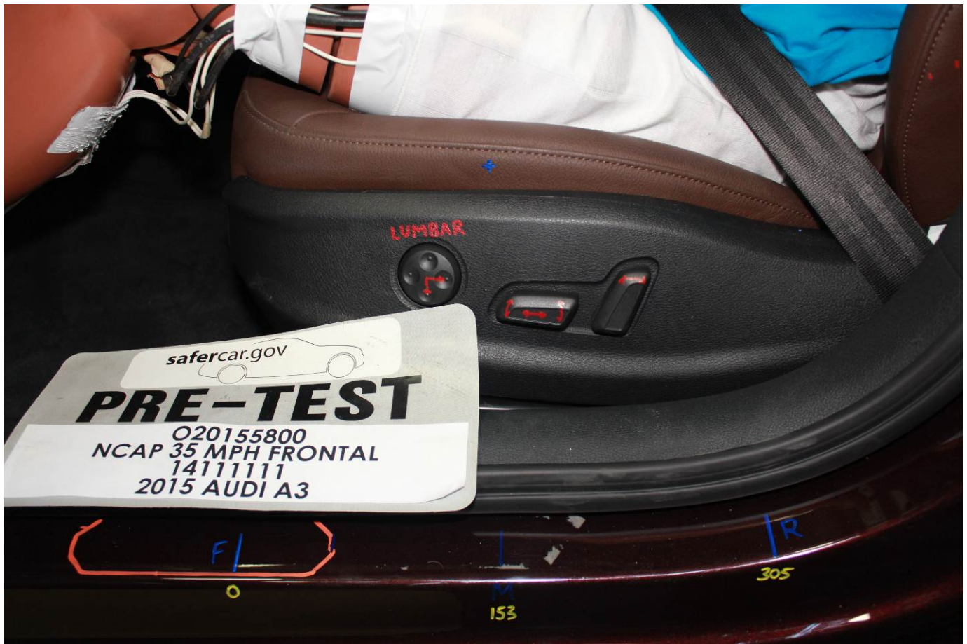
Pre-Test Driver's Seat Fore-Aft Markings
