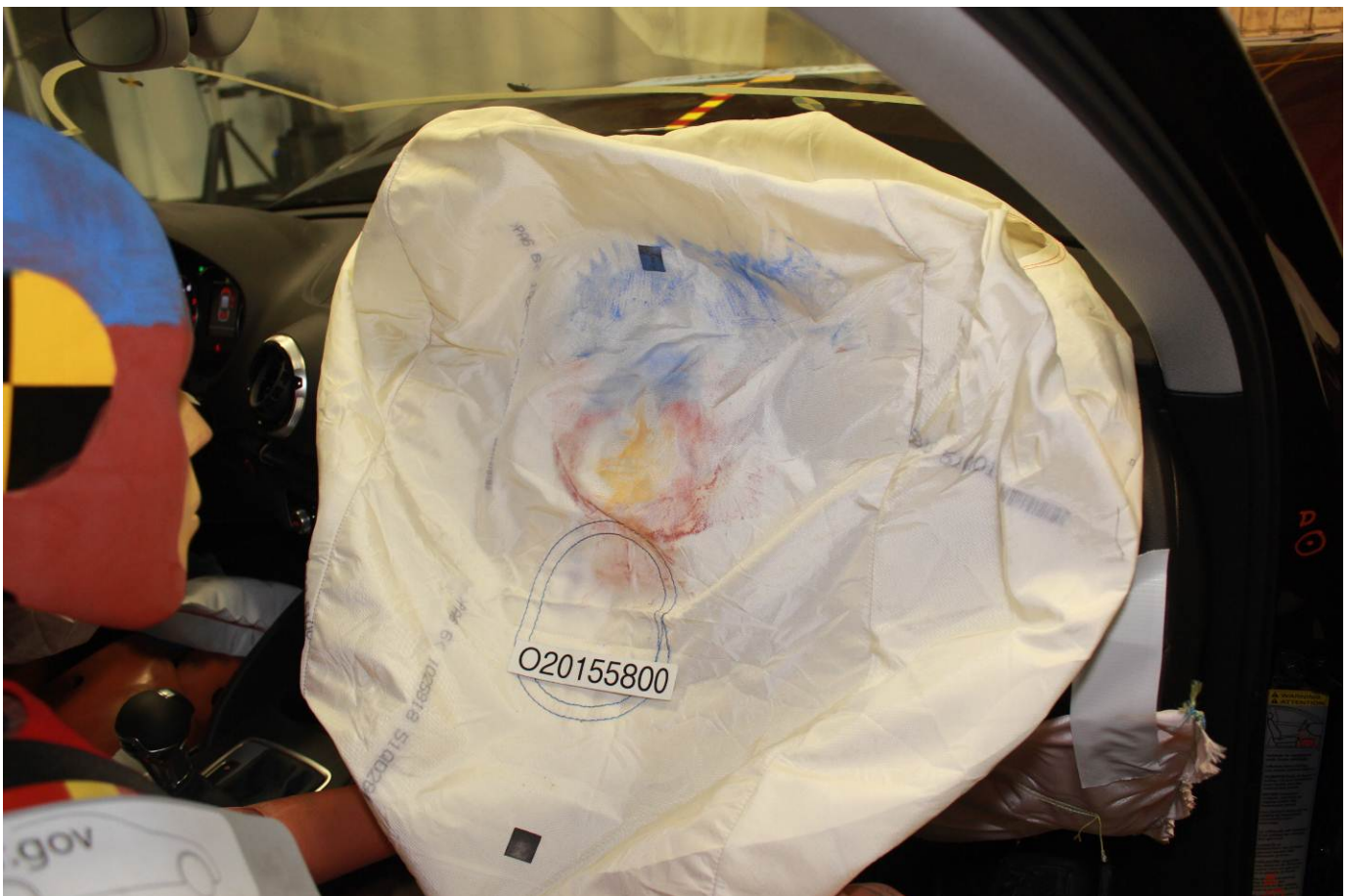
Post-Test Passenger Dummy Contact with Airbag
