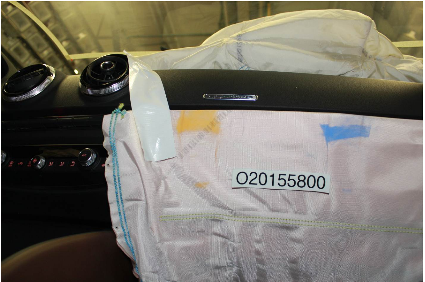
Post-Test Passenger Dummy Contact with Knee Airbag
