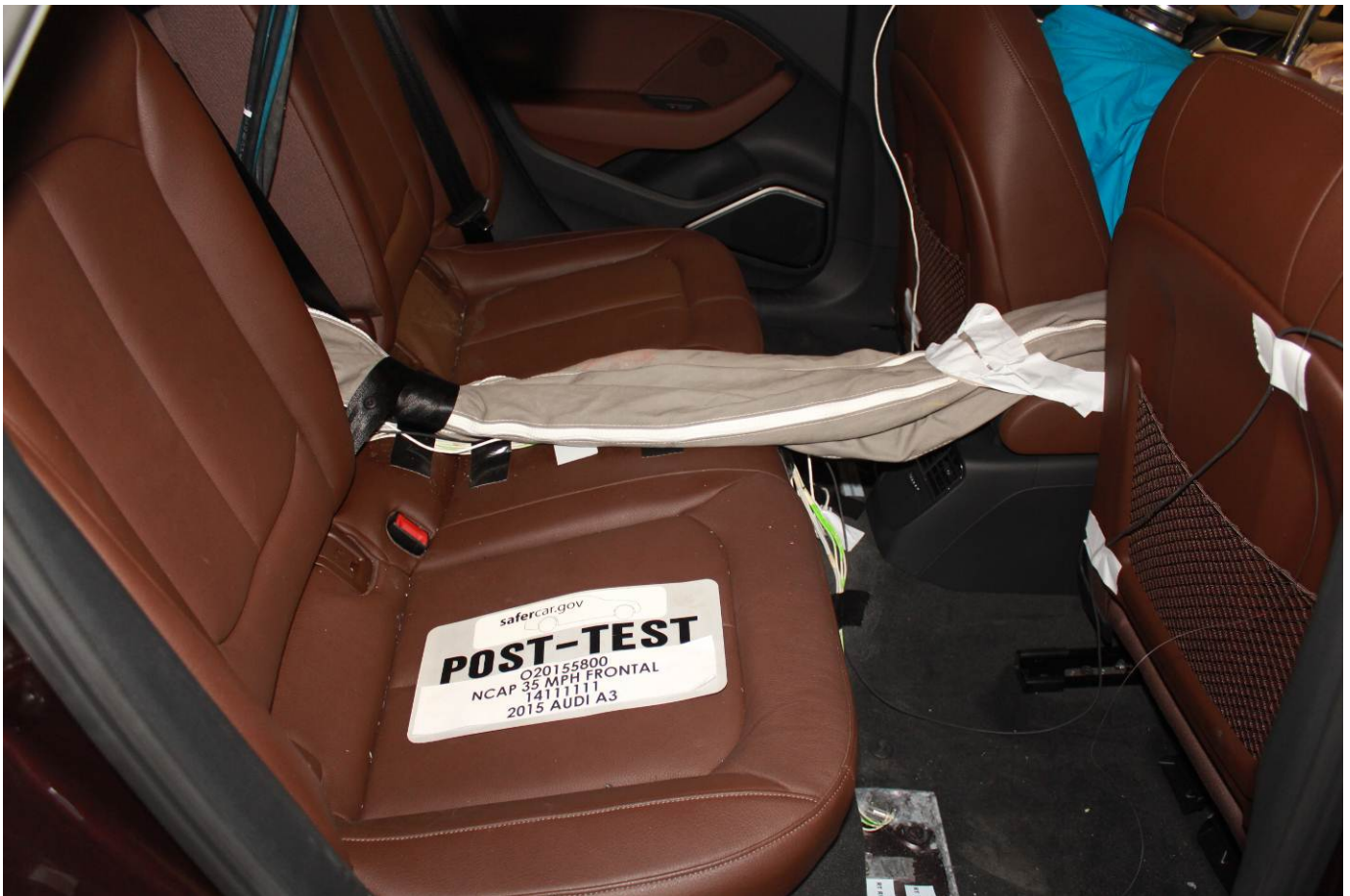
Post-Test Dummy Cable Routing
