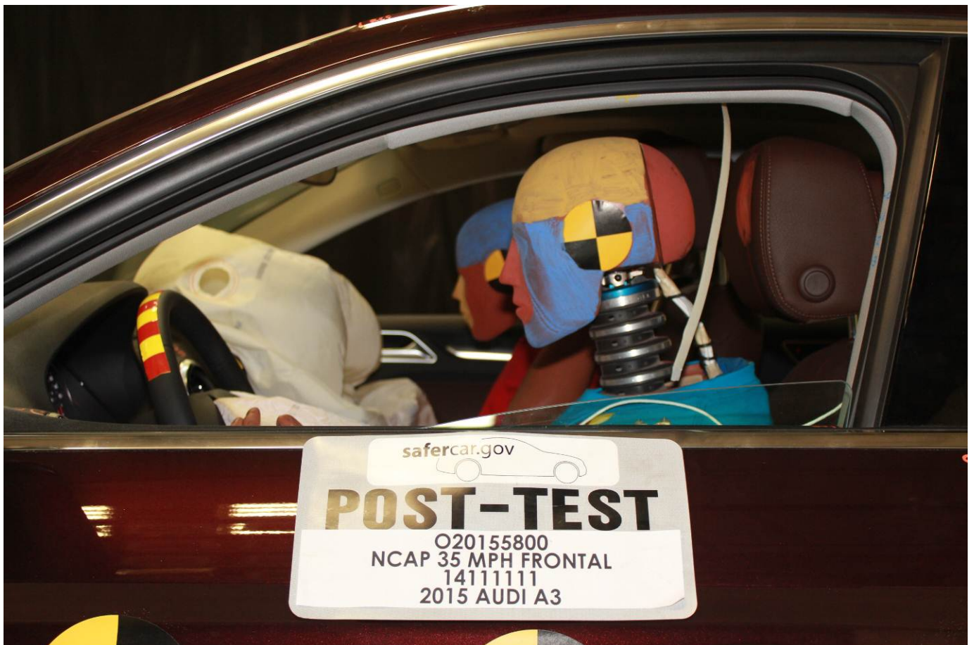
Post-Test Driver Dummy Window View
