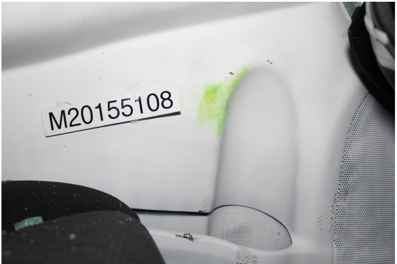
Post-Test Driver Dummy Close-up Knee Contact View
