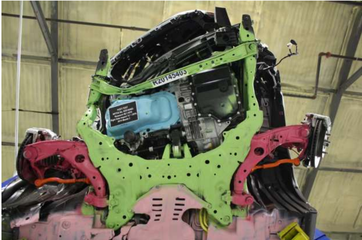
No. 139 Post-Test View of Front Sub-Frame Deformation
