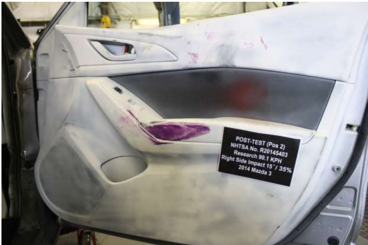
No. 121a Post-Test View of Passenger Body contact with Interior
