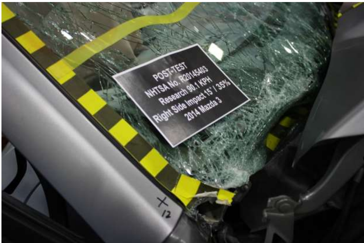
No. 161 Post-Test View of Windshield Separation
