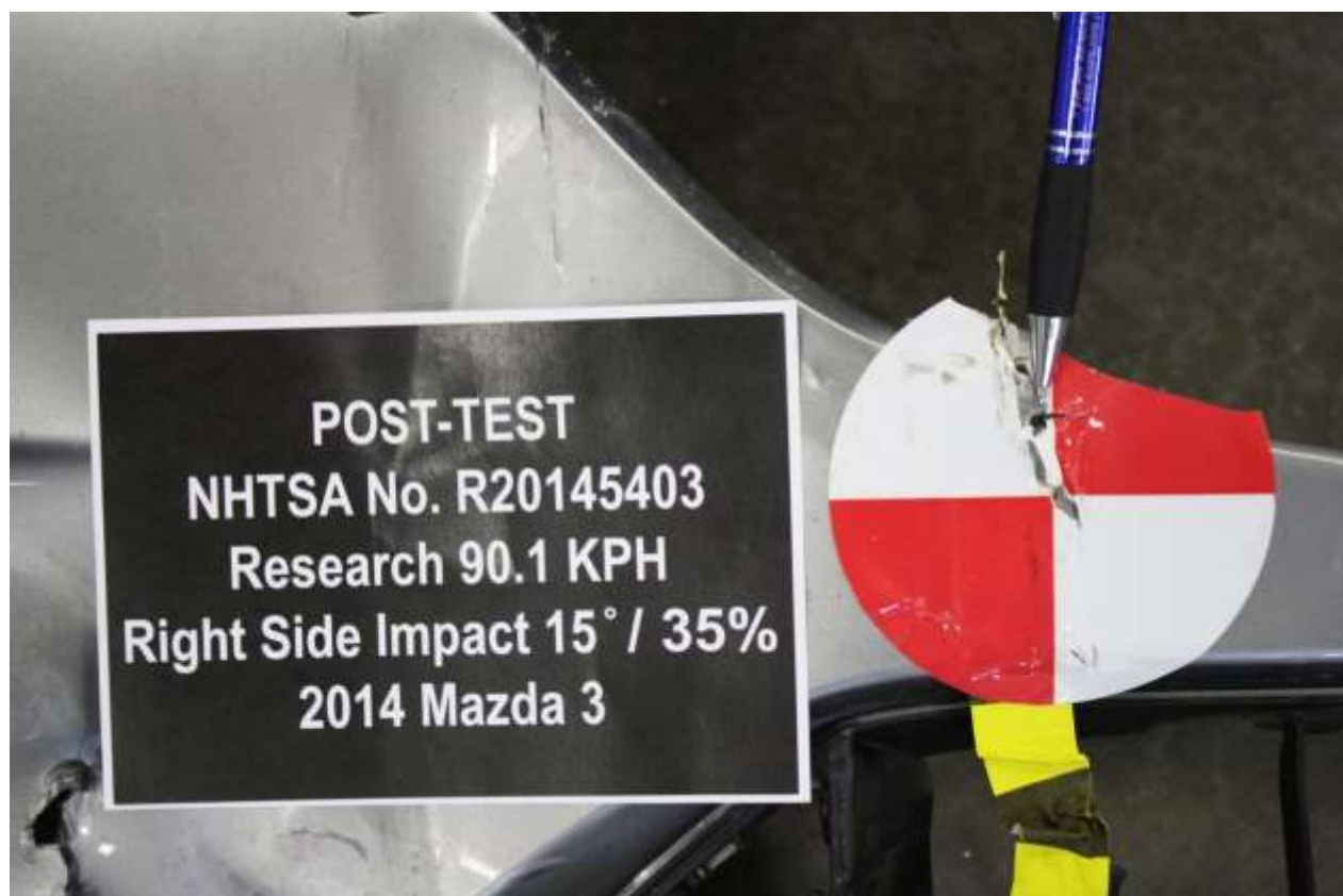
No. 026 Post-Test Close-up View of Impact Point
