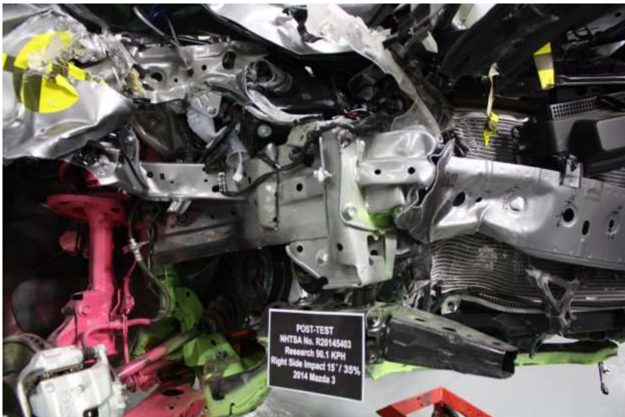
No. 153 Post-Test Right Side \frac{3}{4} View of Front Passenger Shotgun
