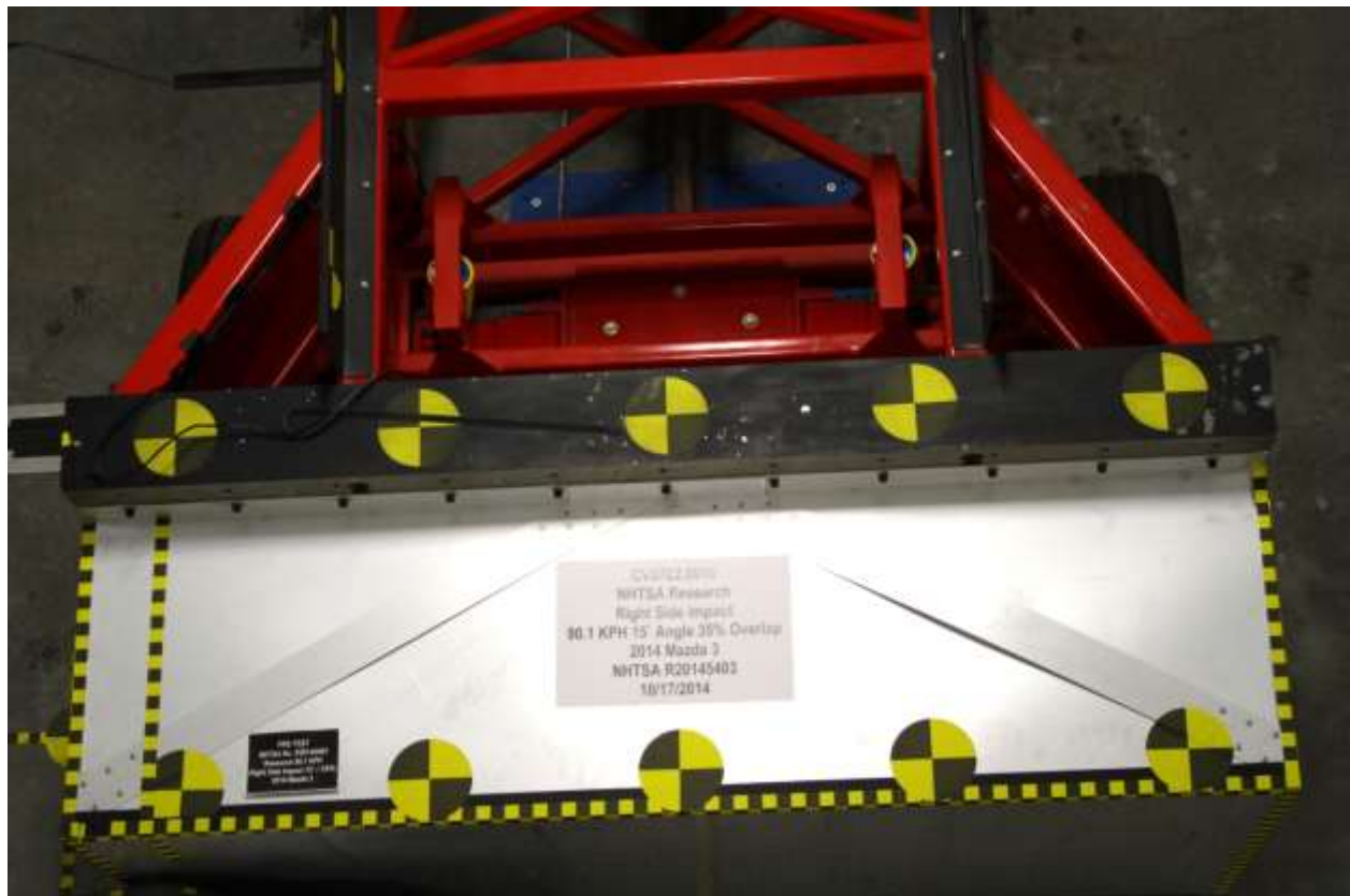
No. 166 Pre-Test Top View of RMDB
