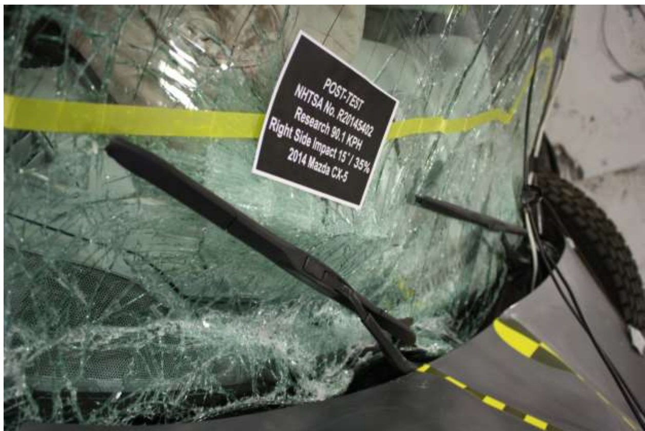
No. 161 Post-Test View of Windshield Separation
