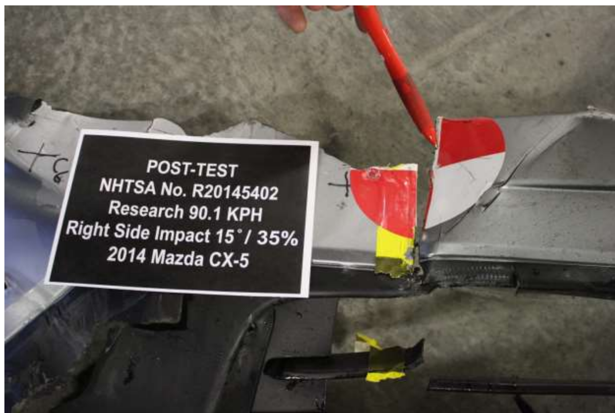
No. 026 Post-Test Close-up View of Impact Point
