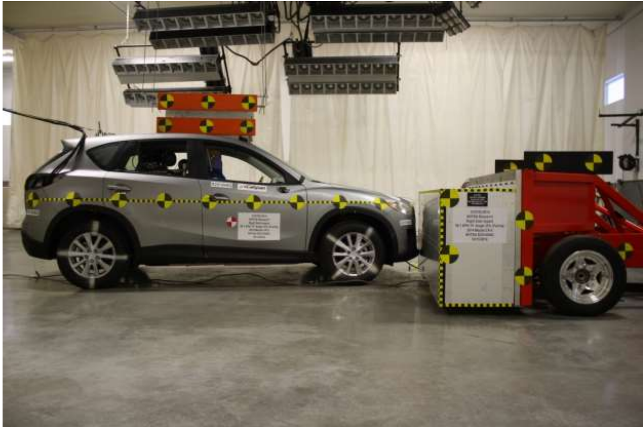
No. 172 Pre-Test RMDB & Vehicle, Left Side
