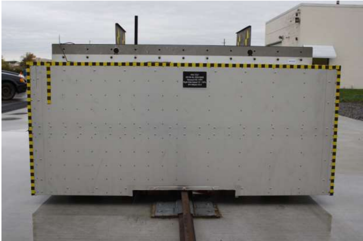
No. 168 Pre-Test Front View of RMDB
