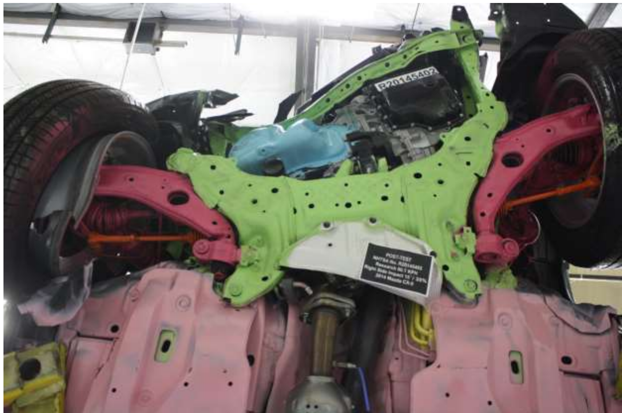
No. 139 Post-Test View of Front Sub-Frame Deformation
