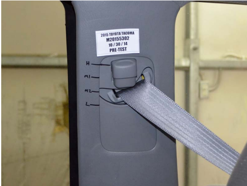
FIGURE 33. Pre-Test View of Belt Anchorage for Dummy
