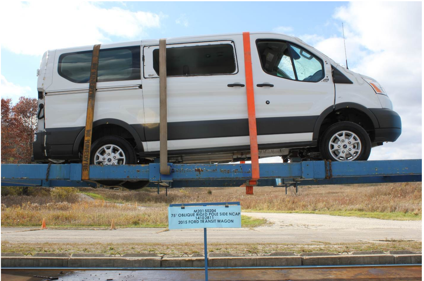
FMVSS No. 301 Static Rollover 0 Degrees
