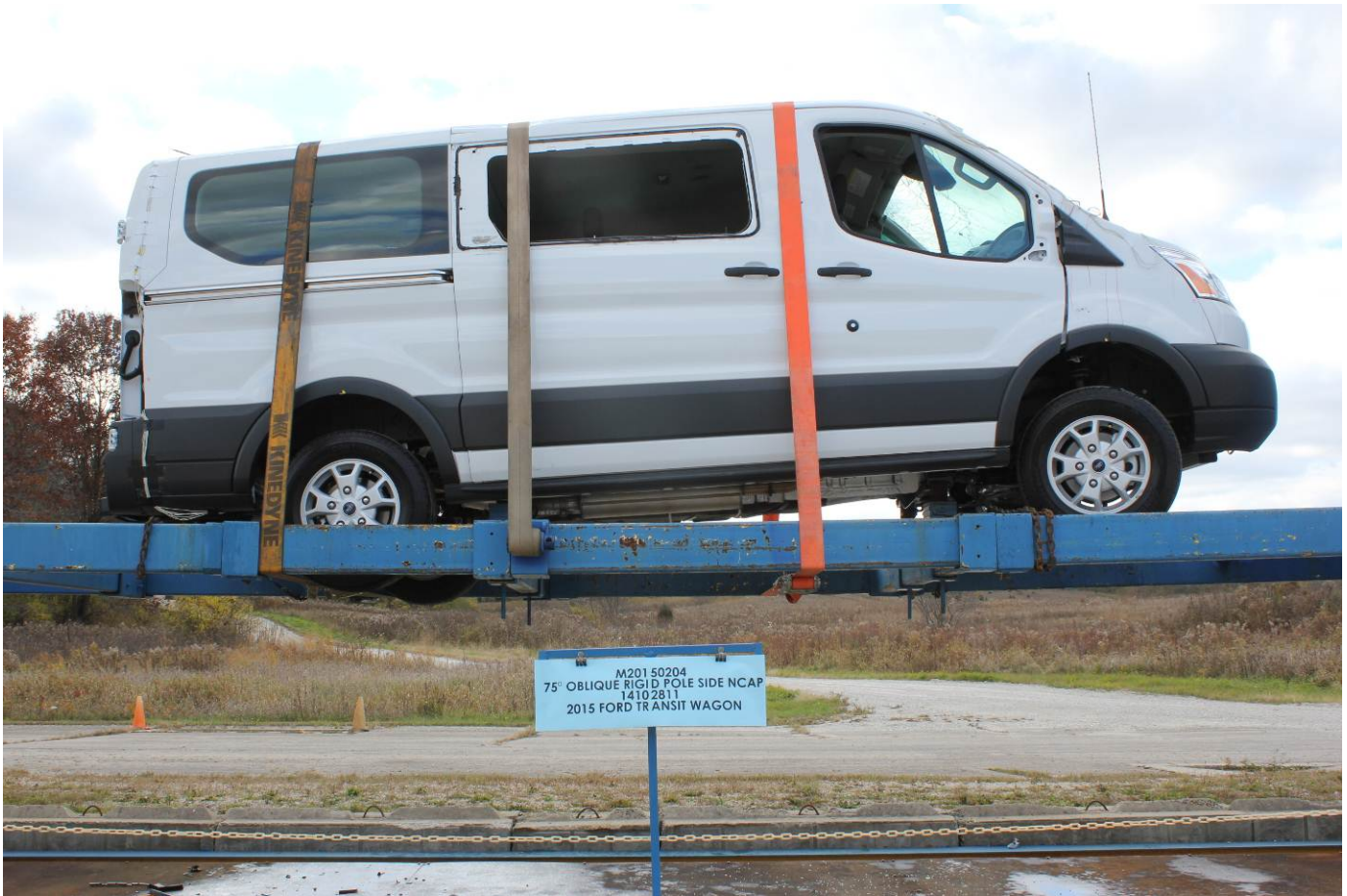
FMVSS No. 301 Static Rollover 360 Degrees
