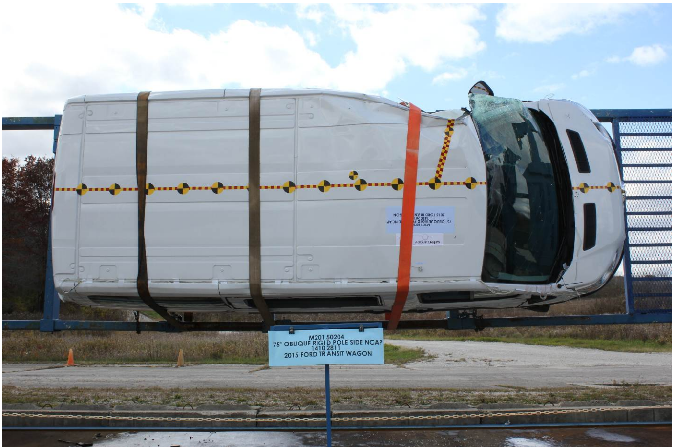
FMVSS No. 301 Static Rollover 270 Degrees
