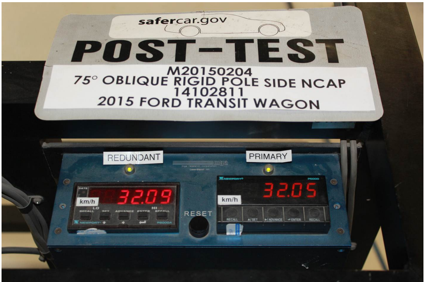
Post-Test Primary and Redundant Speed Trap Read-Out
