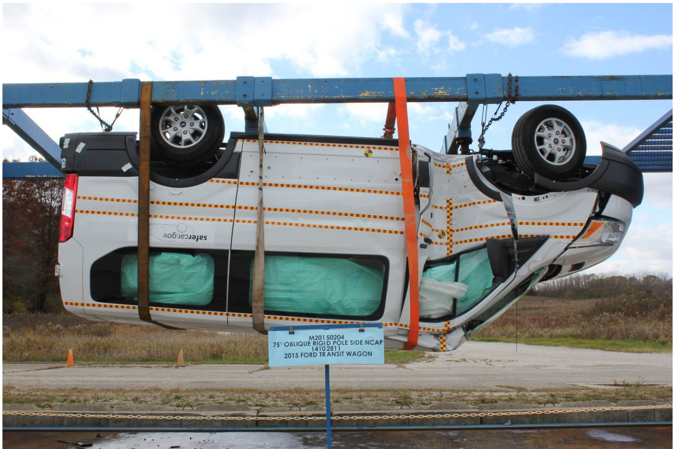
FMVSS No. 301 Static Rollover 180 Degrees
