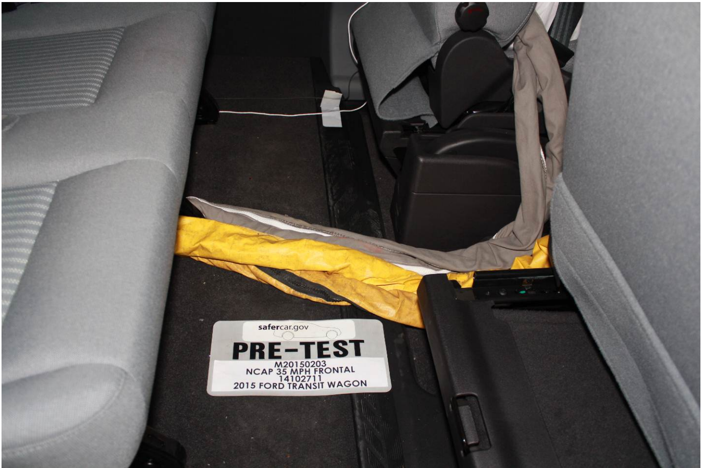
Pre-Test Dummy Cable Routing
