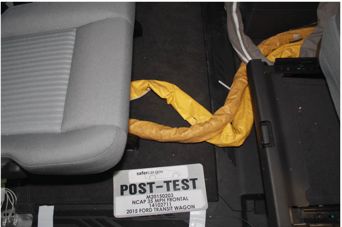
Post-Test Dummy Cable Routing
