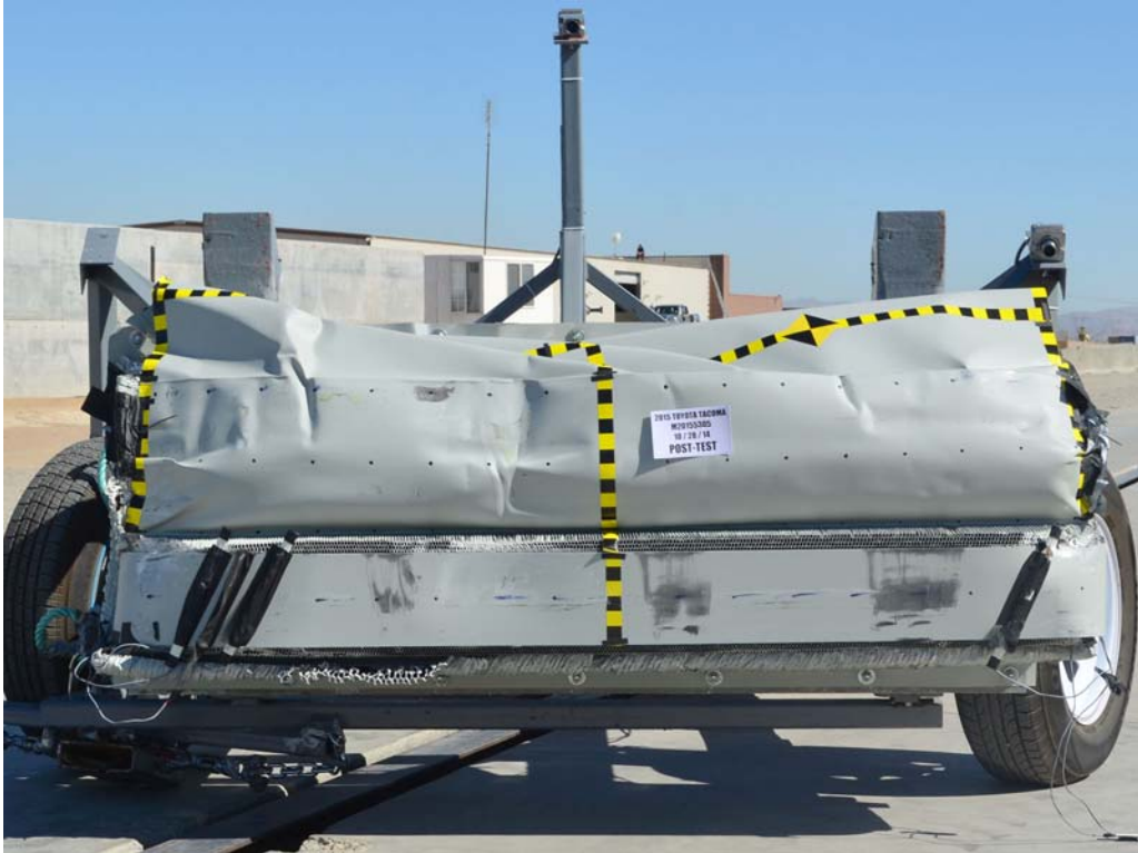
FIGURE 85. Post-Test Front View of MDB Impactor Face
