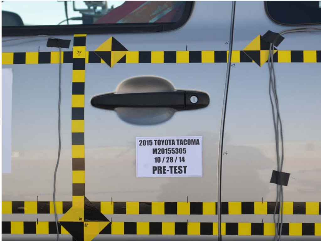
FIGURE 21. Pre-Test Left Front Door Latch Close-Up
