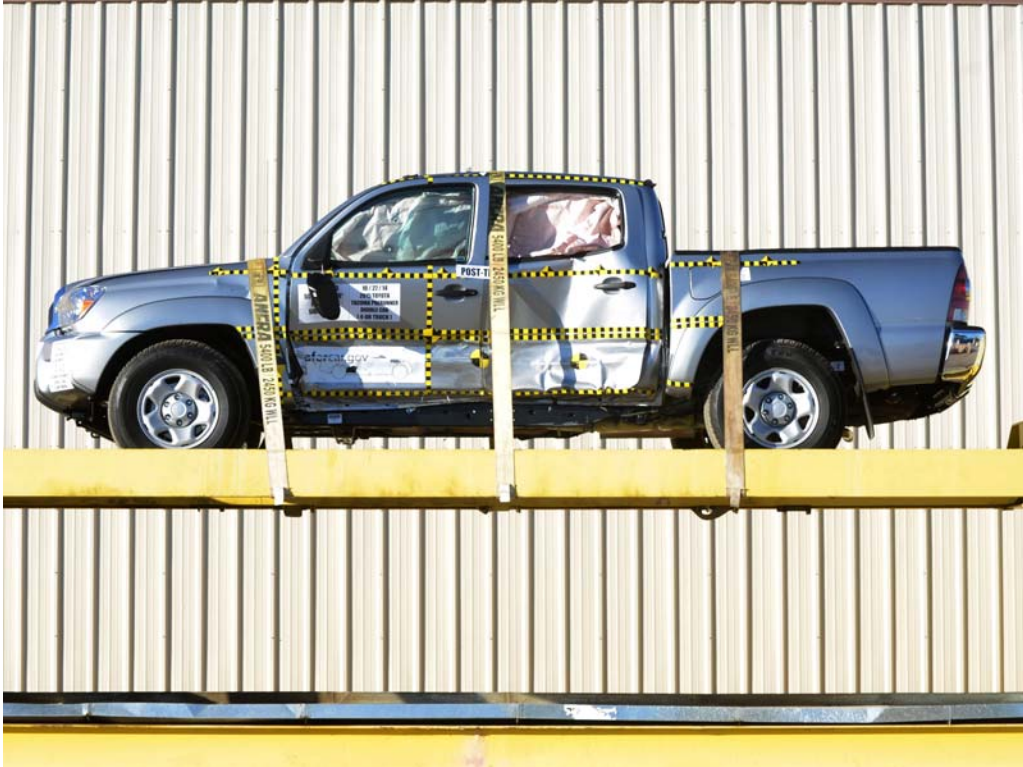
FIGURE 96. FMVSS No. 301 Static Rollover 0 Degrees
