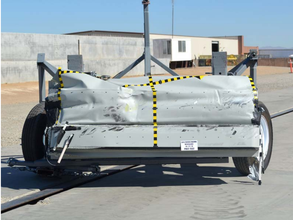
FIGURE 85. Post-Test Front View of MDB Impactor Face
