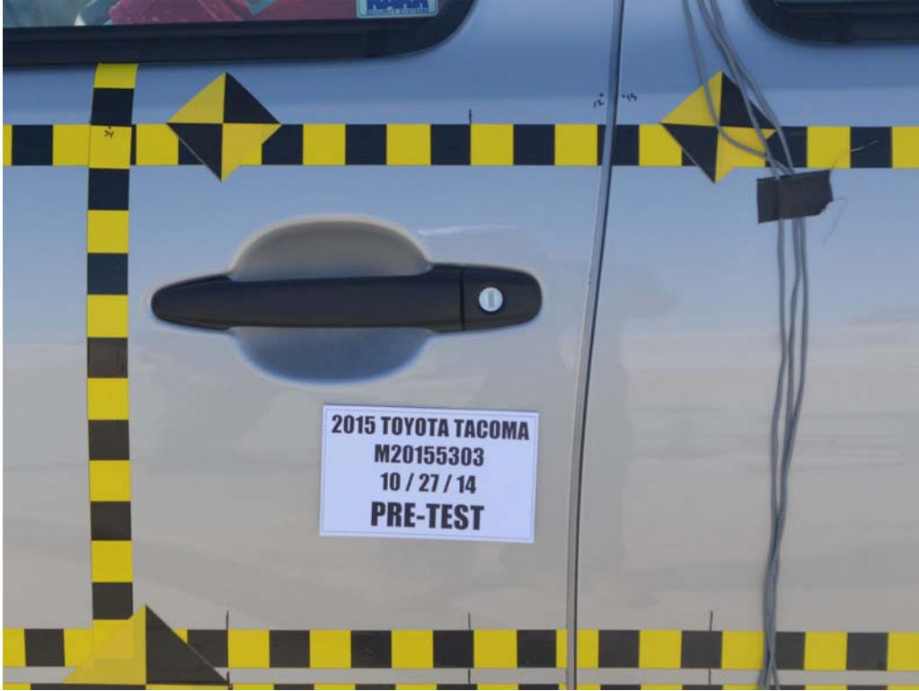
FIGURE 21. Pre-Test Left Front Door Latch Close-Up
