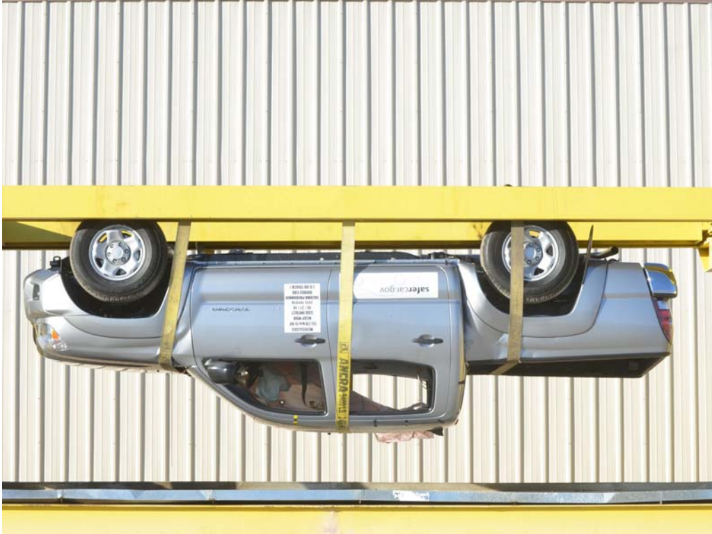
FIGURE 98. FMVSS No. 301 Static Rollover 180 Degrees
