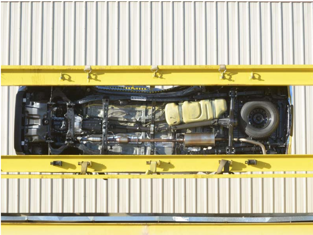
FIGURE 99. FMVSS No. 301 Static Rollover 270 Degrees
