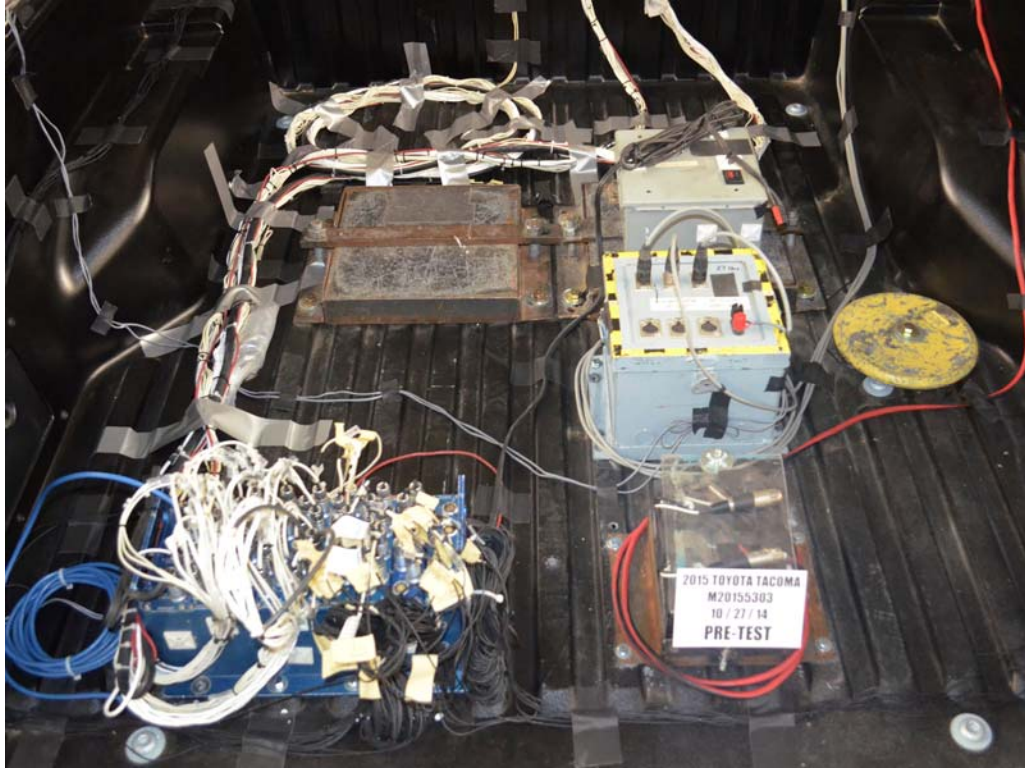
FIGURE 94. Pre-Test Ballast View
