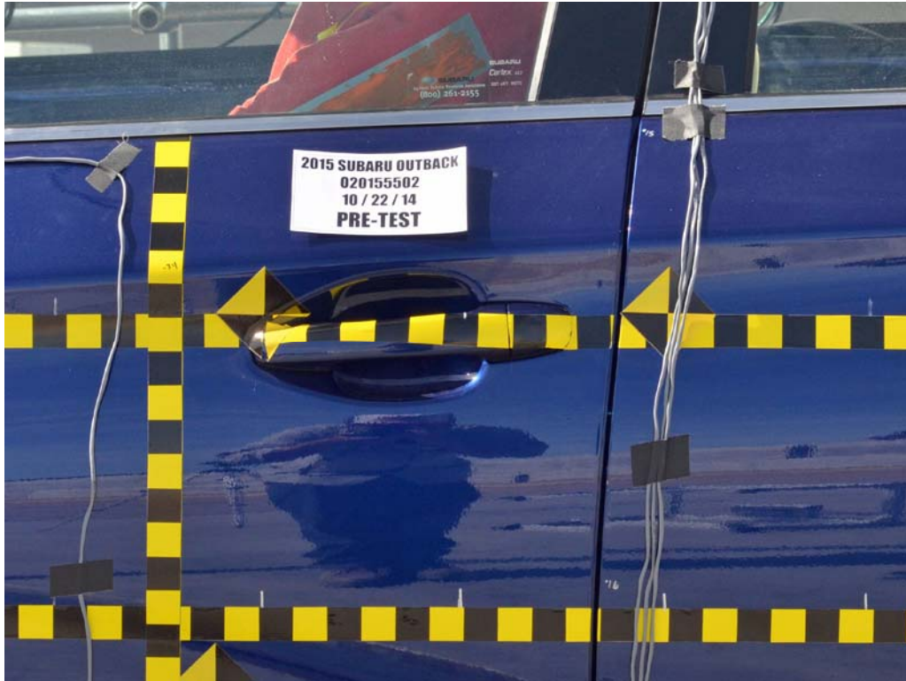
FIGURE 21. Pre-Test Left Front Door Latch Close-Up
