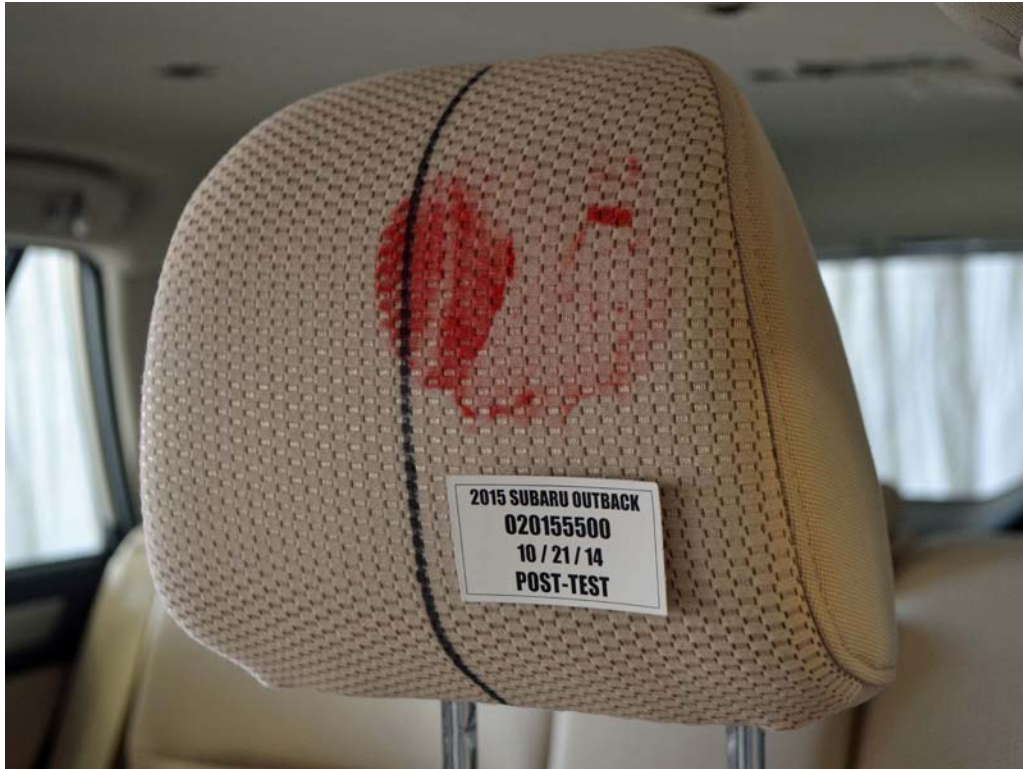
FIGURE 47. Post-Test Driver Dummy Contact with Headrest
