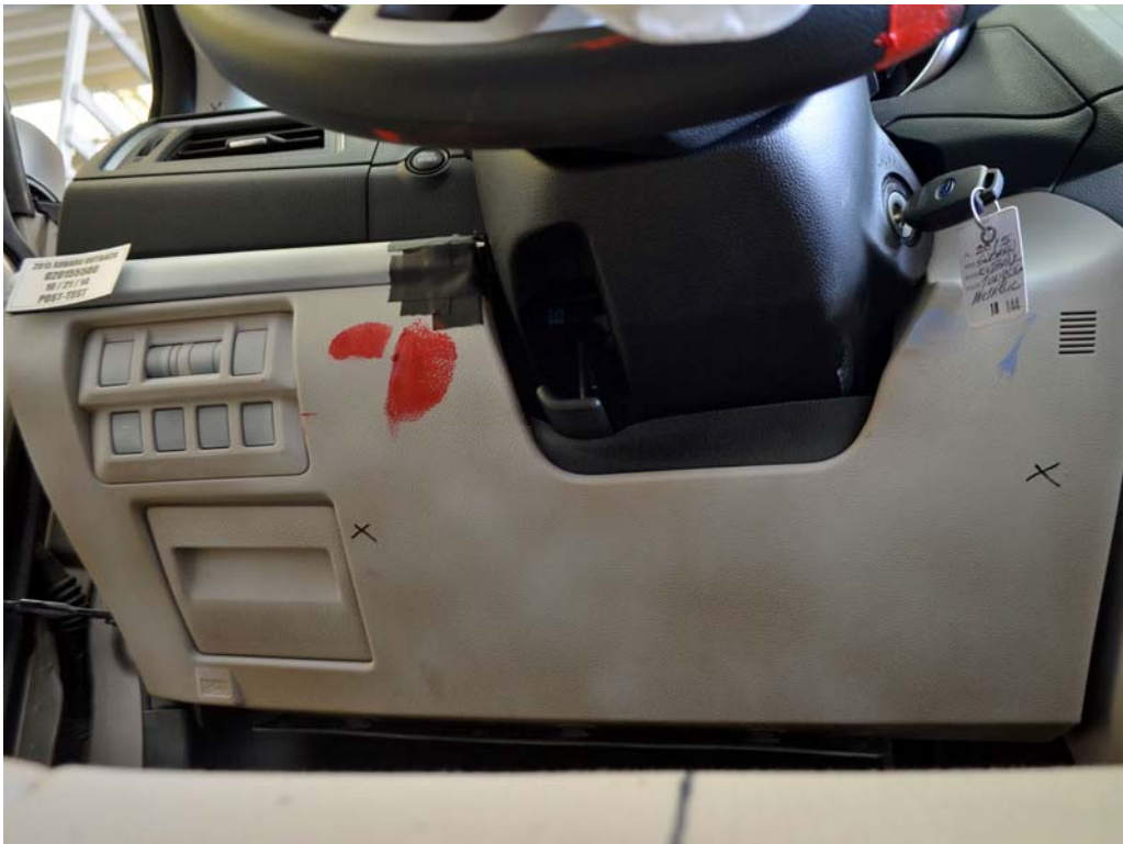
FIGURE 42. Post-Test Driver's Side Knee Bolster
