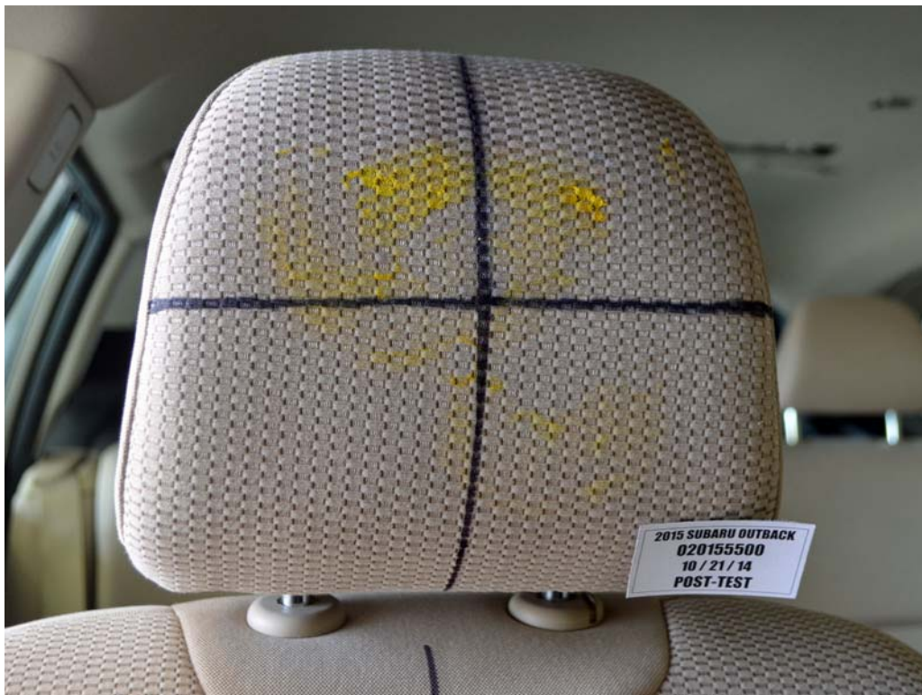
FIGURE 68. Post-Test Passenger Dummy Contact with Headrest
