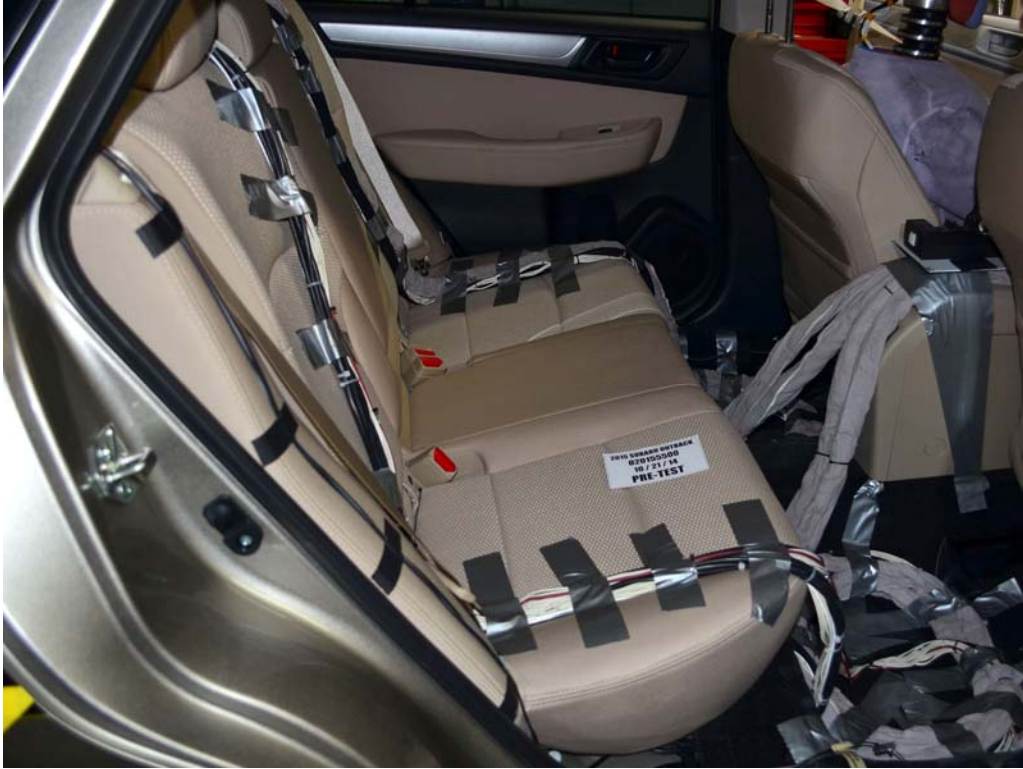
FIGURE 27. Pre-Test Dummy Cable Routing
