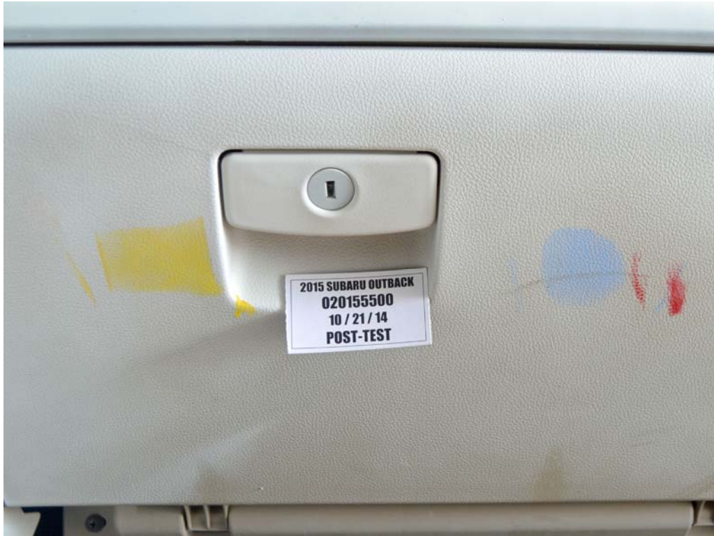
FIGURE 68a. Post-Test Passenger Dummy Contact with Glovebox
