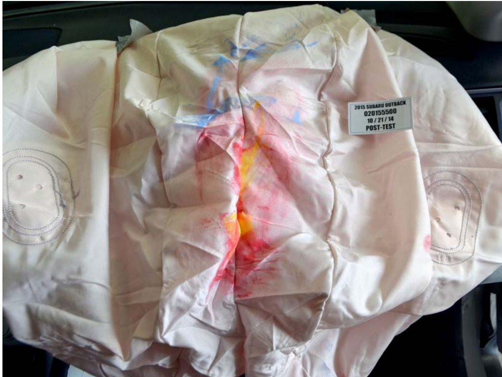
FIGURE 67. Post-Test Passenger Dummy Contact with Airbag
