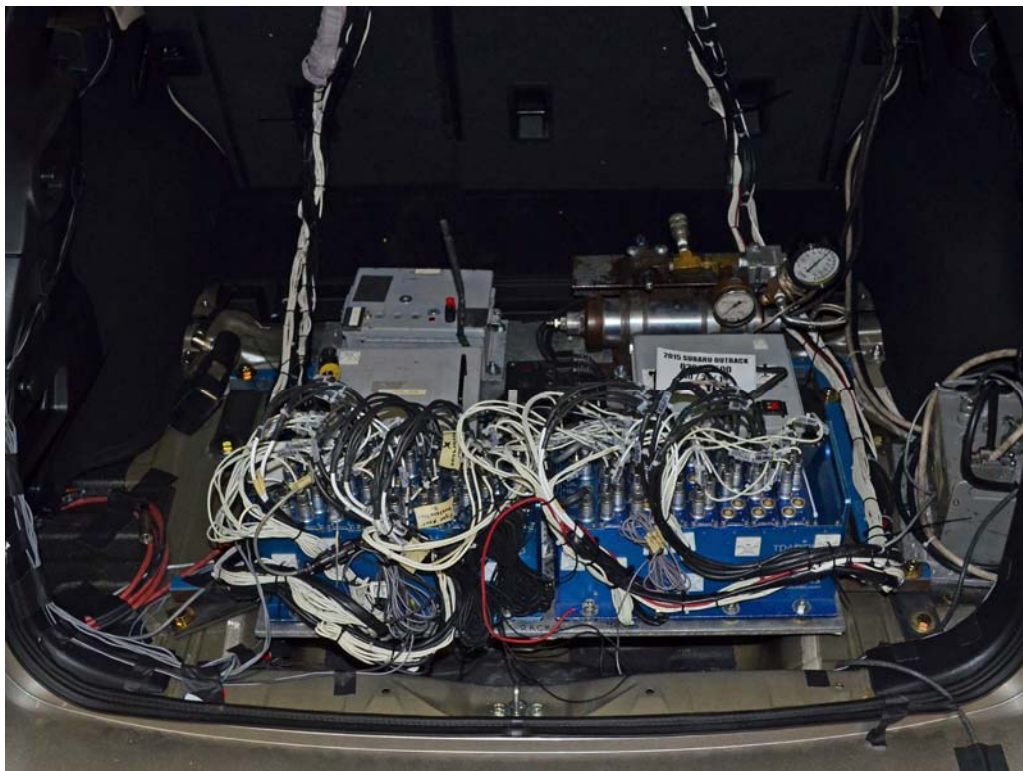
FIGURE 69. Photograph of Ballast Installed in Vehicle
