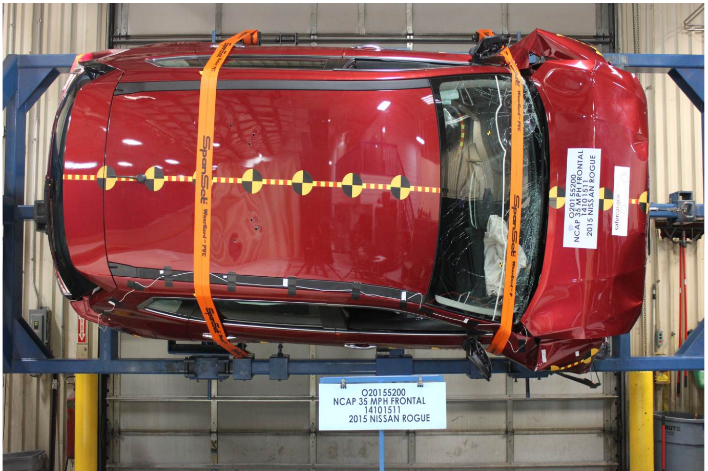
Vehicle at 90 Degrees on Static Rollover Device
