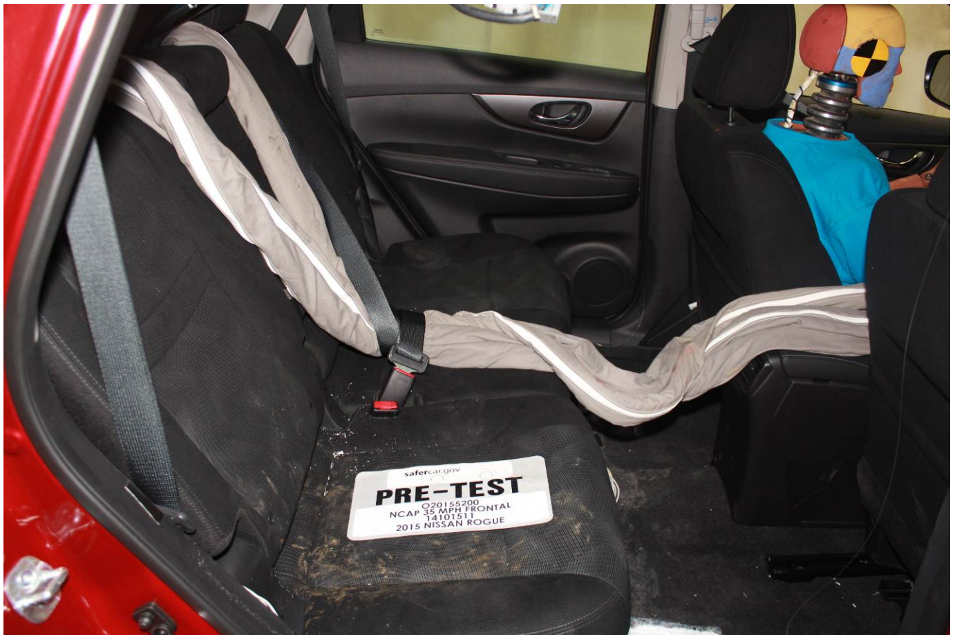
Pre-Test Dummy Cable Routing
