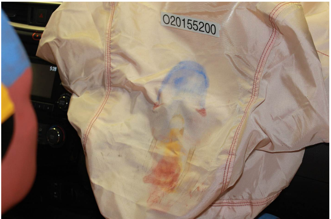
Post-Test Passenger Dummy Contact with Airbag
