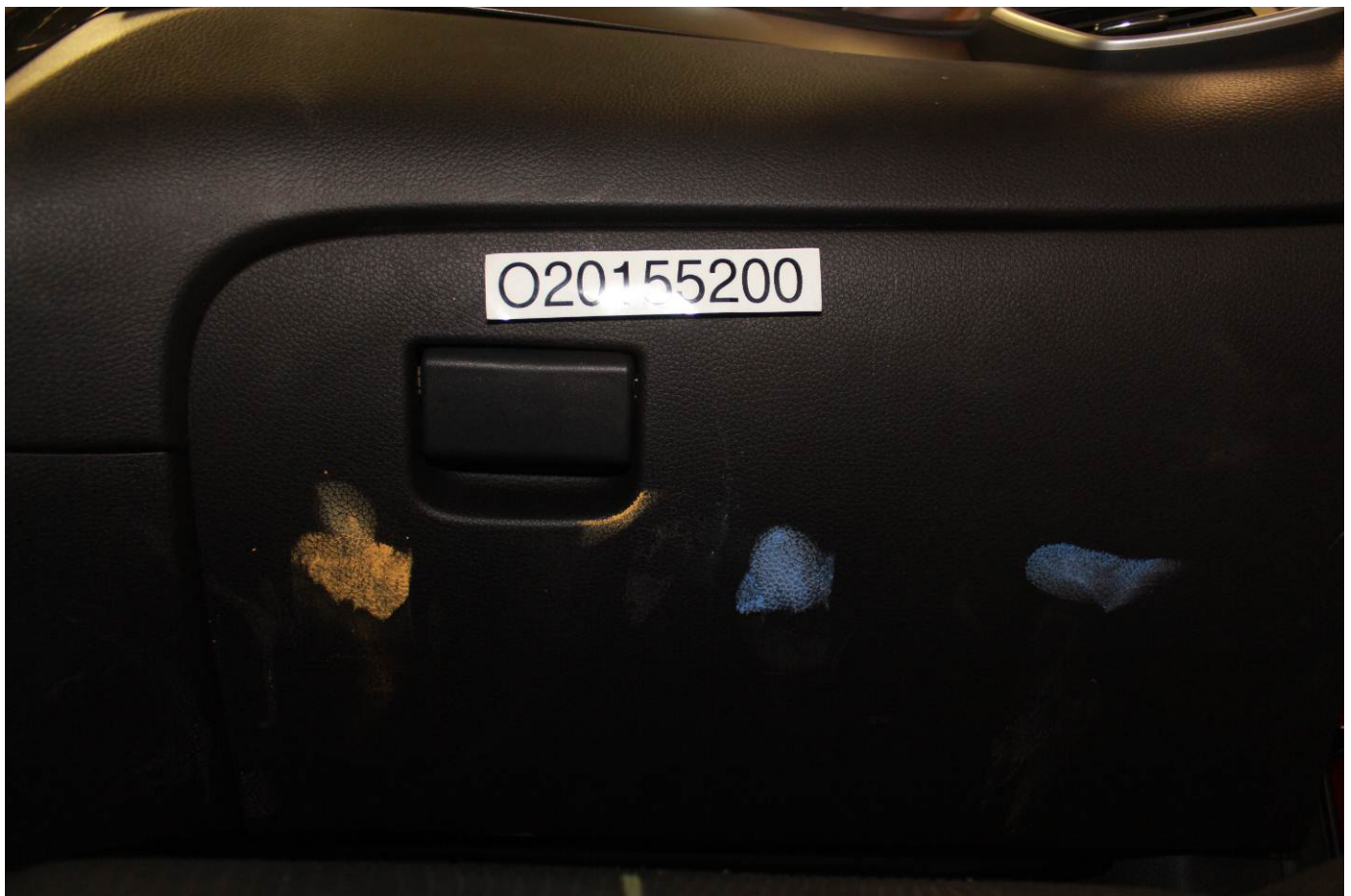
Post-Test Passenger Dummy Contact with Glovebox
