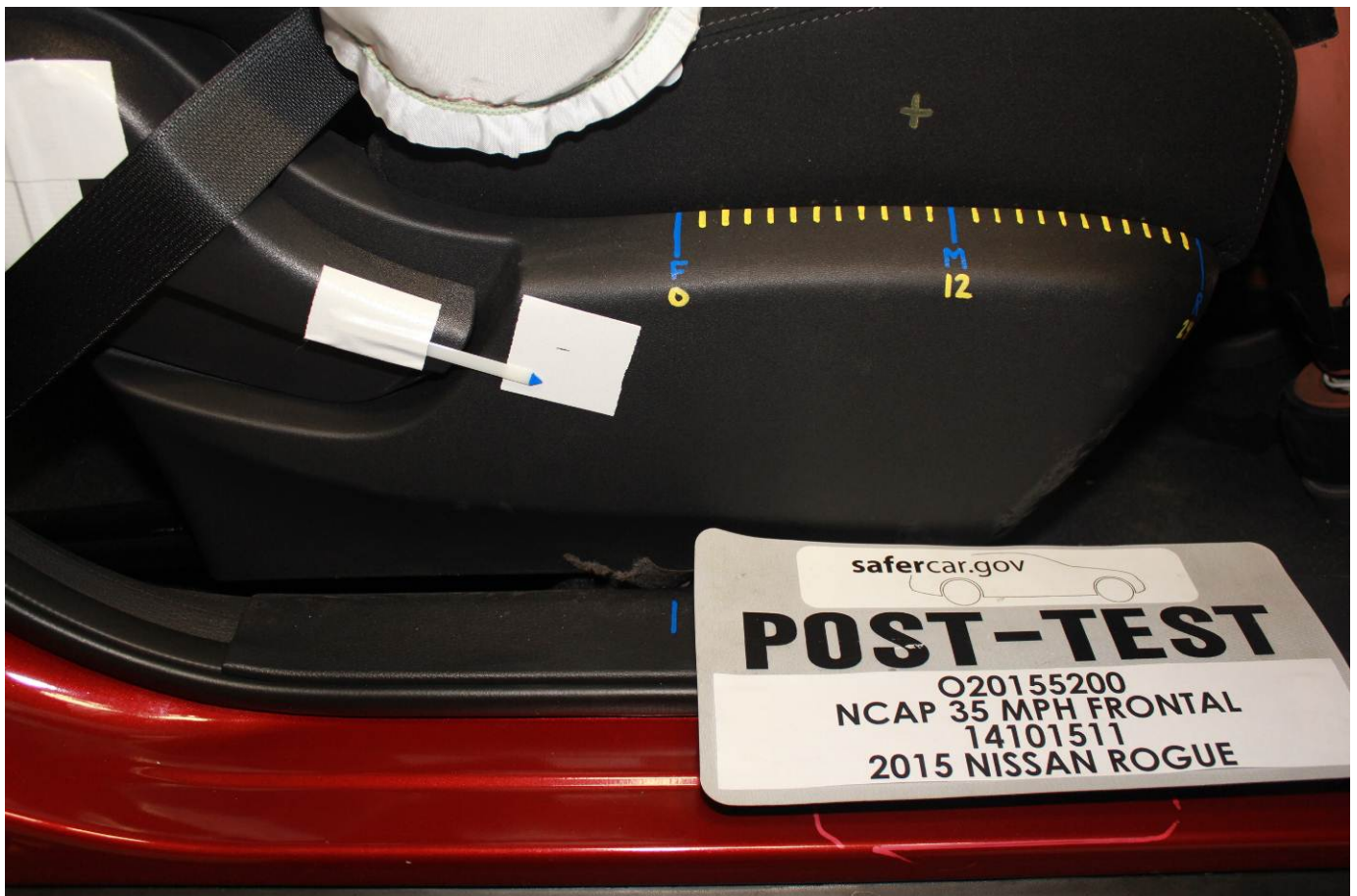
Post-Test Passenger's Seat Fore-Aft Markings
