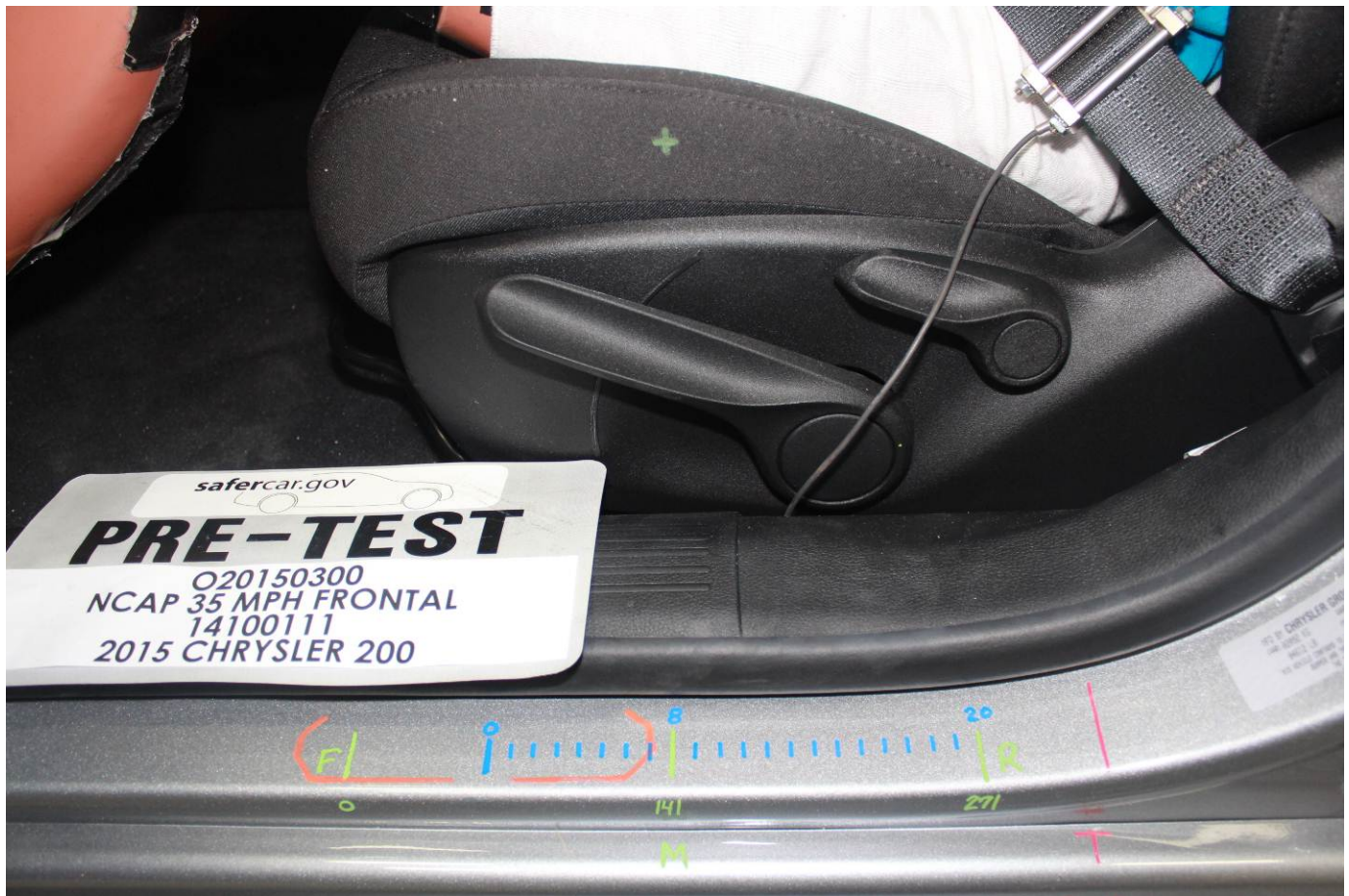
Pre-Test Driver's Seat Fore-Aft Markings
