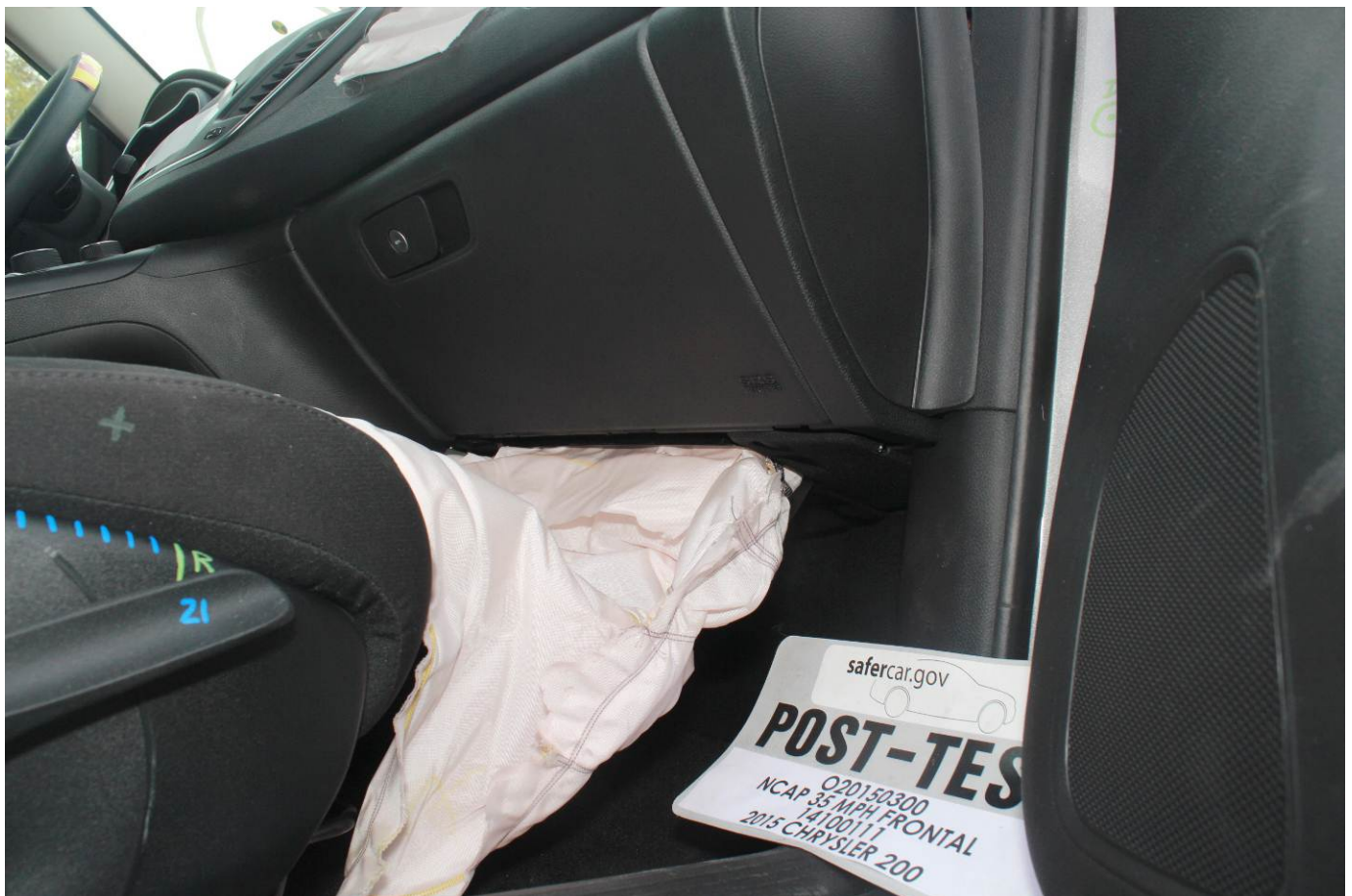
Post-Test Passenger's Side Knee Bolster (without dummy)
