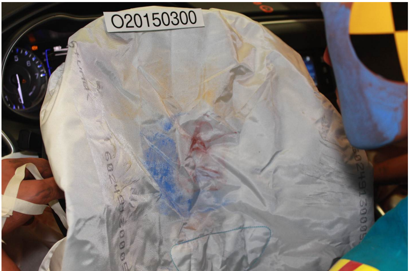
Post-Test Driver Dummy Contact with Airbag
