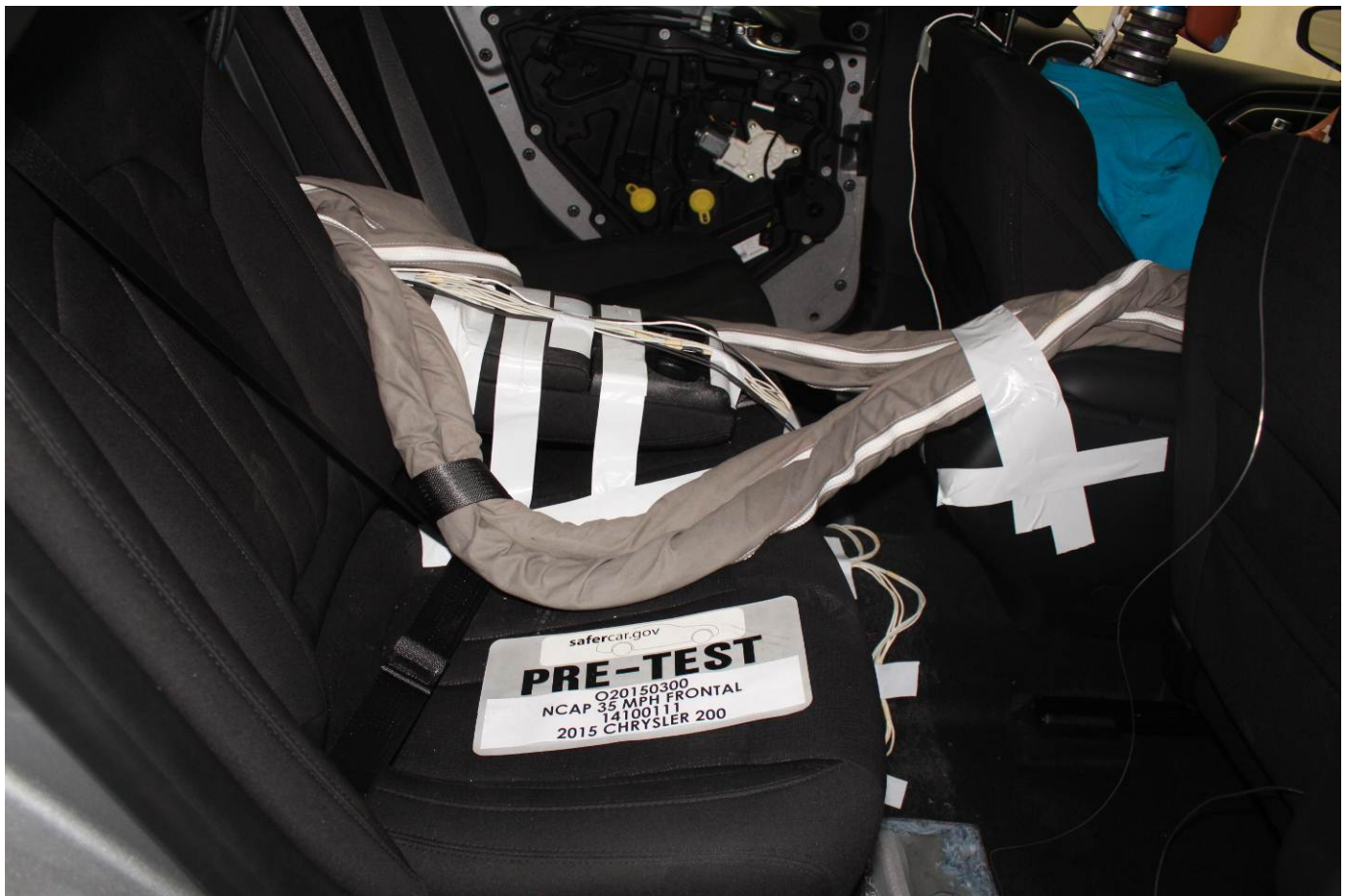
Pre-Test Dummy Cable Routing
