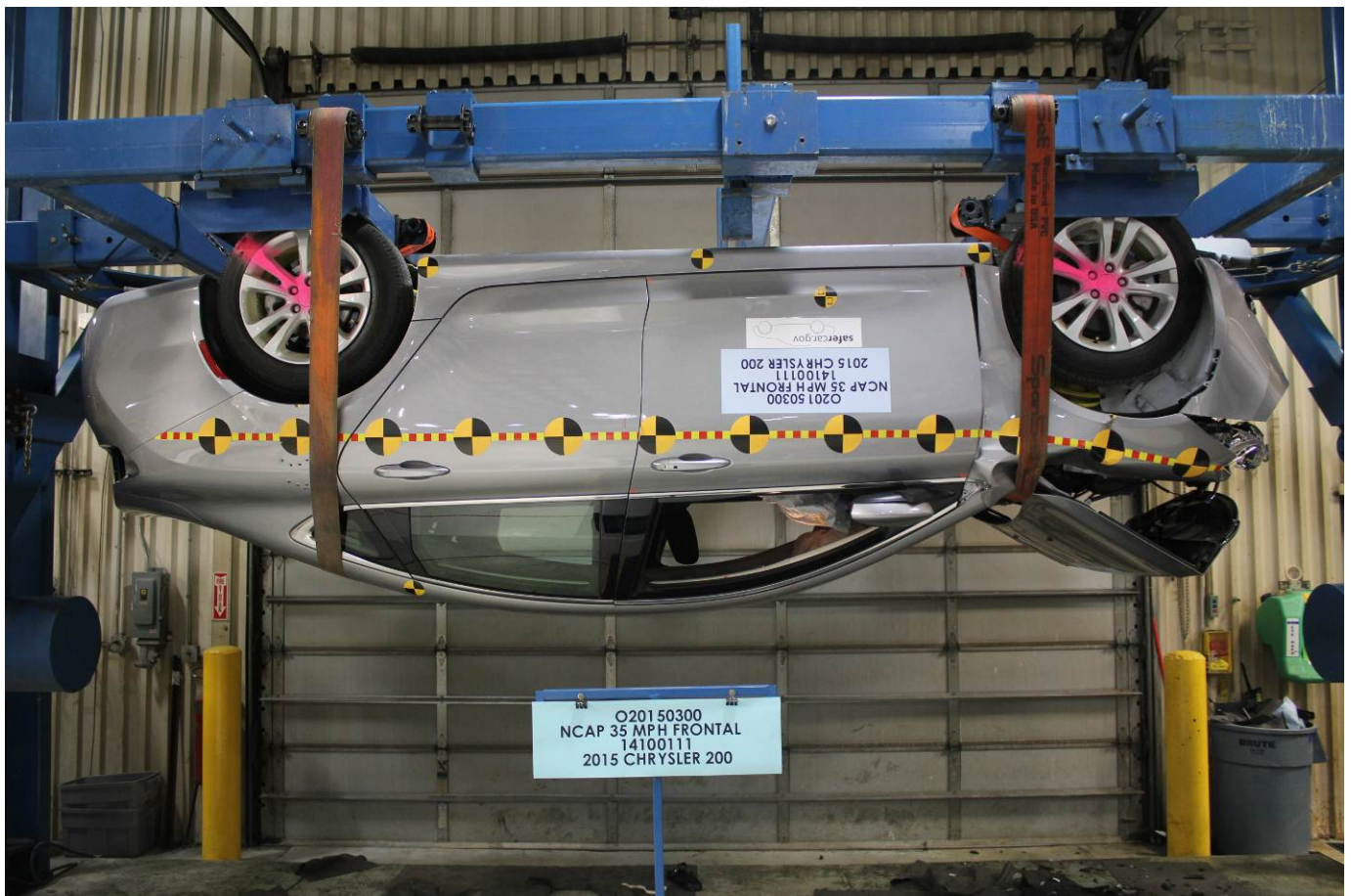
Vehicle at 180 Degrees on Static Rollover Device
