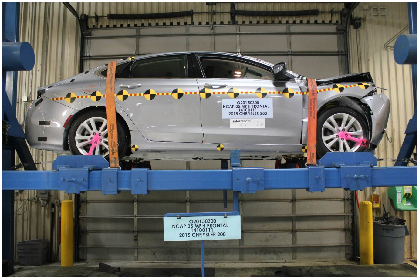
Vehicle at 0 Degree on Static Rollover Device
