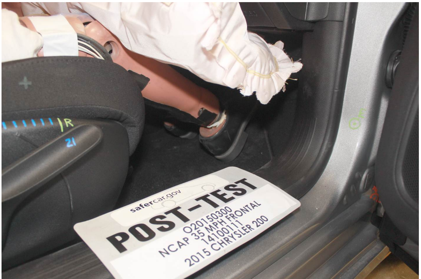
Post-Test Passenger Dummy Feet
