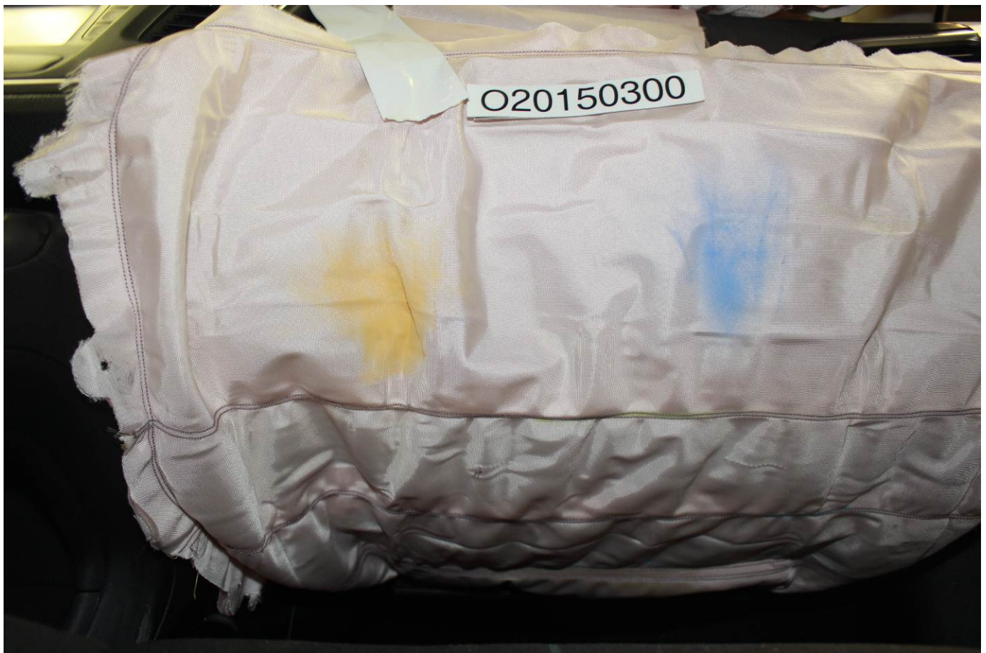
Post-Test Passenger Dummy Contact with Knee Airbag
