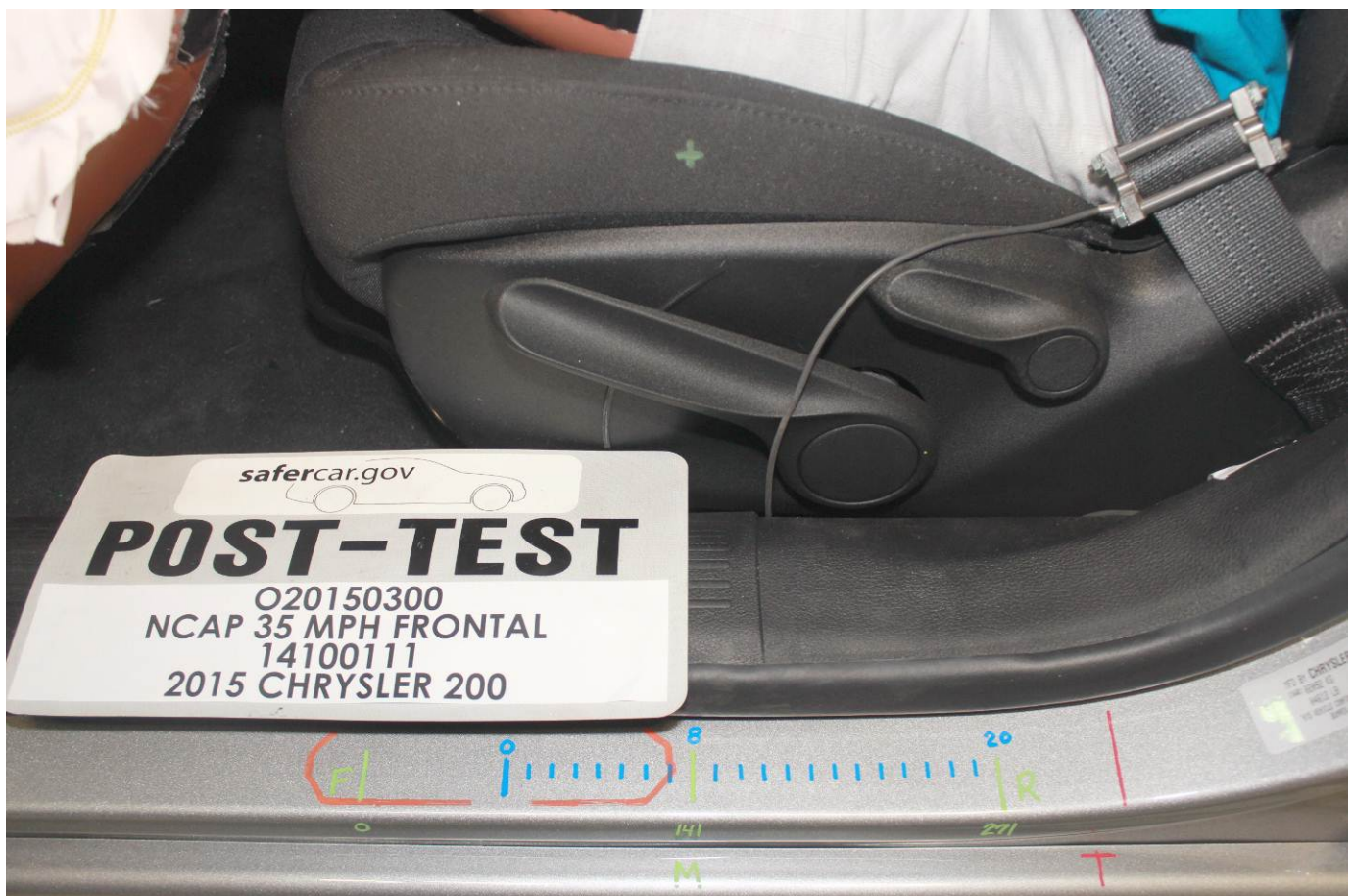
Post-Test Driver's Seat Fore-Aft Markings
