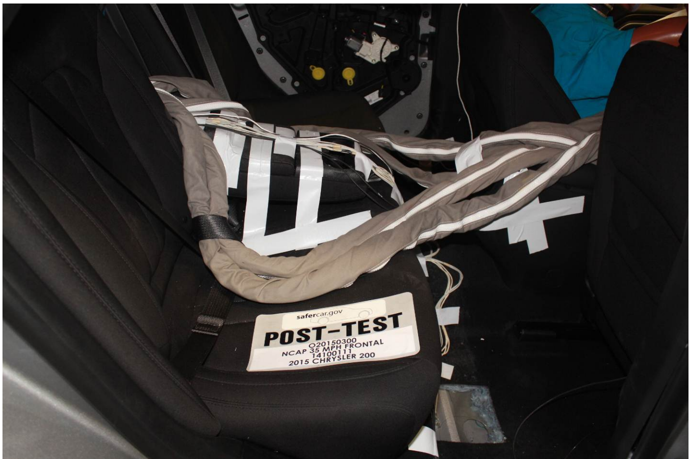
Post-Test Dummy Cable Routing
