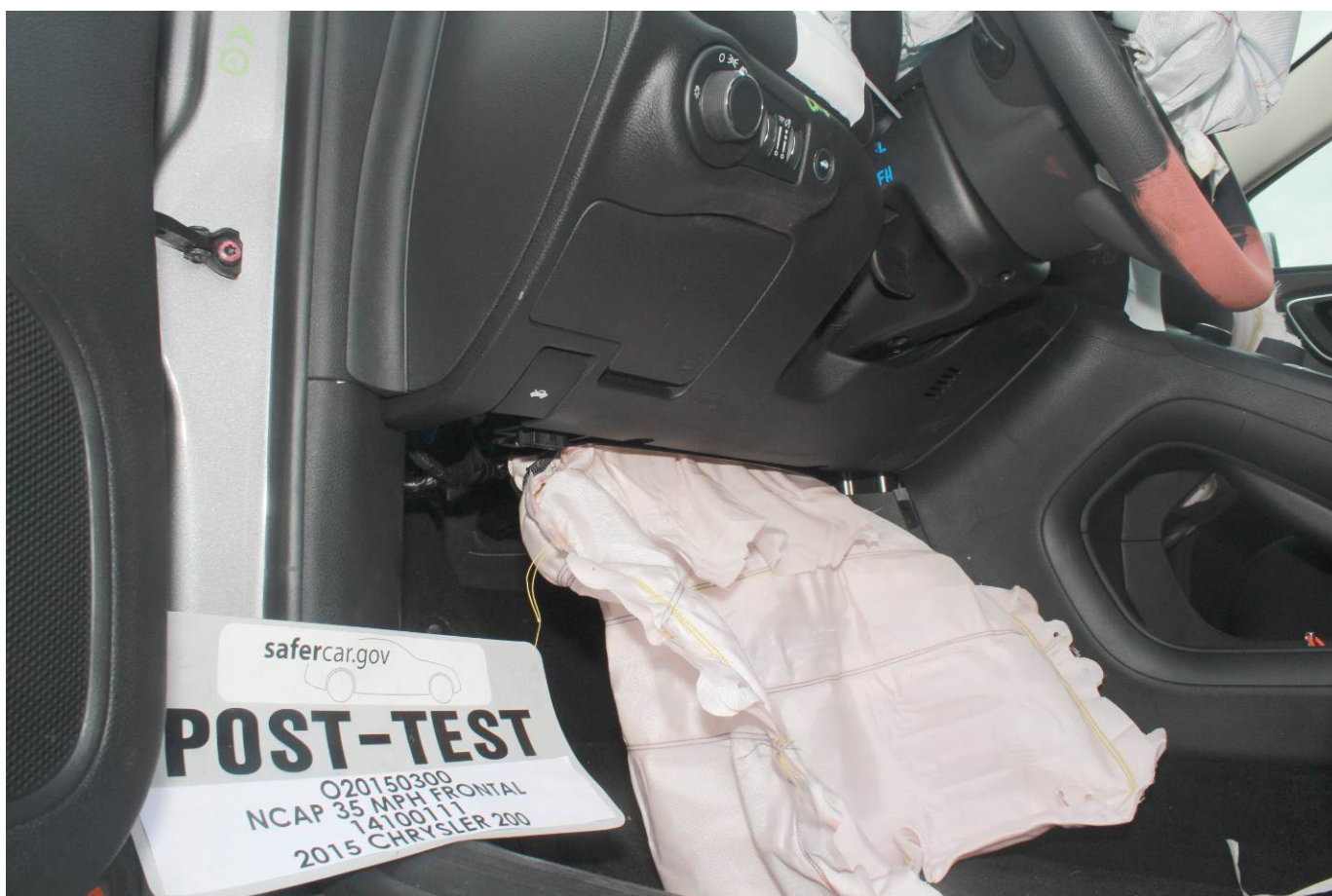
Post-Test Driver's Side Knee Bolster (without dummy)
