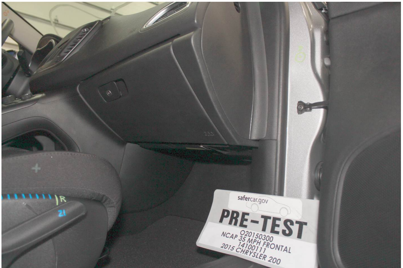
Pre-Test Passenger's Side Knee Bolster (without dummy)
