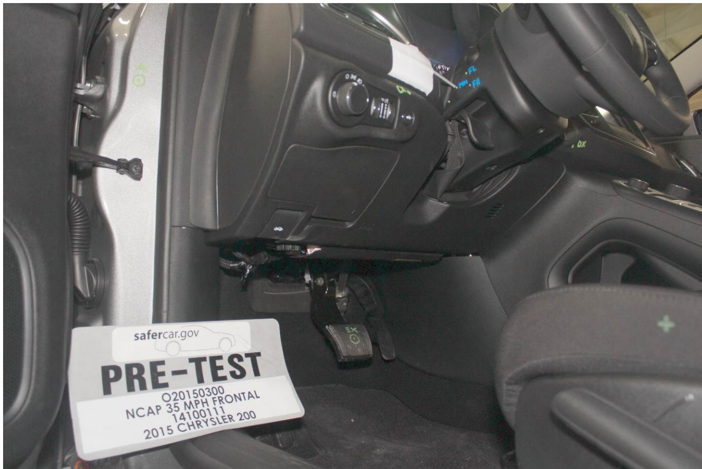
Pre-Test Driver's Side Knee Bolster (without dummy)
