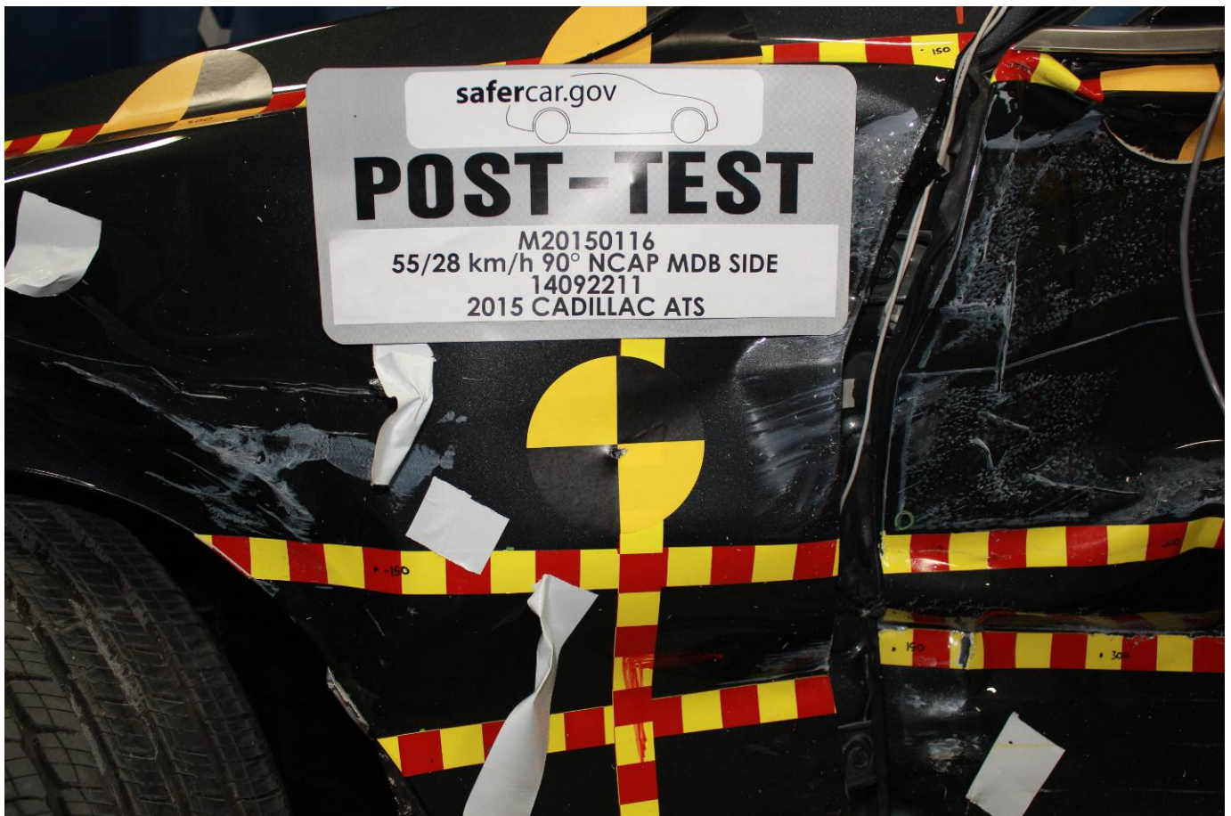
Post-Test Close-Up View of Impact Point Target
