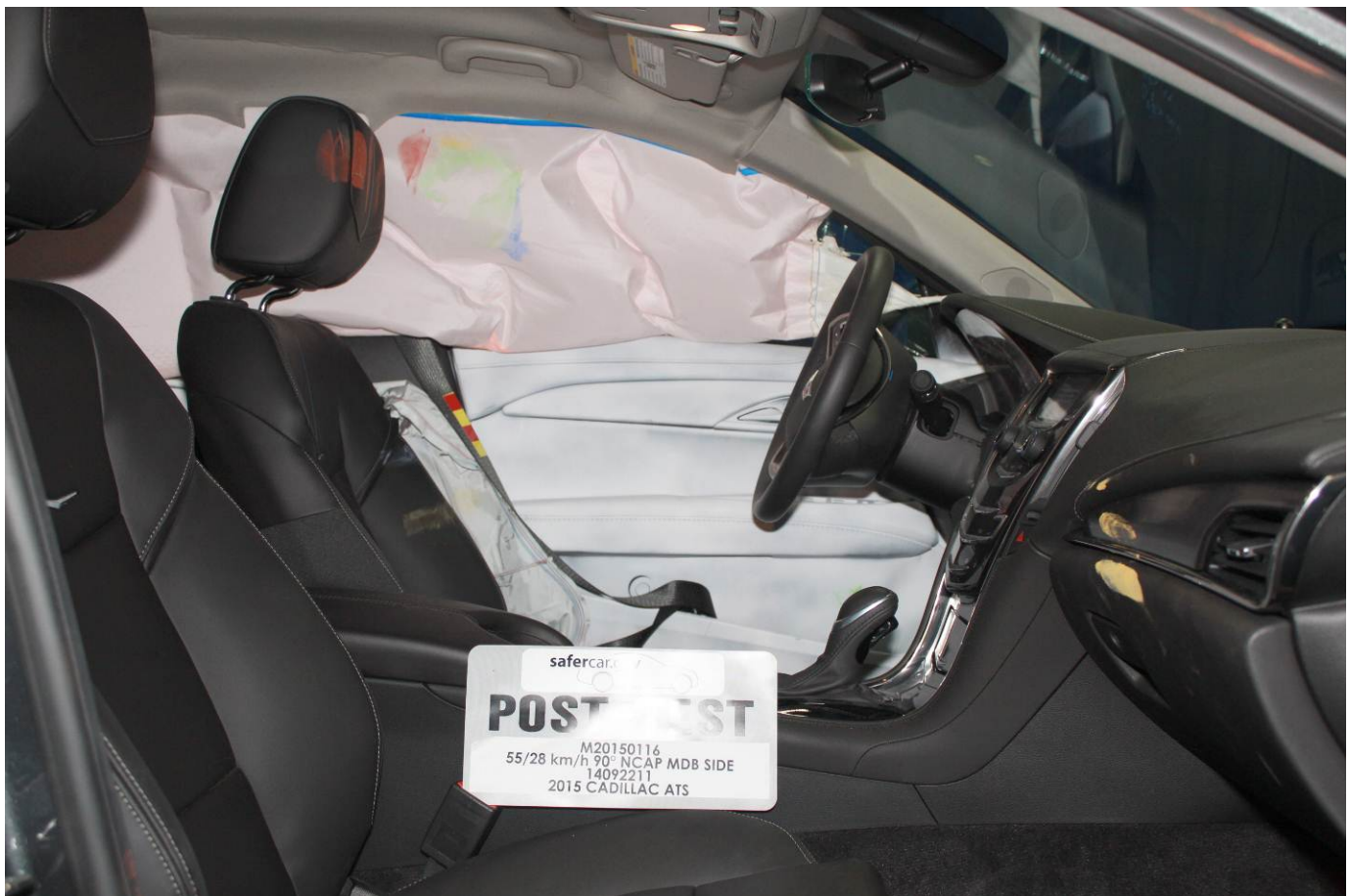
Post-Test Driver Inner Door Panel View
