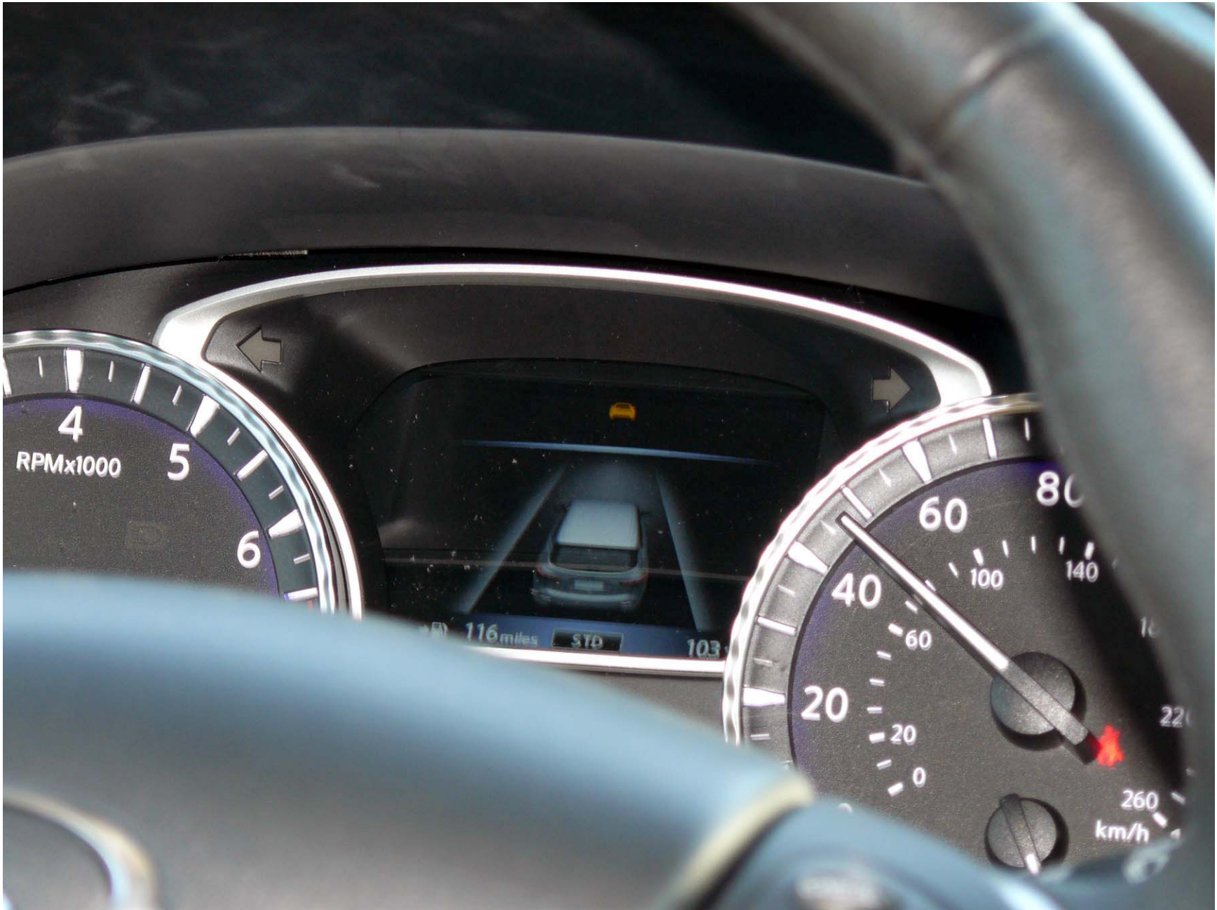
Figure A12. Display for Vehicle Ahead Detected
