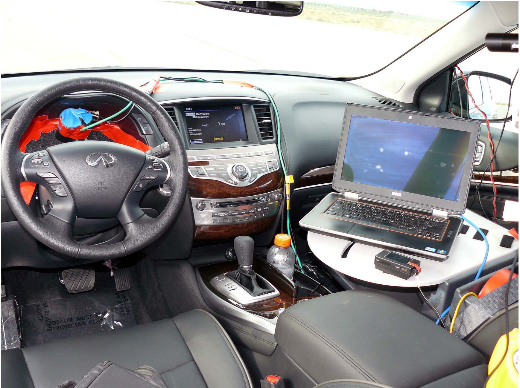
Figure A9. Computer Installed in Subject Vehicle
