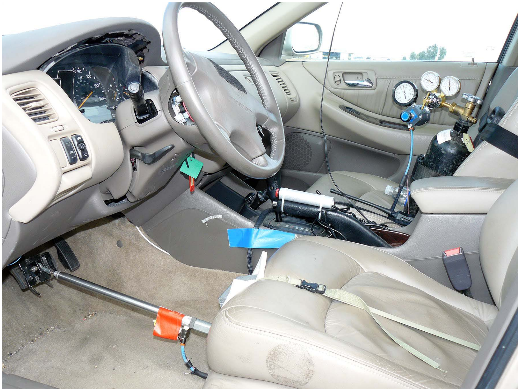
Figure A10. Brake Actuation System Installed in Principal Other Vehicle
