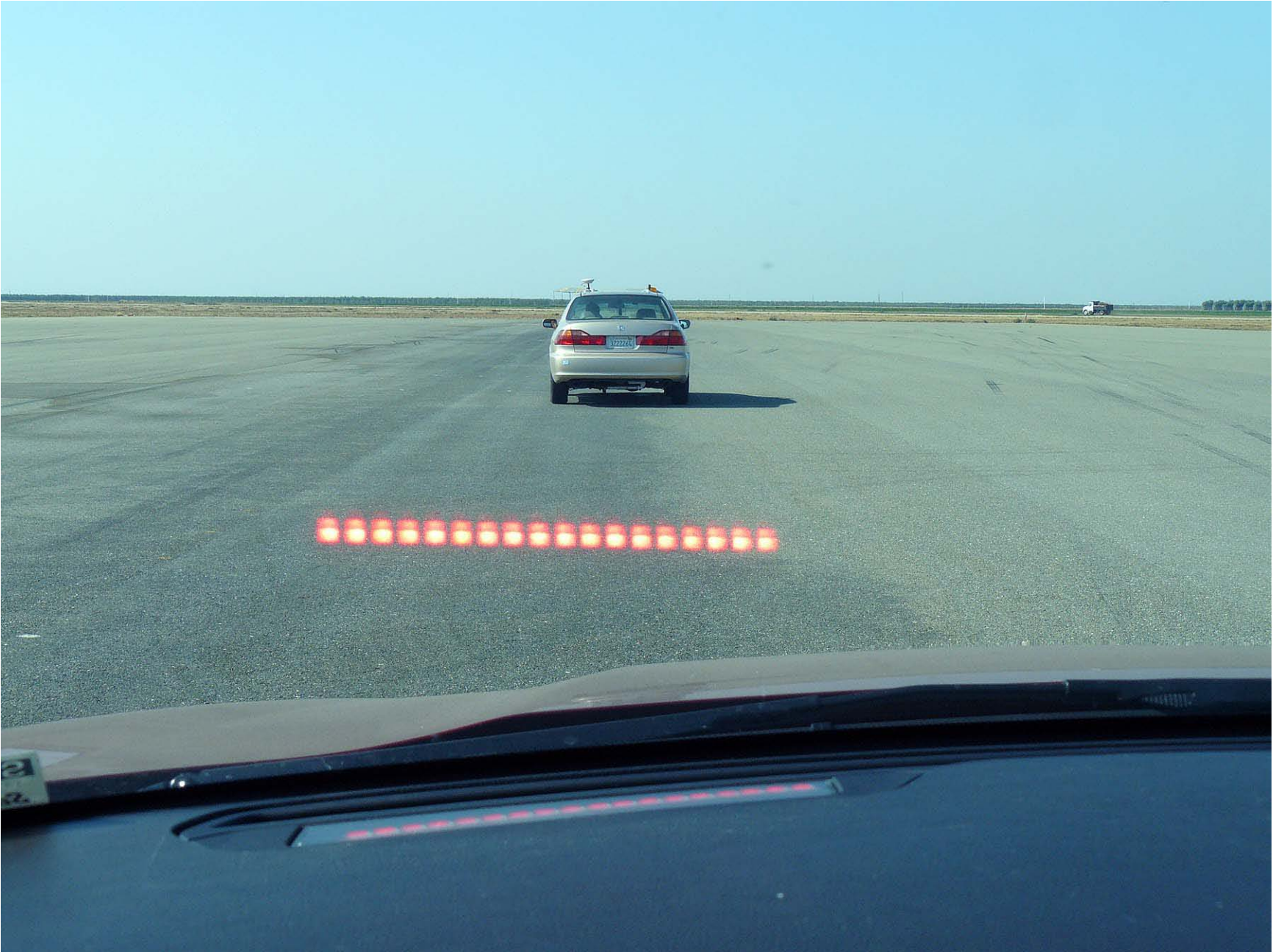
Figure A11. Forward Collision Visual Warning
