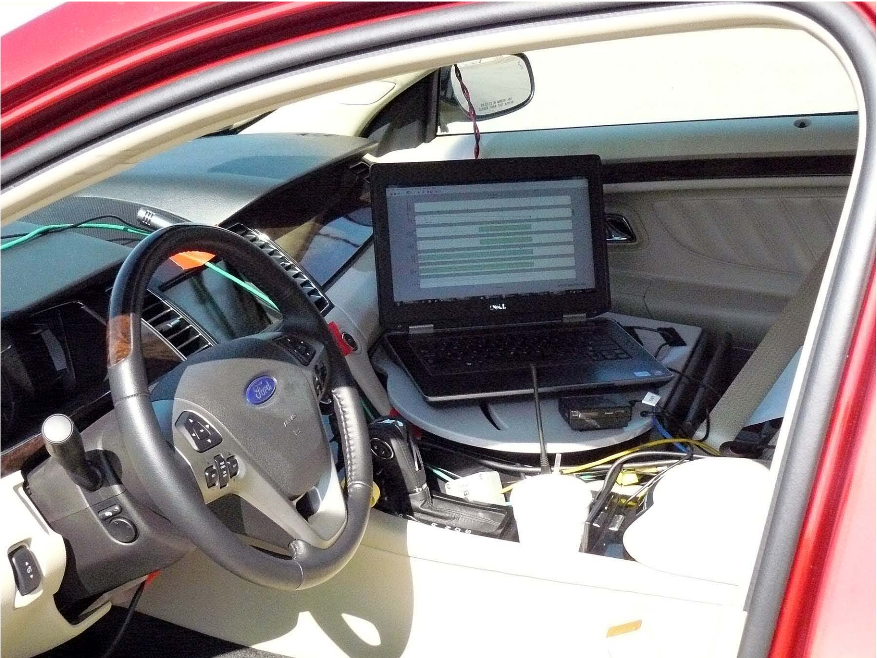
Figure A9. Computer Installed in Subject Vehicle
