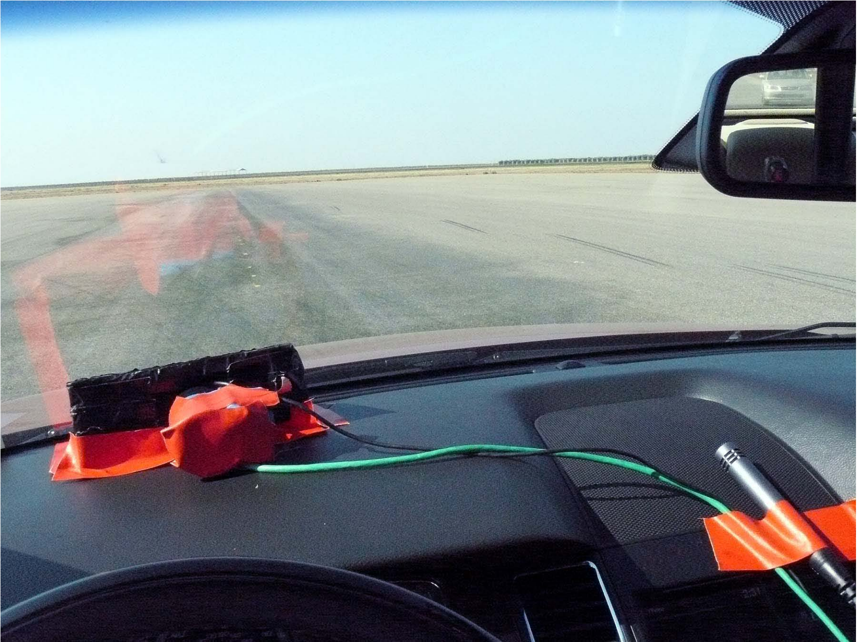
Figure A12. Sensors for Detecting Visual and Aural Warnings
