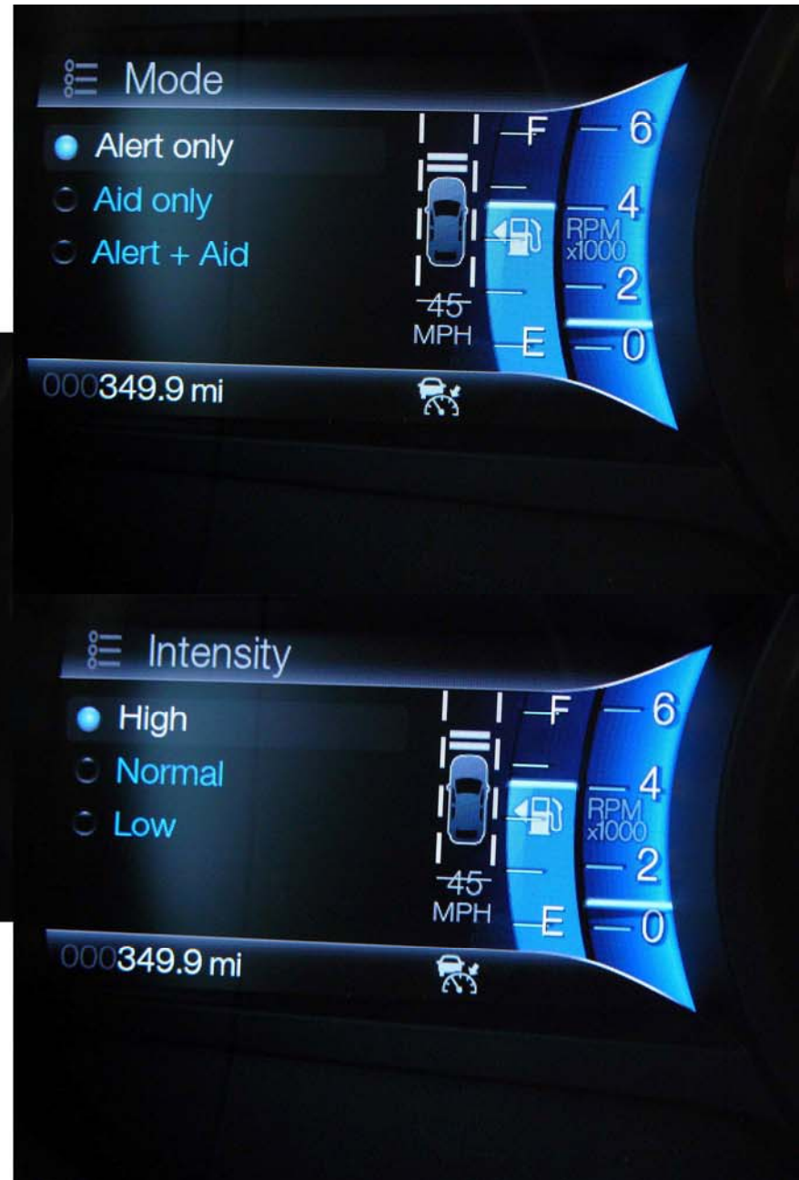
Figure A11. Adjustment of LDW Settings (cont.)
