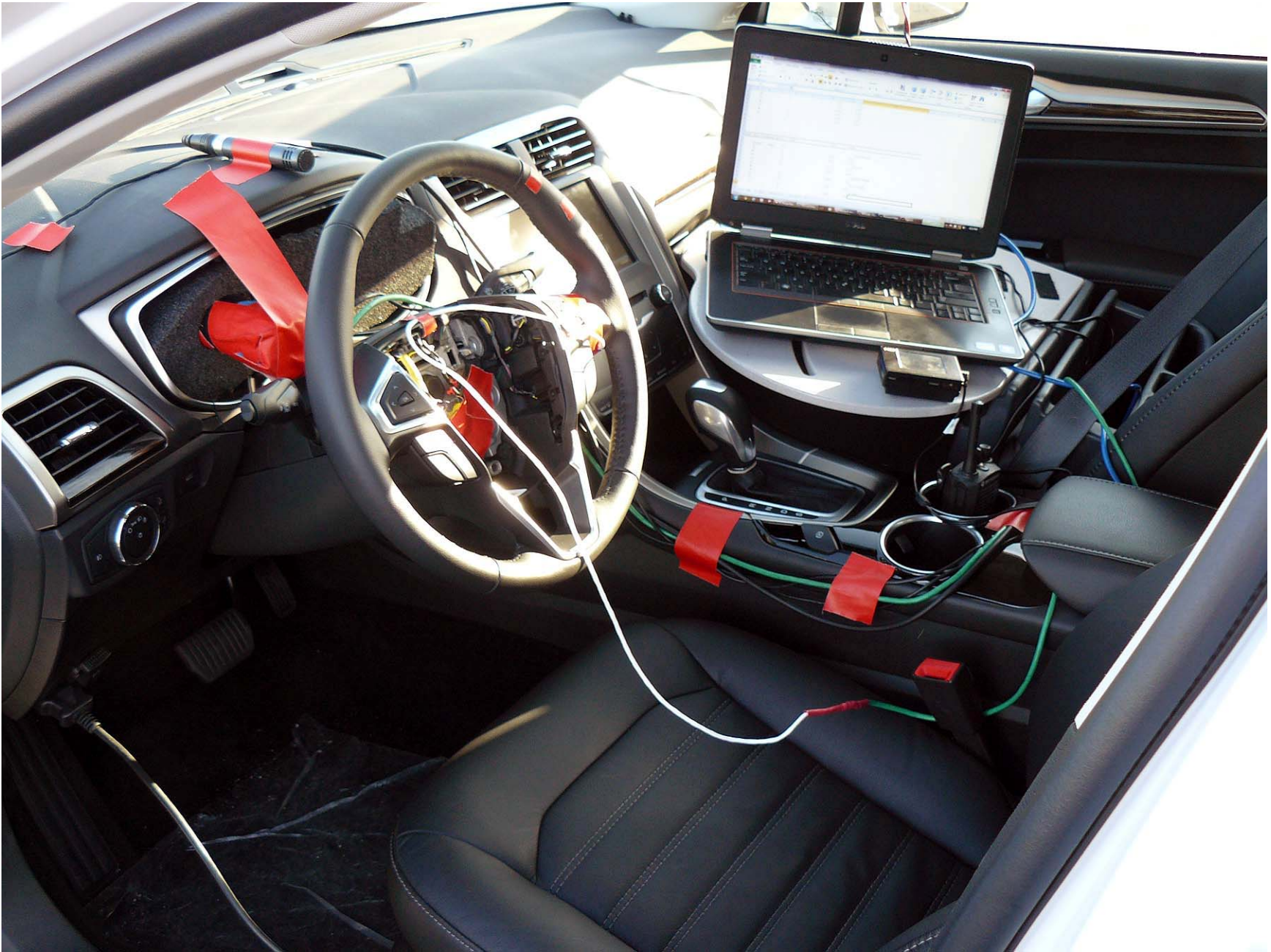
Figure A7. Computer Installed in Subject Vehicle
