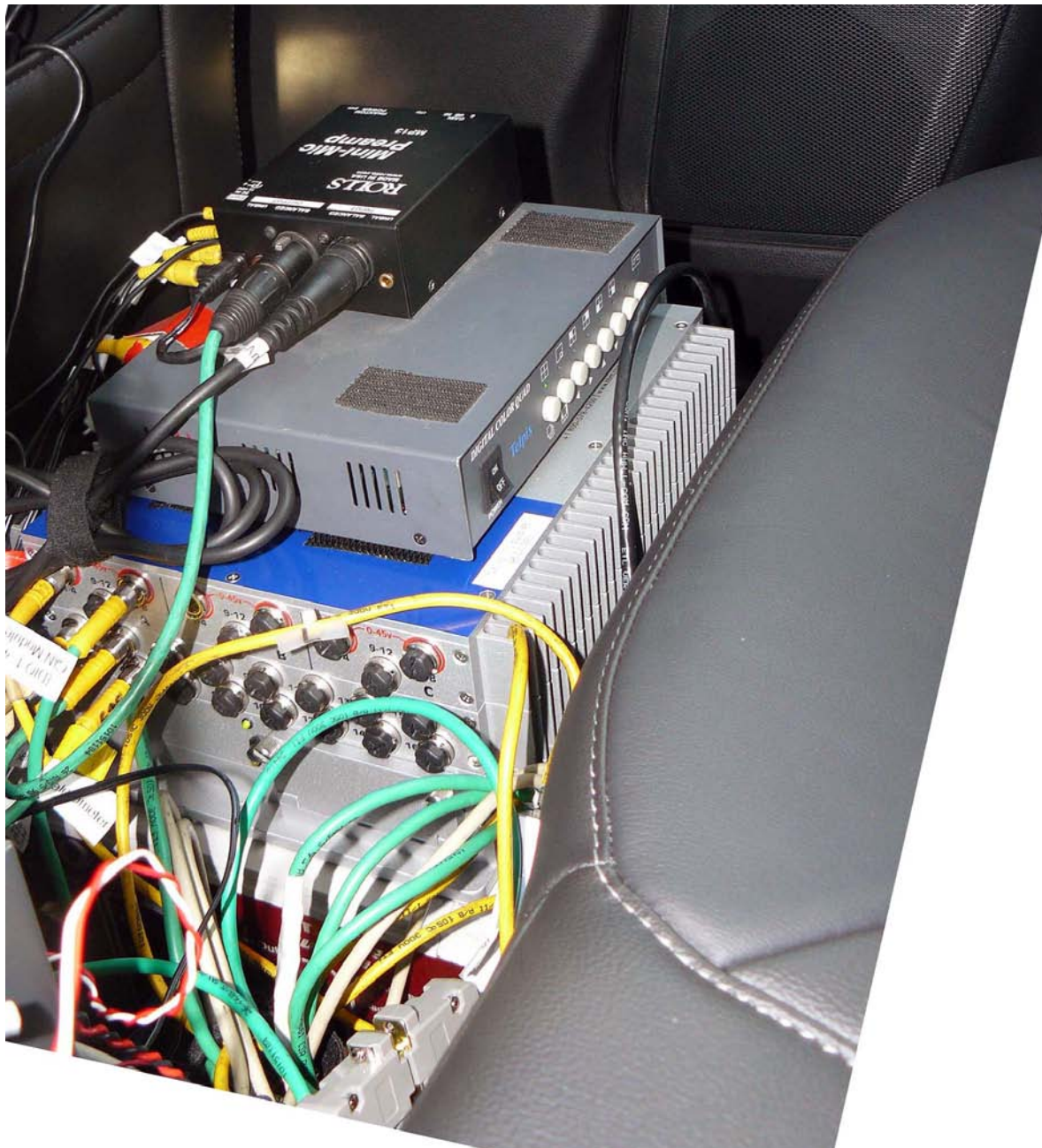
Figure A8. Data Acquisition System Installed in Subject Vehicle
