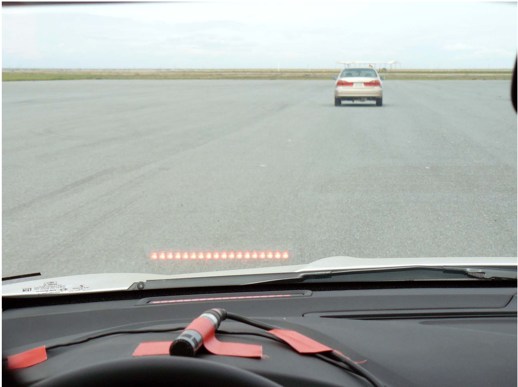
Figure A12. Visual Warning Display
