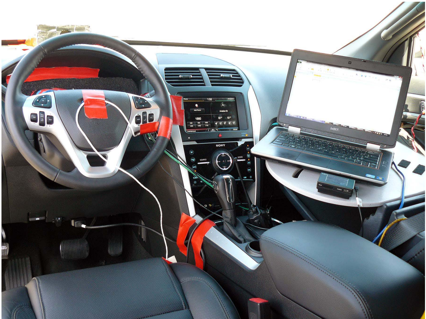
Figure A9. Computer Installed in Subject Vehicle
